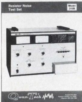
The Model 315B is designed to make resistor NOISE INDEX measurements in accordance with the recommendations of the National Bureau of Standards. (Method 308 of MIL-STD-202B). NOISE INDEX is defined as the measured ratio of microvolts of noise per volt of applied DC voltage in a decade of frequency.
