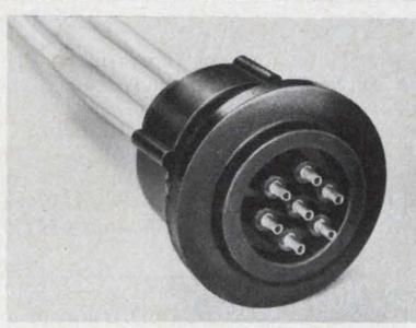
**Compact 7-Position Circular High Voltage Connector.** Military type LGH connector handles 15KVDC pin-to-pin or pin-to-ground. Can be hermetically sealed. Includes positive closure feature. Deeply recessed contacts. From the people with the most experience in high-voltage connectors. AMP Capatron Division, Elizabethtown, Pa. 17022. (717) 367-1105
