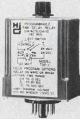
**Model TDP-1:** Each unit easily field selected for delay on make or break; for 24VDC, 24VAC, or 120VAC; and for delay ranges of 0.3 to 10, 3 to 80, or 10 to 300 seconds—adjustable to min/max of each range.
