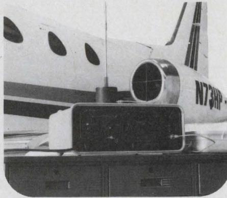
Providing AM, FM, or Pulsed RF modulation for a wide range of receiver test applications, the 8640M brings total signal generator performance to environments previously difficult for lab grade instruments.
