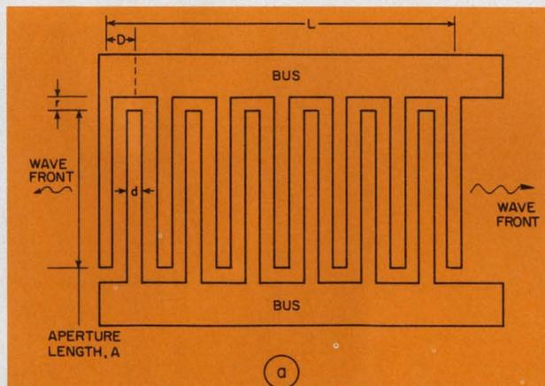
a. Excitation of the device's interdigital transducers generates acoustic surface waves that travel in two directions.
