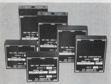
**Modular DC/DC Converters. 1.5 W to 30 W.** Miniature easy to use P.C.B. mtg. Hundreds of standard variations are available. All have low-noise filtered inputs and outputs. Inputs are reverse voltage protected. Regulated units have current limited outputs. (1 to 9) qty from \$37.25 B. H. INDUSTRIES, 5784 Venice Bl., Los Angeles, CA 90019, (213) 937-4763
