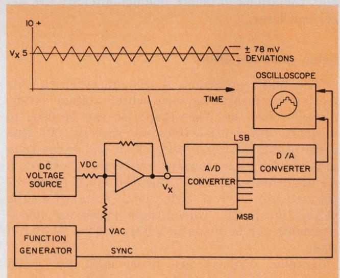
3. With a scope, you can observe and measure the switching points around a major bit, set by  $V_{dc}$ . A triangle,  $V_{ac}$ , is added to  $V_{dc}$  to exercise the LSBs around the set point. The d/a converter changes the information back to analog for display.
