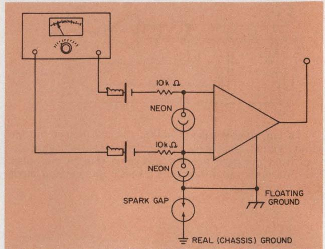
13. Hazards are posed by electrosurgery units and defibrillators, which work at kilovolt levels. Neon lamps and spark gaps protect both equipment and personnel.
