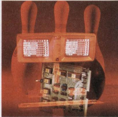
**Automatic recording of bowling scores** is done with the help of a Motorola M6800 microprocessor. Magic Score, by AMF, computes and displays individual and team scores and provides a hard copy printout at the end of a game.
