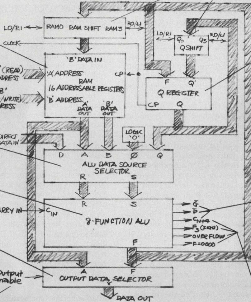
• Auxiliary register for multiply/divide, indexing, etc.
