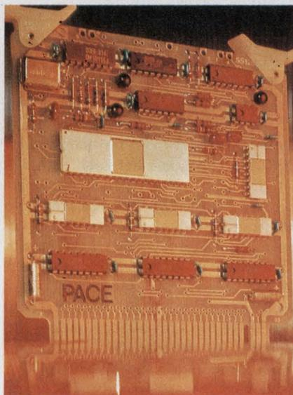
National Semiconductor's Pace microprocessor was the first 16-bit micro on a single chip. It comes in chip form, on a board with some memory (shown here) and also packaged into a prototyping system.
