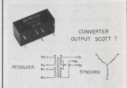
**SCOTT T. TRANSFORMER:** MAGNETICO Synchro driver is 7/8 x 1-5/8 x 11/16 high, rated at 1 volt amp., 2 arc minutes accuracy. P.N. 52155 is 5.9 sine and cosine to 11.8 v. L-L Synchro. P.N. 52156 is 5.9 sine and cosine to 90 v. L-L Synchro. MAGNETICO, 182 Morris Avenue, Holtsville, N.Y. 11742—516-654-1166.
