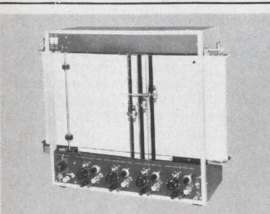
**D-73BP Three pen X-Y, Y<sub>2</sub>, Y<sub>3</sub> T Recorder** features single X-axis common to 3 electrically independent Y axes. Use as a 3-channel recorder for accurate time correlation and greatly extended duration. Sensitivity: 2, 5, 10, 50, 100, 500mV, 1, 5, 10, 50 100V/full scale. Riken Denshi Co. Ltd. 5-5-2, Yutenji, Meguro-ku, Tokyo, Japan. tel (03) 711-6656.
