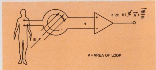
7. Loops in connecting leads should be avoided, since stray fields can couple and induce unwanted voltages into the input. Molded leads avoid the problem.
