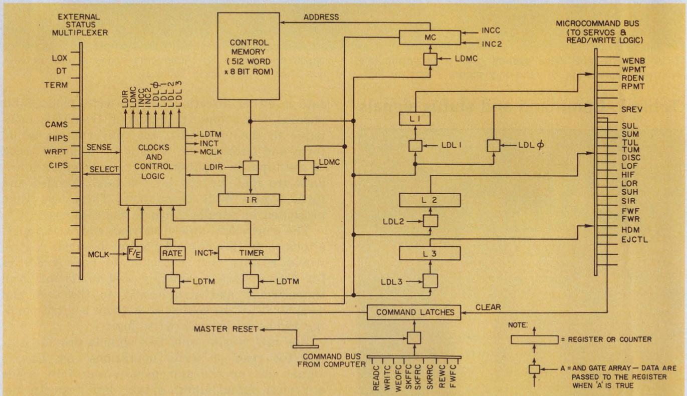
3. The major elements of the controller are a  $512 \times 8$ -bit memory, clock and control logic, and various counters
