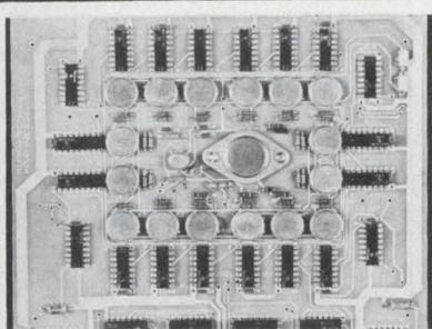
The 5 bit converter constructed on single printed circuit card. Total throughput time 50 n sec, with 20 MHz update rate. Temperature stability over full mil range,  $-55^{\circ}\text{C}$  to  $+125^{\circ}\text{C}$  with drift less than  $\pm 1$  bit over entire range. M.S. Kennedy Corp; Pickard Dr, Syracuse, NY 13211 (315) 455-7077.
