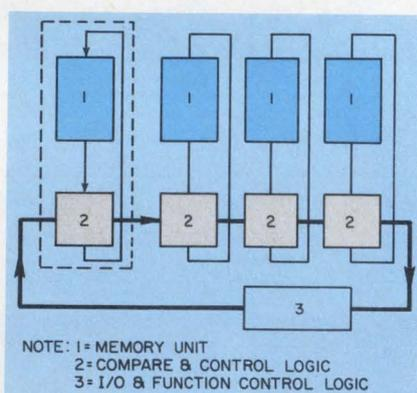
A simple arrangement for a sorting memory is shown above. A segment of the bus is extended to become a memory segment. This consists of a memory unit and the compare and control logic. An additional segment is used as the input-output unit.
