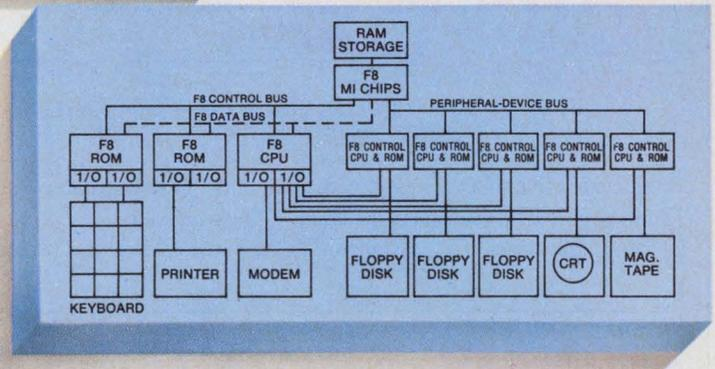
**Key-to-floppy-disk.** Multiple F8 processors are used in this key-to-floppy-disk system. Each controller consists of a CPU and a ROM. The processors are linked through a multiplexed memory channel provided by a DMA chip. This system illustrates the modular approach to expansion achievable with the F8. Because all controllers can operate simultaneously, total system throughput is increased.
