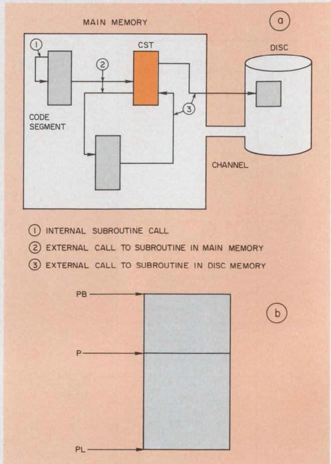
7. A code segment table (CST) keeps track of program segments in main memory (a). The stack simplifies this virtual memory operation, because program and data are separate. Three registers, PB, P and PL, protect and manage the code being executed (b).
