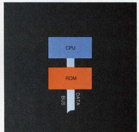
Minimal microprocessor system after the Fairchild F8.
