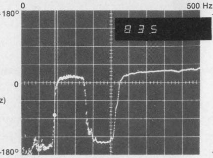
Transfer Function Phase with cursor measuring phase angle (-83.5°).
