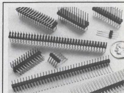
**Straight & Right-Angle Headers** provide an economical method of attaching complete matrices of .025" square posts to PC boards to serve as male contacts for interconnection systems. Available with up to 36 pins per row in several popular pin lengths, A P Products Inc., Box 110, Painesville, Ohio 44077.
