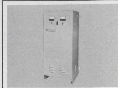
**Series "E" Electro-Pac Inverters**, designed for heavy duty operation, provide a source of highly-reliable well-regulated ( $\pm 2\%$ ) pure sinewave power from inputs of 48, 120, or 240 volts DC. ICS offers inverters from 0.5 kVA to 25 kVA, with 120, 240, 60 Hz or 50 Hz outputs. ELECTRO-PAC Div., ICS Inc. 129 Laura Dr., Addison, Ill. 60101
