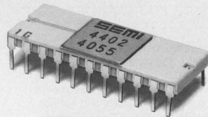
**LOW POWER:** The SEMI 4402 4K static RAM has similar power levels to
