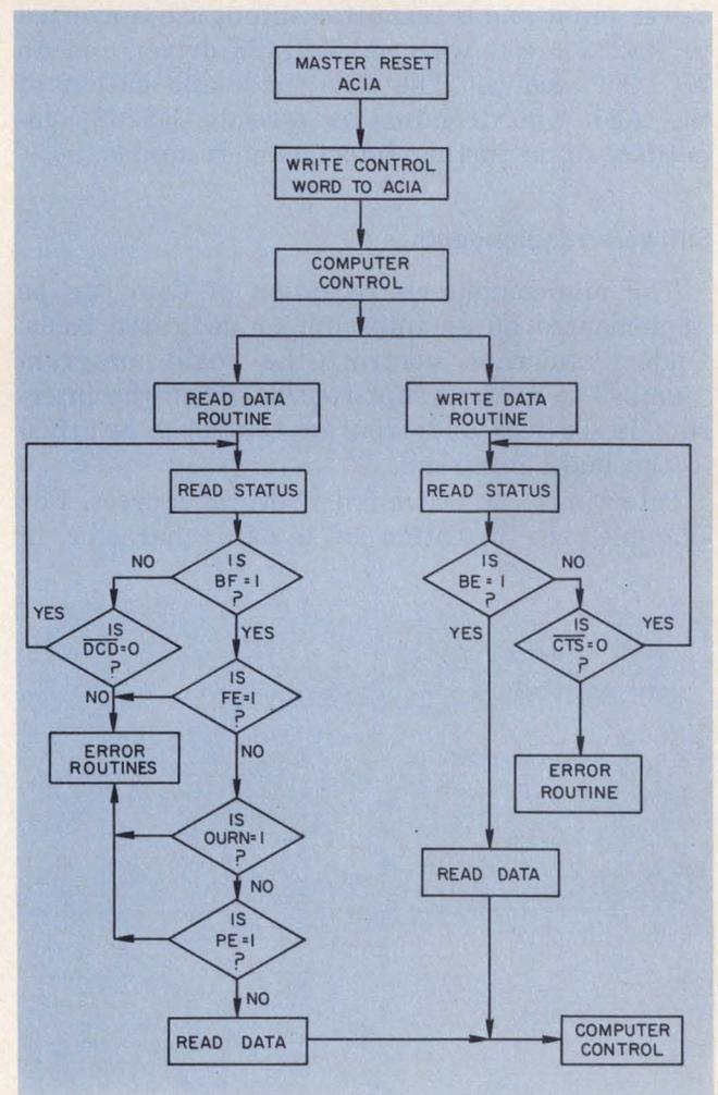
6. Read and write operations for the minicomputer are outlined with the flow diagram.
