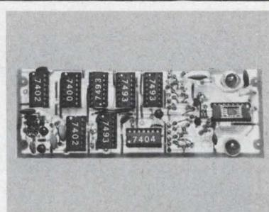
**Low Cost Image Sensing Module** contains a 1024 element (32-by-32) image sensor and all support circuitry on a single pc board. Digital video output may be displayed directly on an oscilloscope. Complete module (SE1024W) is \$150. Kit (SE1024K) is \$90. Cromemco, 26655 Laurel, Los Altos, CA 94022.
