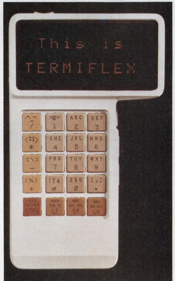
**Termiflex hand-held computer terminal** can generate all 128 ASCII characters and display them in two lines of 10 characters each. An internal 1000-character memory automatically stores incoming and outgoing data. The terminal weighs only 1.5 lb.
