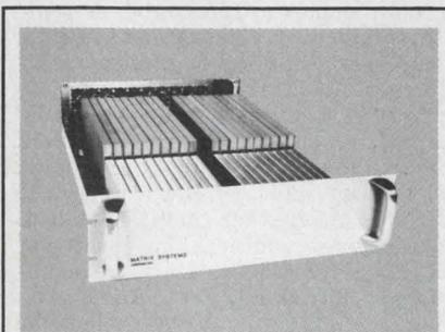
**Programmable Audio Switching System** features up to 400 Two Wire Switchpoints. It may be interconnected in nearly any configuration ie, Multipole, Multithrow, Matrix or Scanner. System may be controlled by 16 bits TTL compatible I/O Buss or 28 VDC. MATRIX SYSTEMS CORPORATION (213) 882-2008.
