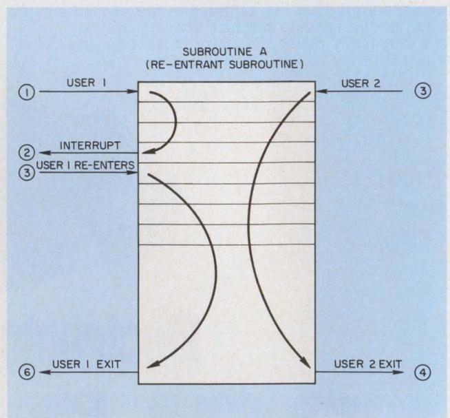
2. When several persons must use the same program, the mixture of instructions with calculated results makes for difficult bookkeeping, especially if the routine can be interrupted then re-entered.
