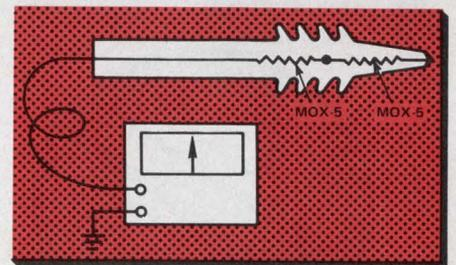
MAXI-MOX resistors have full-load drift less than 1% in 2000 hours of operation, and are available in tolerances of 1, 2, and 5% in values from 10K to 2,500M ohms. A silicone varnish conformal coating provides environmental protection while allowing a maximum hot-spot temperature of 220°C.
