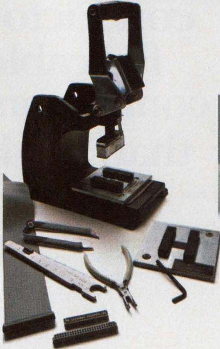
Assembly-cost savings are built in when you design a package with "Scotchflex" flat cable and connectors. But more important, 3M Company offers you the full reliability of a one-source system: cable *plus* connectors *plus* the inexpensive assembly aids that crimp the connections quickly and securely (with no special operator training required).
