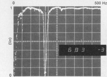
Coherence Function with cursor measuring degree of coherence ( $6.83 \times 10^{-3}$ ).
