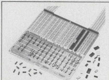
**NOVA/DCC-116** general purpose interface board provides: multiple device selection, 4 I/O registers, DMA zero word count detect, 105 socket positions for 14, 16, 24 & 40 PIN IC's. Basic board (all features of data general 4040 plus multiple device select) \$350. MDB Systems, Inc., 981 N. Main St., Orange, CA. (714) 639-7238.
