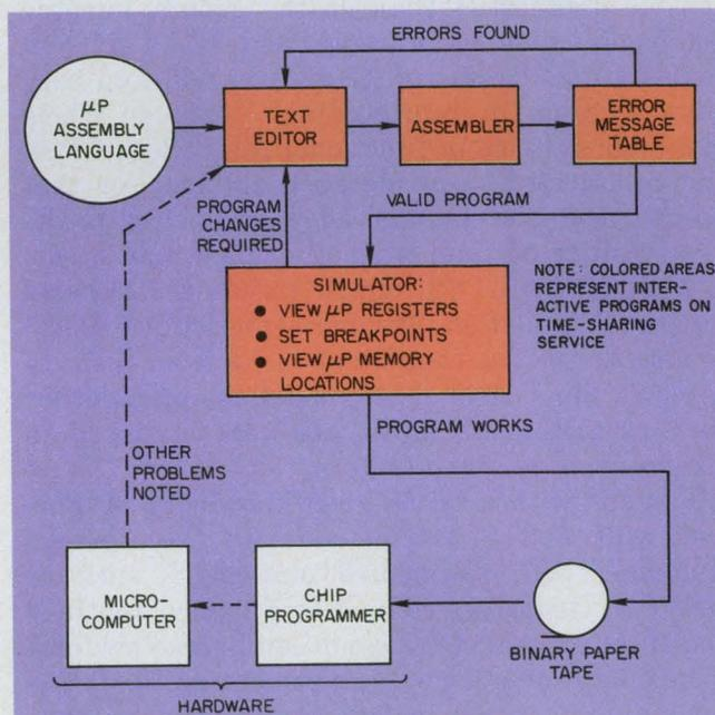
Microprocessor assembler simulators offer 60 to 80% assurance that the final product will work. These interactive programs accept microprocessor assembly language, permit editing of the text and then let you debug the software on a simulation of the microprocessor. A binary tape of a successful program is burned into PROM or ROM.
