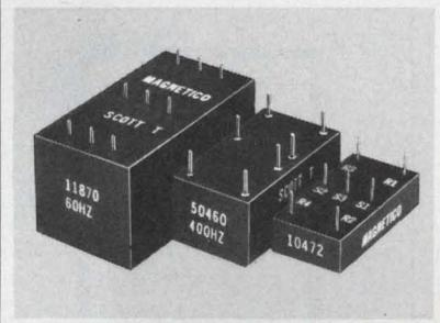
**Scott T Transformer.** 11870: 60HZ, 90v, L-L in. 1.1x2.1x1.1. 50460: 400HZ, 90v, L-L in. 7/8x1-5/8 x11/16. 50642: 400HZ, 11.8v, L-L in. 7/8x1-5/8-11/16. 10472: 400-HZ, 11.8v, L-L in. 3/4x1-1/2x3/8. All with 6v RMS sine & cosine output. MAGNETICO, INC., 182 Morris Ave, Holtsville, N.Y. 11742 516-654-1166.
