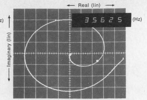
Nyquist diagram of transfer function real vs. imaginary with cursor dot measuring frequency.
