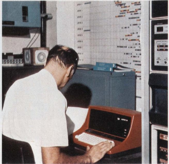
An instant check on baggage handled by the automated system at Eastern Airlines' Miami Terminal is made at the computer. The DEC computer, laser optical readers and conveyors are linked in this Bendix system. The optical baggage tag is a coded bullseye.
