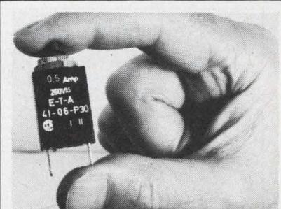
**Overcurrent Protector**, manual reset eliminates fuse replacement. Convenient panel mounting. 15 fractional ratings from 0.1 to 3 amp. Other models up to 400 amp. Trip-free and fool-proof, UL and CSA approved. High quality, low cost \$1.29 ea. in 1000 lots. E-T-A Products Co. of America, 7400 N. Cromame Rd., Chicago, Ill. 60648. Tel: (312) 647-8303. Telex: 253780.
