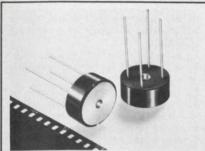
**3/4" Diam 10 amp Bridge Rectifiers** from Tarzian with heat dissipating aluminum base. 240 amp surge rating. Heat dissipation is 25W@10A. Max case temp is 150° C. H-FB Series supplied as standard avalanche, fast recovery or with special terminals. Sarkes Tarzian, Inc., Semiconductor Div., 415 College Ave., Bloomington, Ind. 47401, 812-332-1435.
