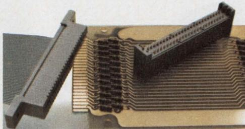
trimming the cable after assembly.
