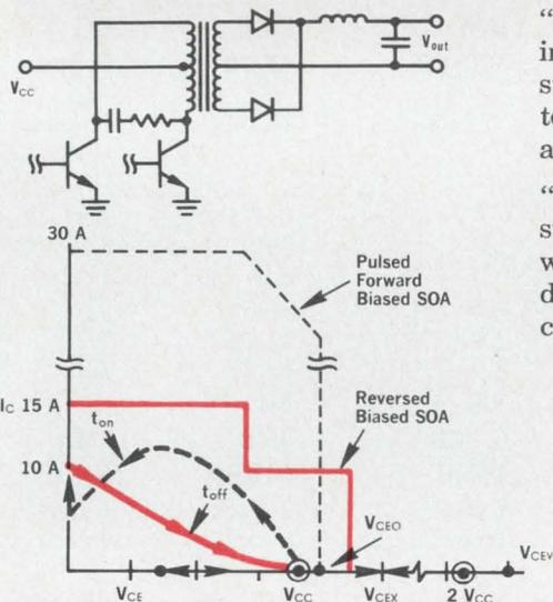
“... both blocking voltage and sustaining voltage are important in switch-mode applications. The circuit illustrated requires high blocking capability since the transistor is subjected to a substantially higher voltage than  $V_{CC}$  after turn-off . . .”
