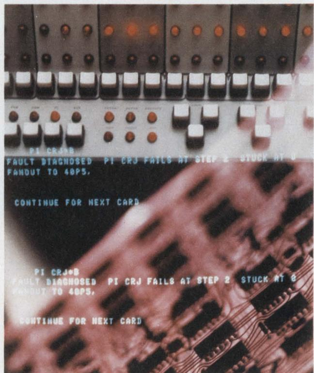
**Diagnosis by computer:** Teradyne's L100 automatic test system checks arithmetic boards for the company's M365 computing controller, and it pinpoints any faults.
