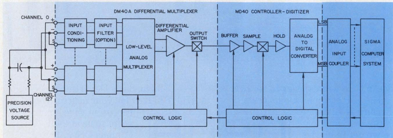
1. To check out a data-acquisition unit, set up a simulated system configuration and apply a precision voltage
