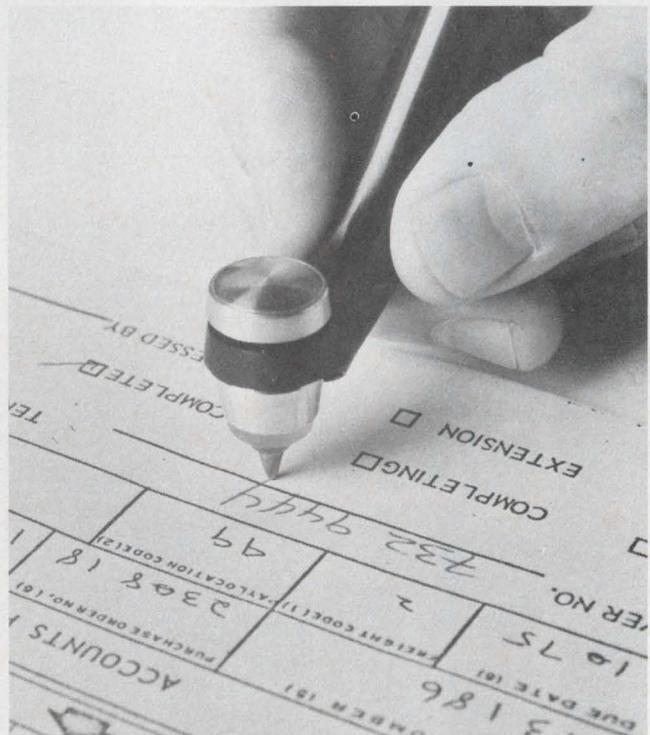
Written data can be entered directly into a computer with the Alphabec 75 ASCII pen from Xebec Systems. Sensors in the head of the pen determine the direction of motion and produce signals that are used to identify the number being written.
