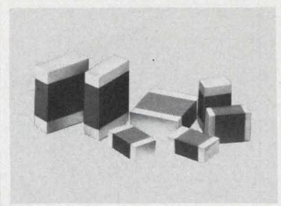
**HIGH Q MULTILAYER CAPACITORS** feature very high quality factors at microwave frequencies. Offered in three standard sizes: .050 x .040, .080 x .050, .125 x .095. Capacitance values from 0.1 pf to 1000 pf with close tolerance and voltages to 1000 VDCW. Johanson/Monolithic Dielectrics Div., Box 6456, Burbank, Ca. 91510, (213) 848-4465.
