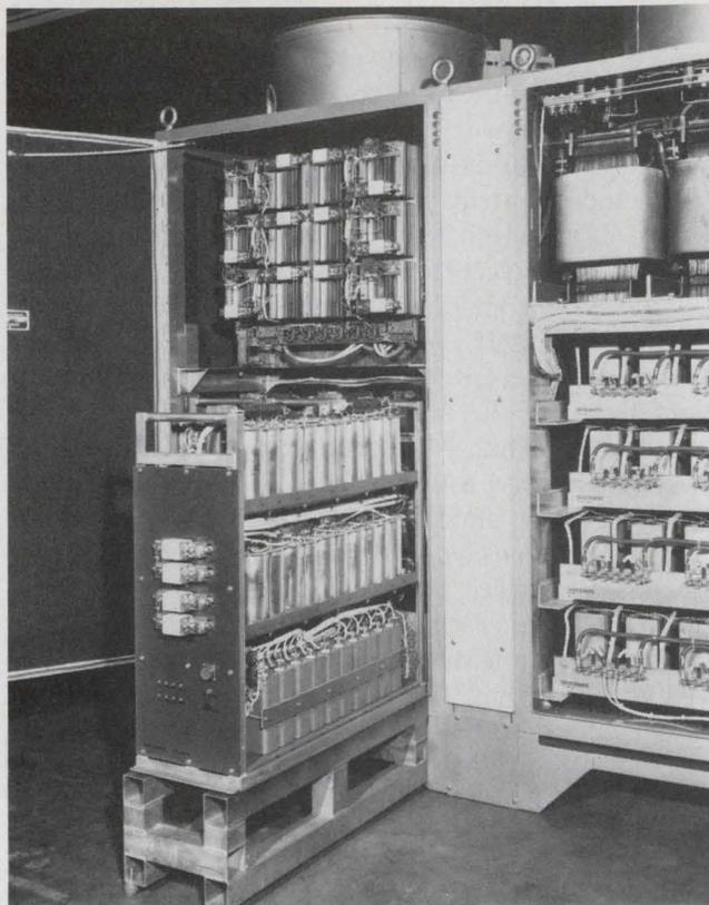
**Massive power source on wheels:** one of three Teledyne Inlet inverter switching sections, mounted on rollers for maintenance convenience.
