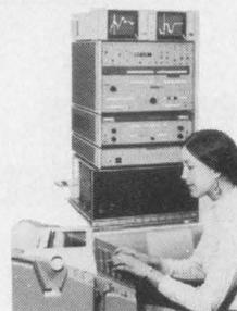
FFT Analyzer with add-on mini-computer for post-processing.
