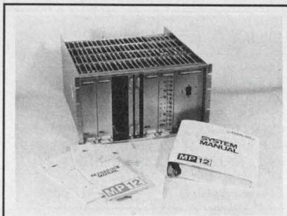
**MP12 Small Computer System.** Configure your own application system with 4k MP12 CPU with programmed I/O, interrupts, DMA. Interface cards for teletype, modems, floppy disk, paper tape, A/D, printer, card reader, mag. tape. Real-time operating system, full supporting software. Fabri-Tek, Inc. 5901 S. Cnty. Rd. 18, Mpls, MN 55436 (612) 935-8811
