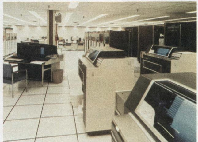
Service centers with multiple computer systems form the backbone of Control Data's Cybernet. The computer network offers time-sharing access to design programs on user terminals, as well as allowing user computers to augment their processing power with the network.
