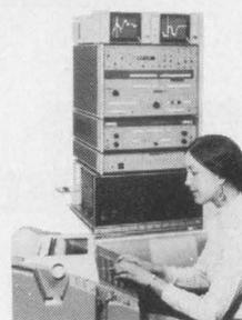
FFT Analyzer with add-on mini-computer for post-processing.
