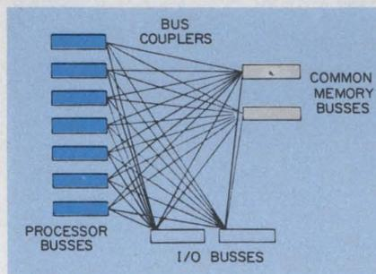
In the Pluribus multiprocessor architecture a novel feature is treatment of all processors as equal units. The hardware is joined together by special bus couplers that permit units on one bus to access those in another.
