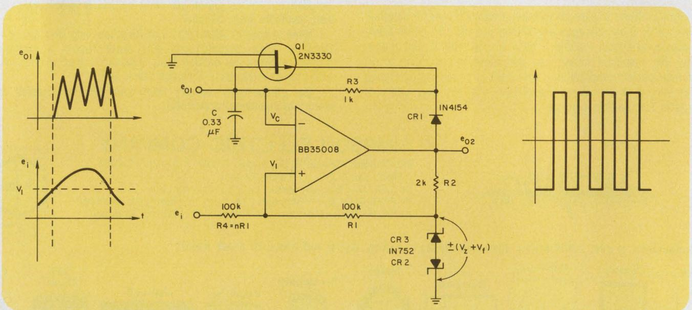
Voltage comparator generates an audio-alarm output when an input signal exceeds the CR<sub>2</sub> and CR<sub>3</sub> voltage.
