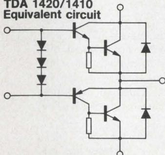
The TDA 1420 integrates a quasi-complementary (NPN/PNP) darlington pair and biasing diodes for perfect electrothermal matching. Applications for this versatile power IC include DC or stepping motor drivers, op amp power boosters, audio output stages, etc.
