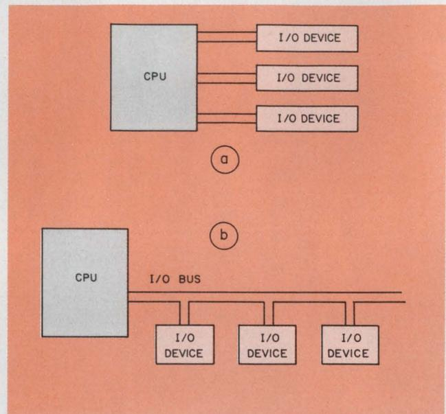
1. **I/O bus structures employ several schemes.** A radial system is the simplest, but it limits the number of I/O units (a). A party-line system reduces the number of lines needed for a distributed system (b). The latter system also comes in a daisy-chain version, which connects devices serially.
