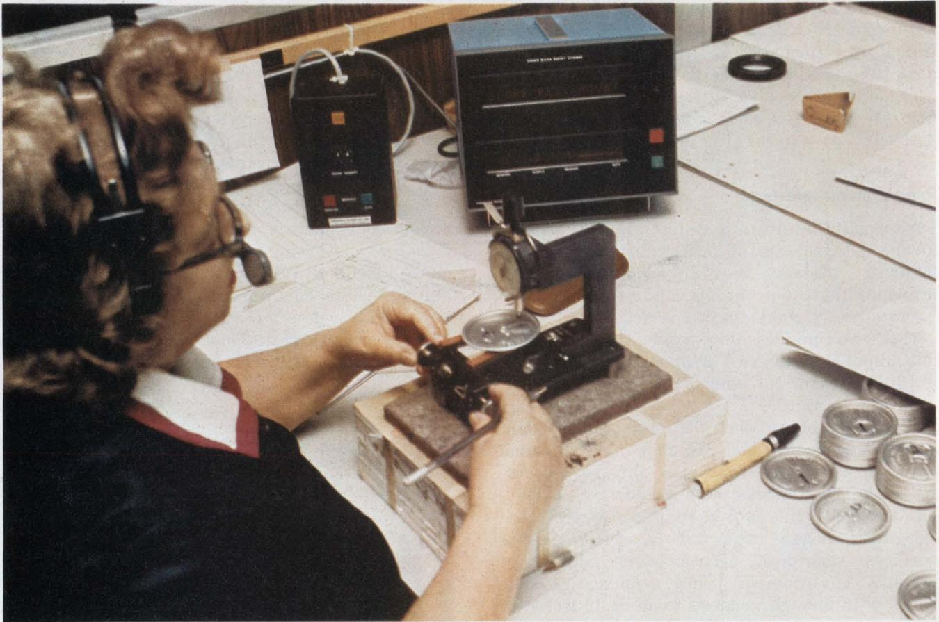
Voice-input systems are being used at Continental Can Co. to enter quality-control data into computers. An inspector makes several measurements on pull-top lids
