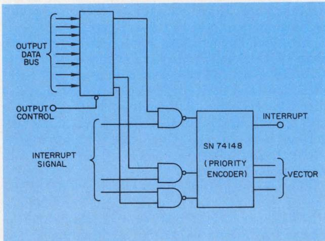
4. Either an enable/disable function or a priority structure can be obtained readily for a microprocessor that has neither. A conventional input port can be used to control the interrupt input.
