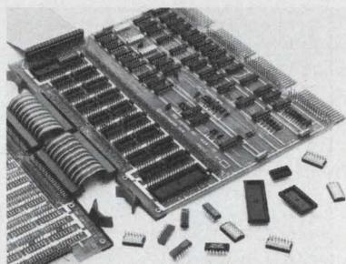
**PDP-11 General Purpose Interface.** The MDB-11C provides all features of a DEC DR11C plus additional 16 bit register, 4 selectable interrupt control levels, 16 decoded device addresses, takes only one quad slot, has maximum Unibus load of 1. Also, 20 wirewrap positions are provided. \$390. MDB Systems, Inc., 981 N. Main Street, Orange, CA 92667.
