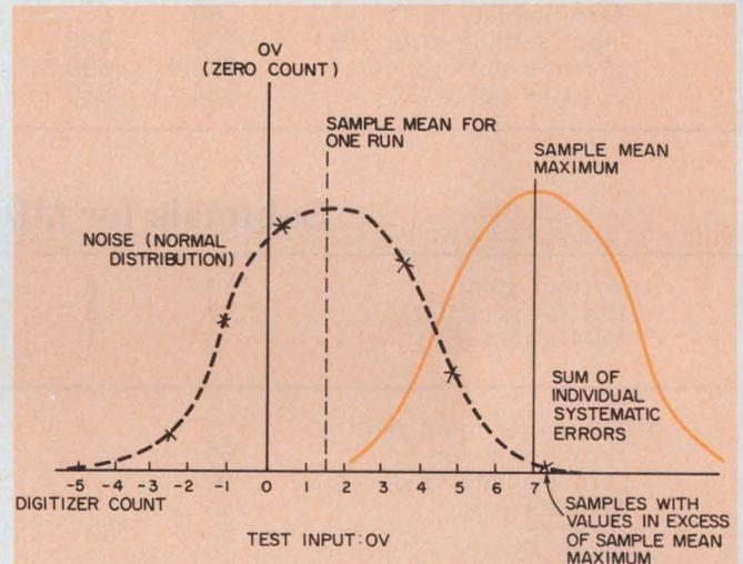
2. Performance capability is bounded by two main factors: cumulative systematic errors and random electrical noise. The computer calculates the mean and standard deviation to compare with calculated values.
