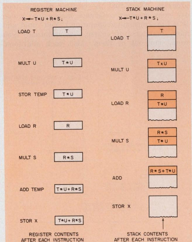
4. A stack machine has virtually an unlimited number of addresses, but a register machine must store to temporary locations.
