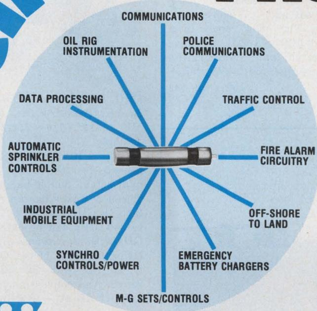
Protect your solid state equipment from junction damage caused by high-current surges due to power switching and lightning transient induction. Ordinary protective devices ground only one wire, allowing currents to reach your equipment through the "other" wire. TII 3-Electrode Gas Tube Surge Arresters simultaneously ground both wires of a signal or power pair. TII protection can end unnecessary service calls and customer complaints. To learn more about surge and how to
