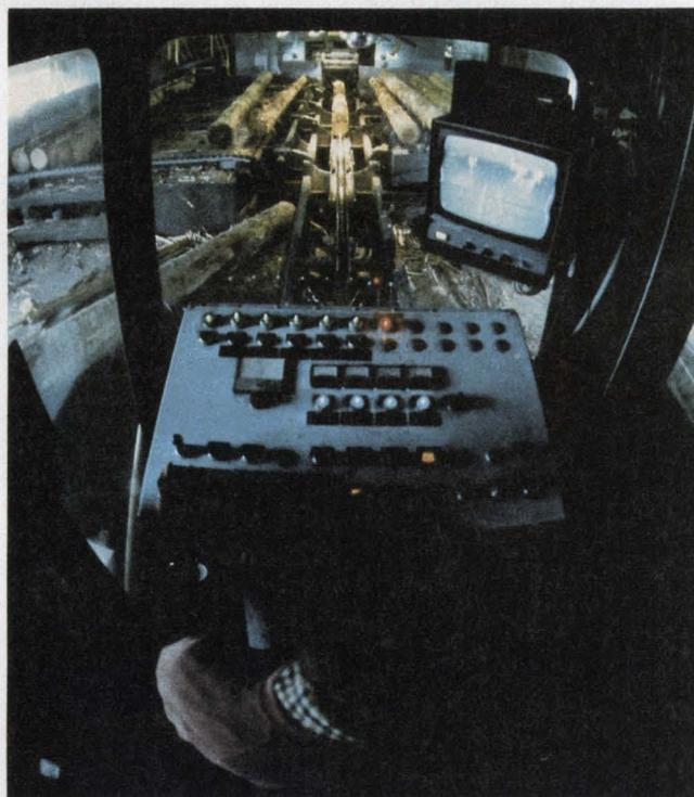
As logs are measured in a sawmill, a PDP-8 tells an operator of a four-blade saw which sizes and lengths to select to get the maximum yield of usable lumber.
