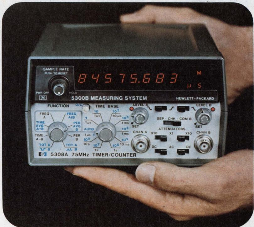
HP's new 75 MHz Timer/Counter is easily held in your hands. Take a look at the front panel: Never before has there been so much counting capability in such a small package at such a small price. Seven other modules snap on to convert to other instruments — including a DMM — or to connect to the HP Interface Bus.
