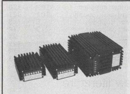
**Logic and Linear DC Supplies** available with single and multiple outputs ranging from 5V to 28V and currents to 25A. Line reg. is 0.05%, load reg. 0.1%. Features Internal OVP (STD on 5V), current fold-back, floating outputs. 220VAC input optional. 16 models in stock. Modular Power Inc., 4818 Ronson Ct. San Diego, CA 92111 (714) 279-1641
