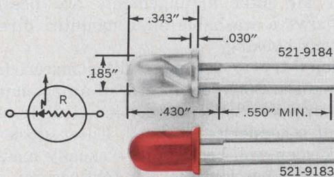
Available in red or clear LED packages with or without a built-in current limiting resistor. Red LED is also made without resistor. Suitable for circuit status indication, alpha-numeric displays and visual indicators. Features long wire-wrappable leads. IC compatible with solid state reliability. High luminous intensity, low power consumption, low cost.
