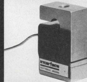
■ The inexpensive Super-Mini Load Cell from Interface offers guaranteed specifications of ±0.03% non-linearity, ±0.02% hysteresis, and ±0.01% non-repeatability. That's not all! The Super-Mini is available in standard ranges of 0 to ±50, ±100,
