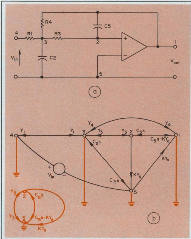
4. Ground the nodes that form paths between input and output to obtain numerator subgraphs. The circuit (a) is a multiple-feedback active filter and (b) its topological equivalent. A path subgraph is shown at bottom left.
