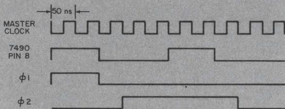
1. In a clock generator for the 8080 microprocessor, a 20-MHz crystal-oscillator signal is divided by 5 and then by 2 to obtain the two phases for its output.
