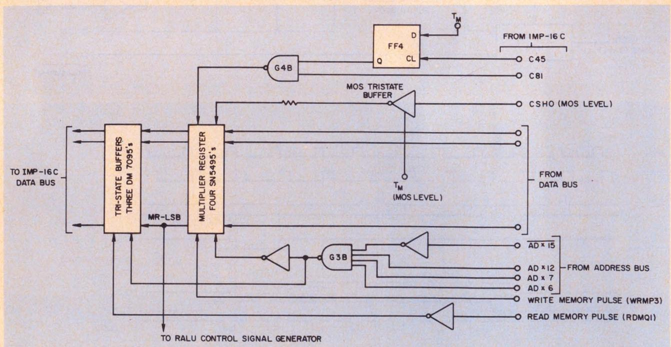
4. The external multiplier register first stores the multiplier operand, then shifts it right 1 bit per microcycle, and then injects the least-significant partial product bits.
