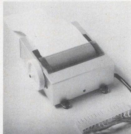
Readout from electronic calculators, instrumentation, cash registers and computers is printed electrostatically by Panasonic's nonimpact printer.
