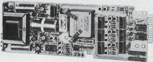
The SN Digital Interface Card accepts your data input on parallel lines, strobed for noise immunity, and stores the data in a buffer register. For isolation, the program is transferred across optical couplers so that your digital signal and the power supply it controls can be up to 1000V apart. The five types of SN Cards offer a choice of BCD or complementary binary programming.
