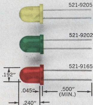
Now available in green, yellow and red. Mini-sized for maximum front panel density and easy panel mounting. High luminous intensity, low cost. Vibration/shock resistant. Solid state for long life. Wide viewing angles. Ideal for applications like panel lighting, film annotation and alpha-numeric displays.
