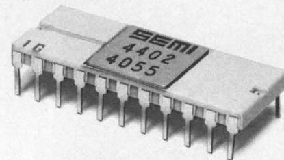
**PERFORMANCE TESTED:** Like all SEMI NMOS components, the 4402 4K static RAM must meet our own tough test standards, since we use it in our memory systems — for example the MICRORAM 3400N. With our reputation riding on its performance, you may be sure the acceptance standards are high indeed. In fact we 100% ac and dc test our components twice — at wafer and again in the package.
