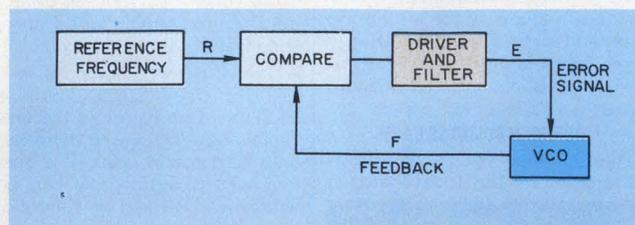
1. A conventional phase-locked loop makes the VCO frequency track that of a reference. For use with motor control, the VCO block is replaced by a motor-tachometer; comparator operation is not changed.
