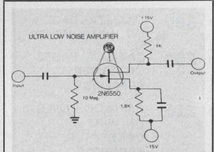
**Ultra Low Noise Fet None quieter**— $2nV/\sqrt{Hz}$  at 1 kHz—our 2N6550 silicon N-Channel junction FET gives highest  $G_M$  available, improved  $A_v$ , high  $I_{DSS}$  within a 10-250mA range and low output impedance. "Data in short transistor catalog." Samples. Prices: 100-999, \$10. Teledyne Crystalonics, 147 Sherman St., Cambridge, MA 02140. (617) 491-1670
