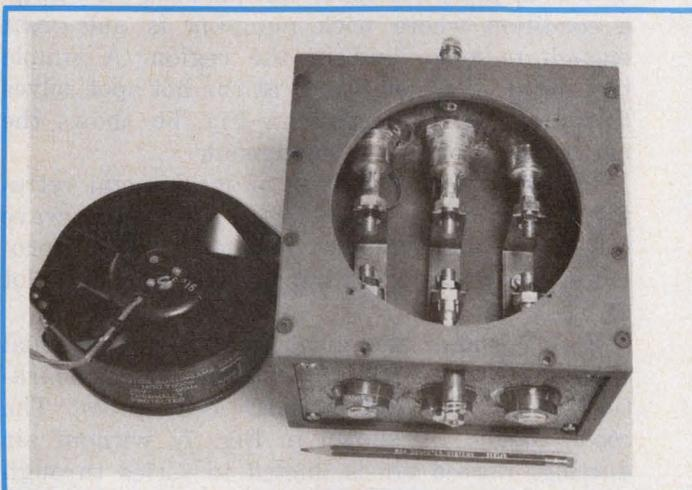
3. In this three-phase, full-wave power-rectifier assembly, six power diodes are mounted on panels that provide low thermal resistance to the cooling air. A half-wave unit would need only three diodes and a single panel.
