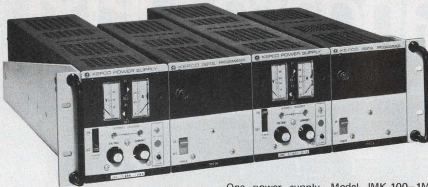
One power supply, Model JMK 100-1M produces 0-100 volts controlled in 12-bit binary; and 0-1 ampere controlled in 8-bit binary. The other unit, Model JMK 15-6M produces 0-15 volts controlled in 3-digit BCD; and 0-6 amperes controlled in 2-digit
