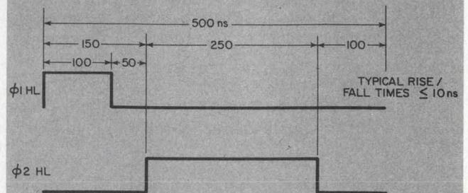
2. A driver circuit converts TTL-level signals to a high level—zero to +12 V—to drive the microprocessor.
