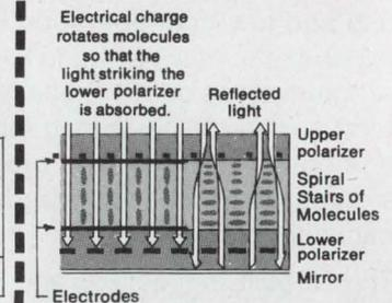
**A few limitations.** LCD's have limitations too. Operating temperature range is one. Liquid crystals slow down and may even cease to function at temperatures below 0°C. Above 50-60°C, crystals go into solution and will not function properly. But extremes do not damage LCD's. Once the temperature returns to normal, operation is automatically resumed.
