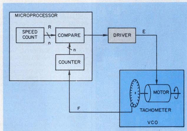
2. A microcomputer furnishes the speed reference and also performs phase and frequency comparisons under program control. Motor inertia provides the necessary loop filter.
