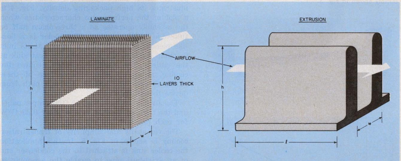
2. The cooling surface of a laminated panel is at least six times greater than that provided by an extruded fin
