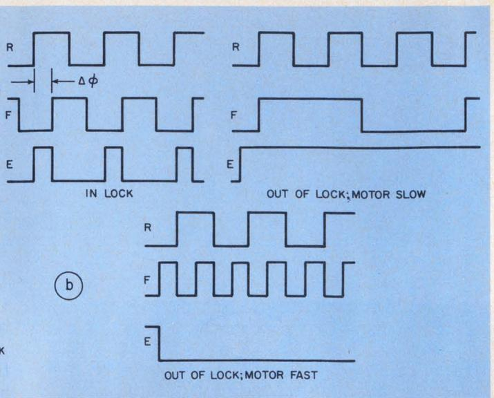
4. The microcomputer driven by an interrupt (a) at the leading edges of R computes the pulse-width-modulated control (b). The internal crystal provides all system timing. The phase angle is measured between the leading edges of R and F.
