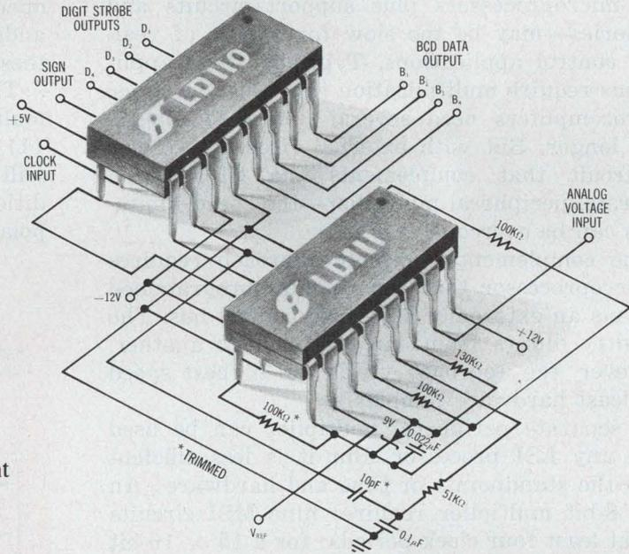
The unique conversion technique uses a single reference and a single full-scale adjustment to achieve a highly-accurate strobed 3½-digit output of up to 3100 counts plus sign. LD111 analog processor employs monolithic PMOS/bipolar construction and interfaces directly with the LD110 digital processor, which has a monolithic PMOS structure. For further information
