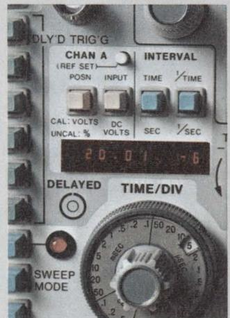
dial settings, automatically computes time intervals and voltage levels, converts time measurements to frequency, and calculates percent. It even signals if you make an erroneous setting. In addition, the microprocessor drives a 3½-digit LED display to give you a direct digital read-
