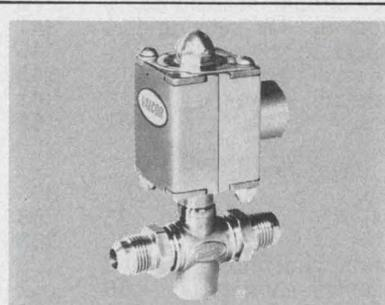
**Cryogenic Solenoid Valves.** New all stainless steel construction. Unique design provides high flow, long life and extreme reliability at temperatures down to  $-423^{\circ}F$ . All joints heliarc welded. Metal to metal seating. Coil suitable for 50,000 hours of operation. Valcor Engineering Corp., 5382 Carnegie Ave., Kenilworth, N.J. 07033 (201) 245-1665.
