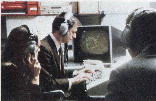
**Synthetic speech** is being produced with 1/50th the previously required digital information. The digital coding scheme developed at Bell Laboratories is ideal for transmission over a fiber-optic link. The screen shows a graphic representation of synthetic speech.
