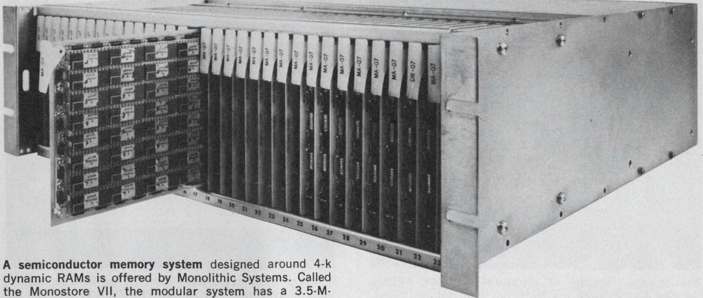
A semiconductor memory system designed around 4-k dynamic RAMs is offered by Monolithic Systems. Called the Monostore VII, the modular system has a 3.5-M-bit capacity, and it contains the peripheral circuitry needed by the RAM chips.
