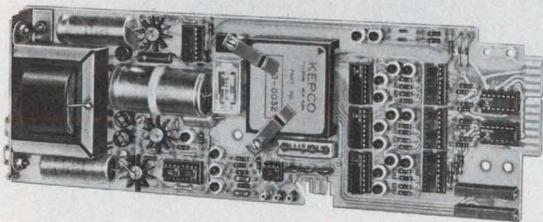
The SN Digital Interface Card accepts your data input on parallel lines, strobed for noise immunity, and stores the data in a buffer register. For isolation, the program is transferred across optical couplers so that your digital signal and the power supply it controls can be up to 1000V apart. The five SN Cards offer a choice of BCD or complementary binary programming.
