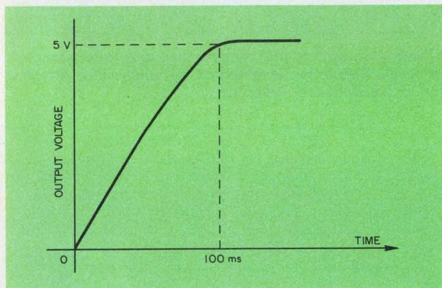
6. Output voltage is "delayed" by limiting of the thermistors until all bias and drive signals are established. Normal operation then begins.
