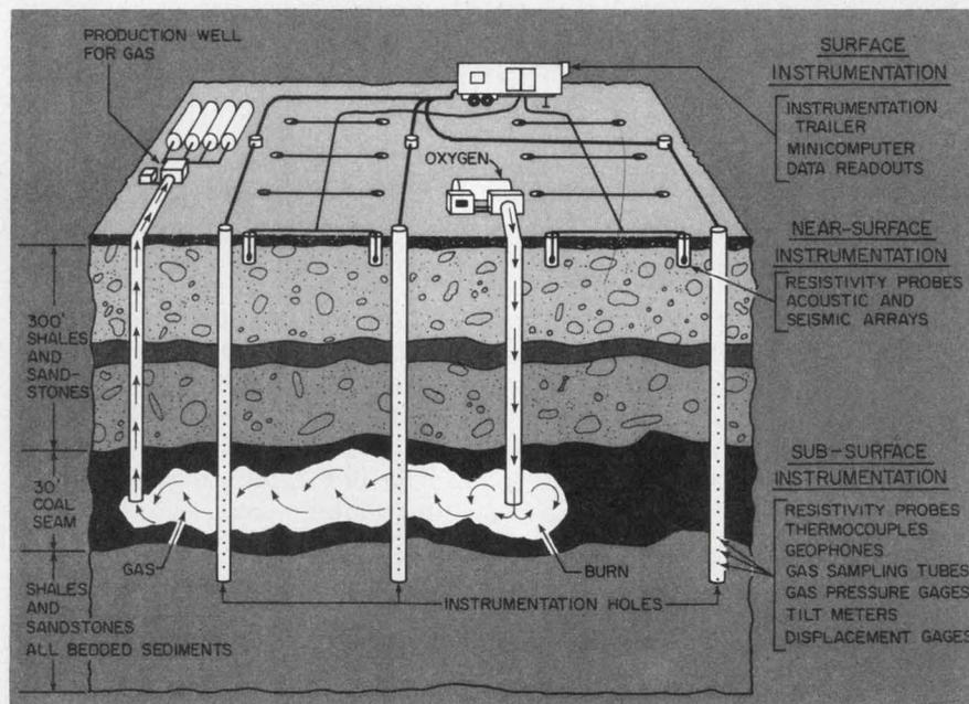
Near-surface instrumentation alone will ultimately monitor burning coal hundreds of feet below the earth's surface in an attempt to generate electricity. Initial tests, however, will require instruments near the burning coal, so the actual performance of the remote sensors can be accurately evaluated.
