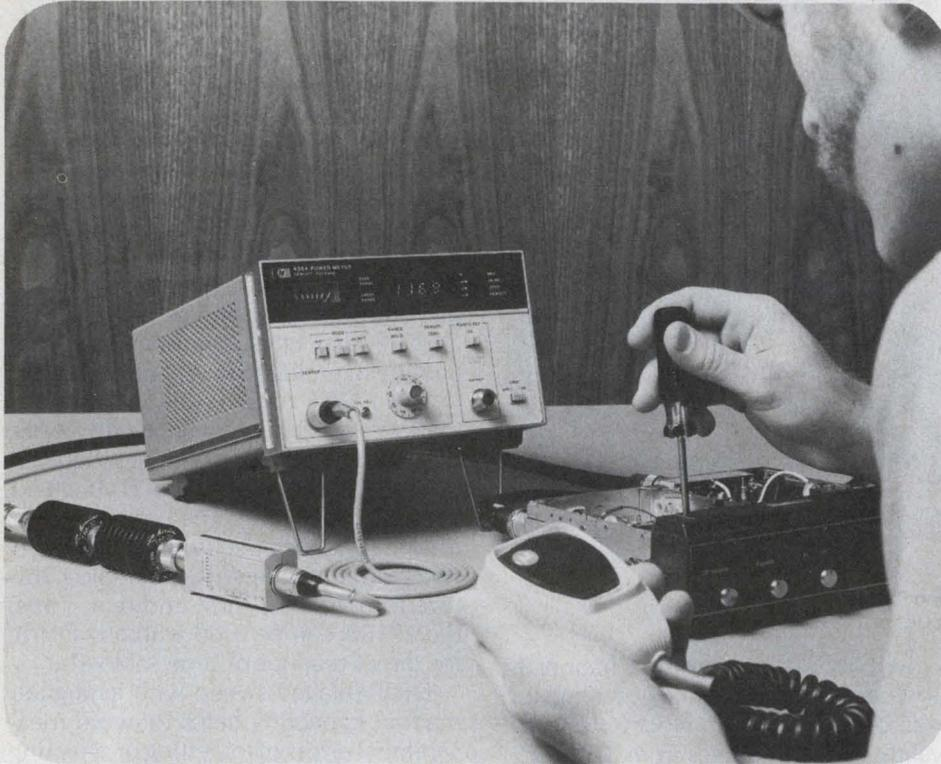
A new digital microwave power meter, the HP 436A, has built-in firmware 'intelligence' to switch automatically among its five power ranges, to translate its reading into watts, dBm or dB Relative, to recognize which of several possible sensors is connected and calibrate its display accordingly, and to locate the displayed decimal correctly.
