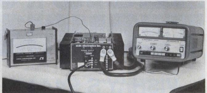
Core temperature is easy to measure with a thermocouple attached to the capacitor's positive terminal.
