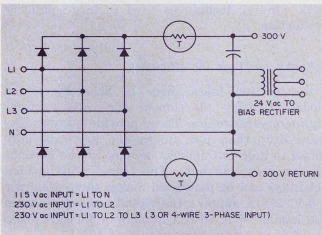
2. A three-phase bridge rectifies the input, which can be 115 or 230 V, single or three-phase. The thermistors limit line-inrush current.
