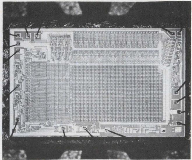
A field-programmable ROM from Harris Semiconductor, the company that introduced PROMs, has a 1024-bit capacity. The PROM features access time of 50 ns.
