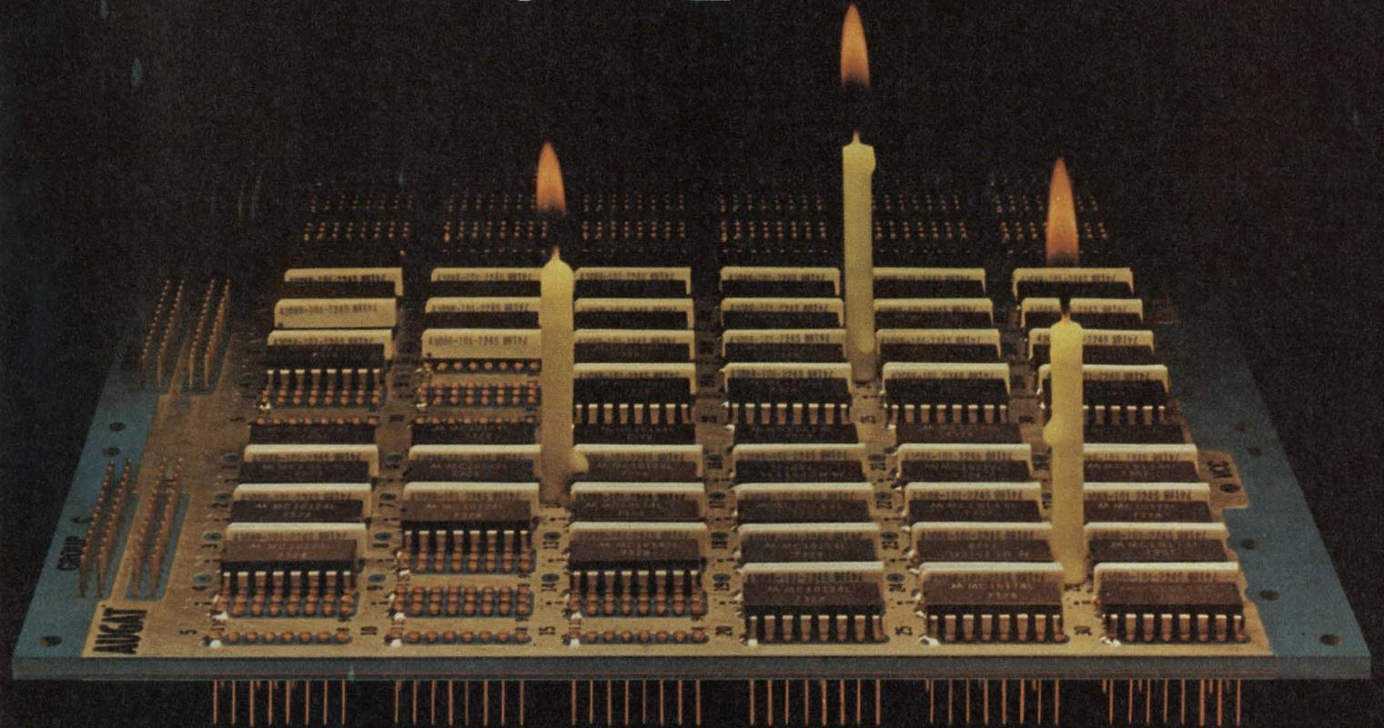
Augat ECL Board with -2 volt bus for terminating single in-line package (SIP) resistor network.
