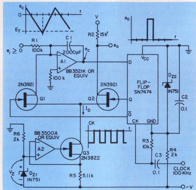
6. If clocked control of the discharge time is used, accuracies to within 0.01% are obtainable.
