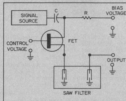
achieved by use of a system made up of several transducers, each of which receives the input signal via a separate FET. The frequency response is shaped by adjustment of the phase relationships of control voltages applied to the transistor gates. A single wideband trans-
