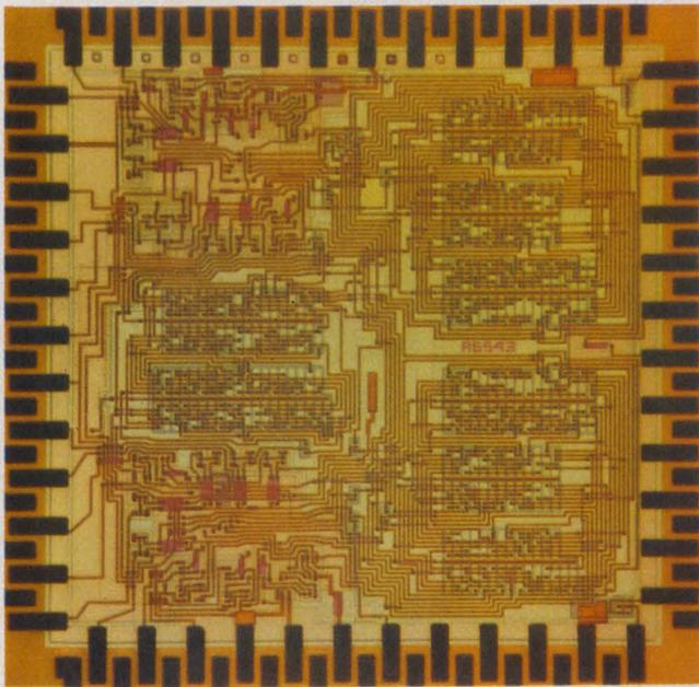
Random logic I<sup>2</sup>L array fabricated by Bell Laboratories has the equivalent of 256 gates on it.
