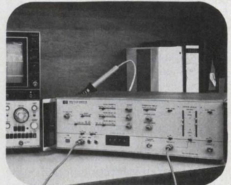
Pulse burst is generated upon receipt of trigger pulse. Length is determined by thumbwheel switches.
