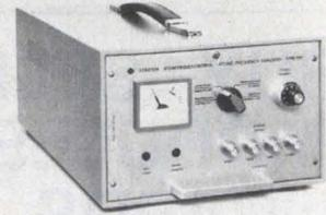
**Atomic Frequency Standard Model FRT for Lab/Field.** Output 10-5-1 0.1 MHz, Short Term Stability  $< 1 \times 10^{-11}$ ,  $\tau = 1s$ ,  $< 1 \times 10^{-12}$   $\tau = 100s$ . Drift typ  $1 \times 10^{-11}/M$ . Coupled with Receiver-Controller EFR. Sync to Standard Freq absolute freq parts in  $10^{12}$ . Efratom Calif., Inc., 3303 Harbor Blvd., E1, Costa Mesa, Ca. 92626 (714-556-1620)
