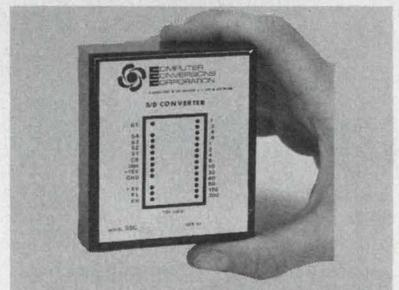
**SYNCHRO TO BCD CONVERTERS:** 3 or 4 decade, unipolar or bipolar output adjustable scale factor,  $\pm 6$  or  $\pm 30$  minute accuracy, 60 or 400 Hz input, zero offset adjustment, module 2.6 x 3.1 x .82" H. Unit price from \$395/ea. Computer Conversions Corp. East Northport, N.Y. 11731 (516) 261-3300
