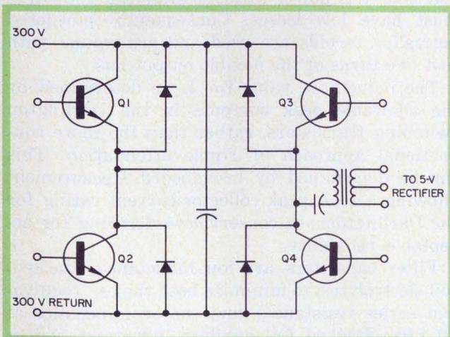
3. Darlington transistors in a bridge arrangement switch the 300-V bus. Transistors  $Q_1$  and  $Q_4$  conduct simultaneously for half the cycle, while  $Q_2$  and  $Q_3$  are cut off. The situation reverses on the second half cycle.
