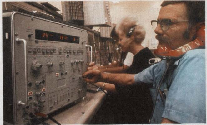
The use of telephone voice channels for digital data transmission requires special line quality measurements. This Hewlett-Packard 4940A Transmission Impairment Measuring Set separates and simultaneously measures six types of transient line disturbances.
