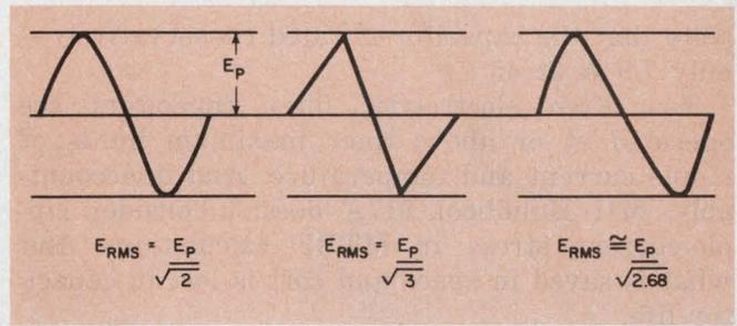
2. The approximate rms value of ripple current can be calculated from the current's peak value and a constant determined from the waveshape.
