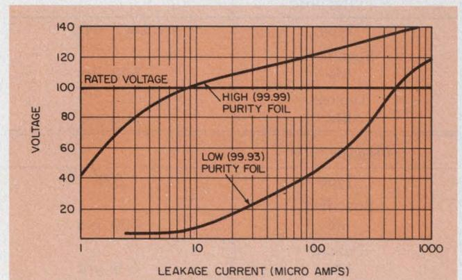
5. Leakage current is strongly affected by the purity of the aluminum foil used in manufacture.
