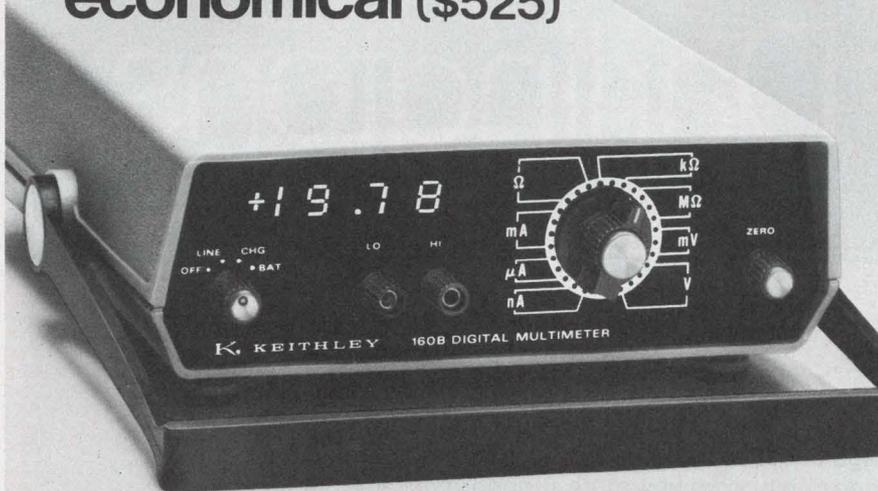
**The Model 160B.** It's the epitome of a DMM for scientific and engineering labs. Sensitivities down to 1 microvolt, 10 picoamps, and 1 milliohm are founded on Keithley's lifetime of expertise in designing and building low-level instrumentation.
