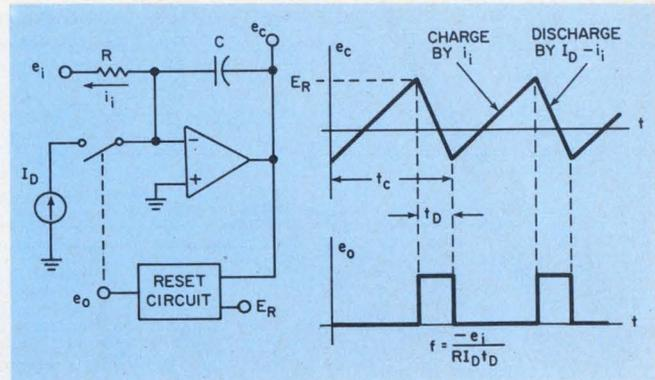
4. Controlled-charge reset circuits eliminate the linearity error caused by a separate reset interval.
