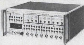
**Unique New Programmable Generator** features multiple function capability. Program as digital pulse or word generator. Programmable time from 50ns to .999 sec. External trigger, 8 or 16 output channels, ROM option, computer interface, expandable memory. Interface Technology, 627 Fremont Ave, South Pasadena, CA 91030 (213) 682-3705
