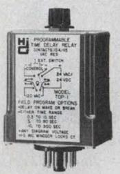
**Model TDP-1:** Each unit easily field selected for delay on make or break; for 24VDC, 24VAC, or 120VAC; and for delay ranges of 0.3 to 10, 3 to 80, or 10 to 300 seconds—adjustable to min/max of each range.
