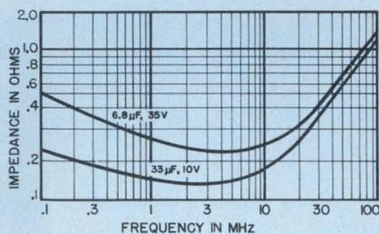
Dual in-line plastic package for mechanical protection and increased reliability. Preferred ratings are 6.8  $\mu\text{F}$  @ 35 V, 15  $\mu\text{F}$  @ 20 V, 22  $\mu\text{F}$  @ 15 V, and 33  $\mu\text{F}$  @ 10 V. Operating temperature range,  $-55\text{C}$  to  $+85\text{C}$ .
