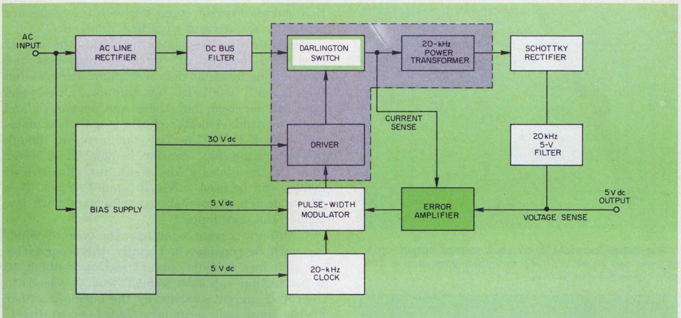
1. In an unusual approach to power-supply design, the ac input is first converted to a 300-V unregulated dc bus. The high voltage is then chopped at 20 kHz by
