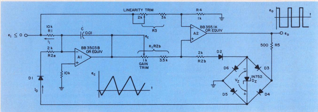
5. A 10,000:1 dynamic range and accuracy of 0.04% are obtained when controlled-charge reset is used.
