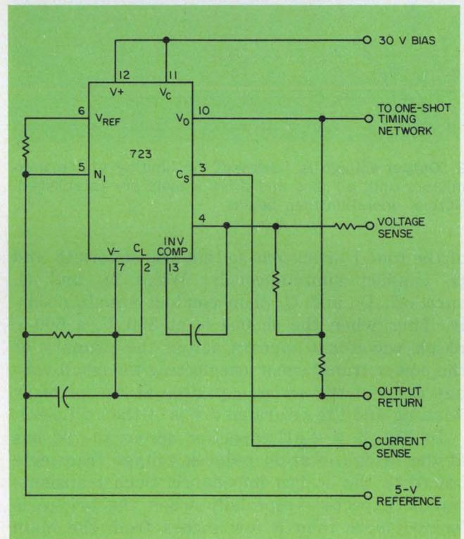
4. Both output voltage and current are sampled and generate an error signal in a 723 regulator. The error signal modulates the pulse width of a one-shot multivibrator to provide the voltage regulation.
