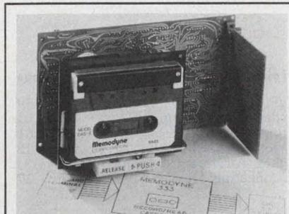
**MEMODYNE** Incremental Digital Cassette recorders read, write, store alpha-numeric data at 50 cps in ASCII or 8-bit parallel. 72,000 character capacity. Low power (CMOS) for data logging, off-line terminals, microprocessors. Interfaces w/wide variety. Lit. avail. Memodyne Corporation, 369 Elliot St. Newton, Mass. 02164 617/527-6600 telex 922537
