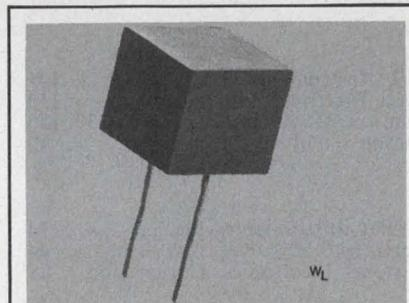
**THE WL 451-T IS A HIGHLY LINEAR THERMISTOR.** Using special semiconductor construction, the positive coefficient unit changes  $+4.93 \Omega/\text{C}^\circ$ . Special features include 1% tolerance, linearity  $\pm 1\%$  from  $-25$  to  $+150^\circ\text{C}$ . Epoxy-cast in a .435" cube. \$9.50 (1-9) Western Laboratories 728 S. Marengo, Pasadena, CA 91106 213-793-0148
