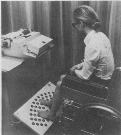
Operator controls are provided on a single three-way switch mounted on the interface unit. They allow the machine to be turned on and off and operated at various speeds, which are selected by varying a resistor in a time-delay circuit. ■■
