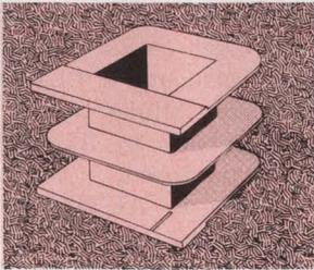
Special "split" bobbin (secondary wound alongside primary rather than over it) effectively isolates primary and secondary and reduces inter-winding capacitance. An electro-static shield
