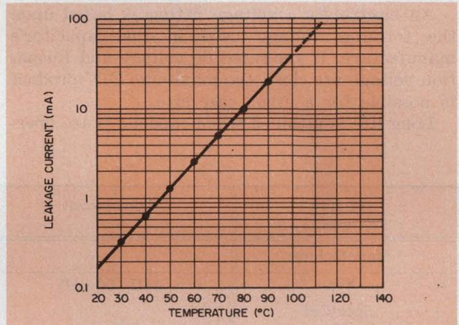
3. Leakage current doubles every time the core temperature rises about 10 C.
