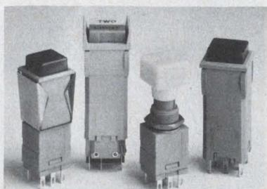
**S190/S410 Switchlights.** Low cost 2 Form C Mom. & Alt. action; Dual wiping contacts. Rating 100,000 cycles @ 2 amp res., 0.5 amp ind., 30 VDC & 125 VAC. Quick connect & solder terminals. Snap-in & rear panel mount. 10-amp power switch UL listed. Varied lens shapes. Clarendar Co., Box 785, Post Falls, ID (208) 773-4541
