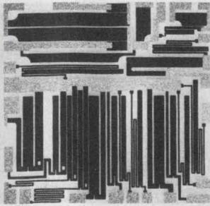
**Complete Functions Offered on a Chip.** High density monolithic thin film processing offers exceptional resistive performance for hybrid assembly. 250 standard variations available to .01% accuracy, tracking to 0.5ppm/°C. Analog Devices, Inc., Route 1 Industrial Park, P.O. Box 280, Norwood, Massachusetts 02062. Telephone: 617/329-4700.
