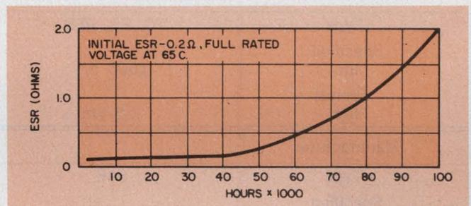
4. A capacitor's ESR increases with the unit's age, mostly because of loss of electrolyte.
