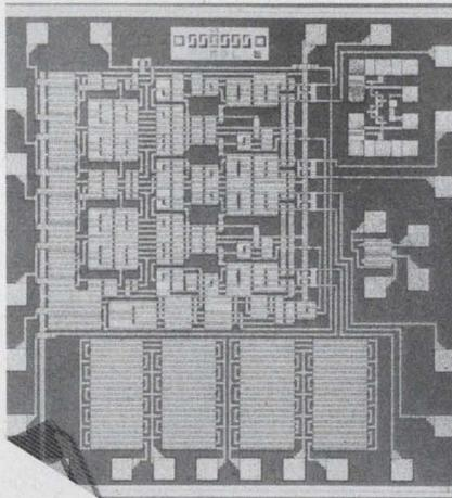
**CMOS silicon-on-sapphire circuits**, such as this 4008-type 4-bit adder from Rockwell International, are undergoing tests to develop radiation-hardened MOS/LSI circuits. This chip has 170-transistor complexity and a chromium-doped gate oxide.
