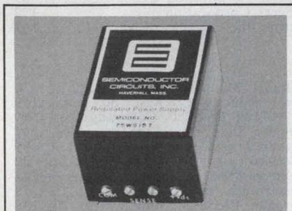
The "75WS15T" provides  $\pm 15\text{Vdc}$  @ 150mA and an isolated 15Vdc @ 200mA with rem. sense. Sense current 200  $\mu\text{A}$ ; Tempco 0.002%/°C; 1500V isolation; current foldback on all outputs, O.V.P. on X-Ducer supply; Price \$196.00; Del 2 wks. Other models avail—contact Semiconductor Circuits, Inc., 306 River Street, Haverhill, MA 01830, (617) 373-9104
