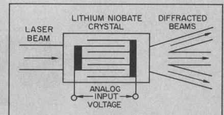
tion of voltage to the electrode system terminals produces spatially periodic variations in the refractive index of the crystal. As a result, a laser beam passing through the crystal is modulated in intensity, as different orders of power are diffracted in controlled directions.
