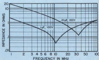
Proven multi-layer construction. C0G(NP0) and X7R temperature characteristics. Preferred ratings are .01, .047, and .1  $\mu\text{F}$  @ 100WVDC. Operating temperature range,  $-55\text{C}$  to  $+85\text{C}$ .
