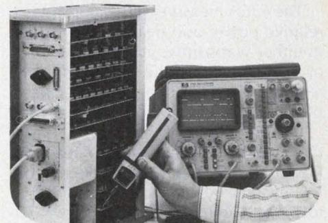
With dual-delayed sweep, two markers select time period to be measured and a proportional voltage output is provided for DVM readout.
