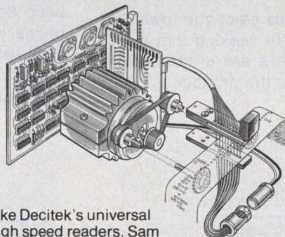
Like Decitek's universal high speed readers, Sam has our patented dual sprocket drive that starts, steps and stops accurately every time, eliminates tape wear. A highly stable fiber optic-photo transistor array reads 5, 6, 7, and 8 level advanced and center feed hole tapes interchangeably without adjustment. For more features that make Sam more than a match for any other low cost reader, write for our brochure.
