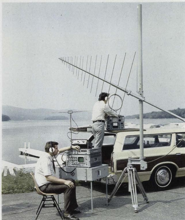
**Battery operation for field use** is another trend in spectrum analyzers. Though it can be used outdoors, Rohde & Schwarz's Analyskop gives laboratory performance.
