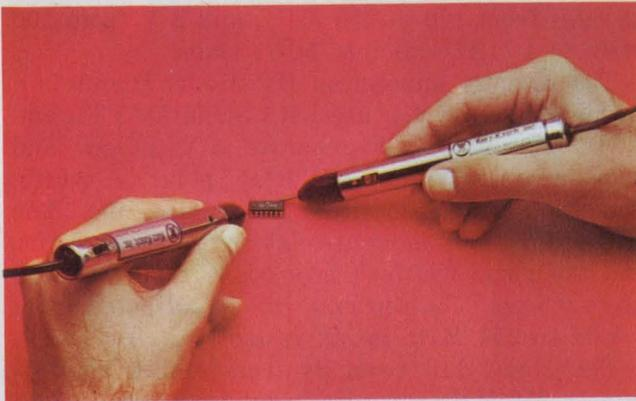
A hand-held pulser and logic probe locate stuck nodes quickly. The Model HL-583 stimulator (left) operates at 5 Hz or in a one-shot mode. The unit can supply up to 1 A for 1  $\mu$ s with CMOS or TTL amplitude levels and takes its power from the circuit under test. The resultant logic state is shown in the probe (Model LP-575). Both units are from Kurz-Kasch, Dayton, OH.
