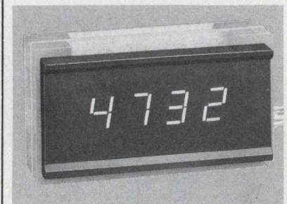
LED Digital Displays have attractive one piece bezel constructed of black anodized aluminum. Units employ H.P. 7750 - .43" high char. 2 thru 10 digits are stock. Options include series resistors or decoder drivers. Standard termination is 30" cable or wire wrap pins. Rochester Digital Displays Inc. 120 N. Main St. Fairport, N.Y. 14450 (716) 223-6855.
