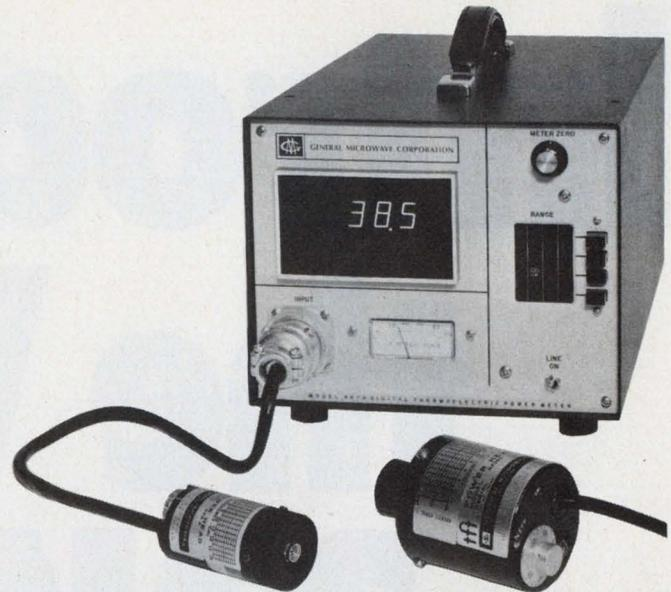
Direct reading from 10 nW to 3 W on a digital display is possible with the Model 467A meter from General Microwave. The unit employs a thermocouple sensor.
