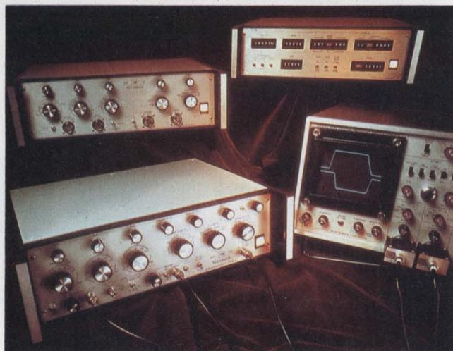
The pulse generator and scope are well-known design aids. But their speed and versatility are greater than ever. The generators from E-H Research Laboratories include a 50-MHz fully programmable unit, the 1501A (top right); a laboratory version, the 135A (lower left), and the EH-129, a 500-MHz unit. An AMC 1100 sampling scope (1 GHz) is an appropriate display unit.
