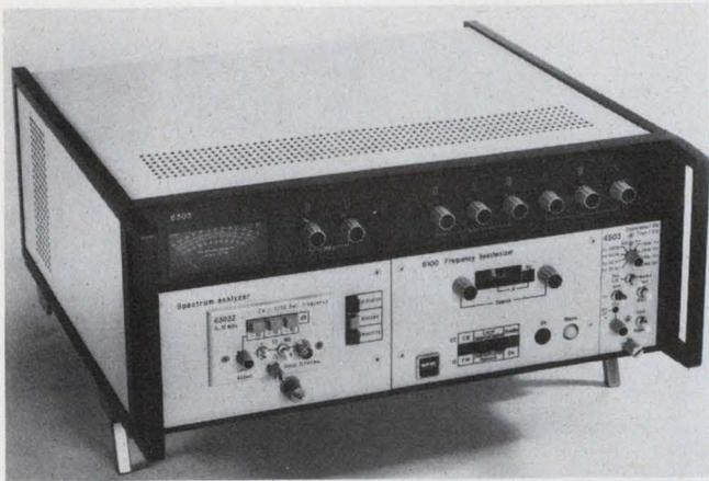
With a dynamic range of 120 dB, the Adret 11-MHz 6303 holds the title for this spec. With a substitution of plug-ins, the unit becomes a synthesizer.
