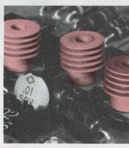
The Triac-Kooler is a low cost (only 17¢ each in quantity) heat dissipator that effectively levels excessive heat rise in triacs, affording greatly prolonged usefulness to the triac. A push-in rivet firmly assembles the Triac-Kooler to the base of the triac. The multiple finned area disperses the heat. The small size of the Triac-Kooler permits dense packaging. The attaching push-in rivet is supplied with each Triac-Kooler. Nothing else is needed. No tools. Send for your sample . . . try it.
