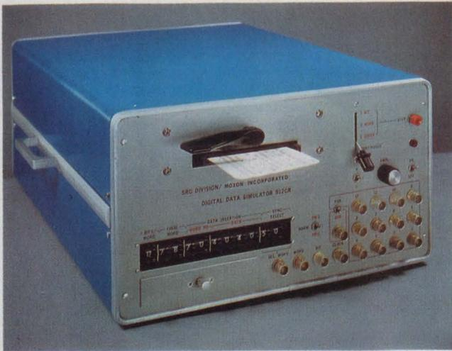
Word generators exercise complex digital gear with pre-set digital pulse streams. The Model 912CR from SRC Moxon operates at clock pulse rates to 10 MHz (serial output) and to 5 MHz (12 parallel bits). A card reader facilitates rapid changes of programmed data—up to 960 bits—with a single IBM card.
