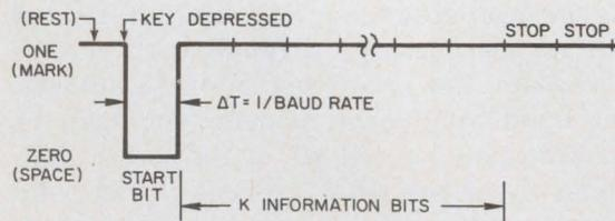
Model 33 Teletype terminals use two Stop bits and ASCII code—that is, 11 bits per character. This is the code used on Western Union's TWX Network at 110 baud. Telex uses the five-bit Baudot code with a rest period of 1.5 baud times, and operates at a 50-baud rate.
