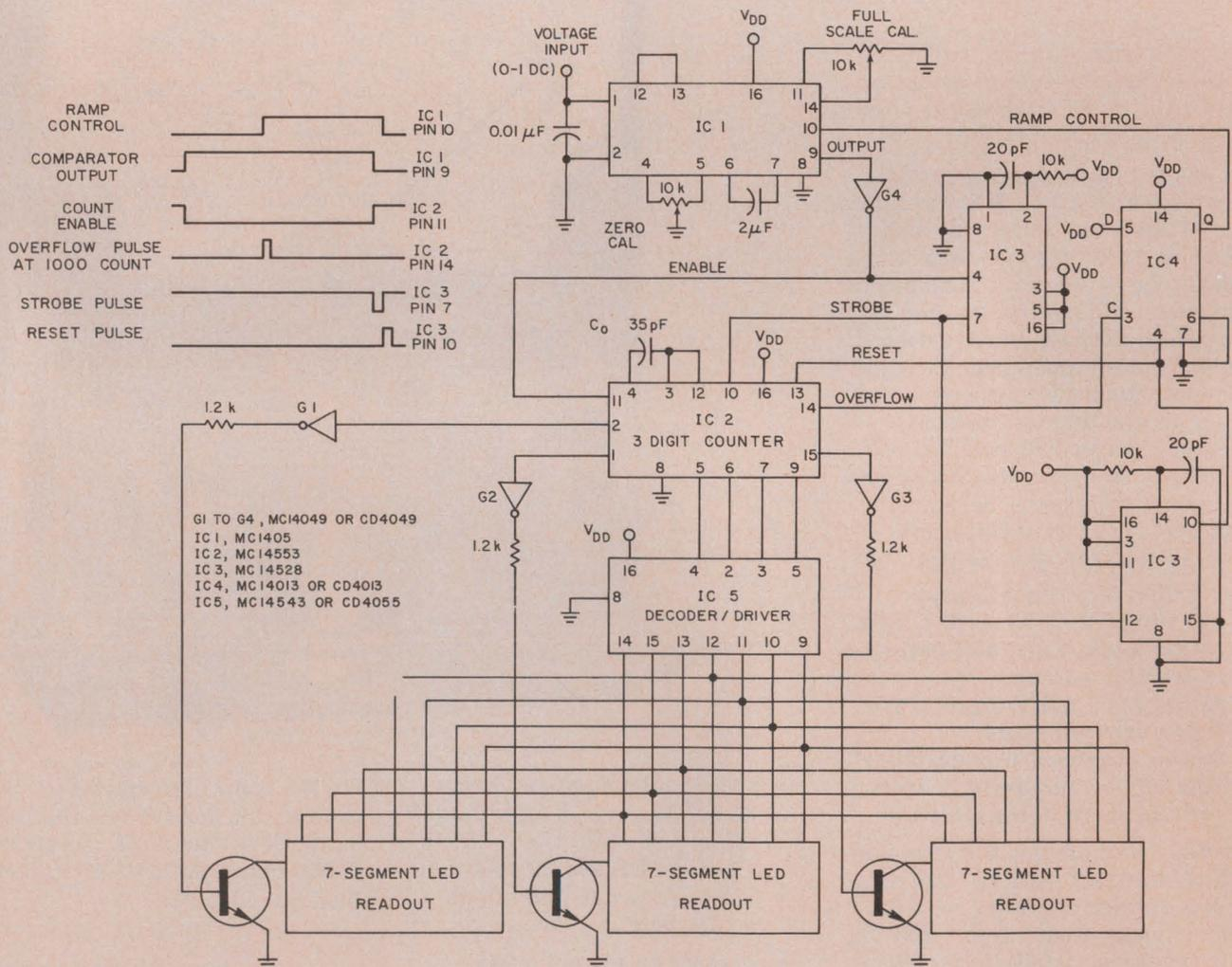
In this CMOS DVM, one decoder driver is multiplexed to drive three, LED, seven-segment digit displays.
