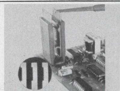
**New PROTO-CLIP®** for power-on, hands-off signal tracing. Eliminates shorting leads. Plastic construction eliminates springs and pivots. Scope probes & test leads lock onto Dynagrip inset. 14-pin: \$4.50 each. 16-pin: \$4.75 each. From distributors or Continental Specialties Corp., Box 1942, New Haven, CT 06509.
