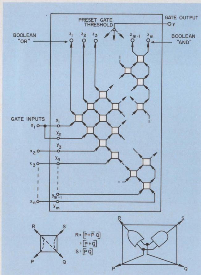
6. A combinatorial array of a digital-summing threshold-logic gate provides the basis for a stable, versatile gate that can be easily fabricated with LSI.
