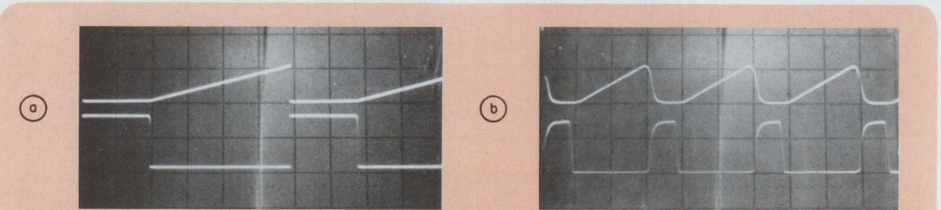
3. The sweep generator covers easily a wide range of speeds; traces range from 0.5 ms to 0.5  $\mu s$  per div.
