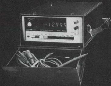
**Model 7004A.** All-function unit measures dc/ac volts, dc/ac current and resistance with excellent overload protection. AC response to 100 KHz.  $\pm 0.01\%$  DC accuracy. Optional internal battery pack and carrying case. Basic price \$650.
