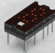
**745-0007** LED hexadecimal display with on-board logic operates from 5 to 6 volt supply, low power consumption. Integral TTL MSI chip provides latch, decoder and drive functions. 0.270" character display has wide angle visibility and mounts into standard 14-pin DIP socket.
