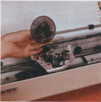
**Daisy-wheel printers**, such as this one from Qume, give high-quality, fully formed characters on six-part forms. Current daisy-wheel printers go up to 45 cps.
