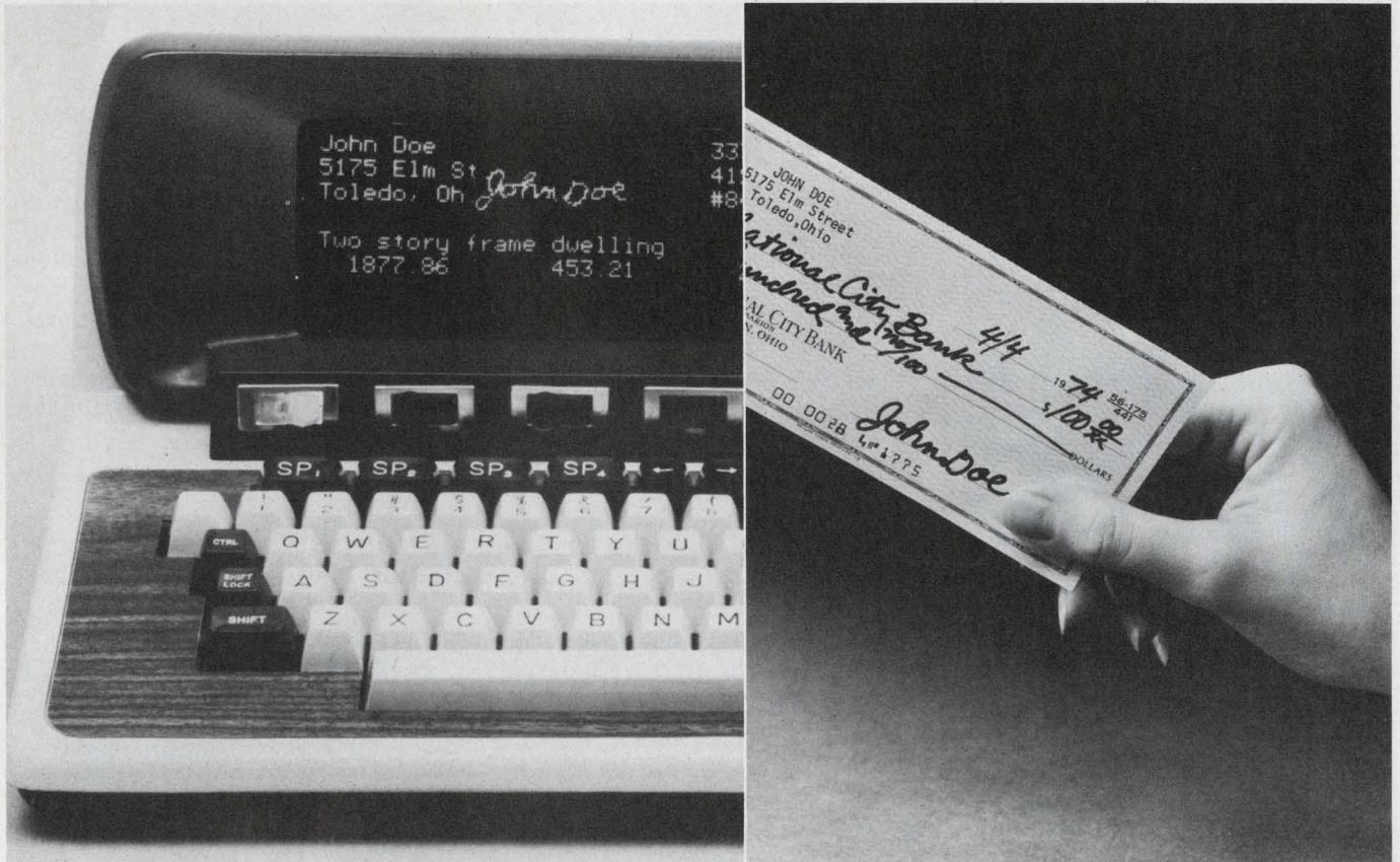
Digivue 80-33 in demonstration unit, showing high-contrast display for use in signature verification.
