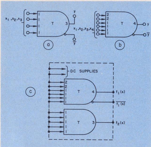
2. Configurations of "universal" threshold gates for functions where  $n \leq 3$  (a) and  $n \leq 4$  (b) can be easily packaged in DIPs. A 16-pin DIP (c) can contain at least one  $n \leq 4$  universal threshold gate plus one five-input unity-weighted gate, which is somewhat more versatile than an  $n \leq 3$  gate.
