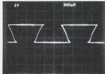
ing edge) of 500  $\mu$ s, a hesitation (trailing edge) of 500  $\mu$ s and a flare (wide top or bottom) of 2 ms.
