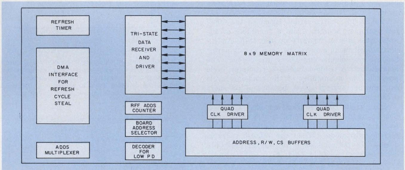
2. A 32-k-word  $\times$  9-bit memory board (photo) uses interchangeable 4-k RAMs from AMI and Motorola Semiconductor. The single board directly replaces four boards using 1-k dynamic (1103-type) RAMs. It is also a quar-
