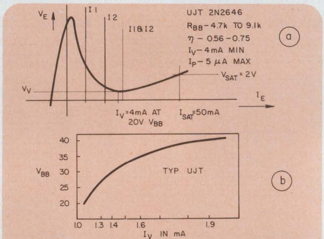
2. Correct design for this sweep generator requires that you determine  $I_V$  accurately. To obtain holdoff,  $I_2 + I_3$  must be greater than  $I_V$  (a). But most typical  $I_V$  vs  $V_{BB}$  curves (b) don't show low values of  $V_{BB}$ . A curve tracer can provide these data.
