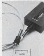
Solid state semi-conductor sensor.
