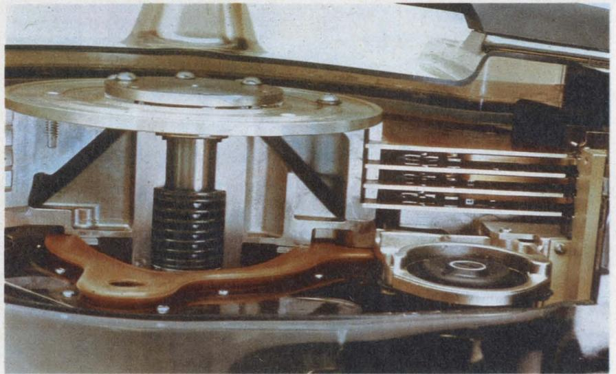
**Incorporating the head-positioning system** and the recording medium in the same module makes the IBM 3340 disc drive unique. Data density on the Winchester is 5636 bpi, and average access time is 25 ms.
