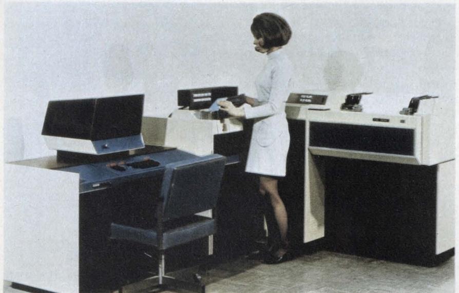
**Remote batch system** from Control Data can be used to support a number of engineering users by providing high speed data entry and printing capability without tying up individual terminals.
