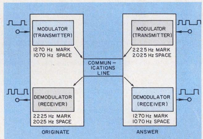
Originate and Answer modems must operate in pairs so that receiver and transmitter frequencies match.
