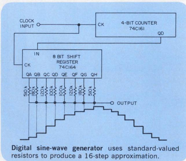
Digital sine-wave generator uses standard-valued resistors to produce a 16-step approximation.
