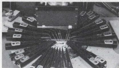
Computer controlled laser equipment provides pretest to insure proper screening and curing and precise adjustment of resistors. Resistor trimming is shown in this view of the laser head.
