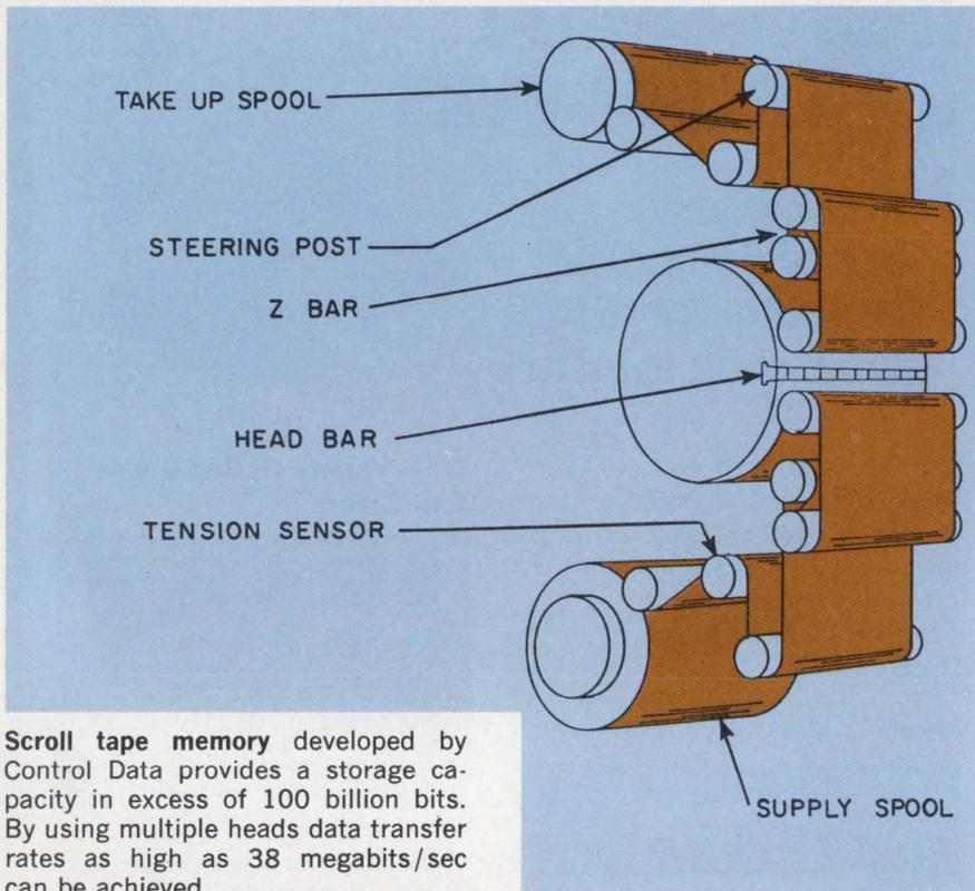
Scroll tape memory developed by Control Data provides a storage capacity in excess of 100 billion bits. By using multiple heads data transfer rates as high as 38 megabits/sec can be achieved.
