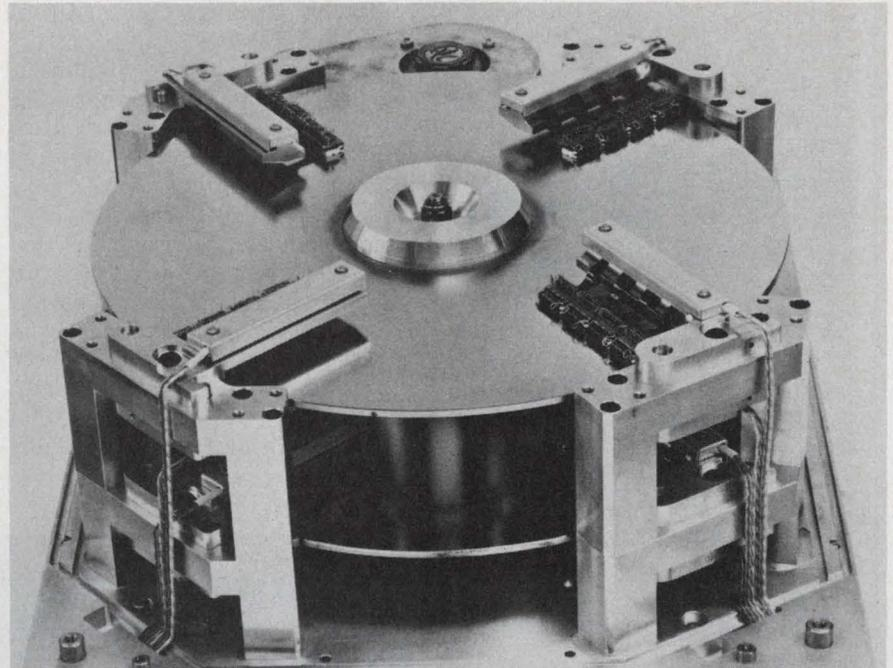
**The Mididisc from SDSI** is a rapid access device designed to hold 40 megabits of storage. It rotates at 3450 rpm, has an average access time of 8.5 ms and transfers data at 4.5 megabits/sec.
