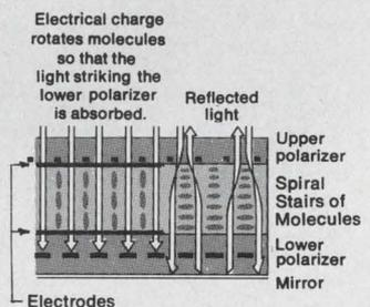
**A few limitations.** LCD's have limitations too. Operating temperature range is one. Liquid crystals slow down and may even cease to function at temperatures below 0°C. Above 50-60°C, crystals go into solution and will not function properly. But extremes do not damage LCD's. Once the temperature returns to normal, operation is automatically resumed.
