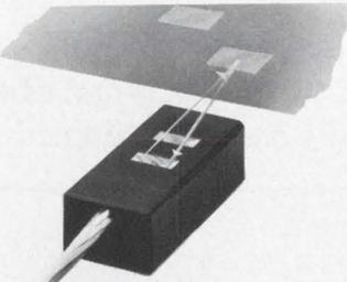
EOT/BOT LED/Phototransistor sensor for 1/2-in. magnetic tape.
