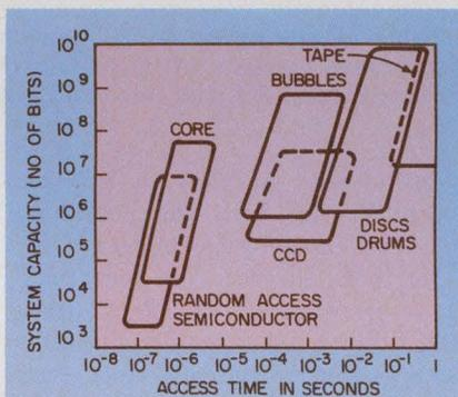
Memory performance can be judged by comparing access time and system capacity for the different technologies.
