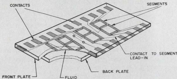
**How they work.** When the liquid is not electrically excited, its long cigar-shaped molecules are parallel to one another in a position perpendicular to the plates. The liquid appears transparent. When an electric current is applied, ion activity of the molecules leads to turbulence causing the liquid to scatter incident light. Depending on the type of nematic liquid used, either a dynamic scattering or field effect display results.
