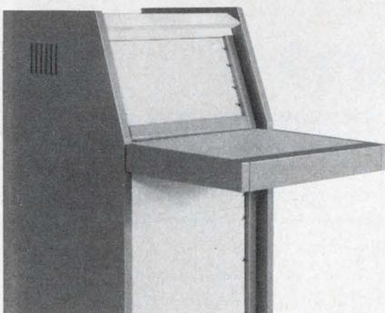
Inclined panel cabinet racks come in three sizes; clear inside depth, 20-1/2". Three extra-deep units are also available with a clear inside depth of 29-1/4". Front panel is positioned 20 degrees off vertical and all panel mounting rails are adjustable, including those in the inclined section.
