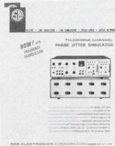
Simulation of telephone channels has become exceedingly important as data transmission increases. For testing, training, and evaluation, controlled impairments must be introduced. These include Phase Jitter, attenuation and envelope delay distortion, impulse hits, broadband noise, harmonic distortion, frequency translation, and phase hits.
