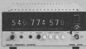
The 5700A Frequency Counter. Range 10 Hz to more than 512 MHz. Nine digit display. Carrier measurements to 1 Hz resolution in 2 seconds of keyed transmitter time. Selective signal tone checks to 0.1 Hz resolution. Sensitivity 10 mV rms with AGC. Stability  $3/10^7$ /month.  $3/10^9$ /day optional.
