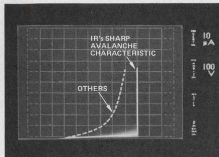
The avalanche curve pictured shows our "sharp" curve and the "soft" curve of the others. Convincing evidence of better junctions that you can operate at full rated specs without a worry.
