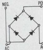
Another **FIRST** from Varo Semiconductor, Inc. An integrated bridge rectifier in a miniature, 4-pin, low-profile DIP.
