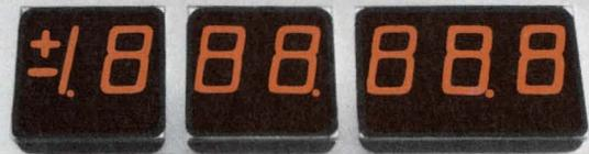
**755 SERIES** High brightness planar gas discharge displays in a 0.550" character. Orange color gives high contrast ratio and allows readability to 40 feet even in high ambient lighting. Designed for interfacing with MOS/LSI, displays have an expected life of 100,000 hours or more.
