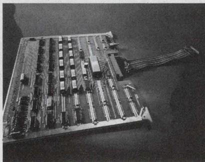
**A trend in microprocessor development** is the incorporation of microprogramming. The microprogram control logic above, by National Semiconductor, duplicates the functions of National's mask-programmed CROM and uses fusible-link pROMs for custom microprogram implementation.
