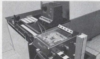
Screen printing is the first step in the **NEW PEC** automated process. Substrates are automatically fed through the printer where precise metallization patterns are deposited before firing.
