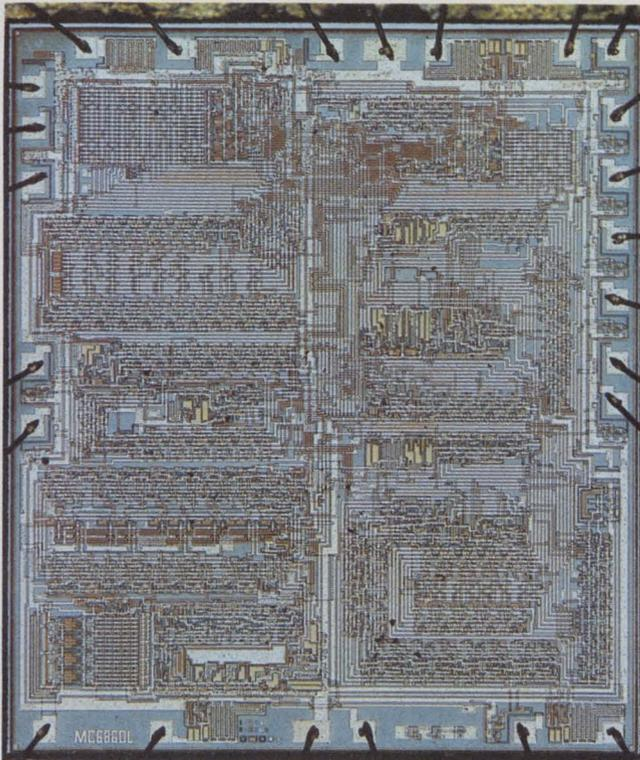
Add external filters and Motorola's NMOS chip, the MC6860, becomes a full-fledged 300-baud modem with all control lines.
