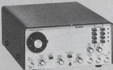
The WB series sweep generators are designed to make complex swept measurements at relatively low cost, are simple to operate having a single center frequency dial with illuminated indicator, push buttons for all on-off functions and well labeled controls with fully descriptive nomenclature. The WB-713, pictured, covers the frequency range 1 to 950 MHz in two bands.
