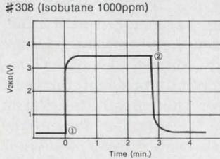
① Point at which sensor is exposed to gas/air mixture.
