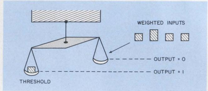
1. A mechanical analogy of a threshold gate shows that the inputs are weighted. And when their summed total equals or exceeds the threshold level, the output is a binary transition from logic ZERO to ONE.
