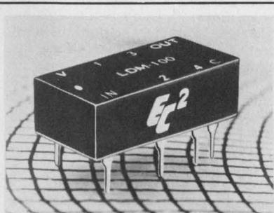
**EC²'s new T²L Compatible Logic Delay Module** features; 14-pin DIP package (.250 high); precise delays from 25nf to 250nf; with 10 T²L input and outputs; tops at 20% increments, each isolated and with 10 T²L fan-out capability. Engineered Components Company, 3580 Sacramento Drive, San Luis Obispo, CA 93401 (805) 544-3800.
