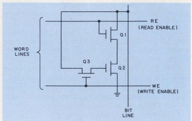
5. This three-transistor-per-bit cell forms the basis of the 6605 4-k RAM. On the chip, the present cell measures 3.4  $\text{mil}^2$  with a new cell design of 2.5  $\text{mil}^2$  expected to appear on the market in the near future.
