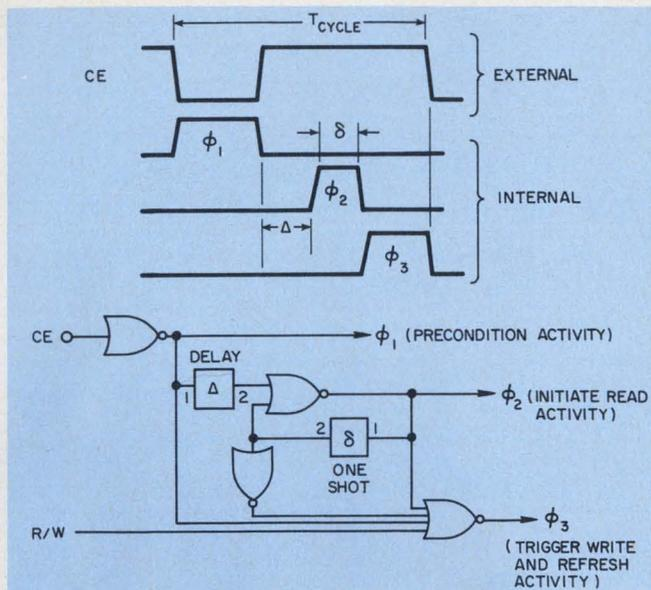
6. A timing generation scheme is needed for the operation sequence. Three sequential pulses— $\phi_1$ ,  $\phi_2$  and  $\phi_3$ —are triggered by a single external clock (CE). The period of the CE signal defines the memory cycle. Delay  $\Delta = \phi_1 - \phi_2$  is required by the decoder circuit employed.
