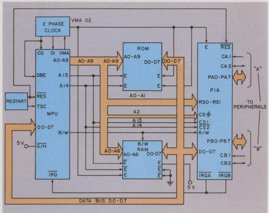
**Better interfacing is provided in the newer microcomputer architectures.** Motorola's M6800 uses an MC6820 Peripheral Interface Adapter (PIA) to interface the microprocessor to peripherals with two 8-bit bidirectional data buses and four control lines. No external logic is required.
