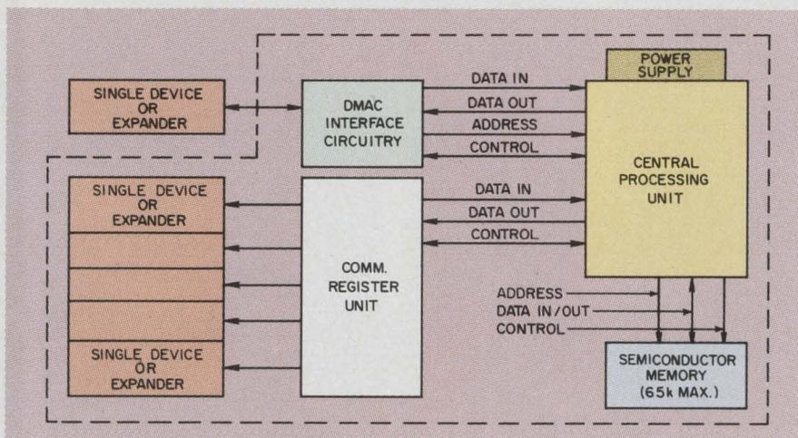
A unique architectural feature for minicomputers, a communication register unit, is provided for TI's 960B in process-control or manufacturing-control operations. This register is used instead of an I/O unit to permit bit-by-bit input and output in serial form.
