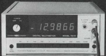
**Model 7205.** 26 ranges. Resolves  $\pm 1$  microvolt DC, 1 milliohm resistance,  $\pm 1$  nanoamp current. Measures dc/ac volts, dc/ac current and resistance with excellent overload protection.  $\pm 0.005\%$  accuracy. Display digits over  $\frac{1}{2}$ " tall. Lead-compensated ohms. Optional isolated BCD output. Basic price \$1095.
