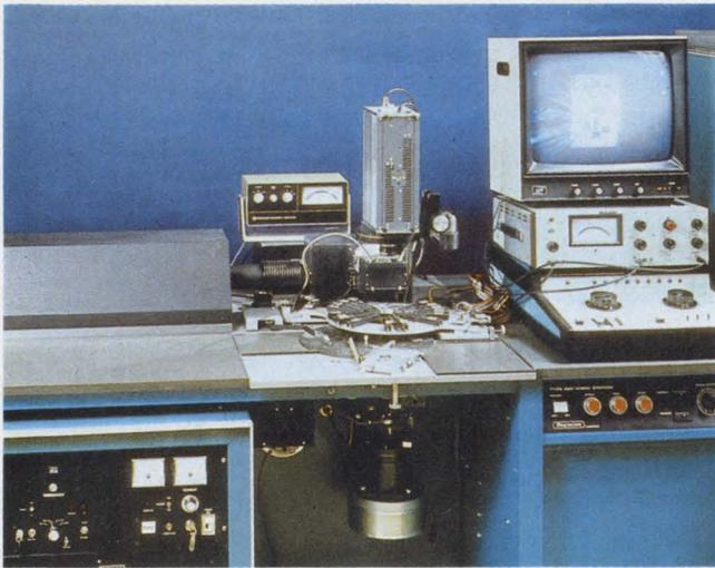
**Laser trimmer sets FSK frequencies** precisely for Cermetek's hybrid modem modules. The unit trims the frequency determining resistors for the 300-baud set.
