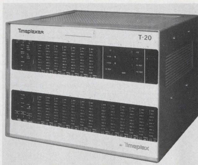
In addition to combining data from multiple channels, a TDM serves as a test center. Switches and lamps help pinpoint problems among modems, lines, other multiplexers, terminals or computers.
