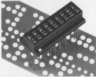
9 NPN Phototransistors mounted on .100" centers.
