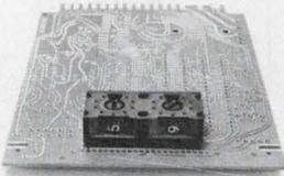
Other facts: it comes in one, two, three, four, five, and six station models (\$1.95 per station, standard); in a variety of codes, including decimal, BCD, Complimentary, Special Binary, and 1, 2, 3, and 4 pole.
