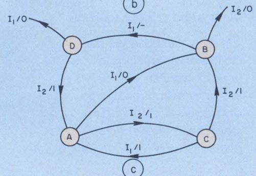
2. Design requirements can be specified by a state table (a), its more compact form (b) or an equivalent flow diagram (c).
