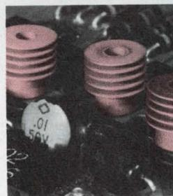
The Triac-Kooler is a low cost (only 17¢ each in quantity) heat dissipator that effectively levels excessive heat rise in triacs, affording greatly prolonged usefulness to the triac. A push-in rivet firmly assembles the Triac-Kooler to the base of the triac. The multiple finned area disperses the heat. The small size of the Triac-Kooler permits dense packaging. The attaching push-in rivet is supplied with each Triac-Kooler. Nothing else is needed. No tools. Send for your sample... try it.
