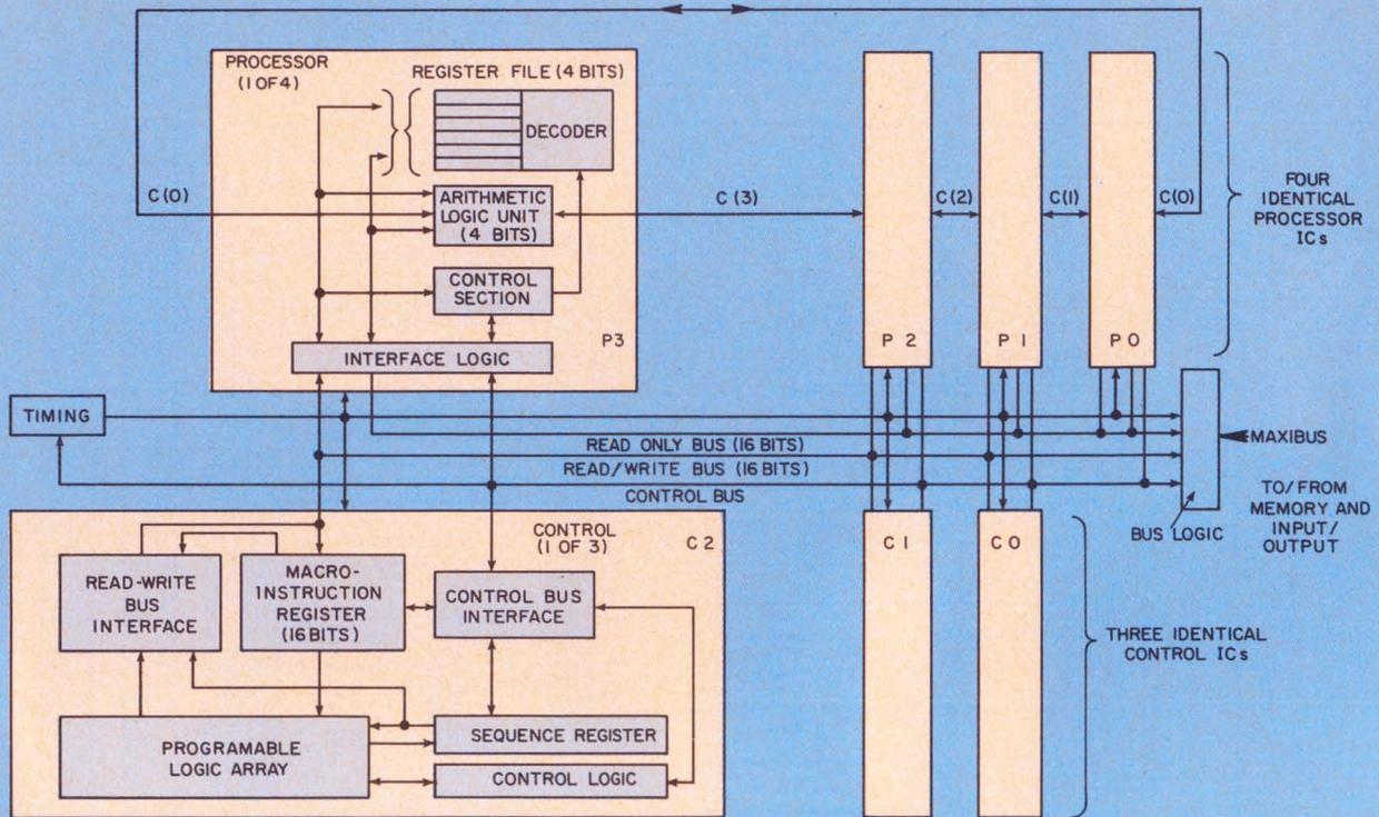
4. Custom microprocessor chips are used in Computer Automation's Naked Mini/LSI. The chips resemble the National Semiconductor's IMP series, in that one IC is de-
