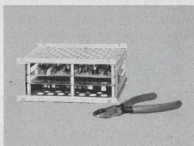
**Model MOD-815 A/D Converter.** Digital data with 8-bit resolution at any random or periodic word rate from DC through 15 MHz. Only 100 cu. in. Power dissipation approx. 20 watts. Computer Labs, 1109 S. Chapman St., Greensboro, N.C. 27403.
