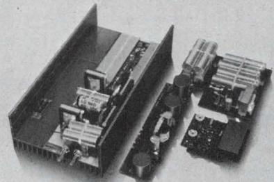
*proven* design and package it in six different case shapes — wide and short or narrow and long — for customer convenience. With a nominal power density of 1.37 watt/cu. in., LH switchers pack more power into a smaller package than any other switchers you can buy.
