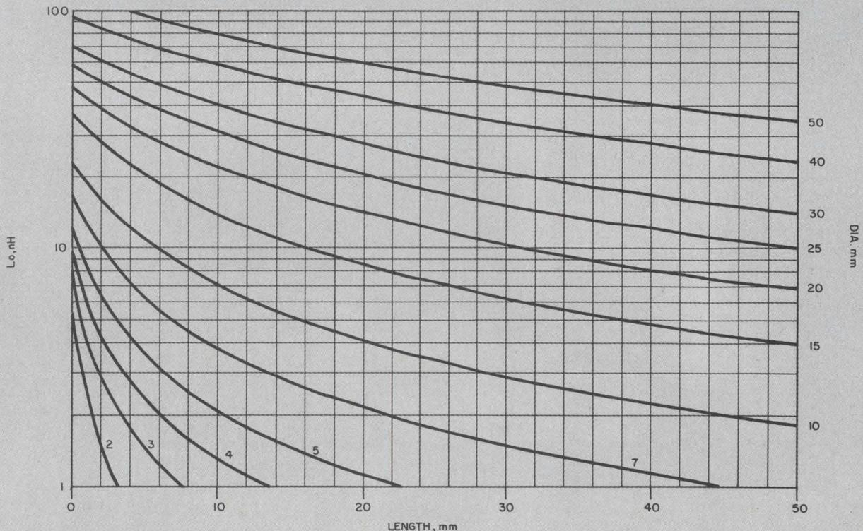
The specific inductance of a small coil can be obtained if you know its length and average diameter.
