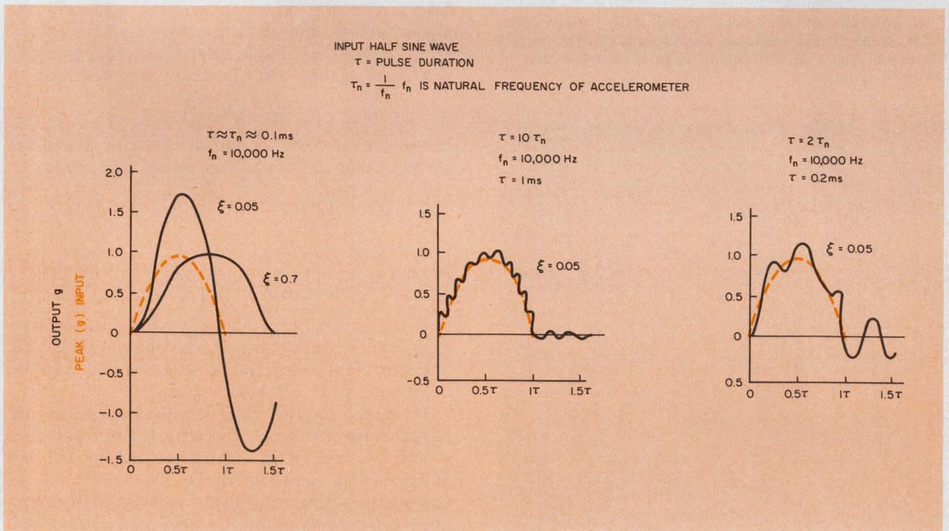
6. With an input of a half-sine-wave shock pulse, a typical transducer output doesn't necessarily follow
