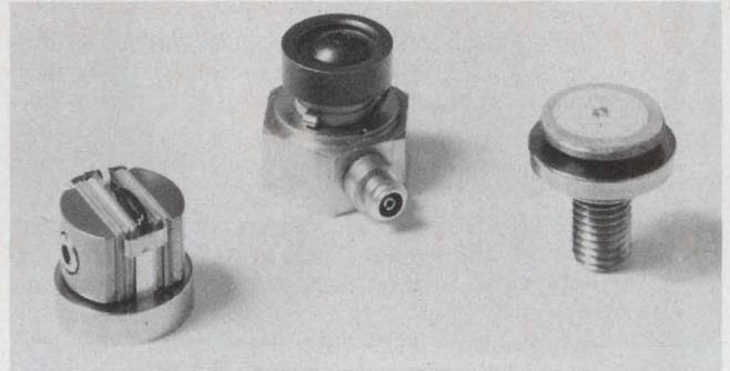
**Piezoelectric accelerometers** (shown without their cases) use one or two slices of piezo material.
