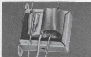
its case. This heating element is connected in series with the secondary coil winding and its load, transferring heat to the MICROTEMP with the flow of current. Should the current flowing through the element exceed normal operating levels, the resulting heat will cause the
