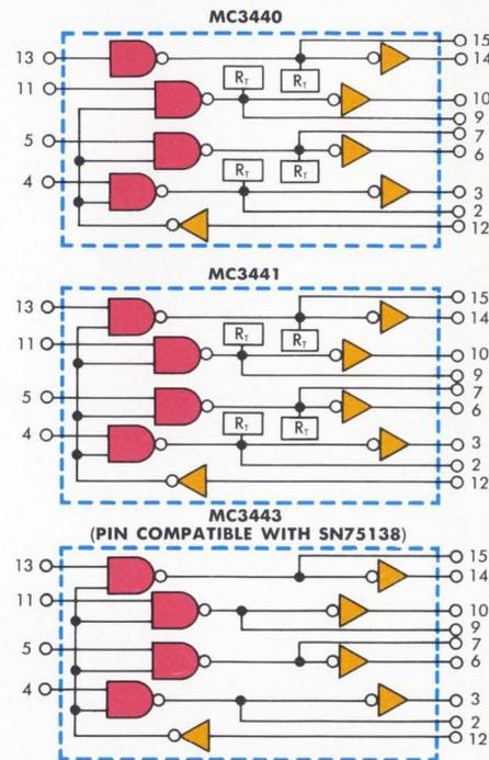
The MC3440 family of Quad Interface Bus Transceivers
