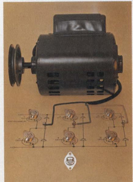
Power Darlington, such as these from TRW Semiconductor, are replacing SCRs in ac motor-control applications. They require less external circuitry than SCRs and are less prone to false triggering.
