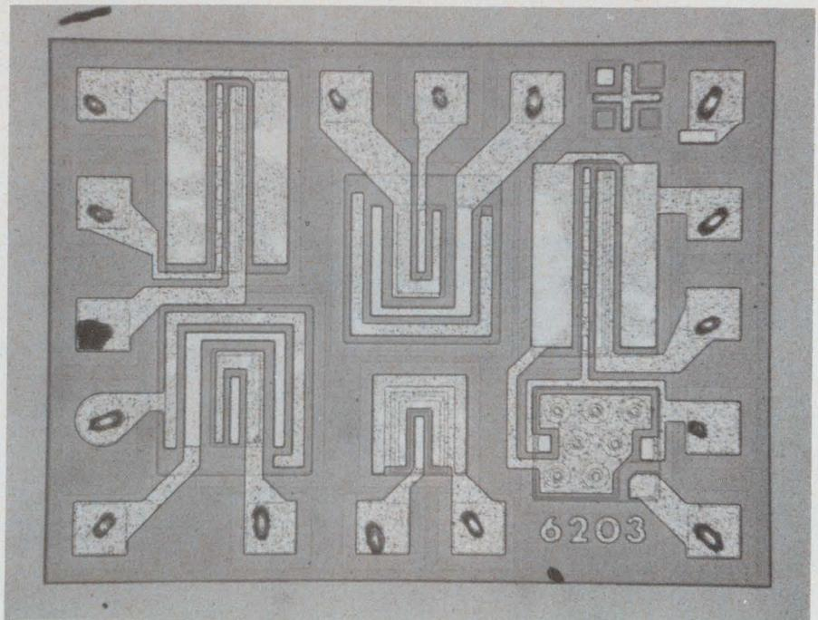
SCRs as part of monolithic ICs are bringing down the cost of controlling very small motors. The RCA CA3097E thyristor/transistor array contains an SCR with 150 mA max forward current, as well as an array of transistors and a zener diode.
