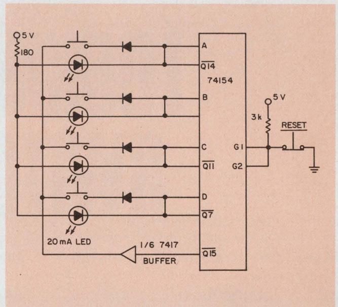
9. **First-to-respond detector** indicates which of the four buttons was pressed first. Feedback from  $Q_{15}$  controls a common ground for all switches. The ground is removed as soon as the quad-flop switches from the OFF to a latched state, and the LEDs indicate which button was pressed first.
