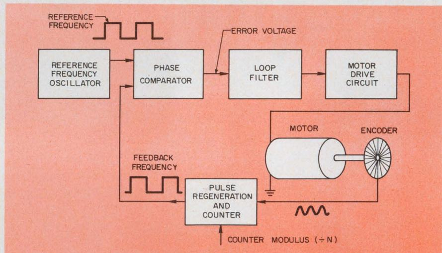
**Digital phase-locked loops** can be used for precision speed control as well as positioning. In this system, from Motorola, a shaft encoder is used to sense motor speed, and a pulse train is fed back to a comparator, to be checked against the reference pulse train. If the motor is not synced to the reference, an error voltage adjusts the motor speed.
