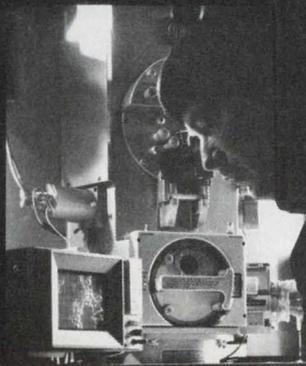
Gray scale capability and variable persistence storage of the 605 are used with a scanning electron microscope to study metal samples in a dental research laboratory.
