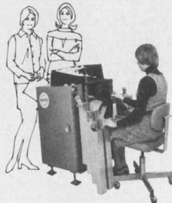
to do the rest: position housing . . . insert terminal to exact depth and lock it in place . . . repeat until the preset number of terminals are inserted . . . then eject the completed connector—*all automatically*.
