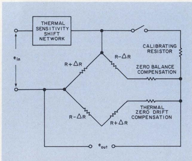
8. The strain-gauge accelerometer uses a balanced bridge network with thermal compensation added to maintain the zero drift and temperature sensitivity with specifications.
