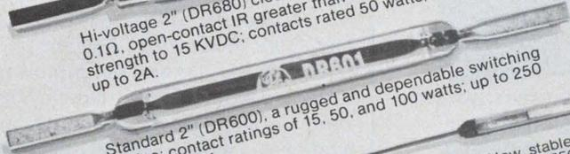
Standard 2" (DR600), a rugged and dependable switching device; contact ratings of 15, 50, and 100 watts; up to 250 VDC, up to 3A.
