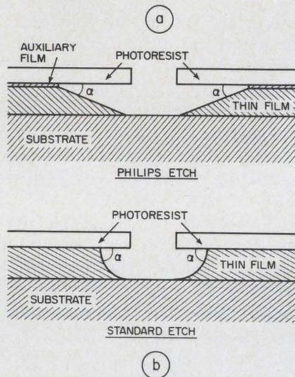
film, the fabricator can control slope of the thin film between 1 and 60 degrees. The Philips process has been fully developed for thin films of gold (to 5  $\mu\text{m}$  thick), for Permalloy (to 3  $\mu\text{m}$  thick) and silicon dioxide (to 10  $\mu\text{m}$  thick).
