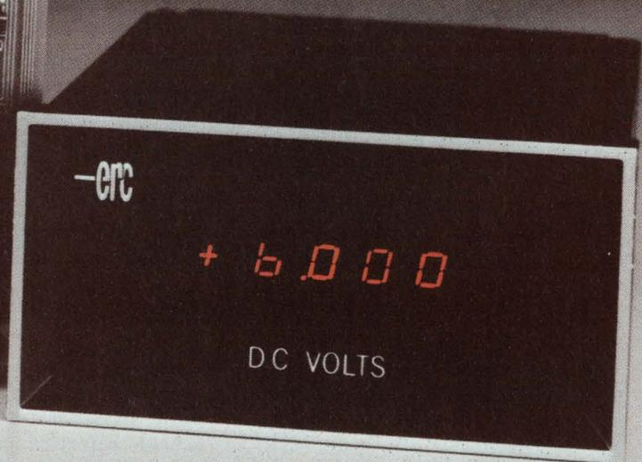
While most DPM manufacturers strive to compress their meters into a one inch cube, ERC has succeeded in making a producible and maintainable low-cost voltmeter with optically isolated parallel BCD outputs and 5999 count full-scale for reliability-conscious engineers in a package only 2.4" H x 5.06" W x 6.38" D, AND for only \$148 in quantities of 100...\$185 in single quantities. If the world's smallest DPM isn't your prime requirement but quality is, contact us for specs and delivery.
