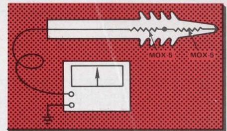
MAXI-MOX resistors have full-load drift less than 1% in 2000 hours of operation, and are available in tolerances of 1, 2, and 5% in values from 10K to 2,500M ohms. A silicone varnish conformal coating provides environmental protection while allowing a maximum hot-spot temperature of  $220^\circ\text{C}$ .
