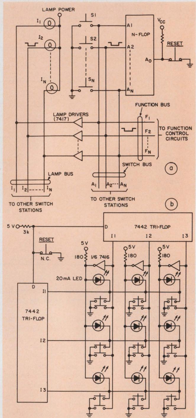
8. These n-flops latch for the most recent button pushed. The first circuit (a) uses single-contact switches. The m × m arrangement (b) uses smaller n-flops.
