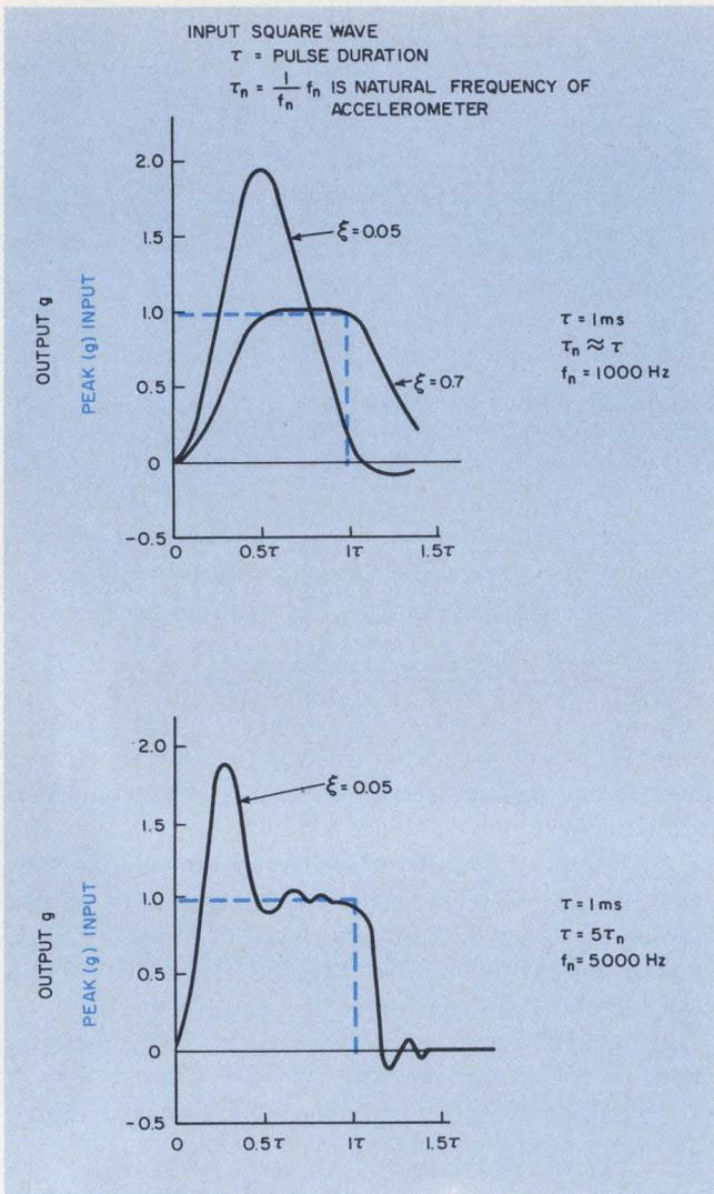
7. If you change the input signal to a square-wave shock pulse, the transducer output will usually exceed the actual value of the shock pulse unless the unit is critically damped.
