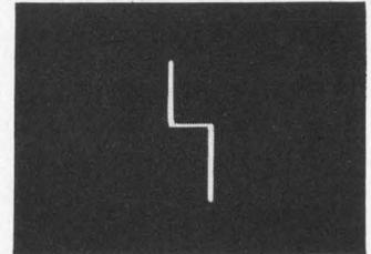
2. It's a "Quicktracer" Transistor/Diode and Component Tester. Typical junction waveform.
