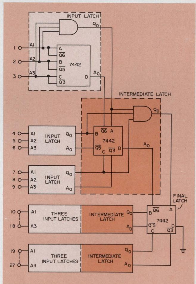
6. The tree structure allows construction of an n-flop of any desired size. Each stage of this 27-flop is essentially a 7442 tri-flop. The addition of more input and intermediate latches allows further expansion.
