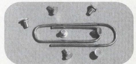
Besides greater power and efficiency, double-drift IMPATTs have lower junction capacitance and lower fm noise compared to single-drift IMPATTs.
