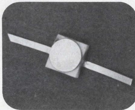
The new Schottky mixer diode has a low noise figure of <math><6\text{ dB}</math> at 9 GHz.
