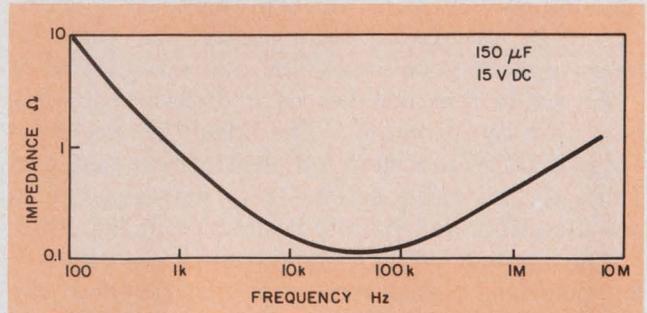
7. An electrolytic capacitor's impedance is equivalent to a series RLC circuit. Minimum impedance, which occurs at resonance, is resistive.
