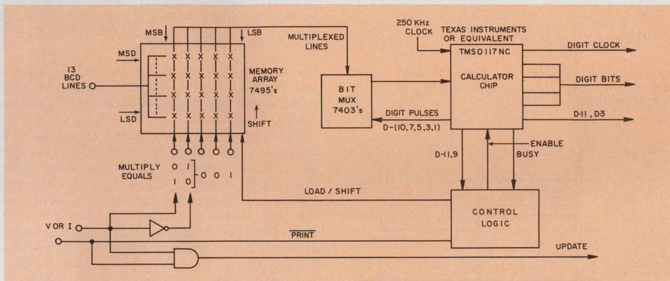
2. Power is derived by direct multiplication in the calculator chip of the BCD numbers for voltage and current.
