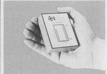
**"Synchro to digital converters** - 10, 12, or 14 bit output, errorless tracking up to 4 r.p.s., accuracy ±4 min. of arc ±.9LSB, resolution - 1.3 minutes, 60 or 400 Hz input, Module 2.6 x 3.1 x .82" H, Price From \$350 in qty. Computer Conversions Corp., East Northport, N.Y. 11731 (516) 261-3300."
