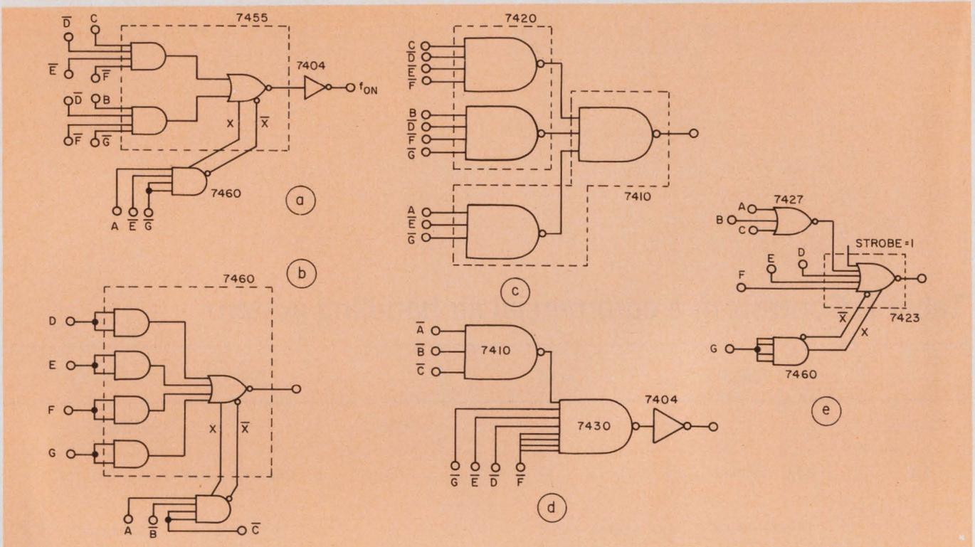
2. IC implementations of a CAD logic function problem (a) and (b) produce the function and complement, respectively, from the computer printout. A third circuit
