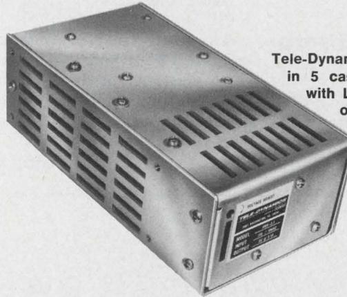
Tele-Dynamics Series HR... 30 models in 5 case sizes... interchangeable with Lambda LM and similar... output 5-28 Vdc, 1.3-20 A... ripple 1 mV rms... line & load regulation each  $\pm$ 0.05%... input 105-125 / 210-250 V, 47-63 Hz... unit price \$113-\$256.
