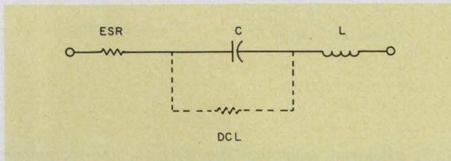
2. In addition to the desired capacitance, an electrolytic capacitor has unwanted dc leakage (DCL), equivalent series resistance (ESR) and inductance. These characteristics are much worse for electrolytics than for most other capacitors.
