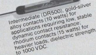
Intermediate (DR500), gold-silver alloy contacts (10 watts) for alloy applications requiring low, stable dynamic contact resistance; rhodium contacts (15 watts) for heavier loads; dielectric strength to 1000 VDC.
