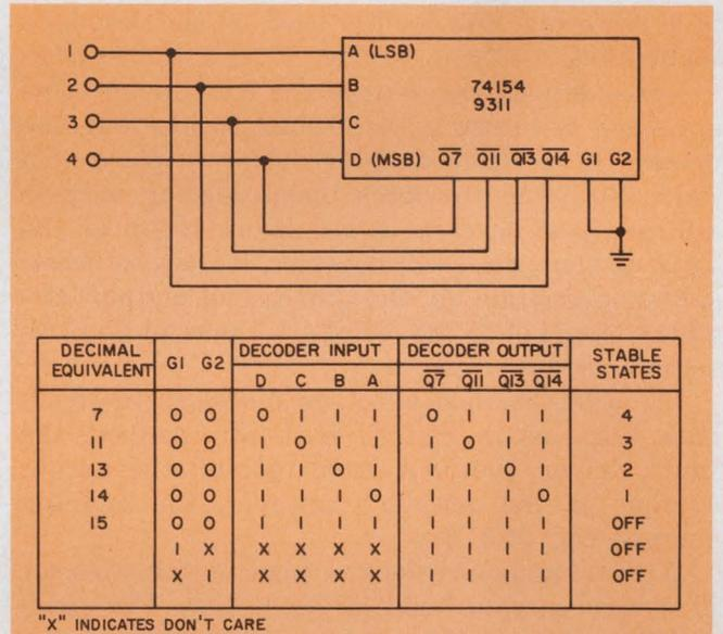
3. This quad-flop is built with a 1-of-16 decoder, as shown by the input-output table. A fifth state (1111) could be extracted with an external decoder, if needed.
