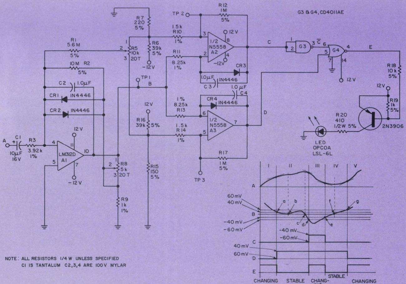
**A LED lights when a slowly varying dc signal stabilizes. A changing signal causes the output**
