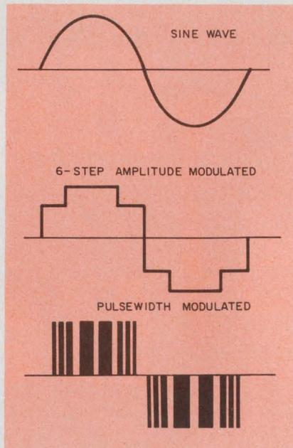
**Inverter modulation schemes** for variable-frequency ac motor control center on simulation of the desired sine-wave output of the inverter. The two primary modulation techniques are multistep amplitude modulation and pulse-width modulation. Pulse-width modulation allows a better approximation of the wave shape and seems to be the wave of the future in ac-inverter design.
