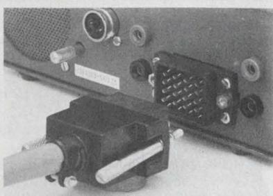
**Rugged and low-cost 36-pin connector.** Suberly designed and produced with simplified construction. Cut your costs up to 50%. Moisture-resistant glass-filled nylon insulator Recessed contacts in both male and female housings. Hood provides positive cable strain relief. Interchangeable. E. F. Johnson Co., Waseca, MN. (507) 835-2050.
