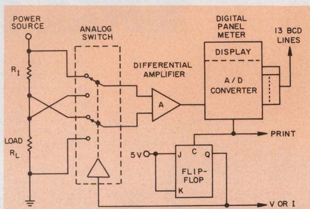
1. Load voltage and current are sampled by the analog switch and then multiplexed to the DPM, where both are changed to digital form by the DPM's a/d converter. The sampling process is controlled by the internal clock of the panel meter. Since voltage and current are measured independently, the meter can handle unstable loads.
