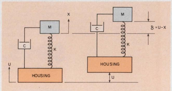
1. **Ideal seismic systems** can be modeled to simulate the transducer and the way it is affected by forces.
