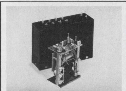
**Modular DC-DC power converters.** Designed to meet military/aerospace specs . . . priced for industrial applications. 12, 28, 48, 115 VDC inputs. 1-6 isolated, regulated (1% & 0.1%) outputs. 1-500 watts. Efficiencies to 85%. 1200 design-as-you-order configurations using standard modules. Arnold Magnetics, Culver City, Ca. (213) 870-7014.
