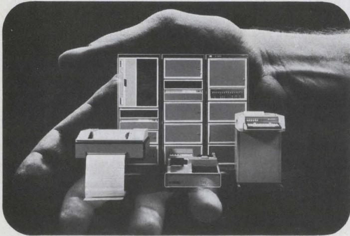
The new HP 3000/model 100 timeshare system is the most powerful BASIC system on the market. Besides offering terminal access to as many as 16 users, the new super-timeshare system simultaneously compiles and executes programs in batch mode, in FORTRAN, COBOL and our own system programming language (SPL). Unlike its competition, the HP system can handle integers, real, long-precision, and complex numbers, *all in the same program.*
