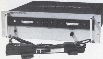
When your application calls for a system or lab power supply in the range of 0-4 kV, HP has six models to fill your need. Three of them are constant voltage/constant current supplies with sufficient output current to power devices such as klystrons, magnetrons, backward-wave oscillators, high-power gas lasers, and electron-beam welding devices. Model 6521A delivers 0-1 kV at 0-200 mA; model 6522A delivers 0-2 kV at 0-100
