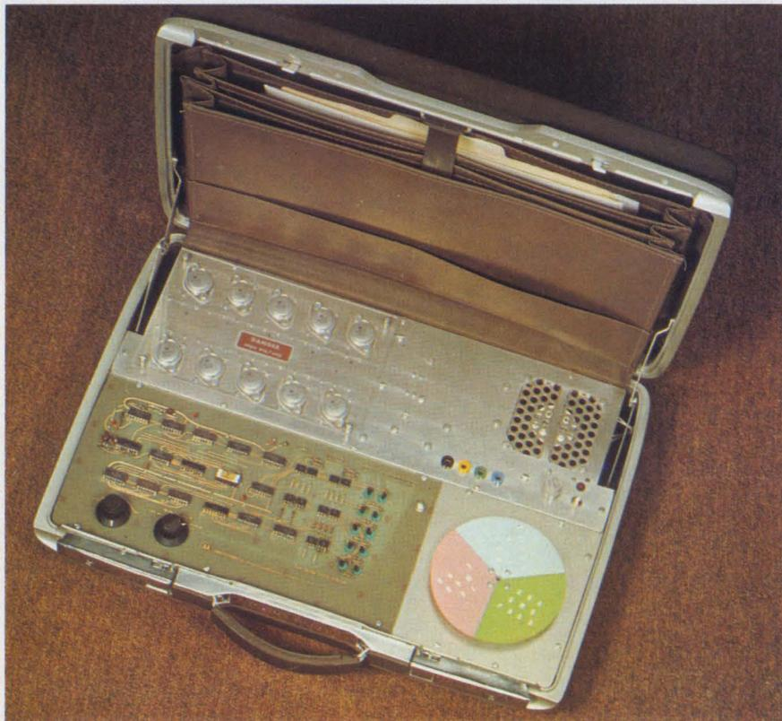
Control of bursts of dc voltage can be used for motor speed control. Varying the width or repetition rate of these pulses changes the motor speed. Motorola uses an MCM14524 CMOS 1024-bit ROM to generate the pulse-width variations in a sine-weighted sequence. The color wheel was part of a strobe-lighted speed control demonstration.
