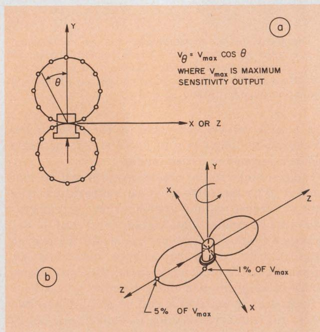
4. Vertical sensitivity of a piezoelectric pickup (a) allows a  $\pm 10^\circ$  off-vertical displacement with only a 2% output variation. Transverse, or cross-axis sensitivity (b), caused the output to change by 7% for a similar angular rotation.
