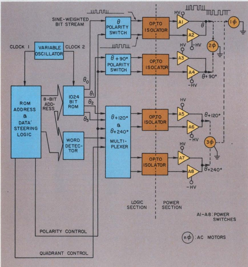
A versatile circuit capable of controlling the speed of four single-phase motors, one two-phase unit, or one three-phase device uses a 1024-bit ROM to generate sine-weighted, pulse-width-modulated trains of pulses having a variable repetition rate. The circuit, by Motorola, uses opto-isolators to decouple the low-level switching stages from the high-power driving stages.
