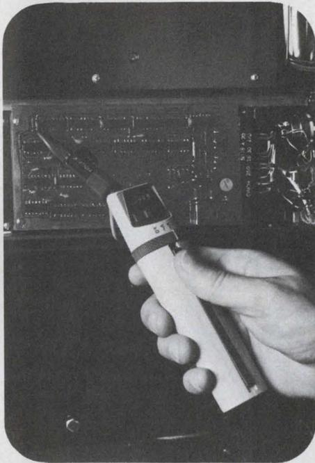
A new RF probe adds 100 kHz to 500 MHz ac measurement range to HP's handheld 970A digital multimeter. Accuracy within this range is greater than 1 dB. The new 97003A RF adapter measures 0.25 to 30 V full scale. Maximum input is 30 V rms, plus 200 Vdc.
