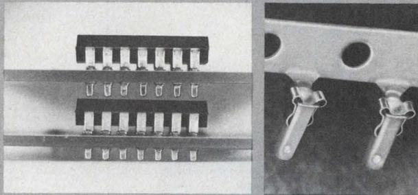
For use where space is restricted; extends just .030" above and .088" below board, allows .400" board-to-board spacing. One size MINISERT\* socket fits wide range of hole sizes—.050" to .058" in diameter. RTV diaphragm seals foreign matter out of the socket. MINISERT socket accepts round or flat leads of DIP's, LED's and LSI's. Free-standing design can be used in any socket pattern. Semi-automatic machine inserts at rates up to 2000 per hour. Write for Bulletin 120, or call:
