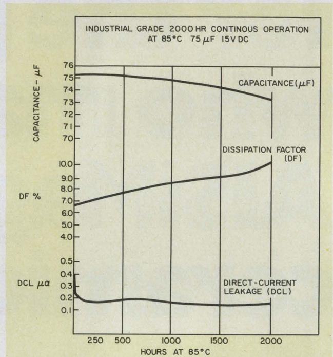
1. Even good grade aluminum electrolytic capacitors lose capacitance and experience an increase in dissipation factor with age.
