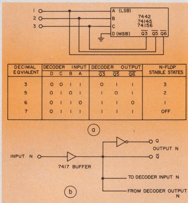
1. A tri-flop is constructed from a 1-of-10 decoder (a). A LOW placed on any one of the three input lines latches that line and releases the others. An open collector buffer attached to the feedback line isolates input and output (b). The inverter, if used, gives the complement of the n-flop state.
