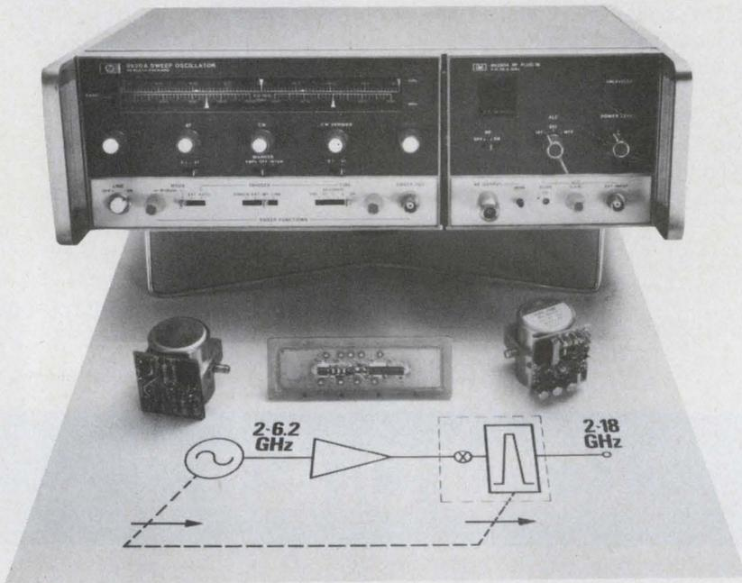
Advanced microwave technology now brings you a broadband 2-18 GHz sweeper with the performance precision needed for stringent lab and production tests, as well as size and weight advantages for field applications. The new 86290A plug-in in the 8620A mainframe is the smallest
