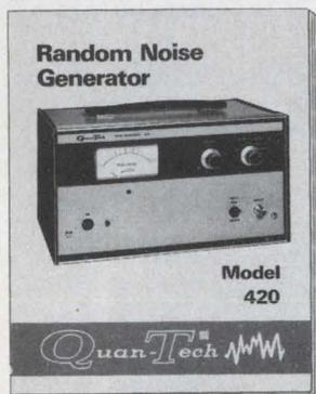
The Model 420 provides a precisely calibrated random noise source with Gaussian amplitude distribution. Spectral density distribution is independent of frequency (white) with lower cut-off approaching D. C. Analog outputs from 0.01 to 1000  $\mu$ V per root Hertz continuously variable and metered. Response is flat from D.C. to 100 KHz.
