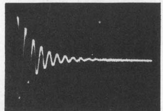
4. It's a "ringing" tester for coils, yokes, transformers. Typical ringing test pattern.
