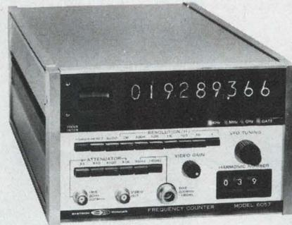
Why pay over \$5,000 for a microwave frequency counter that measures CW only? Systron-Donner's idea: one instrument that measures **everything**: FM, pulsed RF and CW. Result: Model 6057 which measures virtually any microwave signal from 20 Hz to 18 GHz. Price \$5,450. Industry response: One of our
