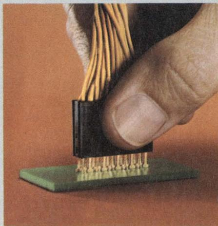
The Locking Clip Connector mates with .025" posts on a true grid. Receptacle contacts are tin-over-nickel plated by a unique process which makes them approach the performance of gold. The connector is available in 4-, 10- and 20-position configurations and will accept #26 to #30 AWG wire. Contacts can be terminated by high-speed, automated machines for uniform reliability at low applied cost.
