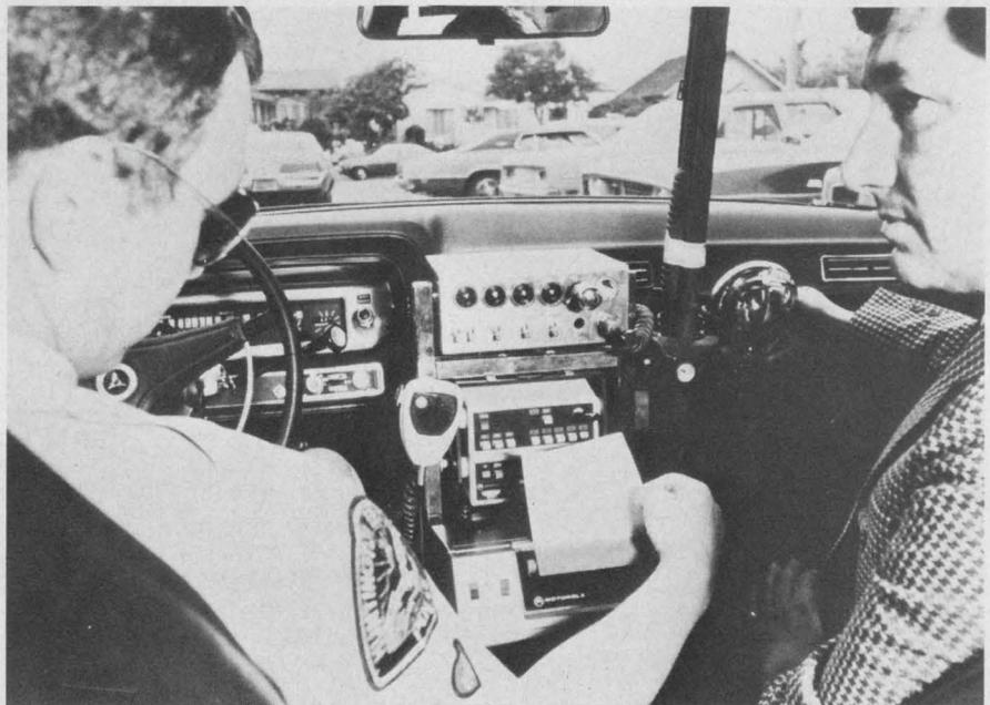
**Hard-copy readout** is provided as part of Motorola's Command and Control digital-communications system. It minimizes the chance of error in the dispatching of officers to a particular location.
