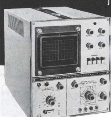
An excellent bench or design scope at low cost. DC-15 MHz vertical bandwidth with 24 ns risetime ...10 mV input sensitivity ...12 calibrated vertical attenuator positions up to 50 V/cm...1 megohm/40 pf input Z protected up to 600 VDC...22 calibrated time bases from 2 s/cm to 0.2 μs/cm... x5 magnifier...normal or auto triggering...AC/DC coupling...ext. trigger input...built-in calibrator...6 x 10 cm screen...120/240 VAC operation. Send for FREE catalog for complete details & specs.
