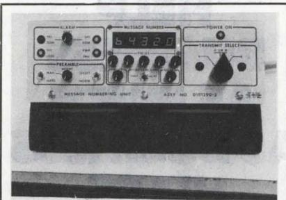
**The Pulsecom Model 461-6** Automatic Message Numbering Device electronically inserts station identification and message numbers. This device saves operator time, and prevents mistakes. The 461-6 operates at 45-1200 Baud with most terminals. Pulsecom Div of Harvey Hubbell Inc., 5714 Columbia Pike, Falls Church, Va. 22014. 703-820-0652.
