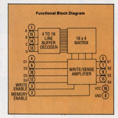
equivalent) has an opencollector output to use whenever data-bus line impedances are defined by other sources. Both have PNP inputs biased for standard 54S/74S threshold levels.
