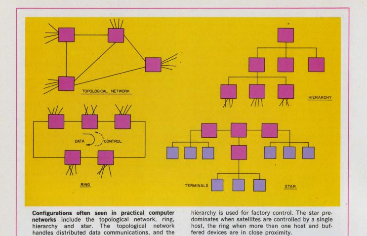
are split off from data collection and summary operations. The user must provide some form of data-transmission path between the "worker" computers and the hosts.
