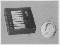
VCXO Crystal Clock Oscillator at freqs. from .00005 Hz to 50 MHz freq. tol.  $\pm$ .0005% 0°C to +50°C, control voltage range +4V to -4V changing freq. 20 ppm/V, linearity  $\pm$ 2%, 1.75" sq. x 0.5", Supply 5Vdc  $\pm$ 1%, Sq. wave 2.4V into 200 $\Omega$  at Vdd = 5V, stock to 5 weeks; Connor-Winfield Corp., W. Chicago, Ill. 60185. 312-231-5270
