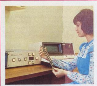
Holographic data retrieval unit from to read data stored on 35 mm that holographic recorder is used to sto
