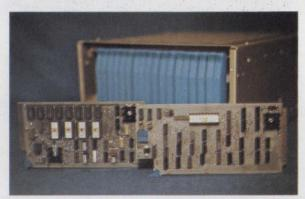
Process Control Systems' general-purpose interface, the Series 2000 (background), uses the Intel 8080 as the heart of a micro-CPU module.
