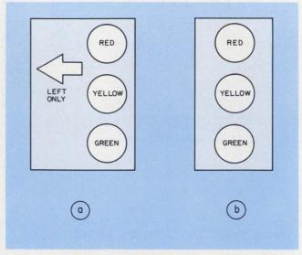
2. Traffic signals under microcomputer control consist of east-west lights (a) and north-south lights (b). The left-turn signal in east-west lights can be independently set to red, yellow or green.
