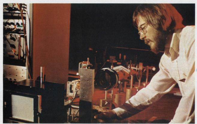
Optical memories like this one from Sperry Univac are being designed to store up to 10° bits of in-
