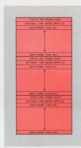
5. A typical data block in memory starts at location x and consists of y words. The status block permits the computation of the subframe or channel at which sampling began. The buffer signals the computer via an interrupt when a block is completed and begins a new block in an alternate buffer area.
