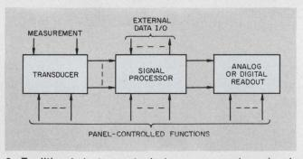
2. Traditional instrument designs use analog signalprocessing techniques to obtain readouts of measured values. Such techniques used to be cheaper.
