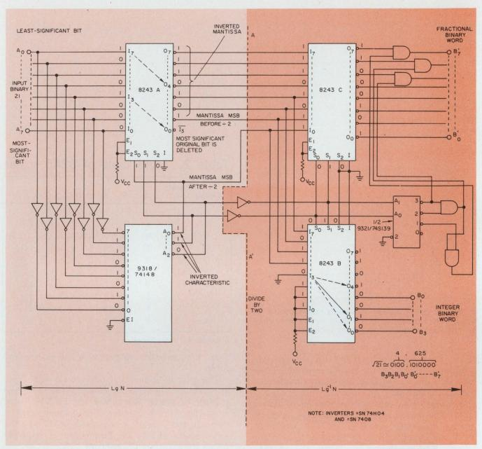
2. A combinatorial 8-bit square rooter needs only a log\_circuit, a wired divide-by-2 and an antilog\_circuit.
