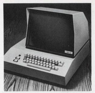
The Microterm series, built by Digi-Log Systems, are microprocessor-based, intelligent terminals that can be customized to a user's specs.
