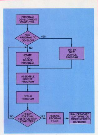
Minicomputer programs can be efficiently developed on large, time-shared systems. System flow for Mimic, a software development system by Applied Data Research, is shown above. The Mimic console language enables simulation of a host of minicomputers. Mimic runs on a DECsystem-10.
