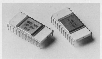
we've crammed all of the following: seven general-purpose registers, a status flag register, an arithmetic logic unit, an I/O multiplexer, and a 16-word LIFO stack that improves speed and performance while conserving main memory. The RALU number is IMP-00H/520D.
