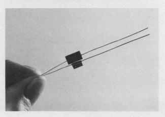
These microminiature solid tantalum capacitors are epoxy-sealed in a polyester sleeve. They're available in both cylindrical cordwood and rectangular modular form, with a choice of axial or radial leads. Capacitance values are 0.001 to 220MFD, working voltages are 2 to 50VDC, and tolerances are  $\pm 10\%$  and  $\pm 20\%$ . They're in excellent supply. We can meet your needs now.
