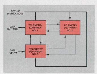
2. **Telemetry systems often have** multiple devices that require computer setup. However, a single output channel is typical.
