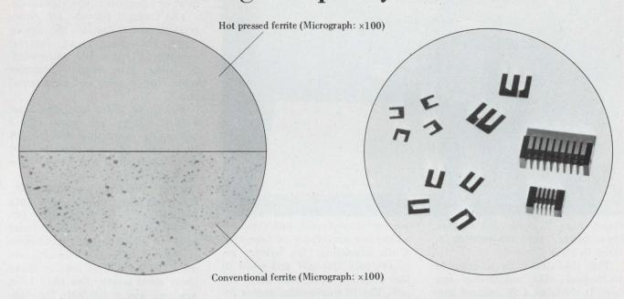
TDK is now producing manganese-zinc ferrite combinations with optimum performance characteristics for computer application. The crystalline powder of these ferrite materials is ground to uniform granular size, hot pressed and sintered into molded head pieces of high density. TDK's Mn-Zn hot pressed ferrite head pieces are free of voids, smooth in finish and have excellent contact wear resistance.
