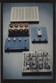
PLUGGABLE BREADBOARDS. Entirely pluggable for use and re-use. No soldering mess or fuss. Fast and convenient with all the accessories for developing your own circuitry.
