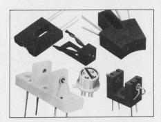
SENSOR AND EMITTER ASSEMBLIES Reflective sensor and optical switch assemblies, utilizing phototransistors or photodarlingtons, are available in several configurations. From a mirror reflection, the phototransistor version generates a 600 microamp signal with 30 milliamps of current on the LED. The photodarlington unit will generate a typical signal of 8 milliamps. These devices are designed for optimum performance at distances ranging from 0.075 to 0.5 inch and are TTL compatible.
