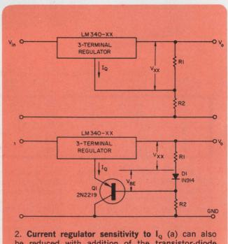
be reduced with addition of the transistor-diode circuit (b).
