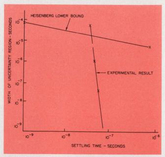
4. Experimental results of the "uncertainty" test are compared with the values predicted by Heisenberg's uncertainty principle. Discrepancies may be caused by thermal noise.
