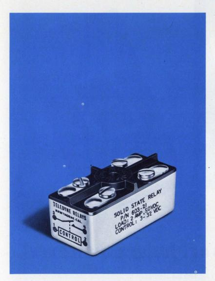
Take a good solid state DC relay — Teledyne's 603, for example — add some shaping circuitry so its response waveshape is carefully altered (rise time, turn-off slope, etc.), and something good happens for designers. In-rush currents for capacitive and lamp loads are limited, and so are turn-off transients for inductive loads. Also, controlled rise and fall time minimize EMI and switching transients.
