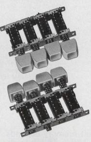
Centralab offers four lockout options for its momentary, push-push and interlocking action pushbutton switch modules. Lockout prevents actuating more than one switch at the same time even if they're not adjacent. Another example of design flexibility. Other features include:
