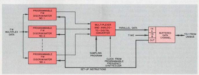
6. FM analog data must be digitized before being inputted to the buffer. The multiplexer controlled by the
