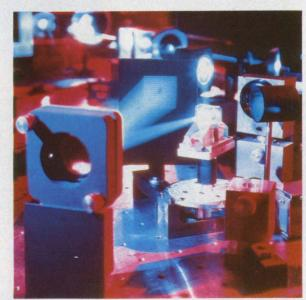
Data beams in this holographic memory from RCA are produced by diffracting laser light off a hologram on which data are stored.
