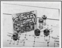
Quartz Crystal Oscillator Kits for \$27. Make bipolar series or CMOS parallel resonant oscillators. Kits include 5 or 6 SX-1 crystals (10 kHz to 240 kHz), in low profile TO-5 cans, a PC board  $(1.3" \times 1.6")$  and design note. Statek Corp., 1233 Alvarez Ave., Orange, Calif. 92668. (714) 639-7810.
