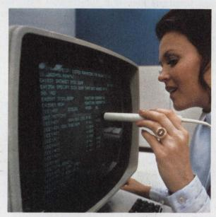
IBM's 3270 terminal is the most widely used intelligent terminal in the field. It is intended for data-entry systems with up to 32 terminals in a cluster to an IBM host computer.
