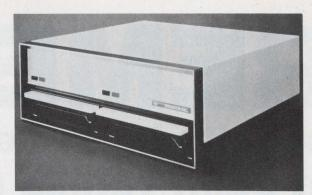
Two fly-head disc drives are contained in the Dynastor Model 40. Each disc has 32 sectors and can store about 2.2 Mb of data. The transfer rate on this drive is 2540-k bits per second.
