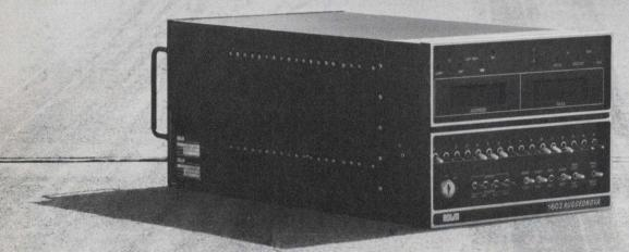
The 1602 is loaded with power features. 450 nanosecond semiconductor memory read cycle time. Memory expansion to 256K words. Dual Port memories. Floating point hardware. Stack processing. Double precision arithmetic. 32-bit instructions and powerful interrupt
