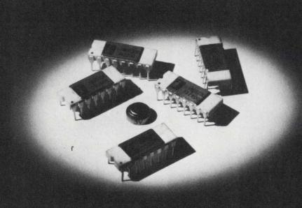
It's fully decoded and buffered, provides static asynchronous operation. Typical access time is 350 nanoseconds. Packaging is in 16-pin DIPs. Price in ceramic DIPs at 100-999 quantities is \$25.60 for commercial (0° to +75°) version and \$46.00 for military (-55° to +125°C), immediately available from Intersil distributors.
