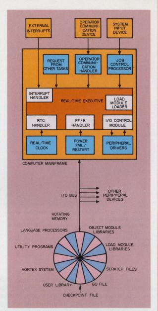
A powerful real-time multitasking operating system, Vortex II by Varian Data, provides foreground/background processing capability, program overlays and simplified I/O operations. Rotating-memory file management is incorporated in the software.
