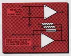
Victoreen MINI-MOX resistors are used widely to modify op-amp characteristics to: 1. Stabilize output and eliminate oscillation. 2. Define gain so measurements can be quantified. 3. Restrict bandwidth to the region of specific interest.
