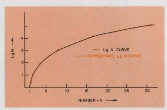
1. A plot of logarithms is closely approximated by straight-line segments between whole powers of 2, which are the logs, of the binary-number sequence.
