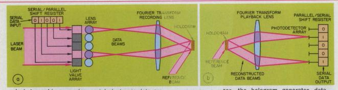
In holographic memories, serial electronic data are converted to parallel optical data and recorded on a holographic storage medium (a). When illumi-
