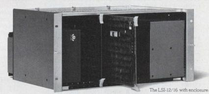
restart, remote cold start, 16 bit parallel I/O interface and up to 2K bytes of semiconductor memory.
