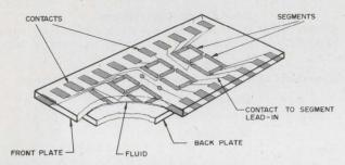
When the liquid is not electrically excited, its long, cigar-shaped molecules are parallel to one another in a position perpendicular to the plates. Thus, the liquid appears transparent. Applying an electric current creates ion activity which leads to turbulence and causes the liquid to scatter incident light. The visual effect is that of a frosted glass. LCD's can be made completely transmissive for back-lighting, reflective for ambient light or semi-reflective for dual mode operation.
