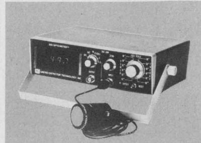
**UDT-80X Opto-Meter** offers low cost photometric/radiometric measuring capability from  $10^{-10}$  watts or  $10^{-4}$  footcandles for \$865. The 80X has  $3\frac{1}{2}$  digit readout, silicon detector, radiometric (flat 450-950 nm) photometric filters, AC and battery operation. United Detector Technology, 1732 21st St Santa Monica Ca 90404 (213) 829-3357
