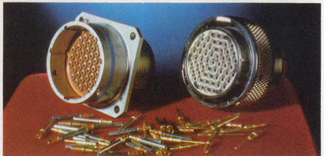
Both Amphenol's Merlin I and Bendix's Pygmy (bottom) lines feature dielectric retention discs. The discs eliminate the need for individual metal clips. This results in lighter and shorter connectors. Also, both lines employ a rear-release method for contact insertion and extraction and crimp-type terminations.
