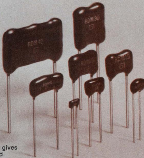
Stable because nature gives mica its conformity and volumetric efficiency. Mica capacitors are perfectly mated to the needs of communications, instrumentation and navigation circuitry. They're best suited for critical circuits requiring maximum long life stability over a temperature range of  $-50^{\circ}\text{C}$  to  $+150^{\circ}\text{C}$ . For circuits involving delay, timing and frequency discrimination.
