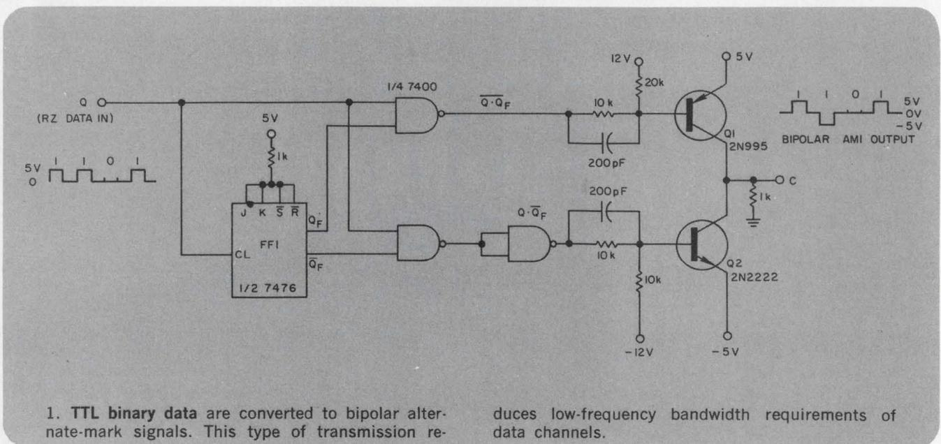
1. TTL binary data are converted to bipolar alternate-mark signals. This type of transmission re-
