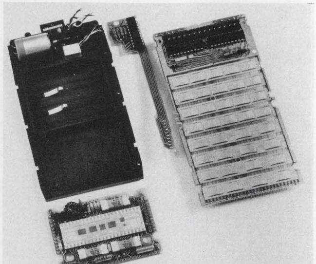
The programmable HP-65 uses hybrid techniques to accommodate 12 chips. A card reader is also included.
