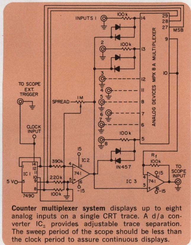
**Counter multiplexer system** displays up to eight analog inputs on a single CRT trace. A d/a converter IC<sub>2</sub> provides adjustable trace separation. The sweep period of the scope should be less than the clock period to assure continuous displays.
