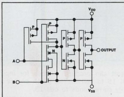
The device utilizes small geometry input and logic transistors to generate the required logic function, then utilizes low impedance output buffers.
