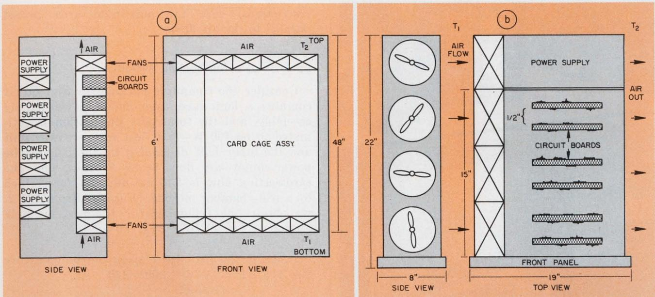
5. Multiple fan systems have advantages. A series fan configuration (a), with one set at the input port and the other at the output, provide double the pressure capability that a single set would. And the parallel arrange-
