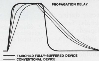
With 1, 2, or 3 simultaneous logic changes, conventional CMOS Gates exhibit differing propagation delays with input pattern. Fairchild CMOS doesn't.
