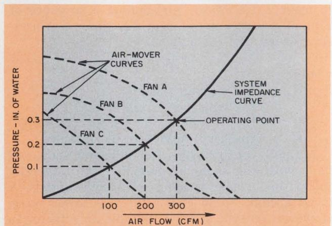
4. The intersection of an air-mover's flow characteristics curve and the impedance curve of the cooled assembly is the operating point of the system.
