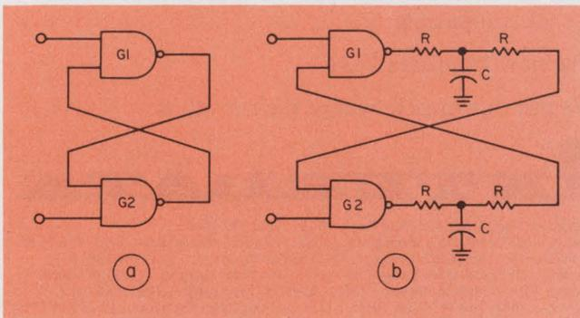
1. **Cross-coupled NAND gates** are commonly used to form the flip-flop in memories and registers (a). A simple RC T-network connected between gates can prevent the network from changing states when a nuclear transient burst occurs (b).
