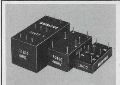
**Scott T Transformer.** 11870: 60HZ, 90v, L-L In. 1.1x2.1x1.1. 50460: 400HZ, 90v, L-L In. 7/8x1-5/8 x11/16. 50642: 400HZ, 11.8v, L-L In. 7/8x1-5/8x11/16. 10472: 400-HZ, 11.8v, L-L In. 3/4x1-1/2x3/8. All with 6v RMS sine & cosine output. MAGNETICO, INC., E. Northport, N.Y. 11731. 516-261-4502.
