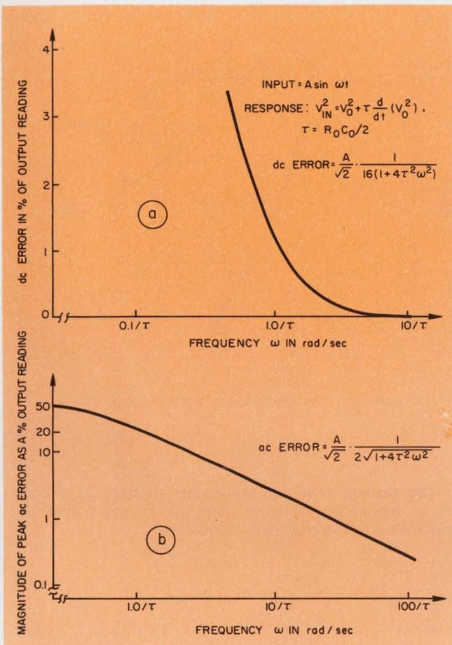
4. The dc error can be plotted (a) as a percentage of output reading; it decreases as  $\omega$  increases. The magnitude of the peak ac error if plotted (b) as a percentage of output reading, also decreases as the frequency  $\omega$  increases.
