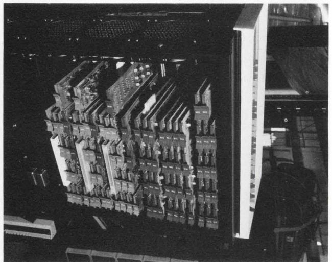
1. Most moderately-dense electronic system packages, as represented by this minicomputer chassis, use forced-air cooling. The use of several fans allows both a more uniform distribution of air and the separation of high-power portions (lower section is the power supply) from the more heat-sensitive logic cards.
