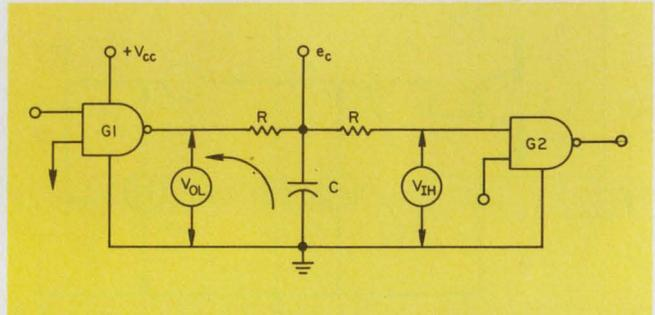
6. When a transient occurs,  $G_1$  is momentarily forced to LOW. But the T network maintains the input of  $G_2$  at  $V_{IH}$  to prevent the gate from changing state.
