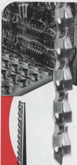
Metal Versamount for isolated boards on chassis. Card guide rivets to Versamount.
