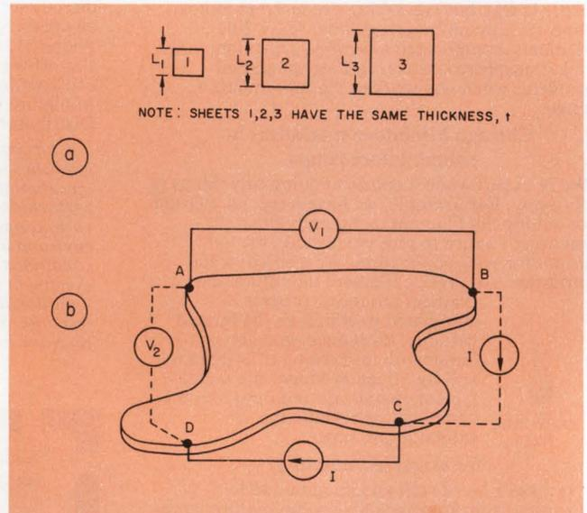
1. Measurement of  $R_{\square}$  depends on the fact that the resistance between the edges of a square sheet is independent of size (a). Thus  $R_{\square}$  can be determined from just two voltage measurements (b).
