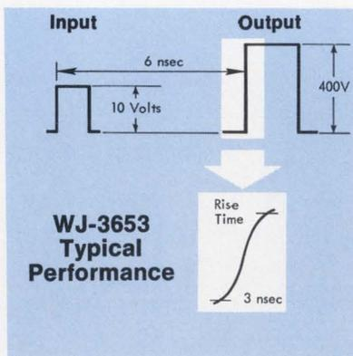
nominal 100-ohm load with less than 3.0 nsec rise time and a total delay from input pulse to amplified output of less than 6 nsec. The WJ-3653 offers over 4 A peak output current capability for operation into primarily capacitive loads.
