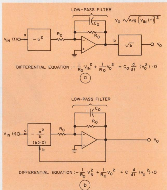
1. The direct (a) and implicit (b) methods operationally compute rms values of sine wave and other ac inputs.
