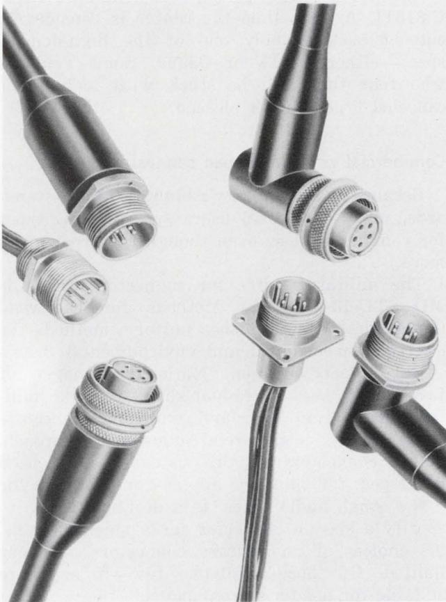
Empire Products' Cam-Lok commercial connectors are made in a non-MIL-spec, "MS style" with the cable vulcanized directly to the connector to replace cable clamps. Rigid clamps can cause breakage of cables that are subjected to continual flexing.
