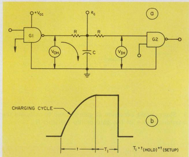
7. To maintain the maximum bit rate with the T network in the circuit (a), the charging time is calculated from the waveform across  $C$  (b).
