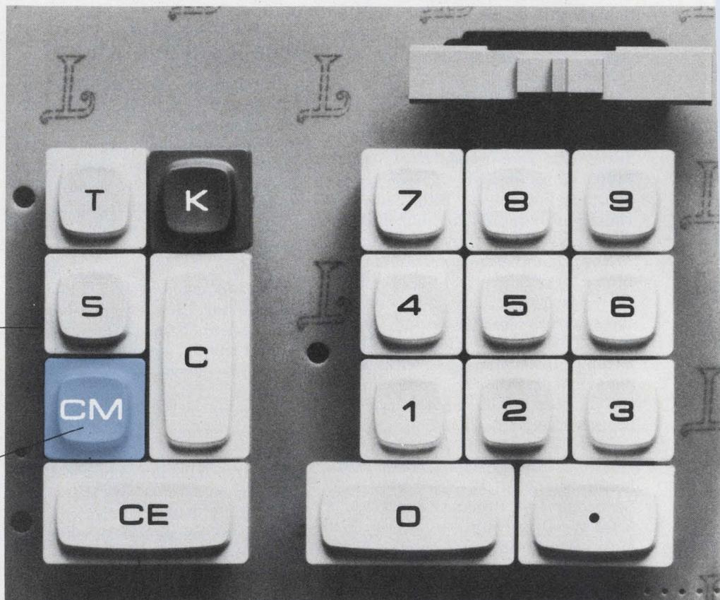
Keyswitch materials and a high length-over-diameter ratio provide the smooth, quality feel necessary for professional users.
