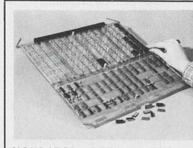
**NOVA/DCC-116 General purpose interface board** provides multiple device selection, 4 I/O registers, DMA zero word count detect, 105 socket positions for 14, 16, 24 and 40 PIN ICS. Basic board (all features of data general 4040 plus multiple device select) \$350.00. MDB Systems, Inc., 981 N. Main, Orange, CA 92667. (714) 639-7238.
