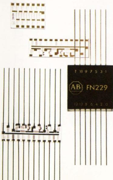
Our chrome-cobalt technology, for example, has been proven in dozens of applications ranging from D/A and A/D conversion, voltage division in digital multimeters and telemetry equipment, to communications paging devices.
