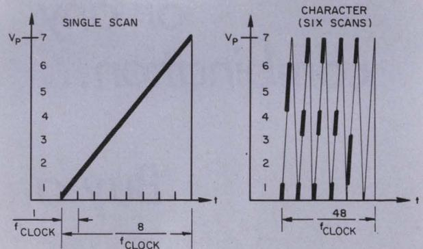
1. Series of six vertical scans provides the raster for character generation. Blank portions of the character are formed by deflection of the CRT spot off the scope face.
