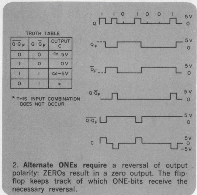
2. Alternate ONEs require a reversal of output polarity; ZEROs result in a zero output. The flip-flop keeps track of which ONE-bits receive the necessary reversal.
