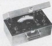
The MODEL VAW, Volt-Amp-Wattmeter, is a multirange transformed-coupled indicating instrument that (1) makes tare-free measurements of AC power, voltage and current, (2) measures all circuit parameters without the necessity of changing circuit connections, (3) has a field current rating for use down to 50% PF or 100% overload and (4) is completely self-contained in a standard portable case.
