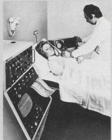
Echo interference module is used with a fiber-optic medical recorder to measure heart valve movements.
