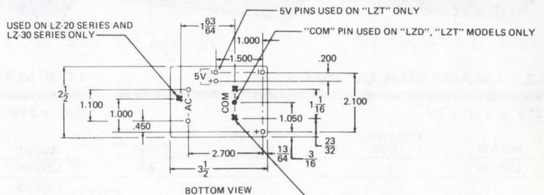
NO. 4-40 TAPPED HOLES FOR CUSTOMER MOUNTING (2 REQ'D ON LZ-10 SERIES) (3 REQ'D ON LZ-20 & LZ-30 SERIES)
