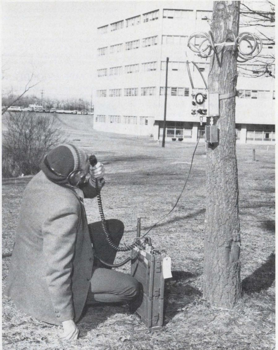
The tree above is radiating a signal at 10.803 MHz. Energy from the transmitter, operated by Kurt Ikrath, is coupled into the tree by means of a matching network in the box on the tree and the toroidal Hemic.
