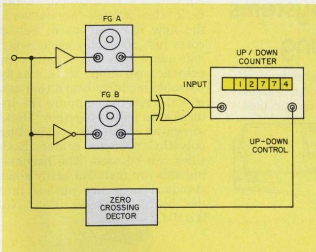
4. An up-down counter gives a direct integration of a bipolar voltage when controlled by a polarity-sensitive signal derived from the input.
