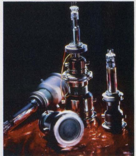
High sensitivity is characteristic of these Westinghouse camera tubes, and low-light level devices.
