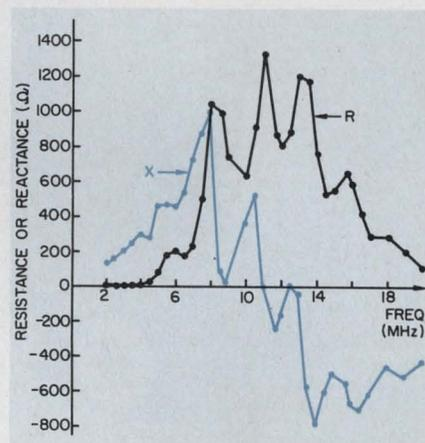
Tree-antenna resistance and reactance are shown here for an oak tree with a Hemac 2.3 m above moist ground in a forest.
