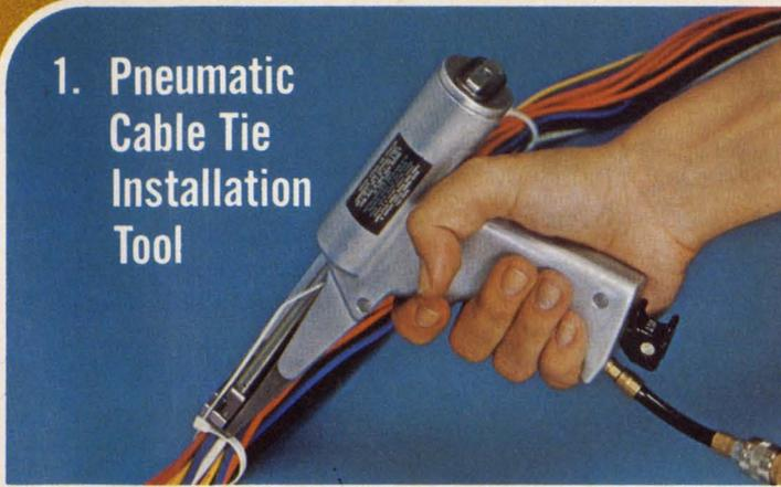
**Fast, Continuous High-volume Production** with new pneumatic cable tie installation tool ■ Lightweight PPTS air tool requires minimum force, reduces fatigue; no training required ■ Installs 36 different PAN-TY® and STA-STRAP® cable tie products ■ Uses standard 70 to 80 psi air to automatically tighten ties to pre-set tension and cut flush ■ No sharp edges—no metal barbs—no twisting ■ Ask for demonstration and lease arrangements
