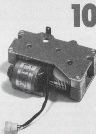
**5.** Drive for a serial printer indexes the printing ball horizontally, provides feedback through a tach generator, and accommodates vertical indexing through the hollow shaft.
