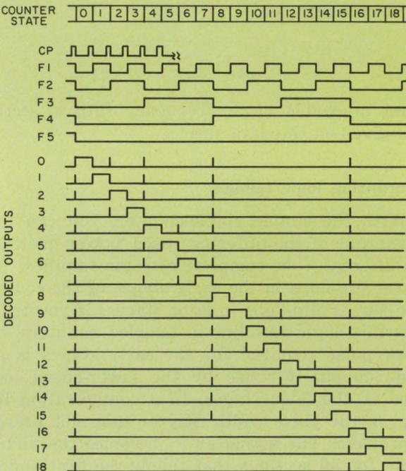
11. Glitches can occur in the identification (or decoding) of synchronous counter sections. Some of these spikes can occur on counts that precede the identified state, which is not the case with simple ripple-counters. Any of the enabling techniques gives rise to the possibility of such spikes.
