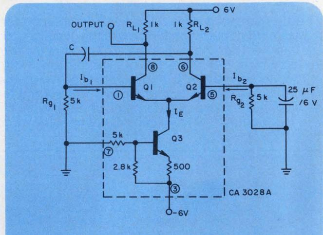
Capacitor C provides positive feedback for this astable multivibrator. Positive starts are assured since  $Q_1$  and  $Q_2$  do not saturate during their conductive periods.
