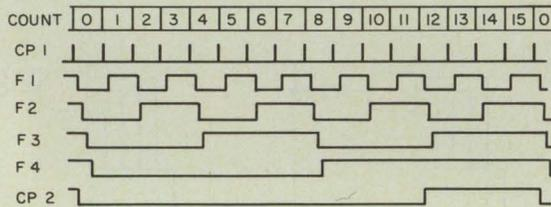
10. Secondary clock pulses should be tailored to the speed requirements of succeeding sections. The secondary clock pulse, taken from a ripple section, is modified in period and width.
