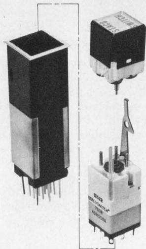
On those rare occasions when a switch malfunction shuts down equipment, STACO's Model 49 Illuminated Pushbutton Switch, with its plug-in switch module, can have things running again in less than 60 seconds. Simply flip a lever to remove the display pushbutton, and pull out the worn switch module. Slip in the plug-in replacement unit and reinsert the display pushbutton. It's that simple... and that fast!
