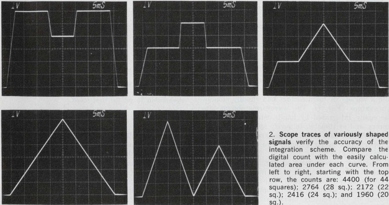
2. Scope traces of variously shaped signals verify the accuracy of the integration scheme. Compare the digital count with the easily calculated area under each curve. From left to right, starting with the top row, the counts are: 4400 (for 44 squares); 2764 (28 sq.); 2172 (22 sq.); 2416 (24 sq.); and 1960 (20 sq.).
