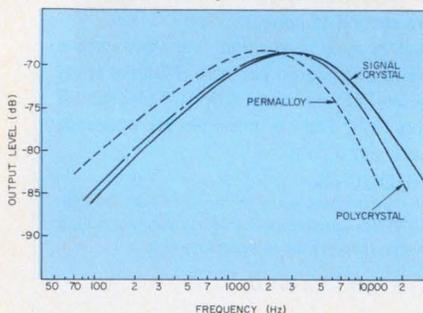
**Wear characteristics** of three tape-head materials with Crolyn tape running against the heads at 4.76 cm/s.
