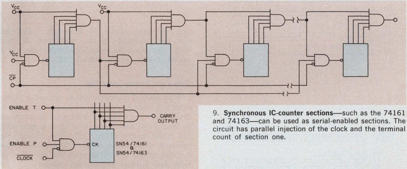
9. Synchronous IC-counter sections—such as the 74161 and 74163—can be used as serial-enabled sections. The circuit has parallel injection of the clock and the terminal count of section one.
