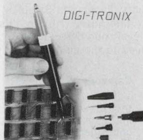
**Low cost, high performance Logic Probe Model HS 50A** for 5 volt logic. Detects and identifies polarity of single pulses to 20 nanoseconds, pulse trains to 25 Mhz. Indicates symmetry/non symmetry of pulse patterns. \$59.00. DIGI-TRONIX, 2309 Saidel Dr., San Jose, CA 95124. (408) 371-4764.
