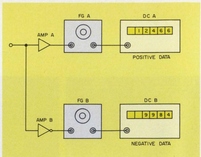
3. To integrate bipolar signals, two duplicate channels can be used. The counts of each channel are then added algebraically to get the final result.
