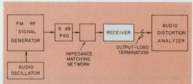
3. The SINAD measuring setup, similar to that for quieting, uses a modulated rf signal and distortion analyzer to notch out the recovered audio tone.
