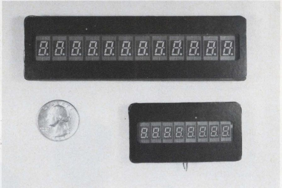
Multigit fluorescent readouts from Ise Electronics lend themselves to easy multiplexing and provide a soft green glow.
