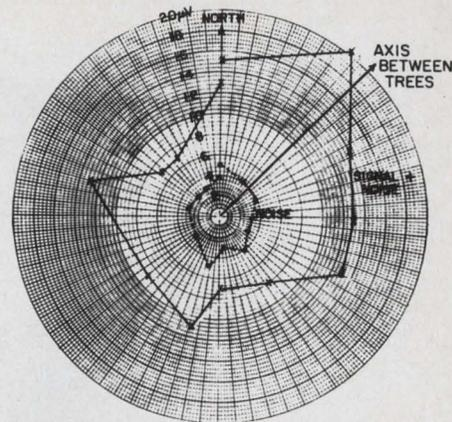
This directional pattern from two trees was obtained by controlling the phase of the energy fed them. Two Hemac couplers were used here.
