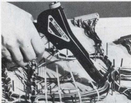
This tool accommodates the same bundle range as the TR-225. With a similar narrow nose and long barrel, it is well suited for close-up work, breakout points and in tough to reach places. This particular design gives the operator the convenience of a long tying stroke with one squeeze of the trigger... the tie is cinched to a preset tension and trimmed flush with the head. The speed of tying is good for smaller volume tying.
