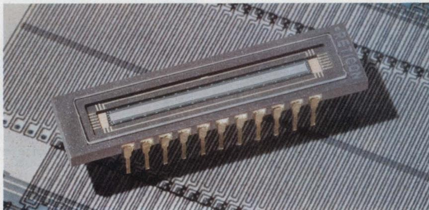
**This linear 1024-element self-scanning array, by Reticon, uses gated diodes. The diodes are sampled by shift registers that open into common drains. Linear arrays like these have been used in line-scan and area-scan cameras.**
