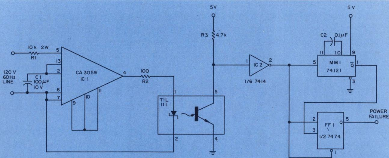
Zero-voltage switch minimizes reaction time of a power-failure detector. MM<sub>1</sub> times out and sets FF<sub>1</sub>
