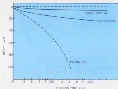
Single-crystal ferrite tape heads from Fuji Electrochemical provide much longer life than conventional polycrystalline ferrite or permalloy heads and extend record/playback response to higher frequencies at a small sacrifice in the lower frequencies.
