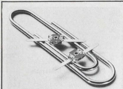
**Thin-Trim variable capacitors** provide a reliable means of adjusting capacitance without abrasive trimming or interchange of fixed capacitors. Series 9401 has high Q's and a range of capacitance values from 0.2-0.6 pf to 3.0-12.0 pf and 250 WVDC working voltage. Johanson Manufacturing Corporation, Boonton, New Jersey (201) 334-2676.
