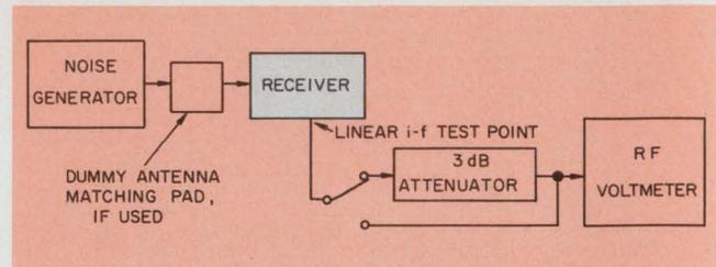
6. When an i-f prelimiter test point is available, this setup can measure receiver noise figure.
