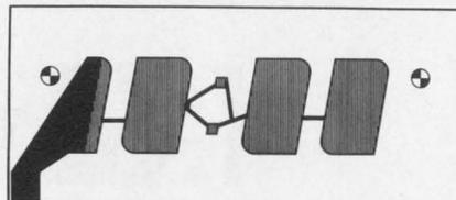
**The comb-like structure** in new field-effect liquid-crystal readouts from Ise Electronics more than doubles the viewing angle to 100° and eliminates the rainbow effect that's common in other liquid-crystal displays.
