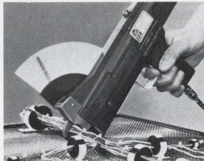
Used in conjunction with our complete series of harnessing aids (routing clamps, corner posts, breakout springs) wires are routed with few nails to facilitate both fabrication and tying.
