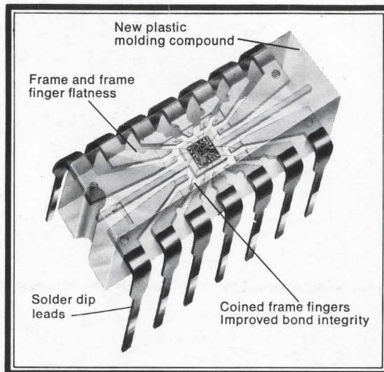
E-55 is a totally new system of plastic packaging. RCA has improved materials, handling procedures and process controls to bring you a low-cost state-of-the-art IC plastic package that matches the reliability of hermetic
