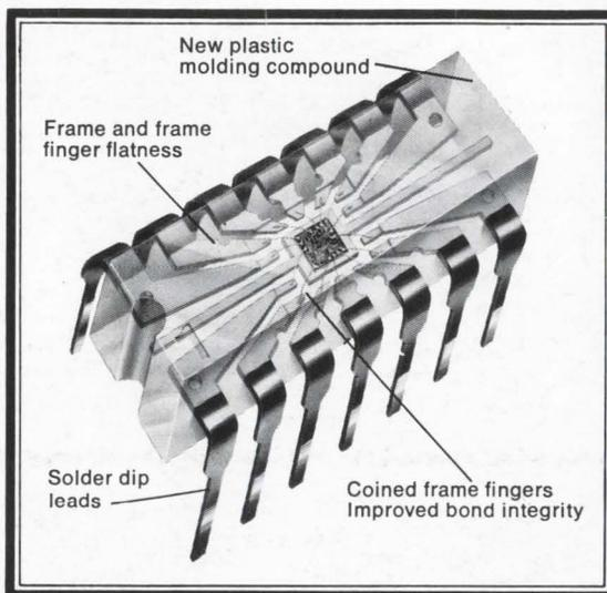
E-55 is a totally new system of plastic packaging. RCA has improved materials, handling procedures and process controls to bring you a low-cost state-of-the-art IC plastic package that matches the reliability of hermetic
