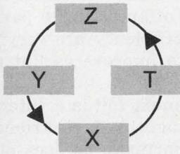
**Operational stack has 4 registers** . . . for automatic storage and retrieval of intermediate solutions. The stack design permits review of stored data at any time.
