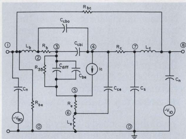
1. An rf-transistor equivalent circuit can be used for large-signal analysis or a precise determination of narrowband performance. Components  $R_{be}$ ,  $R_{bc}$  and  $C_n$  permit the handling of a wide variety of applications.
