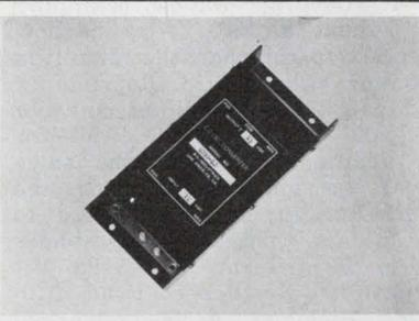
**30 watt DC/DC converter.** ±15 vdc output at 1 amp load with external heat sink. Short circuit protected. 10 mv line/load regulation. Filtered input and output. 12 V to 28V input models. Protected against input over-voltage. Size 2.7 x 5.8 x 1.2 inches. \$119 ea (1 to 9). B. H. INDUSTRIES, Los Angeles, CA, 213-479-8278.
