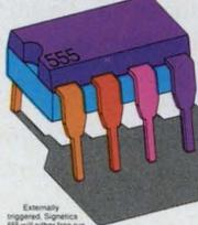
Externally triggered, Signetics 555 will either run or latch in adjustable duty cycles from 50% to 0.01%. Timing can be changed 10:1 with control. Operating from 5 to 15 volts with only a 1% change in timing. Output can source or sink 100mA. Temperature stability: 0.005% per °C.
