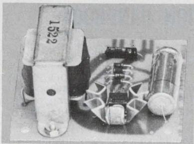
**5 watt regulated power supplies.** Low cost power supplies designed around 7800 series of voltage regulators, these units are available in 5, 6, 8, 12, 15, 18, and 24 volts with a 5 watt output rating. Short circuit protected. \$9.75 in unit quantity. ELCOM Industries, Inc., Civil Air Terminal, Bedford, Ma. (617) 274-6656.
