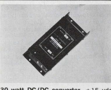
**30 watt DC/DC converter.** ±15 vdc output at 1 amp load with external heat sink. Short circuit protected. 10 mv line/load regulation. Filtered input and output. 12 V to 28V input models. Protected against input over-voltage. Size 2.7 x 5.8 x 1.2 inches. \$119 ea (1 to 9). B. H. INDUSTRIES, Los Angeles, CA, 213-479-8278.
