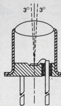
55C, and SSL-56 infrared lamp for precision beam alignment to within 3 degrees of the mechanical axis of the lamp. Power output of each of these lamps is within the less than 2 to 1 range, as published. GE will refund your purchase price or provide replacements for returned lamps not meeting published specifications.
