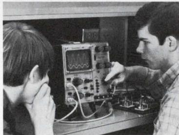
This simple to use, dual trace, 10 MHz D54 gives you low-cost, dependable performance in a wide variety of applications. Like all Telequipment scopes, it is light weight, easy to carry and is backed by Tektronix' warranty and reputation for quality. Students shown are testing amplifier circuit by measuring the gain between input and output signals.
