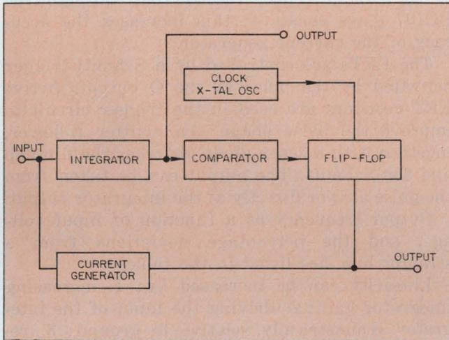
3. Using a crystal oscillator as the timing control device ensures high stability.
