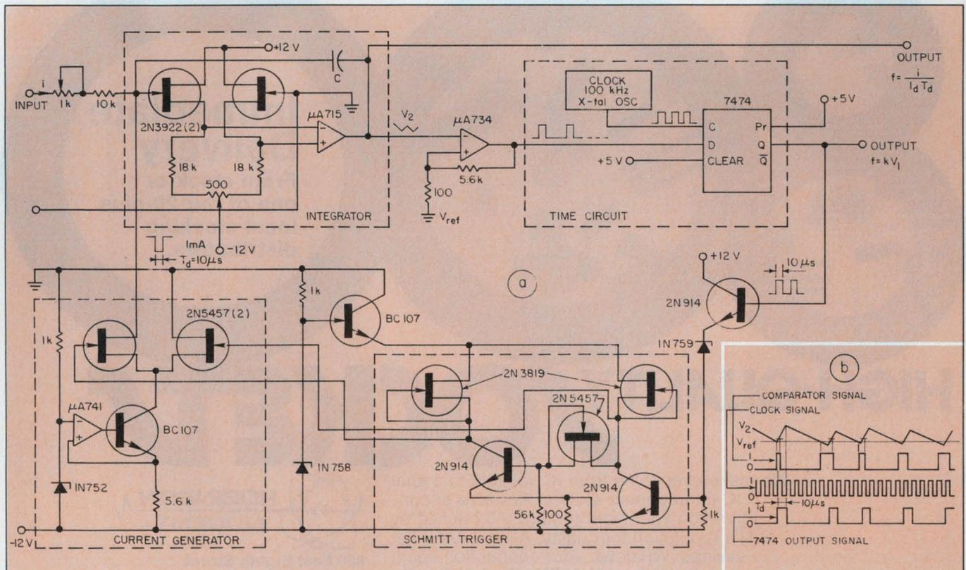
4. Complete v/f converter (a) combines FETs, ICs and bipolar transistors to achieve high linearity over a wide
