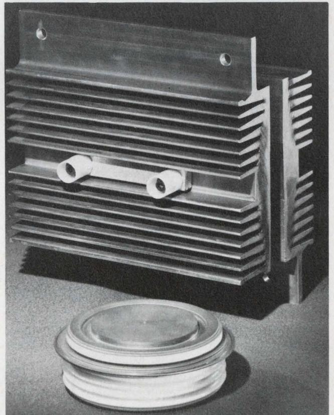
Disc packages, like the one used for Power Semiconductors' 6000-A diode, permit double-sided cooling.
