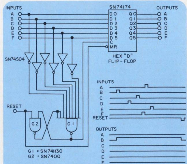
**Hex flip-flop provides a logical output** of the first pulse received. Once  $G_1$  and  $G_2$  latch, the pulse on the input line is transferred to the output of the flip-flop, and further output transitions are inhibited. A momentary ZERO on the reset line clears the flip-flop and arms the circuit for the next set of inputs.
