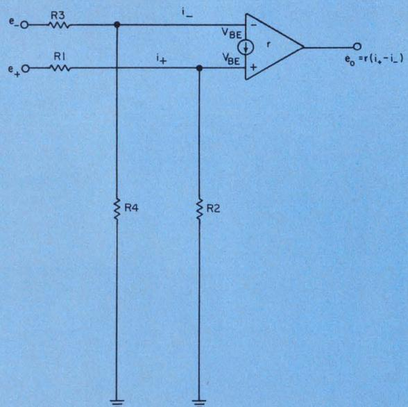
Effect of input  $V_{BE}$  on current-mode amplifiers can be eliminated if  $R_4$  and  $R_2$  are added to the circuit, provided  $R_4 = R_1$  and  $R_2 = R_3$ . The amplifier output equals a constant times the difference in input currents, as usual.
