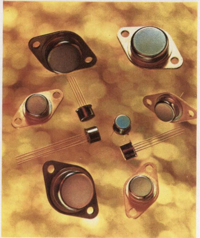
Darlington devices are gaining ground in applications formerly restricted to thyristors. Newer Darlington transistors bring out the second base to form a 4-terminal device.
