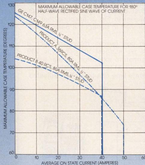
These two new SCRs have low power dissipation, providing an added measure of reliability... run at 15° C cooler case temperature than their competitive counterparts. Hermetically sealed in a 1/4"-28 stud mount package, their more compact size and more efficient operation allows the use of smaller, lower cost heatsinks.
