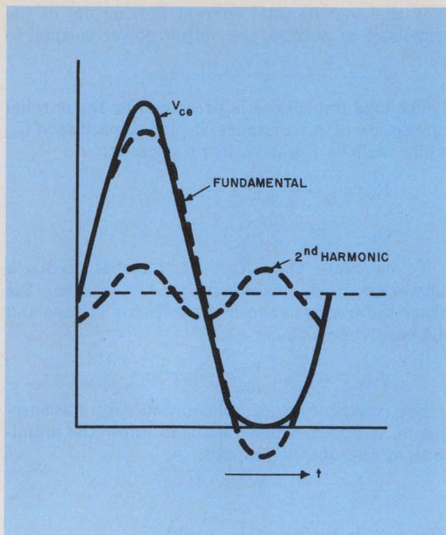
3. Harmonics can affect calculations based on the fundamental frequency, especially when an harmonic and fundamental are in phase.
