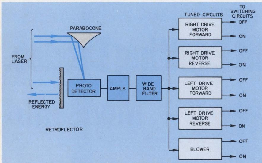
**Receiving system for laser control** reflects beam onto a photodetector. Five subcarrier signals between 10 and 200 kHz are amplified and passed on to tuned circuits that control the switching functions of motors.
