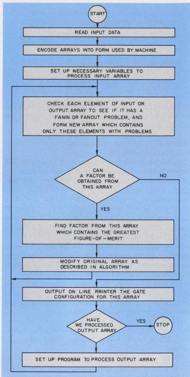
**2. Over-all program flow.** The mainline program controls the operations, reads input data, encodes the arrays and then forwards them for processing by subroutines.
