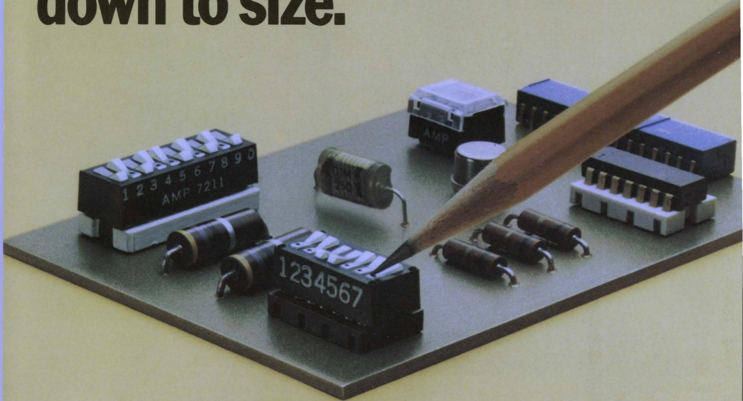
Down to the size of a DIP header — with our miniature Dual In-Line Switch. Because you can use it to program IC's right on the board without remote wiring, it cuts packaging costs, too.
