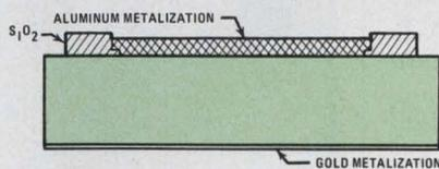
Each 37 mil square Dickson chip contains two totally passivated junctions with a 6.2 Volt or 6.4 Volt temperature compensated reference. Temperature coefficients to 0.0005%/°C are available. The chips are electrically equivalent to the JEDEC 1N821-829 and 1N4565A-4584A series.
