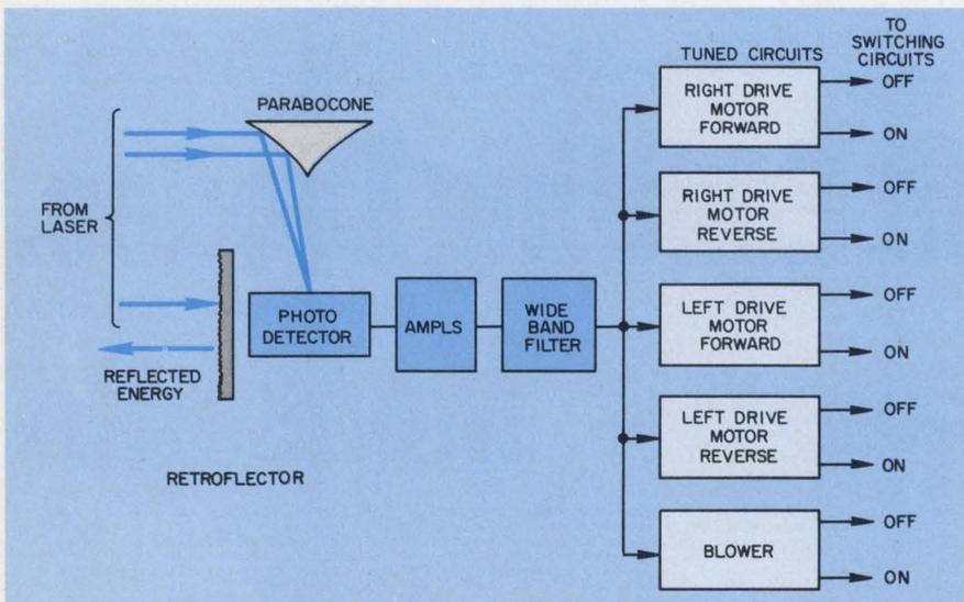
**Receiving system for laser control** reflects beam onto a photodetector. Five subcarrier signals between 10 and 200 kHz are amplified and passed on to tuned circuits that control the switching functions of motors.
