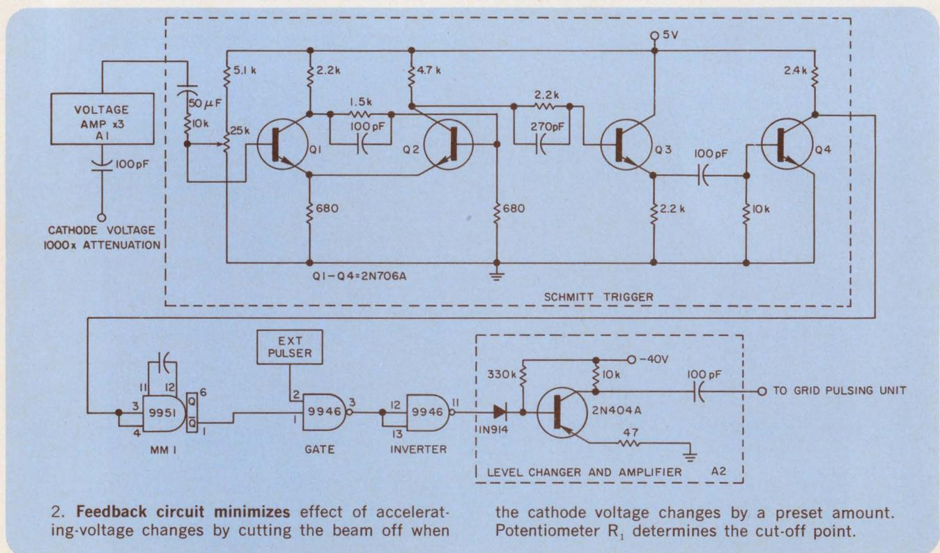
2. Feedback circuit minimizes effect of accelerating-voltage changes by cutting the beam off when
