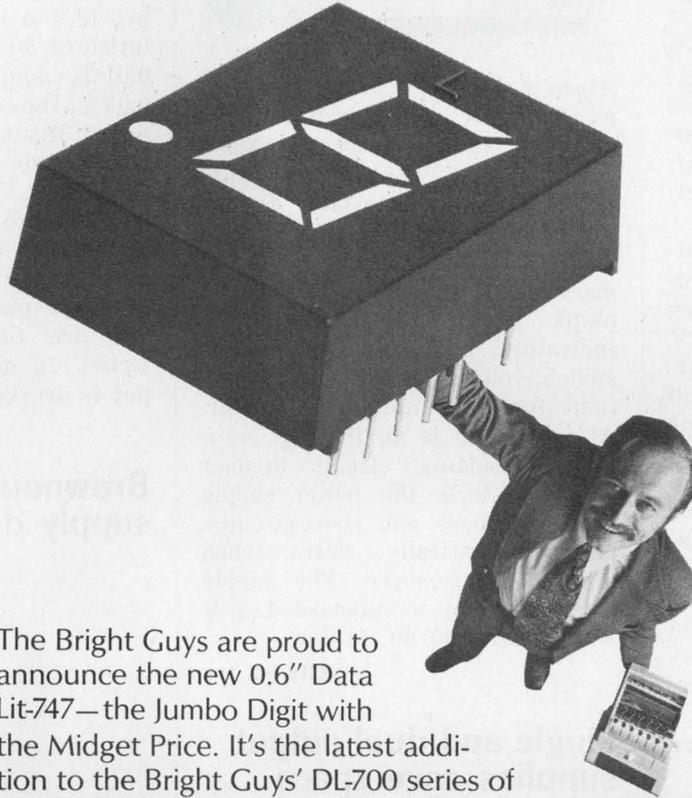
The Bright Guys are proud to announce the new 0.6" Data Lit-747—the Jumbo Digit with the Midget Price. It's the latest addition to the Bright Guys' DL-700 series of light pipe displays constructed with Litronix' Encapsulated Light Diffusion (ELD) process. It's without doubt the best digit buy of the year.
