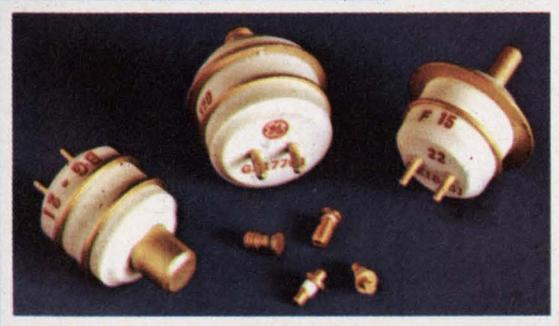
**A** GE Planar Ceramic Triodes deliver acknowledged state-of-the-art performance: thirty years' GE tube research with triodes has resulted in exceptional tolerance to the most adverse thermal, shock and vibration environments; very high ratio of power, efficiency, reliability and gain bandwidth to product size and weight; fast warmup; lower noise levels; and more efficient operation at higher frequencies.
