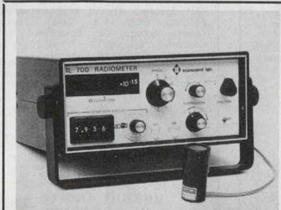
**Model IL700 Radiometer/Photometer** for the precise measurement of dc and pulsed optical radiation from the ultraviolet to near infrared. For studies in pollution, underwater spectroradiometry, densitometry and curing of U.V. sensitive polymers. International Light, Inc., Dexter Industrial Green, Newburyport, Mass. 01950. (617) 465-5923.
