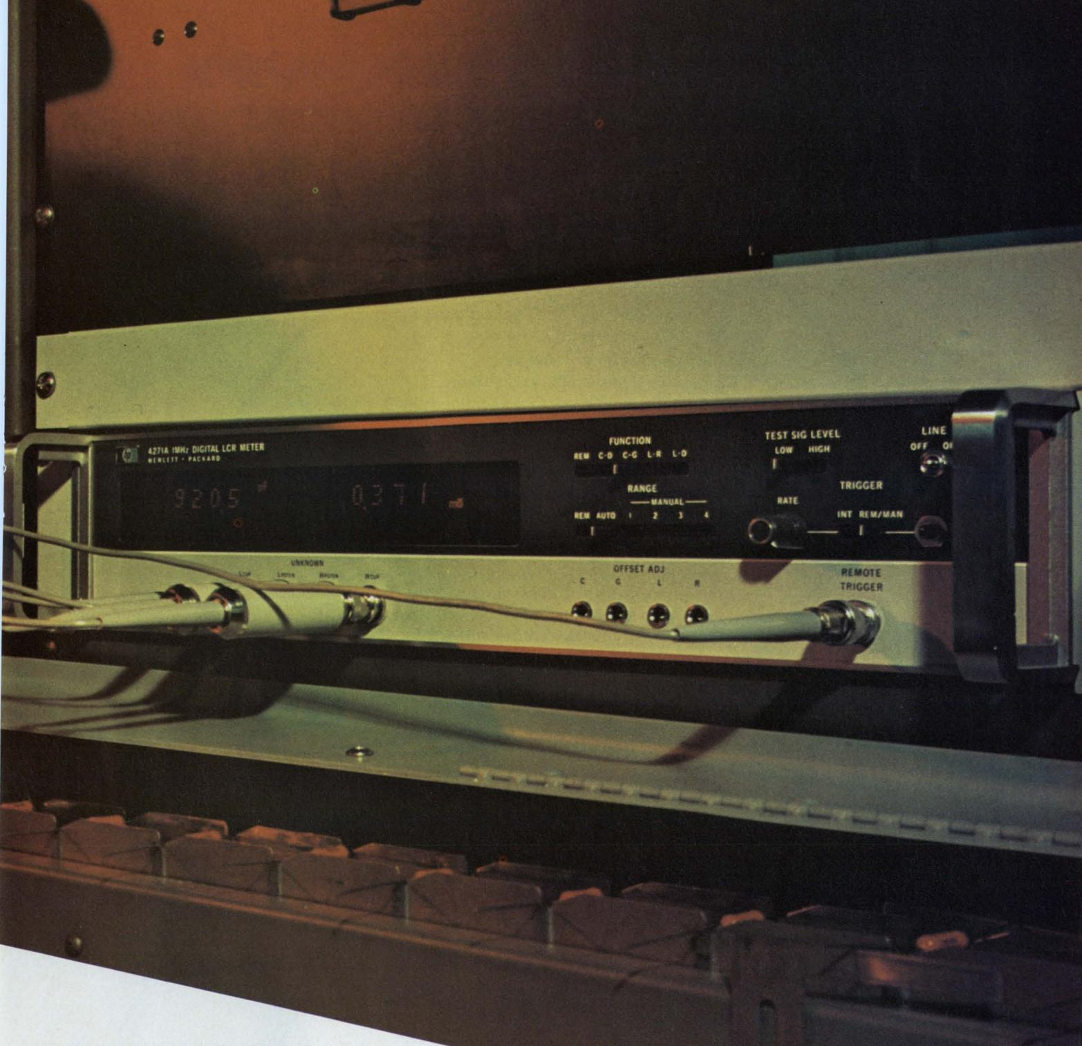
duction line. It's a snap to measure capacitance from 10.000 pF to 19.000 nF, and to measure inductance from 1000.0 nH to 1900.0  $\mu$ H. You'll also find that you can greatly simplify varicap diode testing and other kinds of micro-circuit design measurements with the 4271A and its optional DC Bias Controller. This lets you vary DC bias from 00.0V to 39.9V in 0.1V increments.
