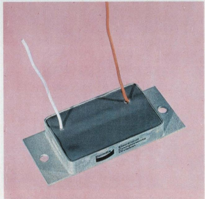
Good heat-transfer and environmental protection is provided by this silicone potting for a Bendix 3000-V silicone rectifier used in a 500-F ambient. The silicone is filled with alumina to improve heat transfer.
