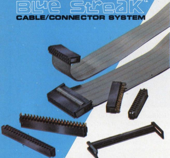
Here's Ansley's new cable for your wiring needs. It's rated for 105°C ... flame retardant ... 50 conductors or less ... .050" centers ... choice of 28 AWG stranded or solid or 30 AWG solid ... cable on 100' reels from stock! Want more features? It's color coded every fifth conductor ... separates by hand for breakouts ... connectors to match from stock.
