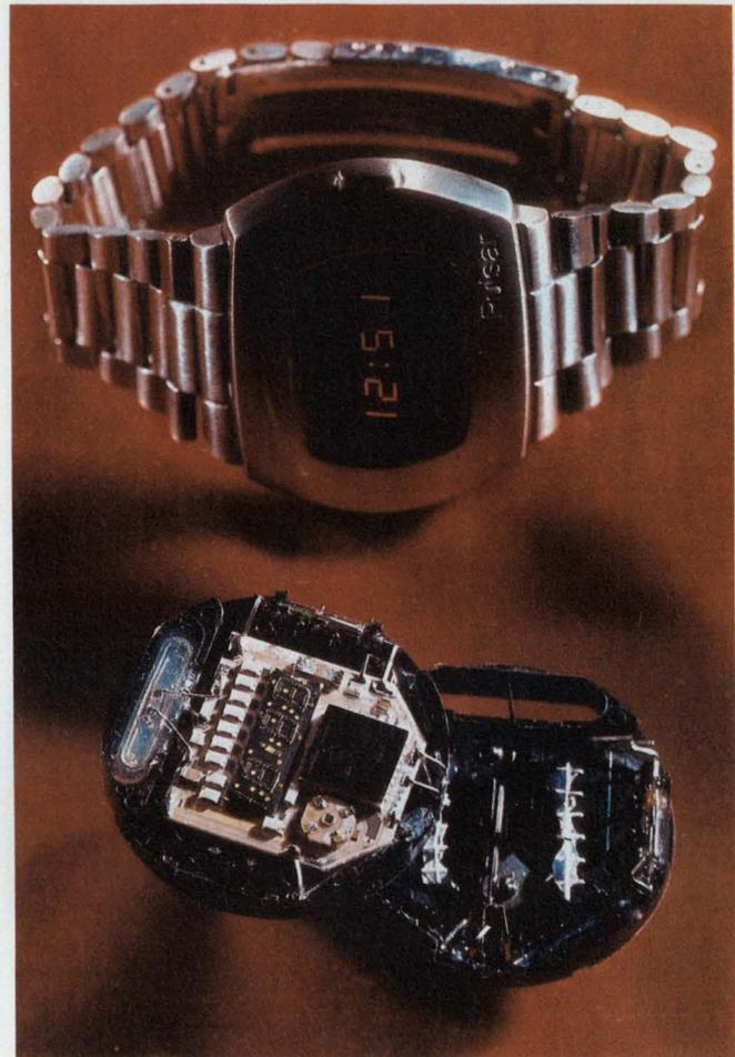
A clear Dow Corning silicone gives this Pulsar watch crystal protection against shock, while black silicone mounts the LED display. The black silicone protects the display against shock and also gives higher contrast.
