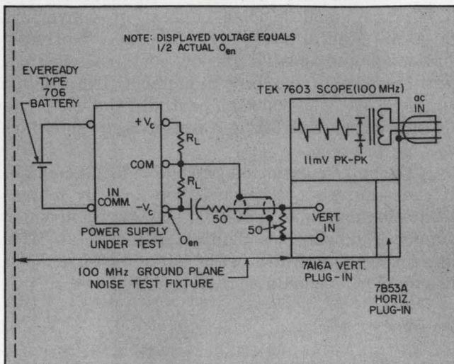
2. Converter output noise measurements, like those for high-frequency EMI, require a wide system bandwidth, 50- $\Omega$  termination and a shielded ground plane.
