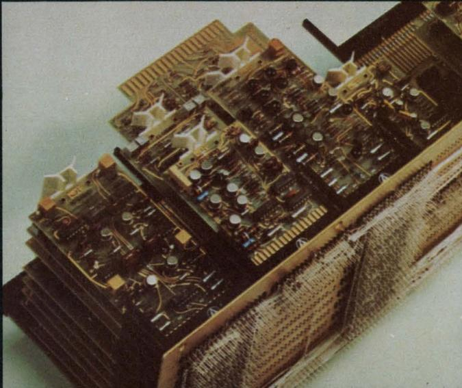
level **3** Direct entry plate assembly offers modular packaging flexibility. Custom designed plates accommodate any size or style PC board with no tooling cost to you. Rectangular posts are true positioned for automatic wire-wrapping.
