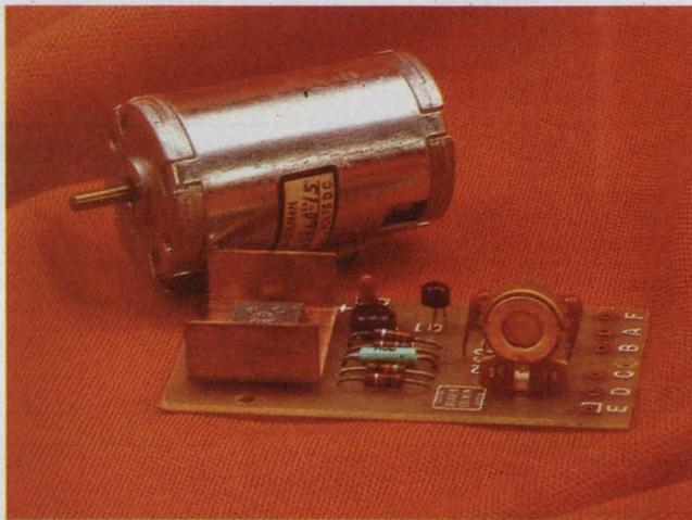
**This speed-regulated dc automotive stereo tape-deck motor** made by Barber-Colman keeps wow and flutter to 0.1%. And the speed can easily be adjusted over the range of 400 to 4800 rpm with regulation held to 1%. The motor can deliver 1.5 oz-in. at 3000 rpm.
