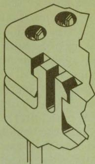
These foldover forks make contact with conductors at four points—not just two—to provide true redundancy. The cover also locks to both sides of the connector housing with
