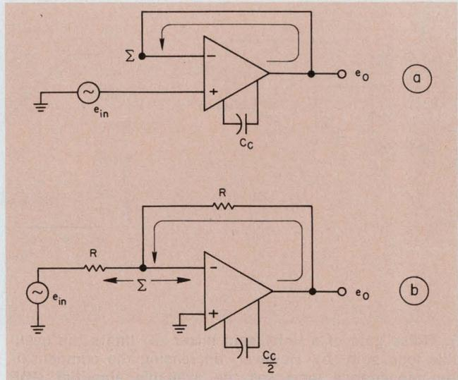
4. Both circuits provide unity operating gain. But the loop gain of the inverter (b) is half that of the voltage follower (a) because of the presence of the divider in the feedback path. The 50% reduction in loop gain with the inverter permits use of smaller compensating capacitors.
