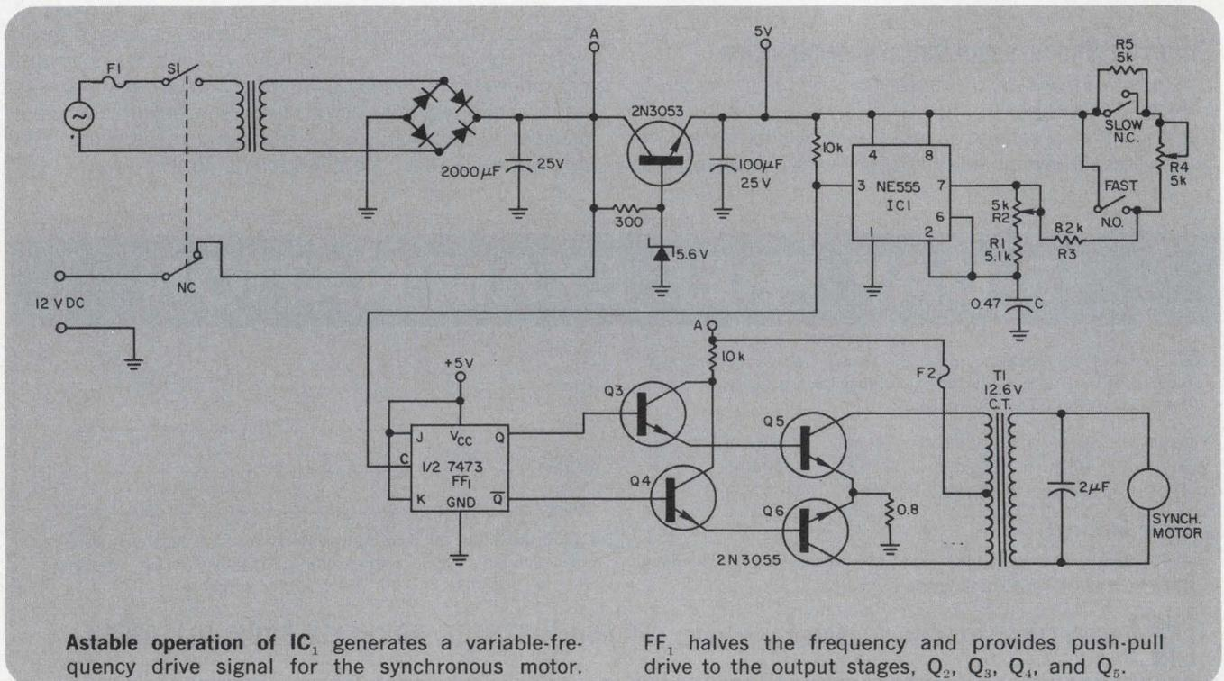
Astable operation of  $IC_1$  generates a variable-frequency drive signal for the synchronous motor.
