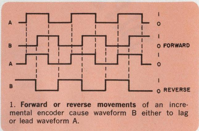
1. Forward or reverse movements of an incremental encoder cause waveform B either to lag or lead waveform A.
