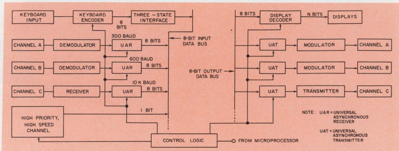
1. The determining factors in the interface design are word length, speed and priority. Transmission of dif-
