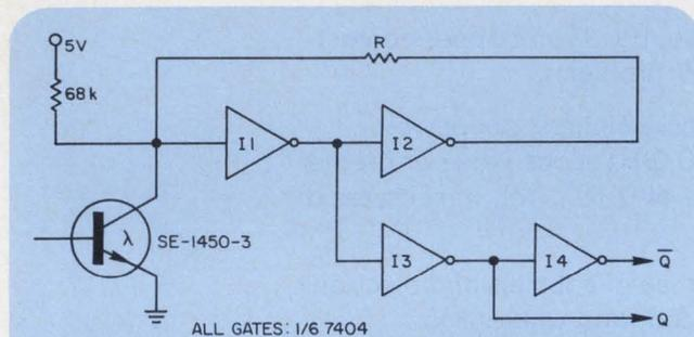
1. Optical Schmitt trigger operates with upper and lower threshold currents determined by resistor R. The controlled hysteresis prevents noise triggering during the time the beam is broken.
