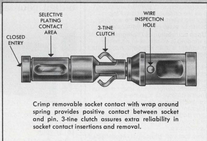
Crimp removable socket contact with wrap around spring provides positive contact between socket and pin. 3-tine clutch assures extra reliability in socket contact insertions and removal.
