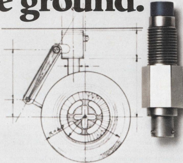
SOLID-STATE FW PROXIMITY HAS SWITCHING & SENSING ELEMENTS SEALED IN SINGLE UNIT. PROVIDES RELIABLE, NO-TOUCH SWITCHING FOR LANDING GEAR AND CONTROL SURFACE POSITION DETECTION. VARIATIONS OFFER SURFACE OR THRU-PANEL MOUNTING, HIGH-SPEED SENSING AND CIRCUITRY OUTPUT OPTIONS.
