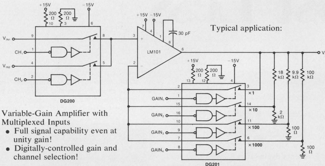
**Variable-Gain Amplifier with Multiplexed Inputs**
