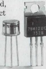
voltage tolerance better than  $\pm 5\%$ . Line regulation 0.01%/Volt. Output impedance 0.03 $\Omega$ . Output current rated at 0.5 Amp (usable to 0.75 Amp, depending on input voltage and heat sinking considerations).
