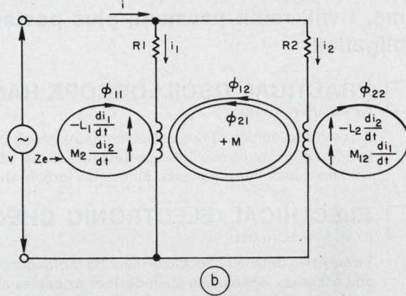
(b) Impedance of parallel branches with mutual inductance adding<sup>2</sup> (assuming constant circuit parameters).
