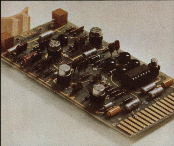
**level 1** Low-cost sockets for transistors in TO packages (above) allow easy replacement and service. ■ New IC sockets are end and side stackable for maximum single board density. Low profile design also allows maximum multi-board density.
