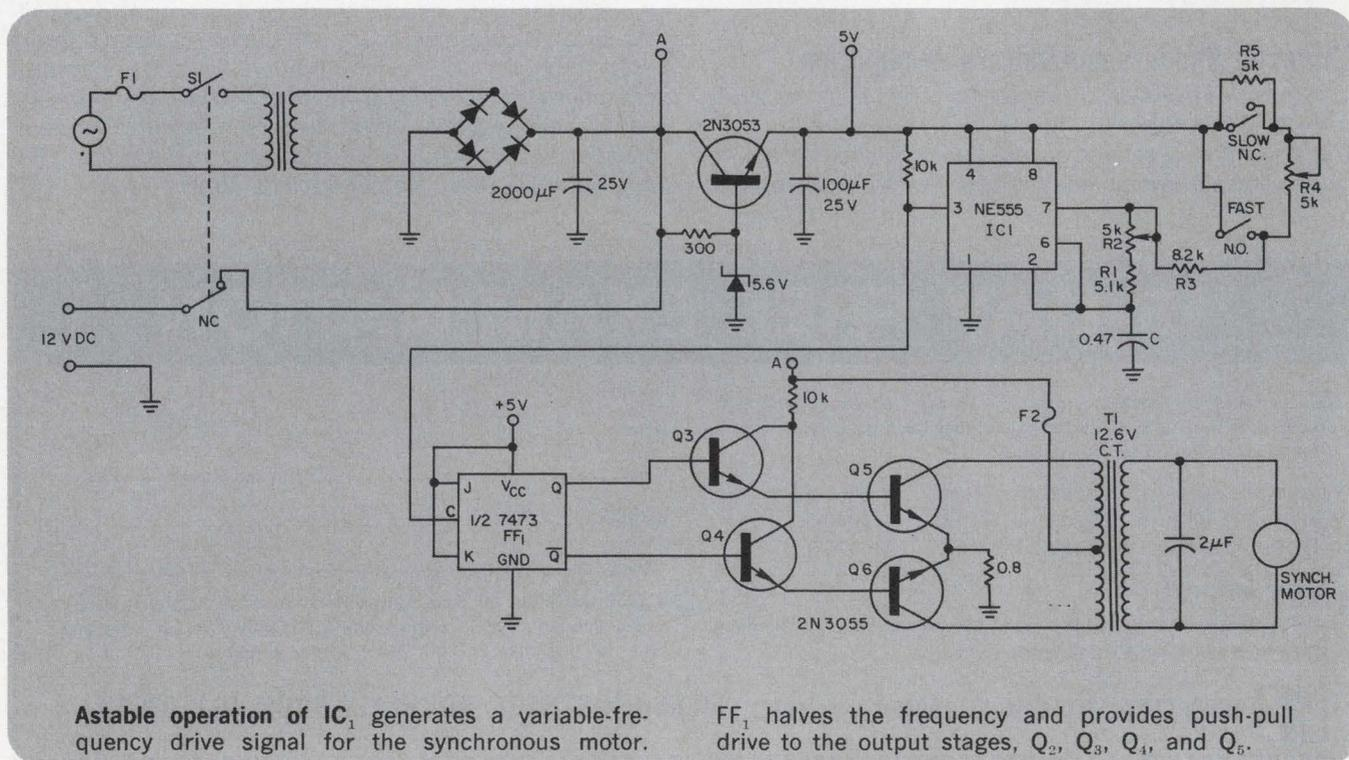
Astable operation of  $IC_1$  generates a variable-frequency drive signal for the synchronous motor.
