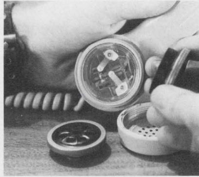
**Tiny drop-in microphone**, being held, is an exact copy of the telephone's carbon button, lying on the table. The device uses the telephone's power to transmit a third of a block.
