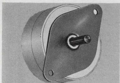
**Permanent Magnet Synchronous Motor.** Low cost motor provides torque to 10 in-lbs at 300 RPM rotor. Features electric reversability, instant start/stop, permanent lubrication, quiet operation, and compact size—2-1/4" dia. x 1-1/8" long. For computer peripherals, control devices, chart drives, and similar applications. ECM Motor Co., 1301 E. Tower Rd., Schaumburg, Ill. 60172.
