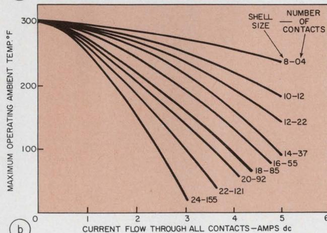
2. Maximum operating ambient temperature at sea level (a) and 110,000 foot altitude (b) with the connector cooled by natural convection.
