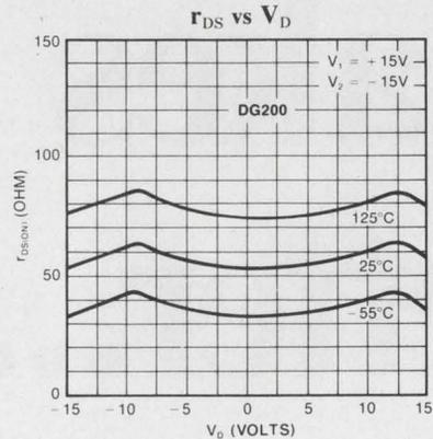
With supply voltage levels less than  $\pm 15V$ , the maximum analog signal always equals supply voltage.
