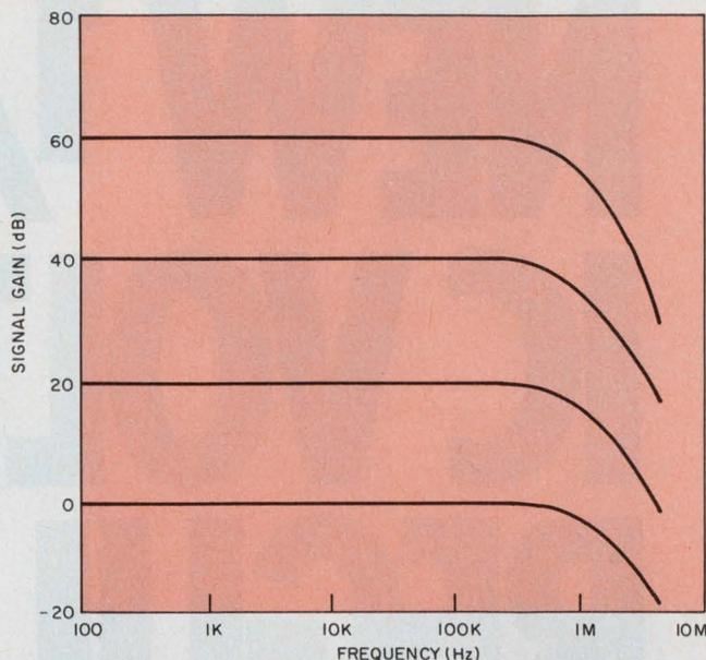
8. Use of optimum compensation for the 709 permits operation with almost constant bandwidth—a characteristic of circuits having adequate loop gain.
