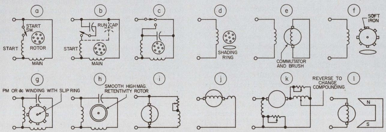
tinuous-duty running torque. For starting, special intermittent-duty windings or other arrangements can provide the extra torque. However, such a motor must also be able to handle the sudden severe current surges and attendant mechanical stresses. Also, overload protection must be provided, and the motor shouldn't be stopped and restarted too frequently.
