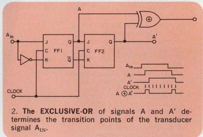
2. The EXCLUSIVE-OR of signals A and A' determines the transition points of the transducer signal A<sub>IN</sub>.
