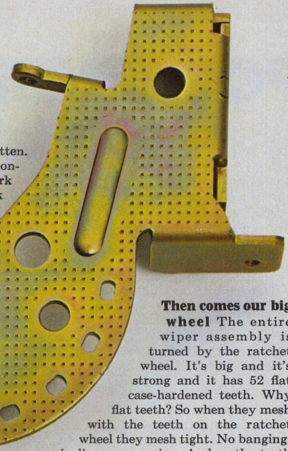
**Then comes our big wheel** The entire wiper assembly is turned by the ratchet wheel. It's big and it's strong and it has 52 flat case-hardened teeth. Why flat teeth? So when they mesh with the teeth on the ratchet wheel they mesh tight. No banging, wiggling, or scraping. And as the teeth wear, they just mesh deeper in the grooves.
