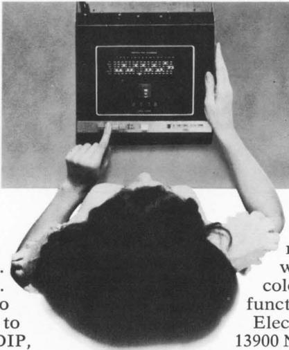
highly visible four-digit test code, is absolute. No comparison with a "good" IC is necessary. Switch settings and test codes for most devices on the market come with the instrument, along with complete instructions including how to test unlisted devices.
