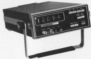
**LX-2.** We do not believe there is a competitive instrument that can match the LX-2's quality for the price. The standard model comes with four full digits—plus a fifth for over-ranging; and measures DC volts, AC volts, resistance, and multi-function ratios — automatic ranging included. Automatic polarity and range selection. Options permit BCD outputs and battery operation. The LX-2 is our fastest selling four plus digit multimeter. Mil Spec (Class II) version is designated as AN/USN-341.
