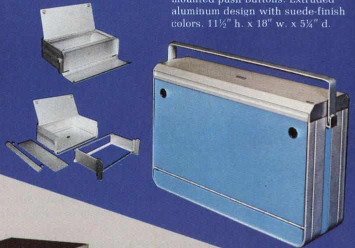
The first truly portable instrument case designed for travel. Removable chassis for assembly line component installation. Hinged control cover and handle fold neatly underneath. Top access panel opened by flush mounted push buttons. Extruded aluminum design with suede-finish colors. 11½" h. x 18" w. x 5¼" d.
