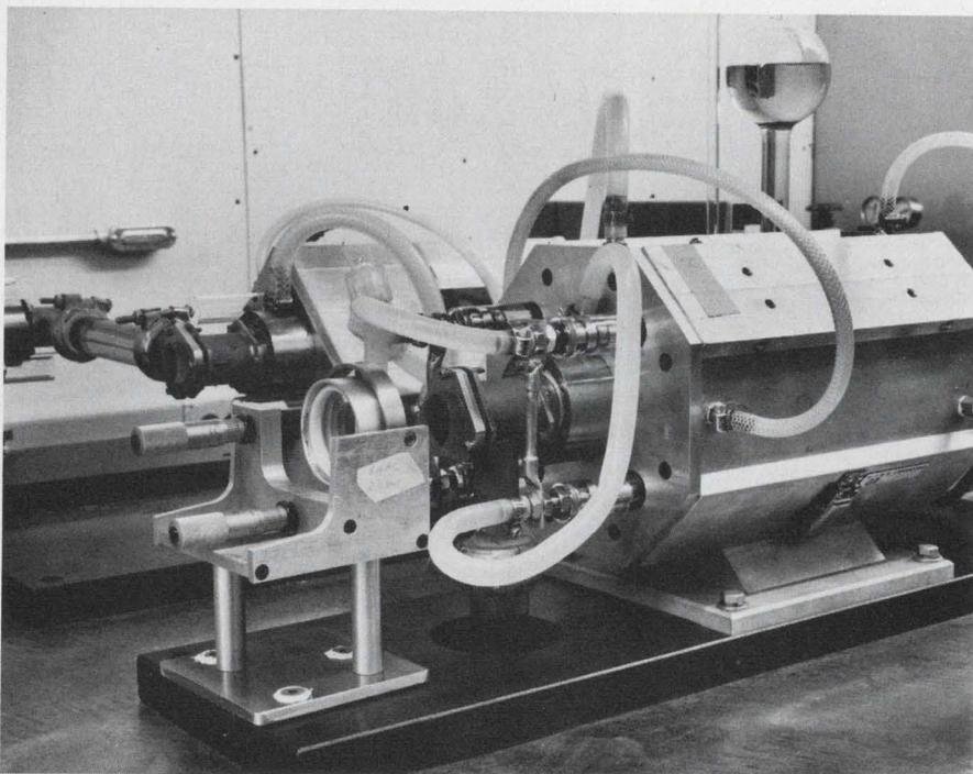
Degradation of output under high-power conditions is prevented in this high-energy liquid laser, right foreground, by using two cooling systems. One cools the laser liquid, the other cools the laser tube and flash lamps.
