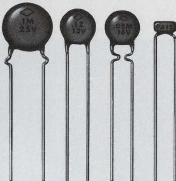
A dissipation factor as low as 3 percent maximum and high insulation resistance up to 1,000 megohms are only two critical design parameters met by Centralab Ultra-Kap capacitors. Also important is Y5F stability which is a maximum capacitance change of  $\pm 7.5\%$  from  $+25^\circ\text{C}$  over a temperature range of  $-30^\circ\text{C}$  to  $+85^\circ\text{C}$ .
