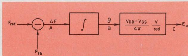
4. To derive the transfer function for the phase detector, represent it by a mathematical model with input in the frequency domain and output in the phase domain.
