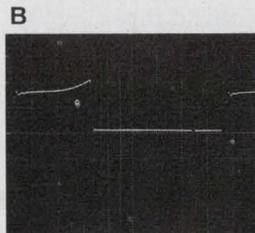
Collector current displayed on channel B. (0.1 A/div.)
