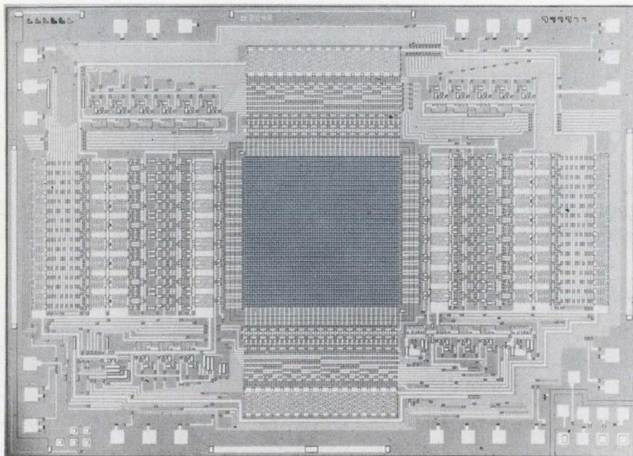
Experimental 2-k MNOS memory chip developed by Univac is organized into a 32-by-64 array (center). Peripheral circuitry includes drivers and buffers.
