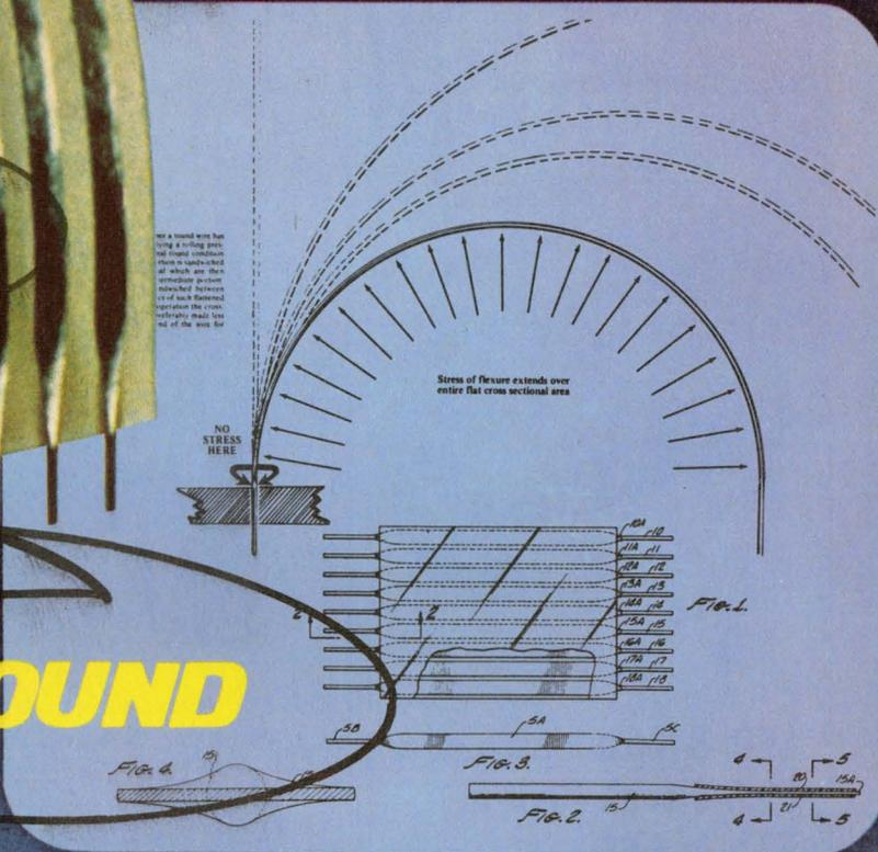
Ansley's new patented FLEX-STRIP Jumpers have flat conductors laminated between high performance insulating materials and are available from stock in thousands of part numbers. The flatness gives them flexibility where it's needed ... the round contacts insert easily into p.c. board holes or sockets. This combination of flat/round provides a generous radius when flexed, thus eliminating stress from the contacts.
