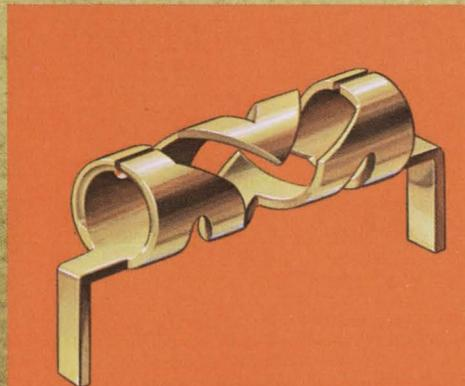
Dual chevron-shaped springs provide positive contact and grip between receptacle and pin, and minimize overall length and diameter of mated contacts.
