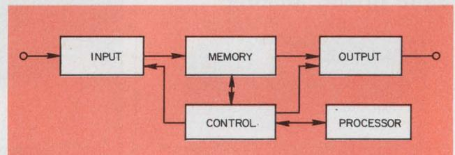
2. The basic architecture of a microprocessor. This functional diagram covers a wide range of industrial and process-control systems.
