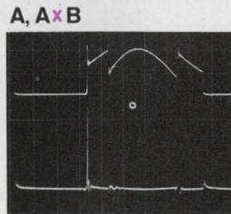
Simultaneous, two - channel display (A and A x B) reveals that the 70 watts is dissipated when transistor switches from current to voltage mode.
