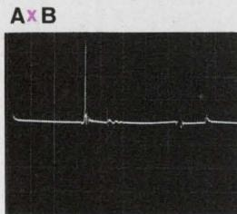
Flicking the mode selector switch to A x B now displays instantaneous collector dissipation with vertical calibration of 20 W/div. (200 V/div, x 0.1 A/div. = 20W/div.) A x B display reveals sharp power transient (70 W) not directly detectable on conventional scopes.
