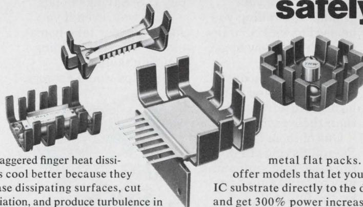
Our staggered finger heat dissipators cool better because they increase dissipating surfaces, cut re-radiation, and produce turbulence in forced air, and now they're available for IC's and microcircuits in special packages as well as standard. TO's, DIP's, .500" and .650" wide ceramics, 1"-square sealed
