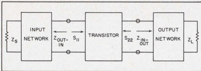
3. Source and load impedances, named  $Z_{out-in}$  and  $Z_{in-out}$ , form part of the input data for plotting against the corresponding input and output  $s$  parameters—the latter being shown as gain circles.
