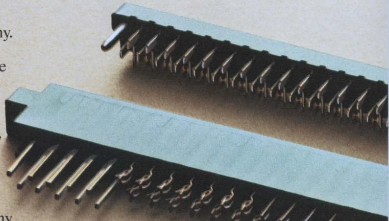
*Two-piece connector with blade-type contacts ensures maximum electrical conductivity; receptacle housing accepts crimp snap-in contacts or posts for point-to-point wiring.*
