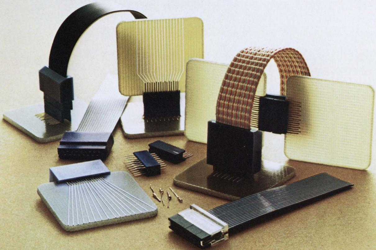
AMP chevron-shaped-contact connectors are specially designed to ensure the maximum density—and reliability—demanded in next generation microelectronic packaging designs. Chevron contact tails are suitable for .050-inch centerlines on double-sided boards or can be easily arranged to suit .025-inch centerline spacing on single-sided boards. They are available in a wide range of connector configurations for board-to-board, board-to-wire and board-
