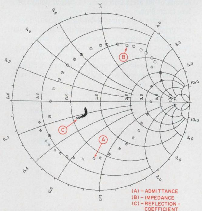
2. Any number of plots can be drawn on a single chart and identified with a separate symbol. Charts drawn by SMITHMOD have abbreviated circles at user-specified boundaries, so they give a neater appearance.
