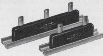
With P.I.V. from 5000 to 15000 volts, new corona free KV-PAC is designed to operate at 0.6 amp when utilized as a half-wave rectifier and 1.2 amps in center-tap, doubler or bridge applications.
