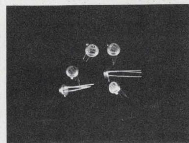
**Microwave Oscillator Transistors.** NEC types V926 and V020 are in popular TO-46 package, and use gold metallization. The V926 is rated at 400 mV output power at 1.7 GHz and the V020 is rated at 300 mW output power at 2 GHz. California Eastern Laboratories, One Edwards Court, Burlingame, California, 94010. (415) 342-7744.
