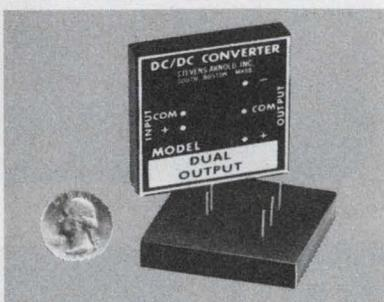
**DC/DC converter power supply.** 4.5 watts of isolated, regulated  $\pm 15\text{VDC}$ ,  $\pm 150\text{mA}$  from a 5, 12, 24, 28 or 48 VDC Input. Low noise, multiple transformer shielding and 6 sided case shield. No derating required;  $-25^{\circ}\text{C}$  to  $71^{\circ}\text{C}$ . Ultra-miniature 2" x 2" x 0.375" module. \$79 (1-9). Stevens-Arnold Inc., South Boston, Mass. (617) 268-1170.
