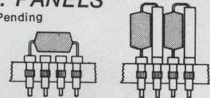
Std. DIP Mounting TIP-DIP Mounting
