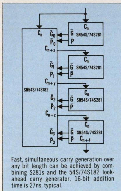
two binary numbers (see above) and can be used in multiples of 4 bits to construct whatever system size desired. It can improve performance, lower costs and reduce board space in "intelligent" terminals, machine/process controllers, minicomputers, and specialized and medium-size main-frame computers.
