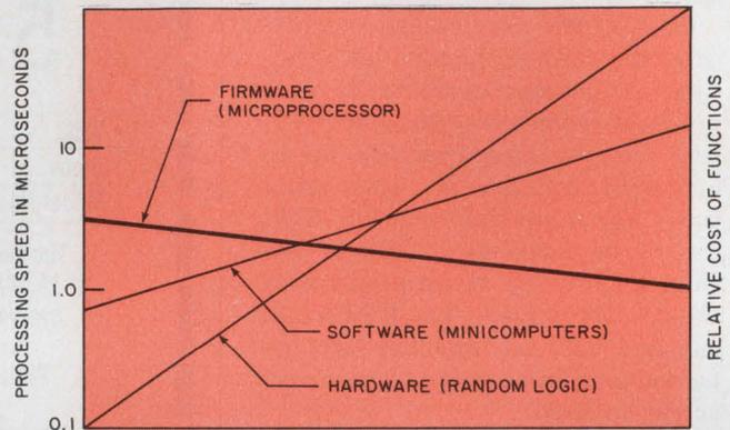
1. Microprocessors offer the lowest cost, but at the lowest speed, with system control provided by firmware. For the highest speed, but at the highest cost, random logic is the way to go. Minicomputers fall between the two approaches in this speed-cost tradeoff.
