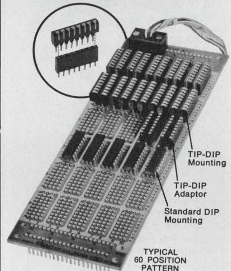
Add more IC's (up to twice as many) on Wire-Wrap panels that fit your present racks! The TIP-DIP concept: reformed DIP leads + Adaptor = more DIP's per inch and shorter wire lengths for faster switching. Standard or Custom Panels. Press available for bending leads.
