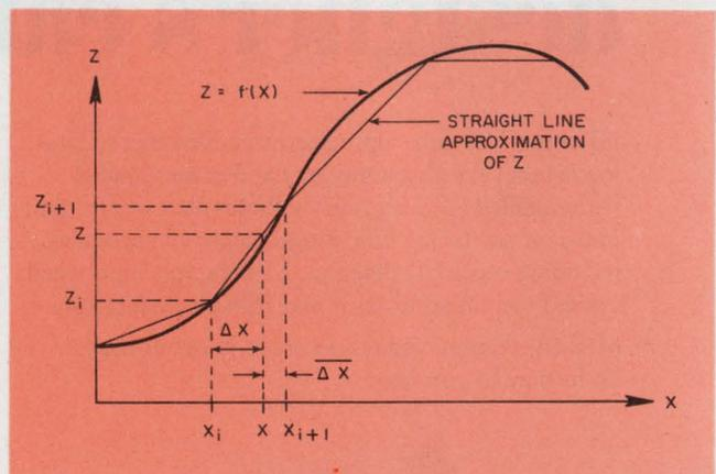
2. Interpolation is a useful technique for providing a limited number of additional decimal places of accuracy between stored values of a function.
