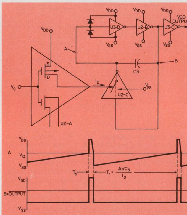
5. The VCO operation is explained by a simplified block diagram and waveforms during one complete cycle. Diodes in the diagram represent the internal CMOS protection circuit.
