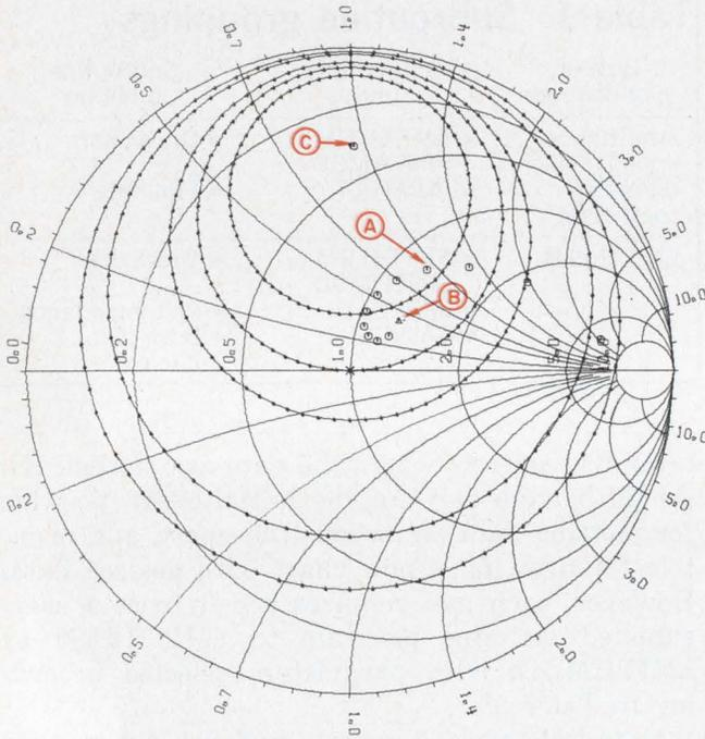
4. Smith Chart plus input gain-circles for 1, 0, -4 and -6 dB. The five circles are plotted for  $s_{11}$  and  $s_{22}$  values at one particular frequency, but the effective source impedance (A) is plotted over a range of frequencies. The largest circle corresponds to -6 dB. The start of the impedance plot is marked by the triangle symbol (B); the lone symbol (C) lies on the line-of-centers (between itself and the center of the chart).
