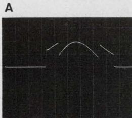
Collector voltage of the power transistor in a DC-DC converter is displayed on channel A of the PM3252. (200 V/div, 0.5  $\mu$ sec/div.)
