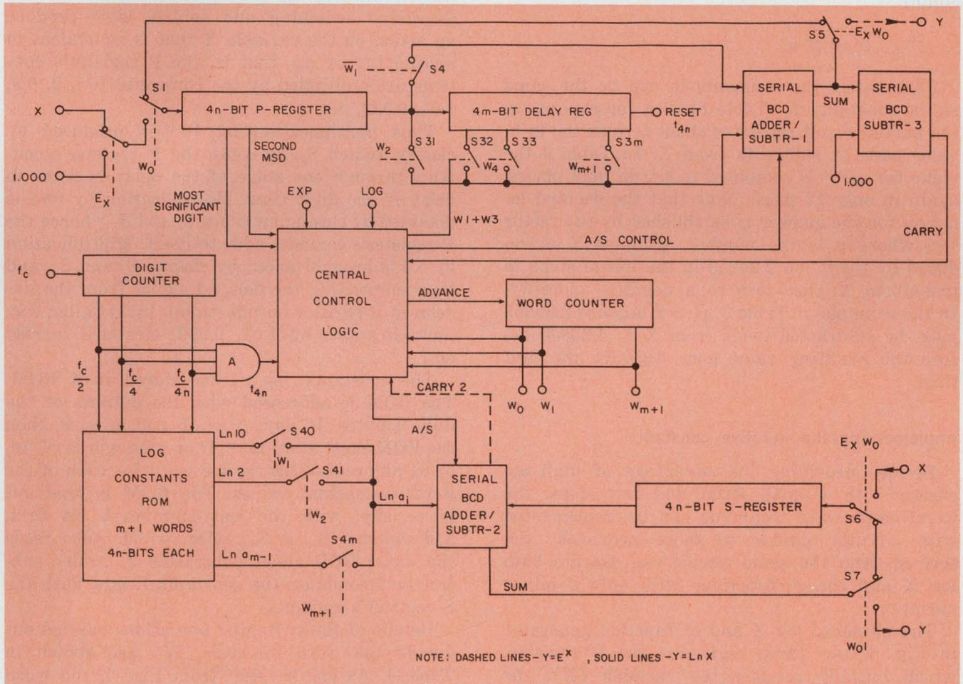
4. With only a short table of iterative constants stored in a ROM, both the logarithm and exponential functions
