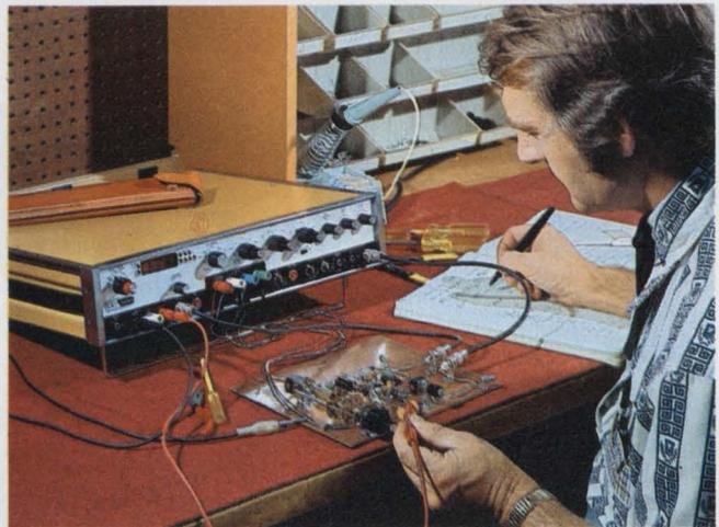
**Bread-board gated oscillator is being evaluated on Systron-Donner's Versatester I. Five test instruments are contained in the Versatester—a pulse generator, sine-wave oscillator, frequency counter, multimeter and three test power supplies (Session 18).**
