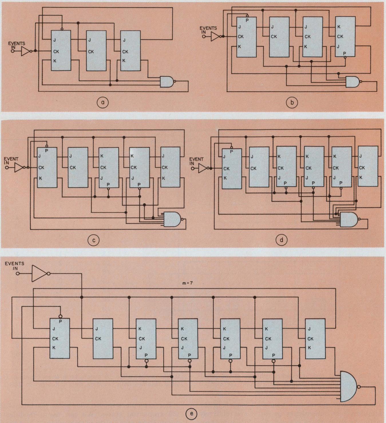
2. Self-correction is added to a residue counter in two ways: by the configuration of its connections and by the
