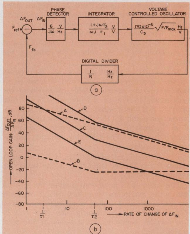
6. In PLL stability analysis, the PLL can be represented by its open-loop block diagram (a). The corresponding Bode-plot is shown in (b). The open-loop gain,  $F_{out}/F_{in}$ , varies as a function of the rate of change of  $F_{in}$  in radians per second.
