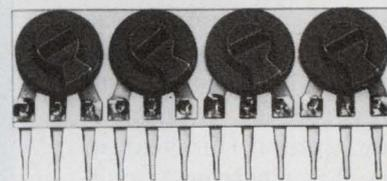
Centralab Slim-Trim carbon and Centrim cermet trimmer resistors give twice the wattage capability of phenolics, yet cost no more. Ceramic substrates mean higher wattage in a smaller space. Plus the ability to withstand high operating temperatures without shrinkage. No flux migration during flow soldering either.
