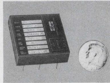
**VCXO at freqs.** from .00005 Hz to 50 MHz freq. tol.  $\pm .0005\%$   $0^{\circ}\text{C}$  to  $+50^{\circ}\text{C}$ , control voltage range  $+4\text{V}$  to  $-4\text{V}$  changing freq. 20 ppm/V, linearity  $\pm 2\%$ , 1.75" sq. x 0.5", Supply 5Vdc  $\pm 1\%$ , Sq. wave 2.4V into 200 $\Omega$  at Vdd = 5V, stock to 5 weeks; Connor-Winfield Corp., West Chicago, Ill. 60185, Tel. 312-231-5270.
