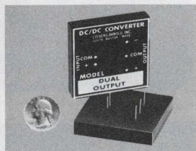
**DC/DC converter power supply.** 4.5 watts of isolated, regulated  $\pm 15$ VDC,  $\pm 150$ mA from a 5, 12, 24, 28 or 48 VDC Input. Low noise, multiple transformer shielding and 6 sided case shield. No derating required; -25°C to 71°C. Ultra-miniature 2" x 2" x 0.375" module. \$79 (1-9). Stevens-Arnold Inc., South Boston, Mass. (617) 268-1170.
