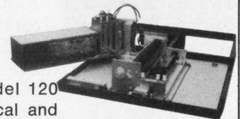
The complete OEM Model 120 printer contains mechanical and electromechanical components, interface, control logic, character generators, motor drive circuitry, and a tractor feed paper transport.
