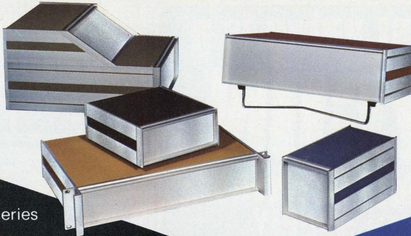
Buckeye's ingenious assembly concept of anodized aluminum extrusions gives these instrument cases strength and flexibility for configurations in all industry standard heights from 3½" to 10½". For rack mounting or bench work, using retractable locking tilt-stand.
