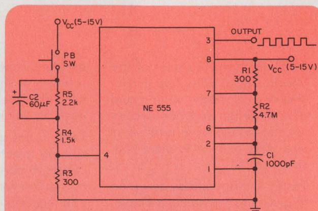
Depressing the pushbutton provides square-wave tone bursts whose duration depends on the duration for which the voltage at pin 4 exceeds a threshold. Components  $R_1$ ,  $R_2$  and  $C_1$  cause the astable action of the timer IC.
