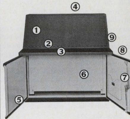
1. 24", 36", 48", or 60" width. 2. Hinged sloping control panel. 3. Optional writing desk. 4. Instrument panel top available. 5. Neoprene gaskets for complete oil tightness. 6. Accessory subpanel. 7. Three-point latches and key-locking handles. 8. Doors on both front and back. 9. All seams continuously welded. 10. NEMA-12 construction. 11. Many modifications available. Write for Bulletin C-14.
