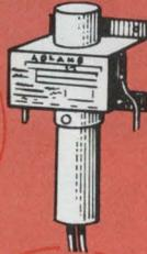
Time delays from 0 to 20 minutes; N.O. or N.C. slow "make" and N.O. slow "break" switching. AC and DC operated units, -37 to 200°F operating temperature range. 0.5-15 ampere ratings, non-inductive at 115 volts, 60 Hz. Screw terminal or pigtail leads. U.L. listed types.
