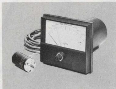
**Control Meter Relay Speed Indicating System** for use in process & control machinery. Adjustable single/dbl set pt systems, accuracy  $\pm 2\%$  full scale, repeatability 0.5%, speed ranges 10rpm to 12,000rpm. Dbl set pts adjust to 0° ea other. Servo-Tek Products Company, 1086 Goffle Road, Hawthorne, NJ 07506 (201) 427-3100.
