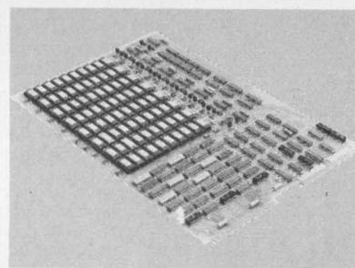
**Low cost semiconductor memory system monostore IV/Planar 4K x 20** on a single card 9-3/4" x 14". Cycle 650 ns. Includes timing control, refresh, address register, decoding, sense and memory array. TTL compatible. 0.5" card spacing. 4Kx16 \$900 from stock. Monolithic Systems Corp., Englewood, Co. 80110 (303) 761-2275.
