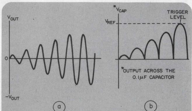
2. Typical output signal from the bandpass filter (a) contains only the desired ultrasonic frequencies. Peak-detector output voltage (b) builds until it reaches  $V_{REF}$ , the trigger level of the comparator.
