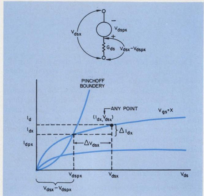
5. The origin of any  $V_{gs}$  curve is set at the pinch-off boundary to maintain the needed continuity along the boundary. Voltage source  $V_{dsp}$  is used to account for the difference between this origin and the actual one.
