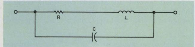
3. No component can provide a pure impedance, whether resistive, capacitive or inductive. Each one of the three passive components has, to some degree, the characteristics of the two others.
