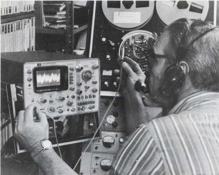
Here, a 1703A storage scope is used to check the audio circuits in a videotape machine
