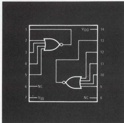
Pin for pin compatible with CD-4002A.
