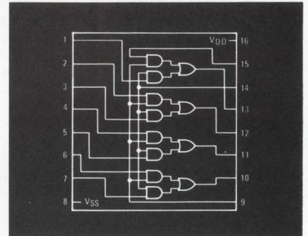
Pin for pin compatible with CD-4019A.
