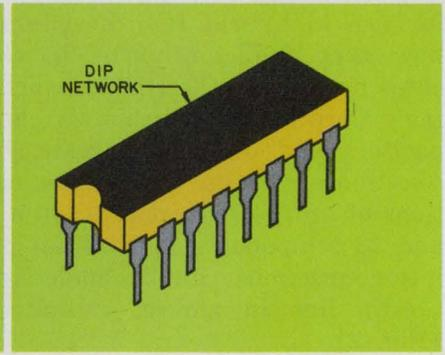
2. For compatibility with popular DIP circuits, passive components are also packaged in DIP form, as in Corning's Cordip line. Custom network designs, and an
