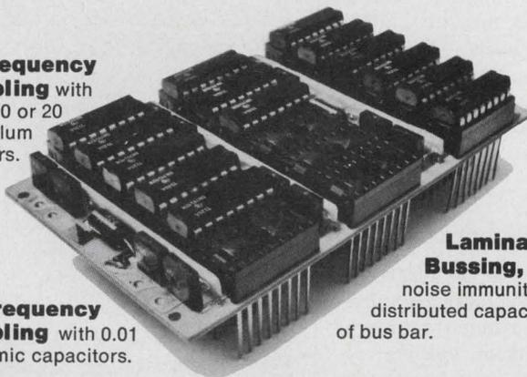
**Laminated Power Bussing**, maintains high noise immunity. 40 to 80 pf of distributed capacitance per inch of bus bar.
