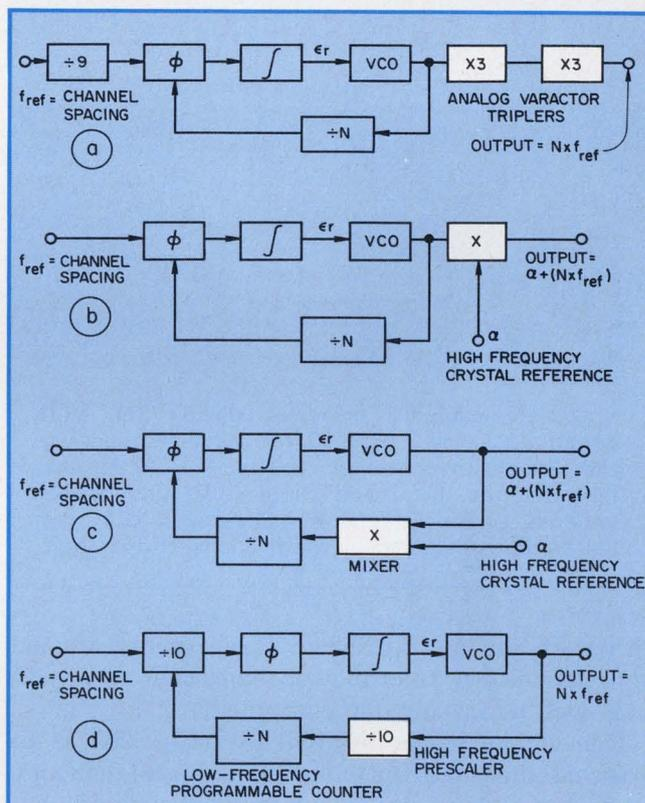
2. Higher frequencies can be obtained by multiplying the VCO output (a), by adding a serial mixer to produce a suitable offset frequency (b), by adding a mixer in the loop (c) or by inserting a high-frequency prescaler into the feedback loop (d).
