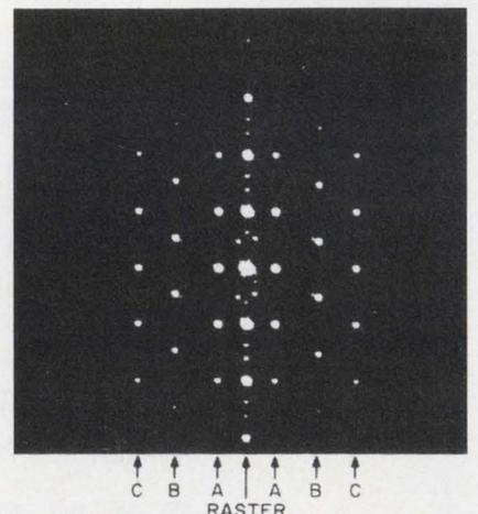
3. Synthetic gratings formed by modulating laser with three carriers have a unique white-light pattern.
