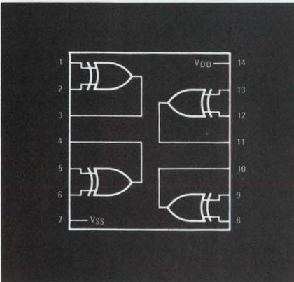
Pin for pin compatible with CD-4030A.
