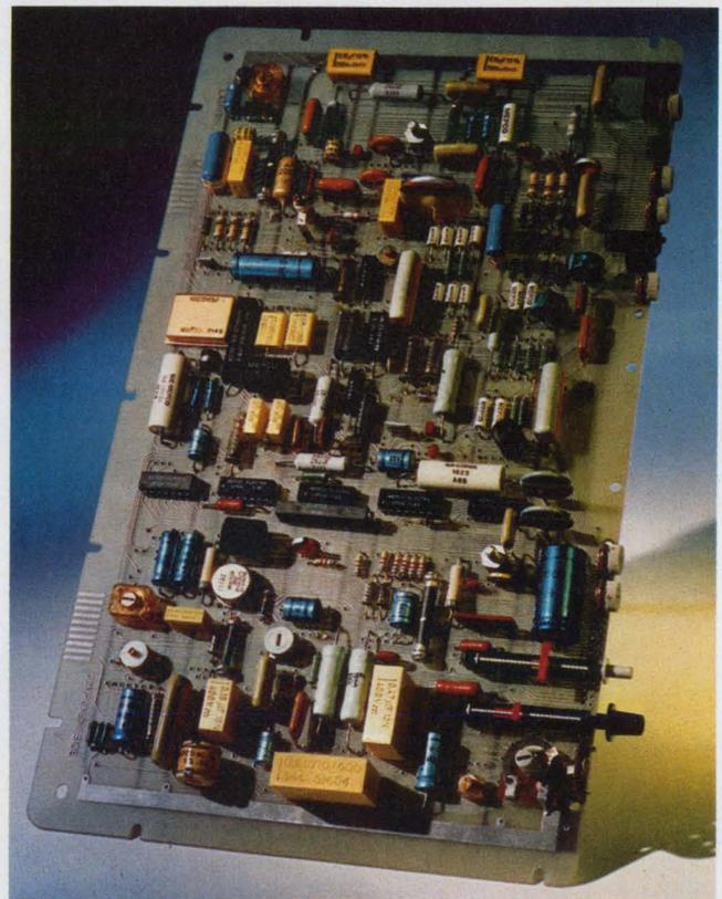
Conventional components are being used side by side with the latest chip, thick-film and thin-film networks in dual-inline packages as on this Mepeco PC board.
