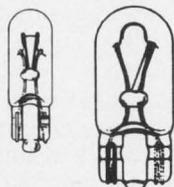
its big brother — the T-3¼ wedge base lamp with a .405" max. diam., the filament is always positioned in the same relation to the base.
