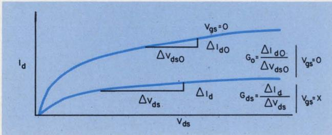
3. Conductance in the pinch-off region is normalized to the  $V_{gs} = 0$  curve slope,  $G_o$ . This conductance can be interpolated from manufacturers' curves.
