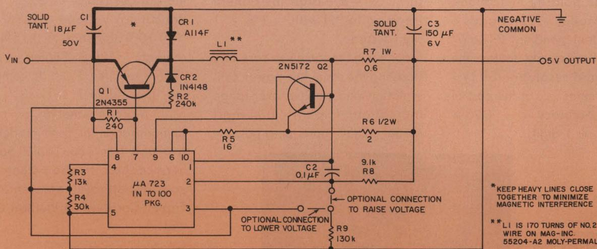
Switched regulator with current limiting can deliver half an amp using a low-cost plastic-packaged out-
