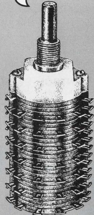
There's no better value than a Stackpole rotary switch. Fast delivery and quality features, but at a price you can afford. Unique design achieves a totally enclosed rotary, without sacrificing complex switching capability. Rigid construction and molded terminals produce a switch so tight it's explosion proof. Samples immediately. Production quantities in 1 to 2 weeks. Including switches with PC mounting. For details, send for Bulletin 73-103.
