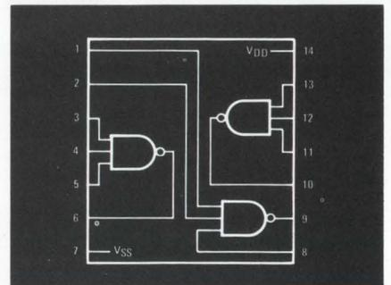
Pin for pin compatible with CD-4023A.
