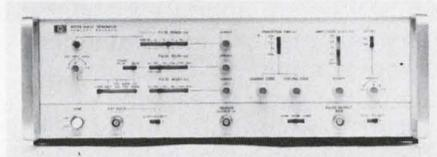
Both the plug-in (top) and stand-alone (bottom) pulse generators can be externally triggered and their pulse widths, externally controlled.
