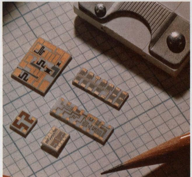
9. Resistor networks, such as these TRW TanFilm units, are filling industry needs for package-compatible components for hybrid and DIP configured circuits.
