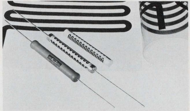
7. Caddock's serpentine film resistors have a minimum of inductance—little more than that of a wire the length of the resistor.
