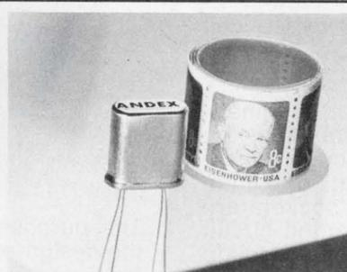
**Ceramic low frequency bandpass filters**, available from 6 kHz to 55 kHz for military and commercial applications. Sealed in HC-6/U crystal cans. Typical parameters are 0.9% minimum 3 dB BW., 20 dB/3 dB skirt ratio < 13, insertion loss < 5 dB, 30 dB stopband to 100 kHz. Analex Corporation, Middleburg Hts., Ohio, (216) 842-5339
