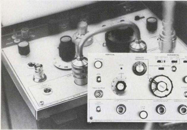
The 1818A time domain reflectometer is easy to use and extremely practical for field measurements
