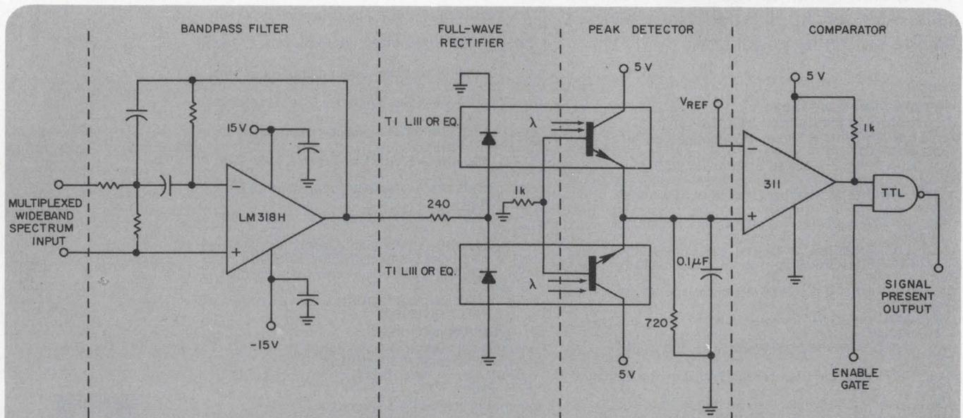
1. Ultrasonic detector with optical isolators avoids need for a transformer and bridge rectifier.
