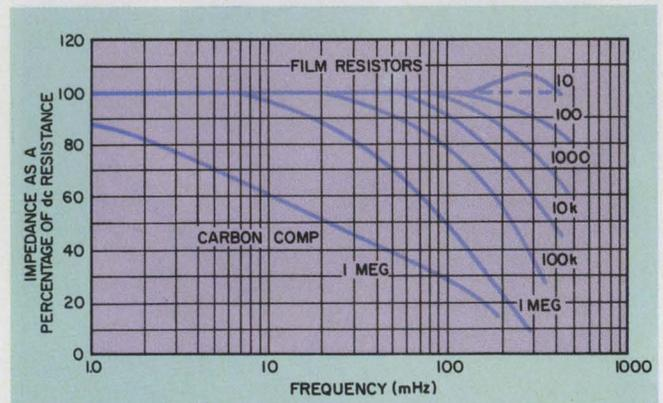
4. The impedance of composition and film resistors generally drops at higher frequencies because of capacitive shunting. Note that only the Mepco 10- $\Omega$  film resistor shows an inductive effect above 150 MHz. Wound resistors, of course, show the greatest inductive effects and film resistors the lowest capacitive effects.
