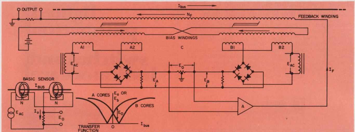
Here's a tough problem: Measure a bipolar dc current of up to 10,000 A without breaking or touching the line and without loading. And do this to within a linearity of 0.015% and with a circuit that's not affected by temperature changes, line-voltage variations, magnetic fields or aging.
