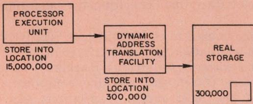
2. Real-storage addresses required by the processor execution unit are derived from the program's logical, or virtual, addresses through the DAT translator.
