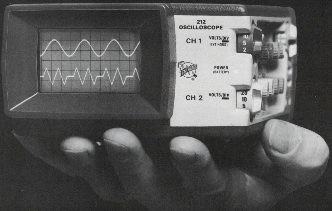
With the 212. A completely new DUAL-TRACE, 500-kHz, 3 x 5¼ x 9-inch scope that weighs only 3.4 pounds and costs just \$725. The high-impact plastic case withstands severe environments — double-insulated construction protects you while floating the scope to make high-voltage measurements.
