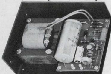
Six models of this slot supply provide continuous coverage from 5V to 24 V DC and up to 3 amp load current.
