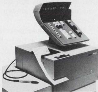
Pitney Bowes-Alpex is incorporating an Intel micro computer in their SPICE™ point-of-sale terminal to perform arithmetic and data processing functions.
