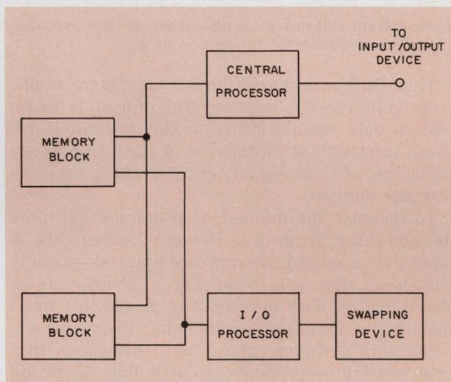
2. **Independent overlapped operation** is a characteristic of an asynchronous system design. It greatly improves efficiency and processing power by having the CPU execute a program in one memory block while programs are exchanged with the other block.
