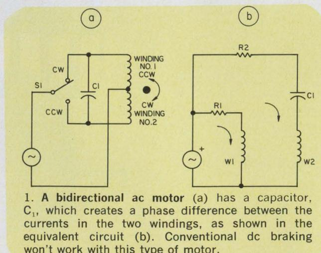
1. A bidirectional ac motor (a) has a capacitor,  $C_1$ , which creates a phase difference between the currents in the two windings, as shown in the equivalent circuit (b). Conventional dc braking won't work with this type of motor.
