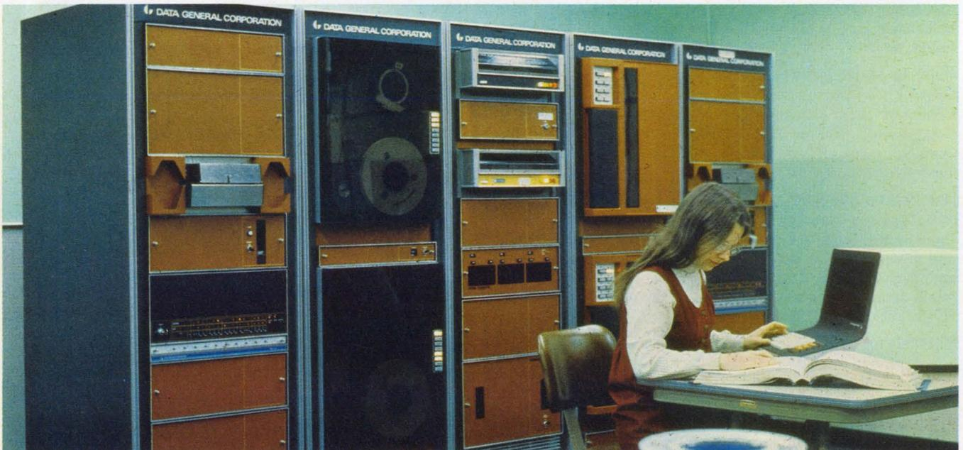
A variety of peripheral equipment is used in this dual-processor system from Data General. Included in the system are two Nova 1200 computers, three on-line disc
