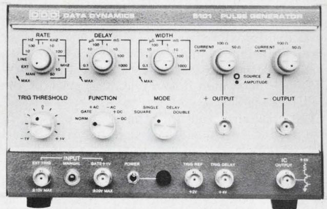
Outputs of the Data Dynamics' 5101 include positive and negative pulses to 50 MHz, double pulses and a separate output to test TTL, RTL or DTL ICs.
