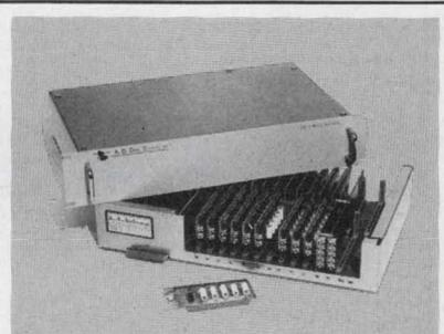
**Coax matrix switch** for high frequency test equipment applications, now available in a modular and expandable 19" rack mounted unit. Computer compatible, the switches latch and unlatch with 250 ns TTL pulses. Signals up to 15 MHz with low distortion and crosstalk. ADDS, 830 Linden Av., Rochester, N. Y. 14625. 716/381-2370.
