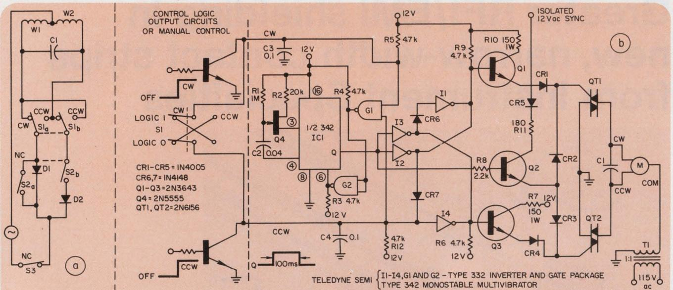
2. Braking can be accomplished by using a mechanical scheme (a) or electronic switching (b) to
