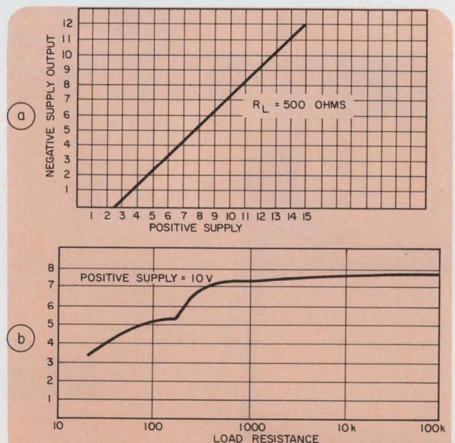
2. The negative output voltage tracks the dc input voltage linearly (a), but its magnitude is about 3 V lower. Application of a 500- $\Omega$  load (b) causes a 10% change from the no-load value.
