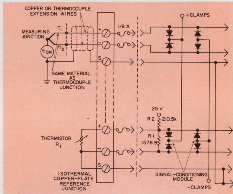
1. A thermistor monitors the reference-junction's temperature and the computer uses this information to correct the thermocouple readings. When the temperatures  $T_1$  and  $T_2$  are equal, the extension wires from the thermocouple material to the reference can be made of copper. But special low-cost extension wires, matched to the thermocouple material, should be used when  $T_1$  and  $T_2$  can vary from each other.
