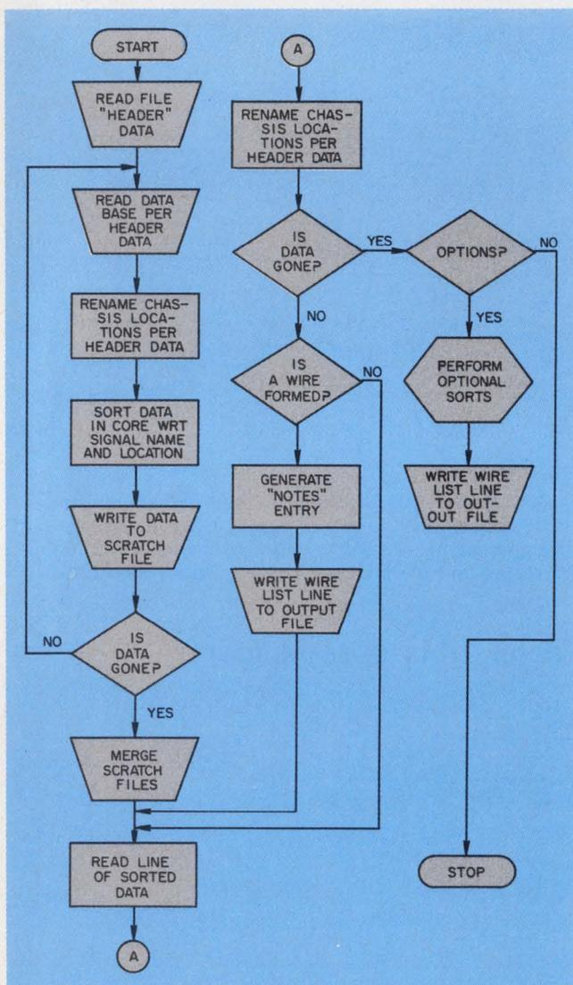
5. A sort merge procedure arrays the data file in report order. Header data alter the sort order of the location fields to conform with preset priorities. Notes are handled by special procedure.
