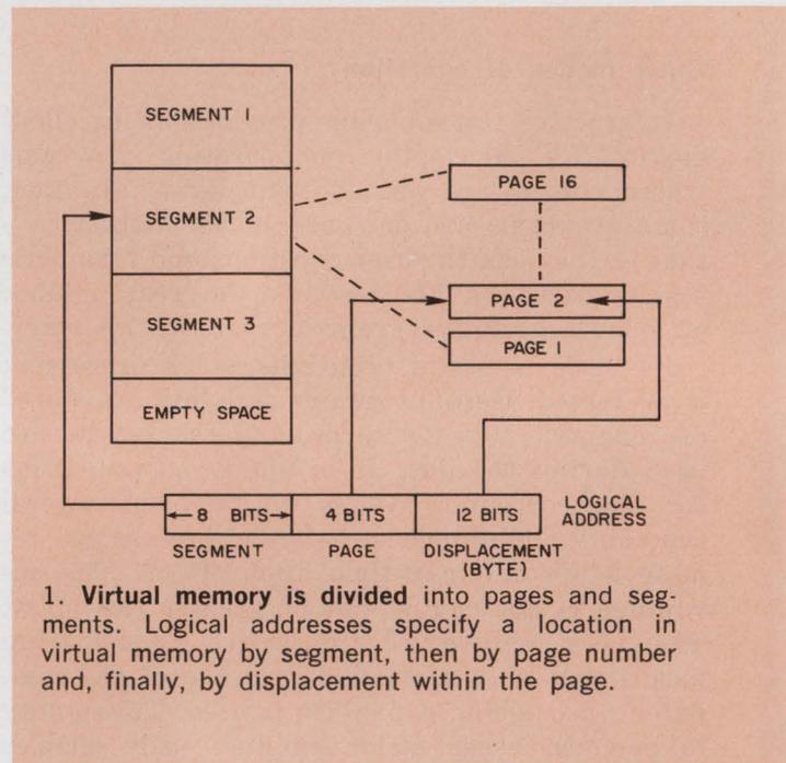
1. Virtual memory is divided into pages and segments. Logical addresses specify a location in virtual memory by segment, then by page number and, finally, by displacement within the page.
