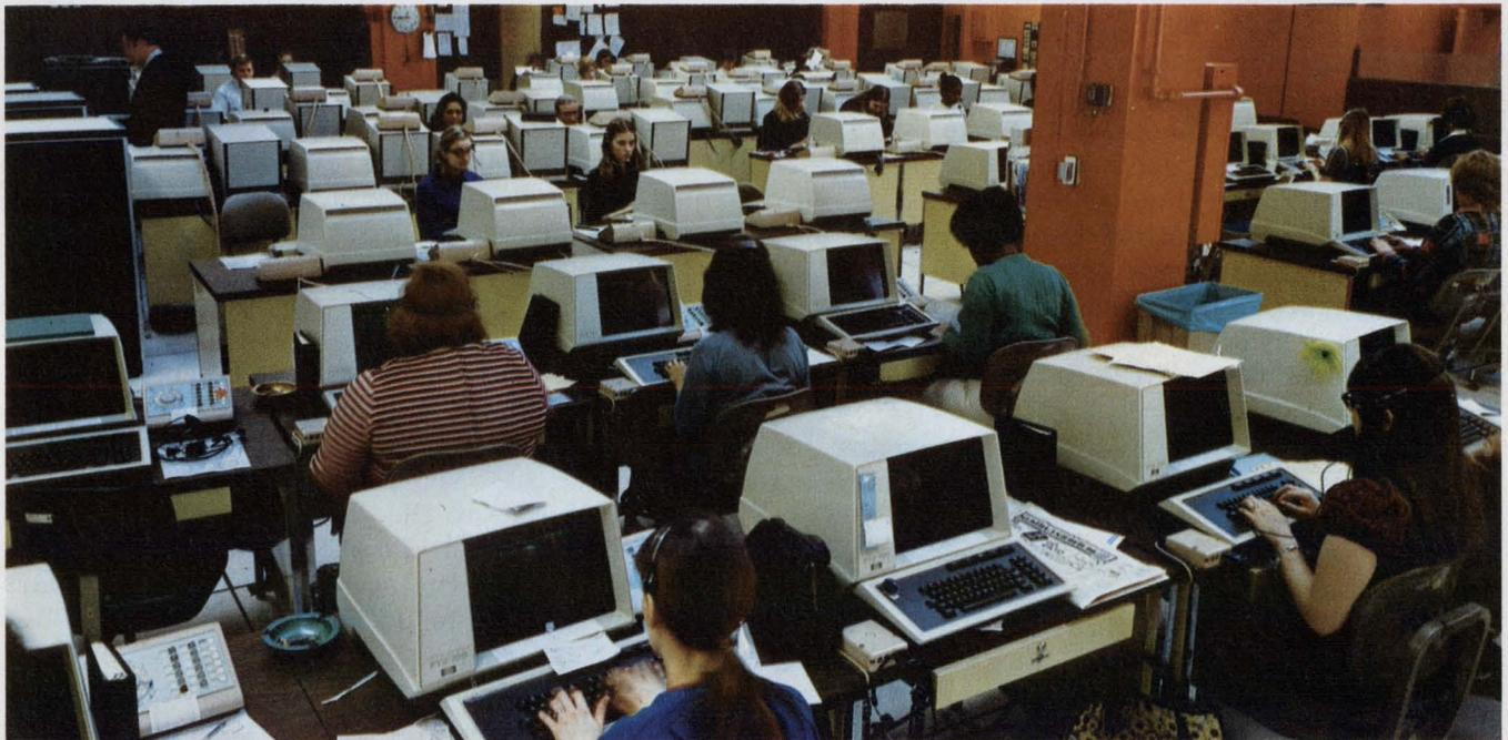
Raytheon's PTS-100 data terminals at the Trans Union System Corp. of Chicago operate into a large central computer credit-verification system. Each terminal needs
