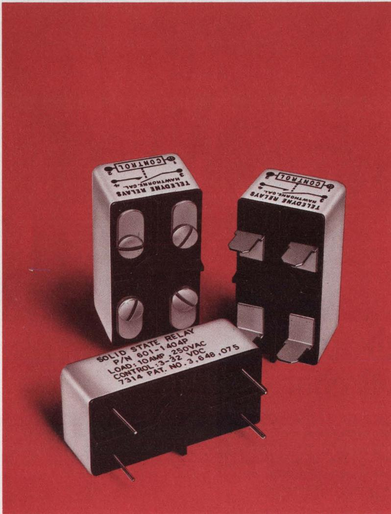
The new 601-1400 series features LED optical isolation and synchronous/zero voltage switching to virtually eliminate RFI for any resistive or reactive load, up to 10 amps steady state. 1000% surge current capability assures maximum reliability without derating for the toughest loads — lamps, solenoids, motors, transformers, etc. High dv/dt rating assures maximum output transient immunity. The 601-1400's sensitive control input is TTL compatible, accepting drives from 3 to 32 VDC.
