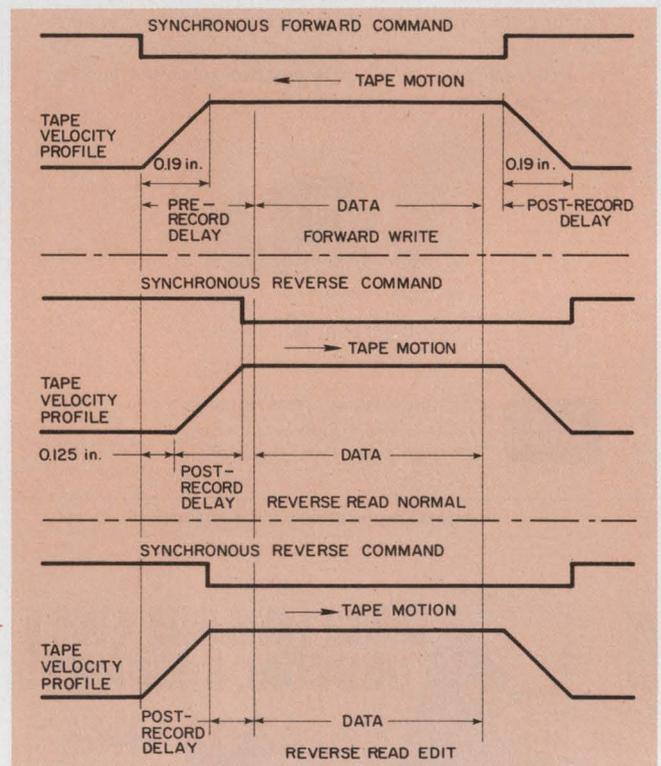
1. Accurate positioning of a data block during selective editing of a record on magnetic tape is a function of the interblock gap (IBG). If this gap becomes less than 0.5 inch, successful selective editing becomes impossible.
