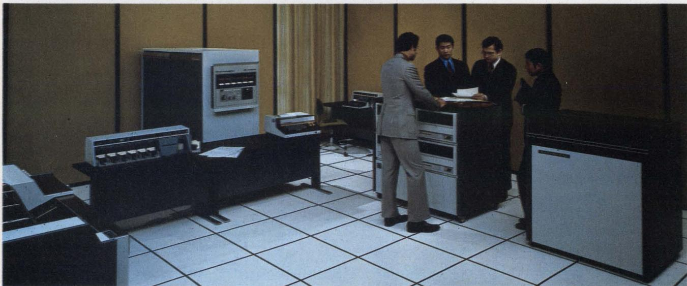
Variable micrologic alters the run-time environment according to the language processed in the Burroughs B1700 series. The system runs Cobol, Fortran, Basic
