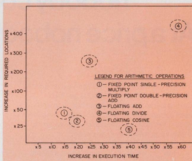
1. The relative computational power of a typical large-scale computer and a 12-bit mini with a minimum hardware-instruction set. The required number of instructions and the execution time of the large computer are taken as unity and other data are normalized.
