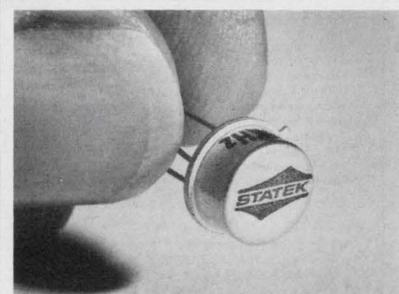
**Low cost quartz crystals in TO-5s:** For 10 to 250 kHz oscillators, filters, tone generators, timers . . . Rugged—Accurate—High vibration and shock resistance. Prices low as \$.95 ea. in 100k qty's. Send your written application. We'll send a sample. Or, write for literature. Statek Corp., 1233 Alvarez Ave., Orange, Calif. 92668. (714) 639-7810.
