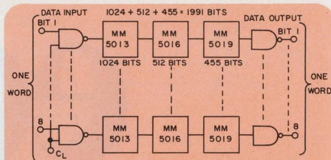
3. Use of the double clocking technique reduces the package count of an equivalent register from 24 to 16. It also saves the cost of ordering a custom-masked MM5019 register.
