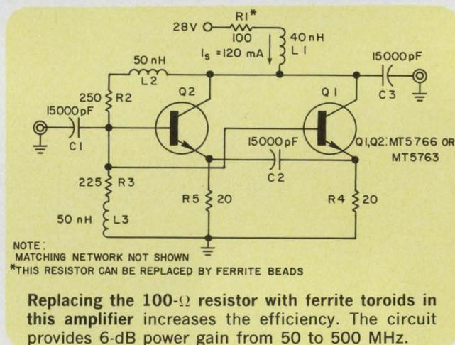
Replacing the 100- $\Omega$  resistor with ferrite toroids in this amplifier increases the efficiency. The circuit provides 6-dB power gain from 50 to 500 MHz.
