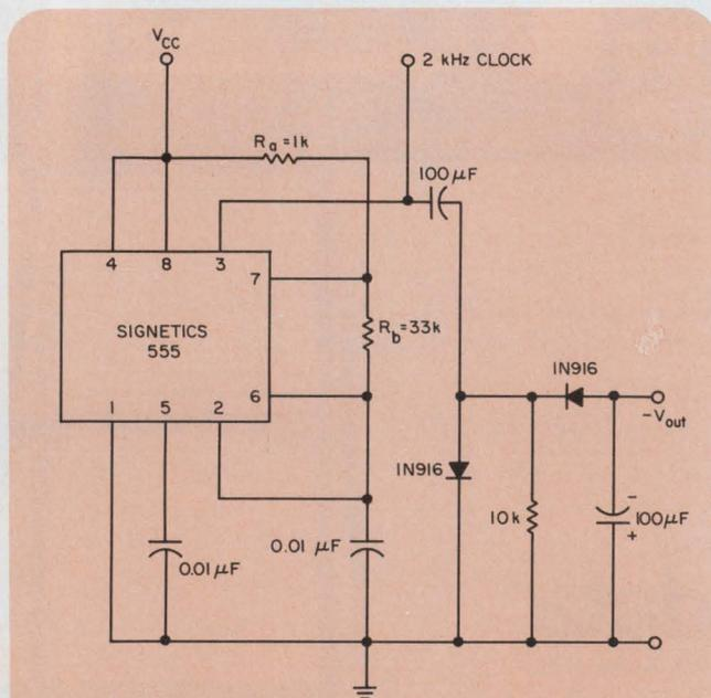
1. Transformerless dc-dc converter derives a negative supply voltage from a positive. As a bonus, the circuit also generates a clock signal.
