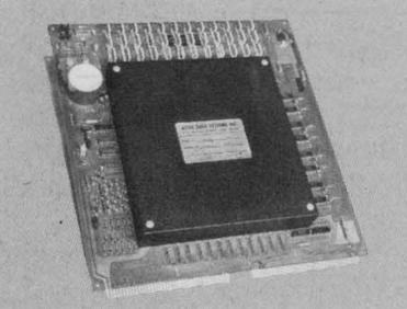
**Aztec Data Systems** has developed the only single board electrically alterable read-only memory in configurations of either 1K X 16 or 4K X 16 bits on a 15" X 15" PC board. Priced in quantity as low as 5¢ per bit. AZTEC DATA SYSTEMS, INC., 17805 Sky Park Circle, Irvine, Ca. 92707. 714-540-8445.
