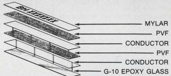
Laminated DIP Bus Bars from BH Electronics feature tinplated copper conductors separated by stable high-dielectric polyvinyl fluoride (PVF). Evenly distributed capacitance (75 PF/inch @ 1 MHz) provides effective noise reduction.
