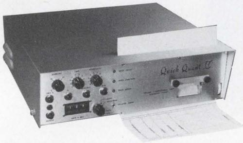
Helena Laboratories is using an Intel micro computer in an instrument that measures the protein content of blood, printing a separate quantitative reading for each of several different proteins.
