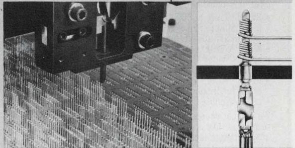
You save time and costs with BergPost .025" square pins and application machines that give in-plant capacity to build wrapped-wire panels, and let you control quality. Insertion machines stake on a .100 x .100 minimum grid with semi-automatic or N/C production, without capital investment. Change pin length merely by changing reels. Pins accept wire-wrapping, crimp-to-wire disconnects, card connectors, and multiple contact housings.
