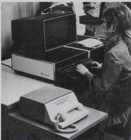
AT&T's new data terminal features a combination high-speed printer and cathode-ray-tube display.
