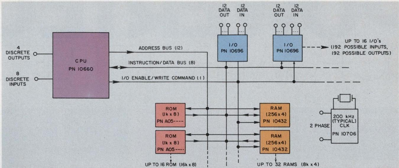
Rockwell Microelectronics' parallel-processing system uses the 10660 central processor, which has a basic instruction cycle of only  $5 \mu\text{s}$  and a 50-instruction set repertoire. Data can be handled internally at four times the rate of the external clock; the processor divides the
