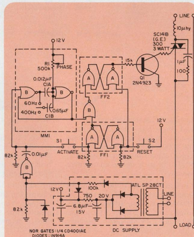
Initiation of load power occurs at a precise point on the ac waveform after depression of S<sub>1</sub>. The controllable-pulsewidth of MM<sub>1</sub> (R<sub>1</sub>, C<sub>1A</sub>, C<sub>1B</sub>) determines the moment FF<sub>2</sub> is latched and the triac gated on.
