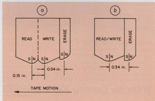
2. Turning off write and erase currents on a dual gap head (a) must be done immediately after the last character is written because of an additional distance that the tape must travel to reach the read gap. Slower turn-off can be tolerated in a single-gap head (b).
