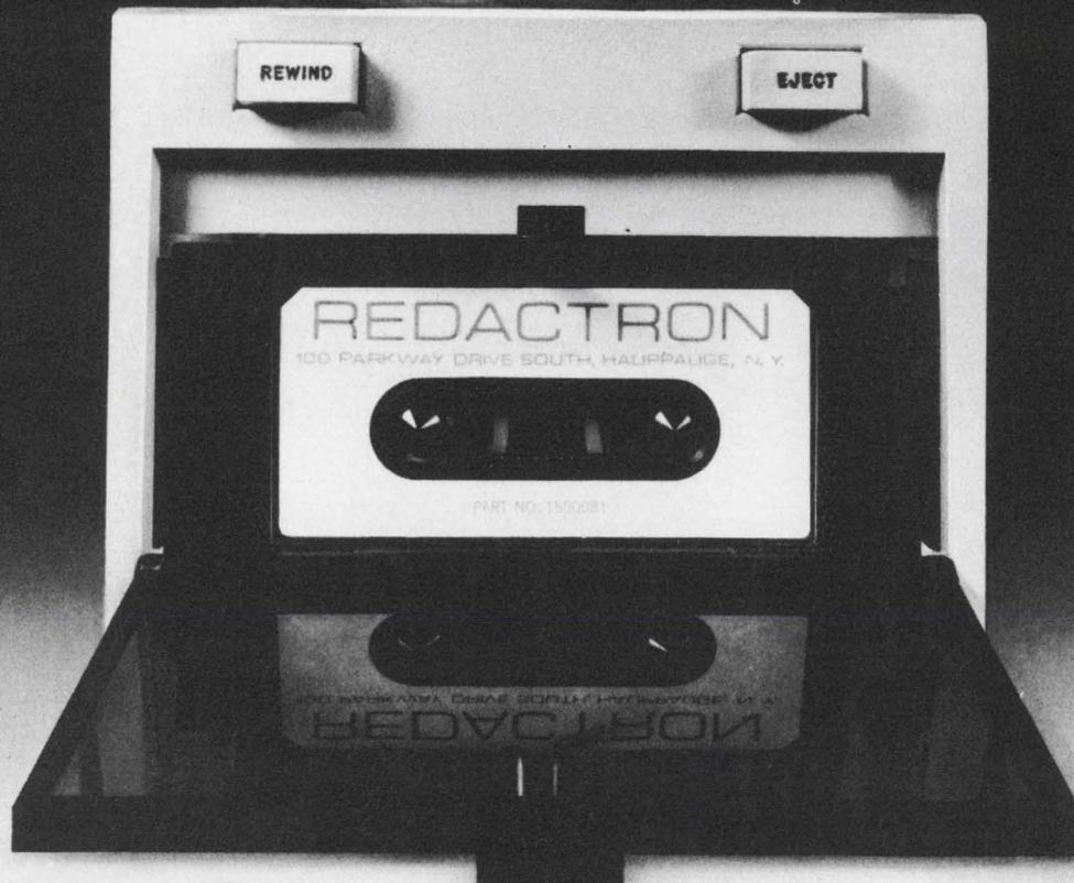
Our Cassette Transport has no pinch roller, capstan or servo system to clean, maintain or cause problems. We've shifted the burden of tape speed regulation from mechanics to electronics ... and you get added reliability at a lot less cost.
