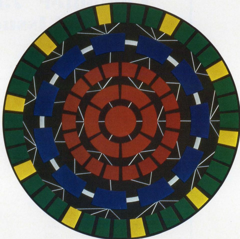
**Symbolic concept of General Electric's Mark III Information Services Network.** Outer ring of blocks represents low-speed remote concentrators. Blue colored blocks represent high-speed data concentrators.
