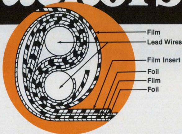
Chalk up another capacitor first for Paktron. The Polypropylene Micromatic Capacitor is truly designed for highly automated production. Close capacitance tolerance . . .  $\pm 1\%$  to  $\pm 20\%$ . Capacitance value range 100pf to 0.15mfd., 200 and 400 volts. And this is a completely self-encased capacitor. No outside wrapping needed. Nor is there any separate lead attachment because the
