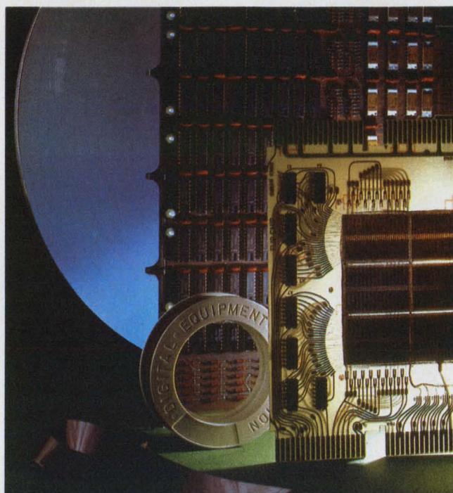
Key elements of memory technology include MOS semiconductor devices, magnetic ferrite cores, magnetic discs and magnetic tapes.
