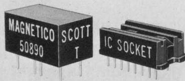
**Scott T transformer—dual in line size.** In a DIP type size and pin spacing, Scott T No: 50890 converts 400 Hz 11.8V RMS line to line synchro information to 6V RMS Sine and Cosine resolver outputs. Accuracy is 2 arc minutes. Cost is \$25.00 in qty. For any Scott T call: Magnetics, Inc., East Northport, N.Y. 11731. Tel: (516) 261-4502.
