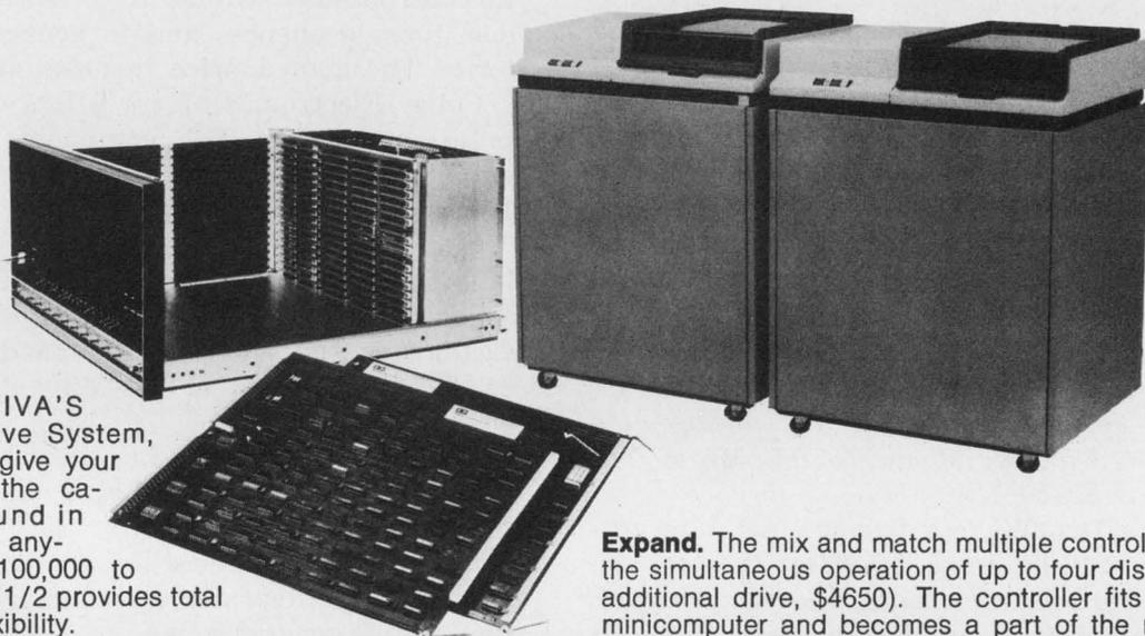
**Maximize.** DIVA'S Dual Disc Drive System, DD-11/2, will give your minicomputer the capabilities found in maxis costing anywhere from \$100,000 to \$400,000. DD-11/2 provides total operational flexibility.
