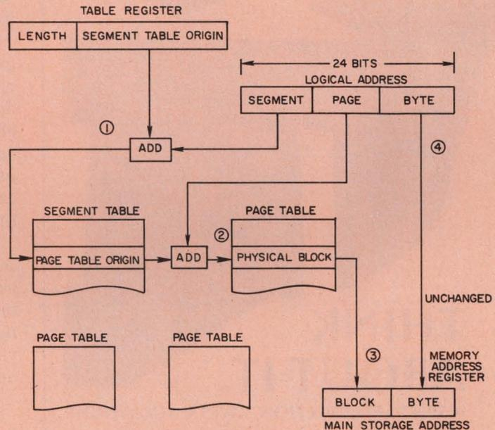
megabytes of virtual storage into the smaller domain of real storage. Mapping maintenance is done by the software portion of the package—the control program.
