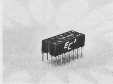
**EC's "DIP Series" Lumped-Constant Delay Lines** are packaged in a low silhouette epoxy encapsulated, 14-pin dual in-line configuration. EC<sup>2</sup> offers over 200 variations of DIPs, featuring either fixed or tapped delays, from 4 to 150 nanoseconds. Engineered Components Co., 2134 W. Rosecrans Ave., Gardena, Calif. 90249. (213) 321-6565.
