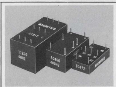
**Scott T Transformer.** 11870: 60HZ, 90v, L-L In. 1.1x2.1x1.1. 50460: 400HZ, 90v, L-L In. 7/8x1-5/8 x11/16. 50642: 400HZ, 11.8v, L-L In. 7/8x1-5/8x11/16. 10472: 400HZ, 11.8v, L-L In. 3/4x1-1/2x3/8. All with 6v RMS sine & cosine output. MAGNETICO, INC., E. Northport, N.Y. 11731. 516-261-4502.
