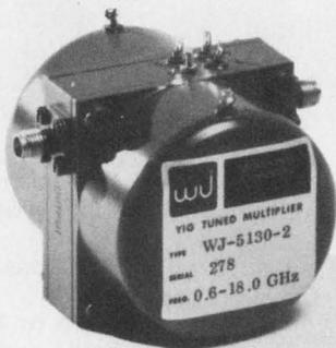
The WJ-5130-2 multiplier is one of a series of harmonic power generators created for commercial applications.
