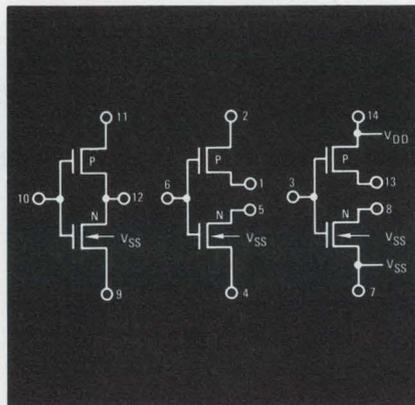
Pin for pin compatible with CD-4007A.
