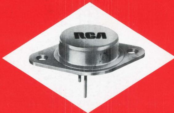
No we haven't changed the Darlington circuit. We've just turned it into the Darlington transistor. By putting the whole circuit on a single monolithic chip.
