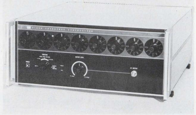
The popular Fluke 6160A indirect synthesizer offers output to 160 MHz, BCD programming with 0.5-ms switching time, and a signal-to-phase-noise ratio of 62 dB.
