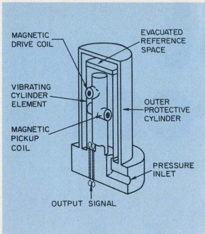
**Key to the new all-electronic altimeter** is Hamilton Standard's digital pressure transducer. The pressure-sensing element is a cylinder that is driven magnetically to vibrate at its natural frequency of about 4 kHz. As the static air pressure increases, internal forces increase the stiffness of the sensing element, increasing the frequency in proportion to the change in pressure.
