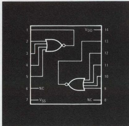
Pin for pin compatible with CD-4002A.
