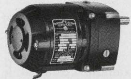
**N-1D Gearmotors:** Parallel shaft helical and spur gearing. Ratings thru 40 Lb-in. Ratios thru 900:1. Only 3.41" square.
