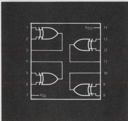
Pin for pin compatible with CD-4030A.
