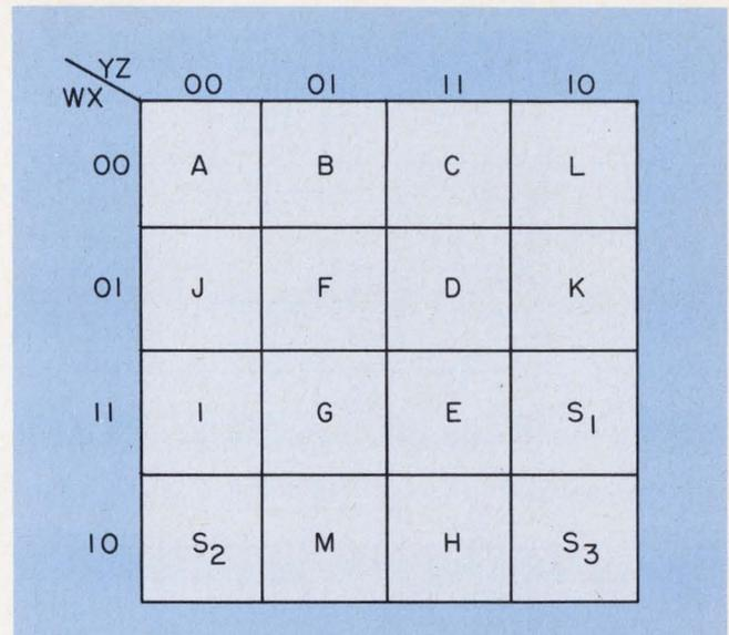
5. The Karnaugh map for the a/d controller must include the unused states, S<sub>1</sub>, S<sub>2</sub> and S<sub>3</sub>. These states must also appear in the J-K input equations. Should the system fall into one of these unused states, the circuit must automatically transfer to Standby (state A) on the next clock pulse.
