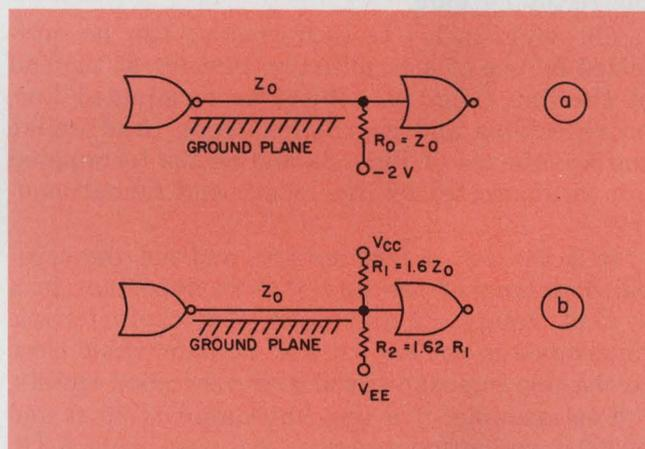
2. Terminations can eliminate reflections. The possible termination techniques include resistor  $R_0 \approx Z_0$  connected to a termination voltage (a) or the use of an equivalent resistor network (b).
