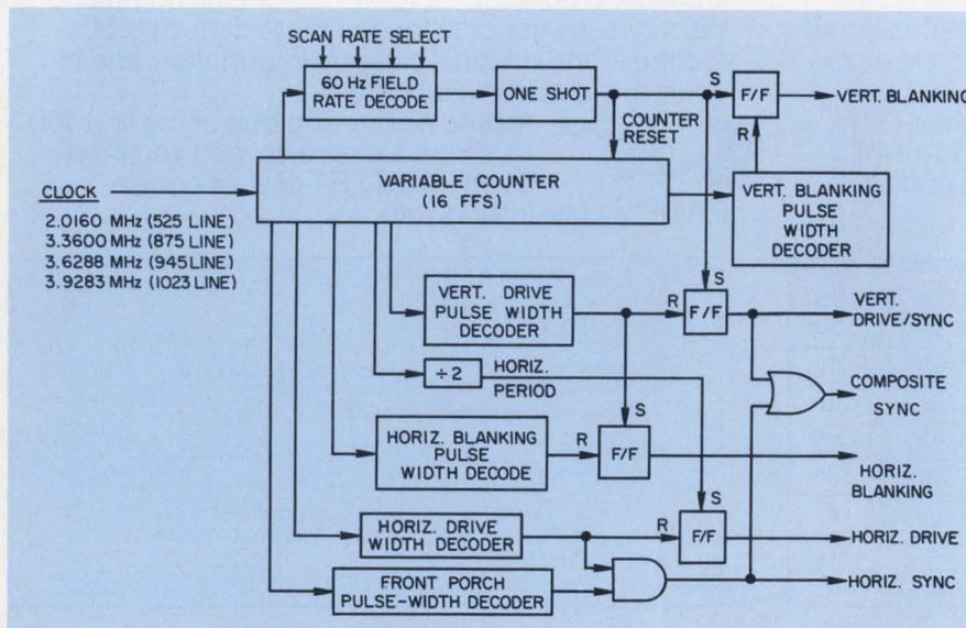
The ripple binary counter in the TV sync generator can be set to perform any one of four divisions. The clock frequency is provided by a crystal-controlled circuit that provides precise timing of sync signals.
