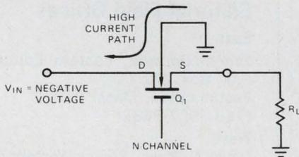
**Figure 2.** Intersil's Floating Body Process eliminates latch-up with a diode between the N-channel FET body and the positive supply.
