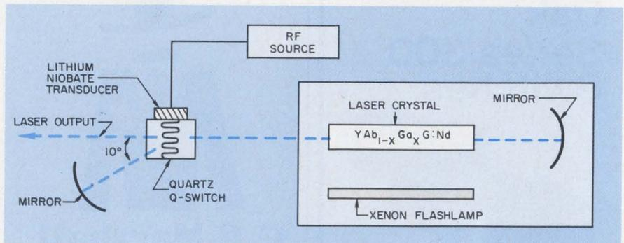
Quartz Q-switch with lithium niobate transducer is expected to allow acousto-optic modulation of 1-J/pulse laser energy.
