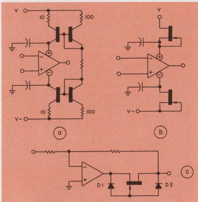
4. Precise, selectable current-limiting results when current sources are added in series with the power supplies (a, b). To limit both current polarities, a FET current source in series with the output may be added (c).
