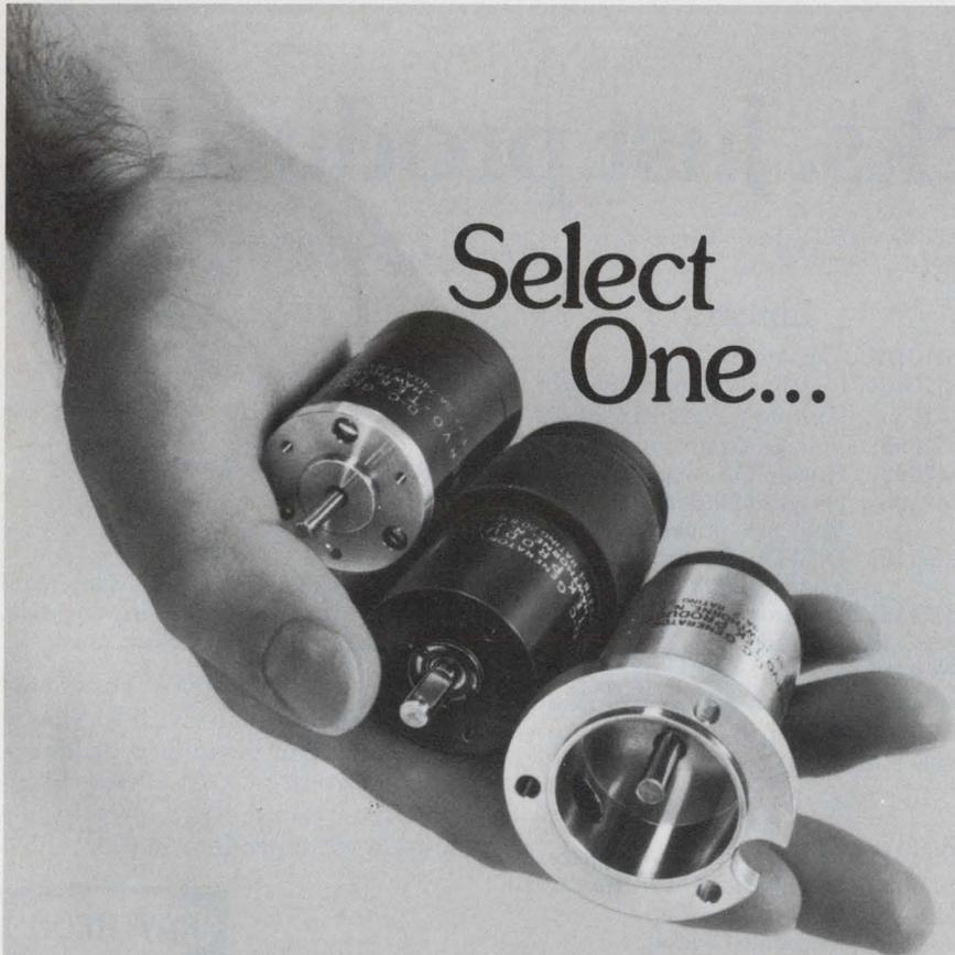
One of these tachometer generators is suited to your application. We offer them in two-bearing and single-bearing versions, no-bearing overhung versions and in sealed housings for use in environments containing oil and hydraulic fluids. Outputs range from 2.6V/1000rpm to 45V/1000rpm; brush life up to 100,000 hours—that's over ten years!
