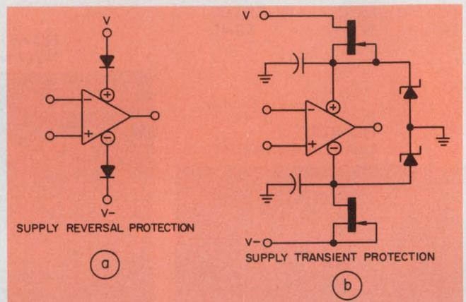
1. Damage from power-supply faults is prevented because diodes block currents during voltage reversals (a) and clamp the power-supply terminals to limit transient voltages (b).
