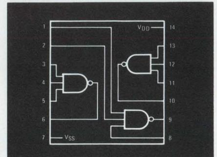
Pin for pin compatible with CD-4023A.
