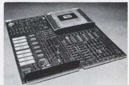
**15-by-16-inch printed-circuit board** contains an entire minicomputer, including 4-k, 16-bit words of core memory. The large packages on the left side of the board contain the central processing unit and microprogram control on silicon-gate MOS/LSI circuits.
