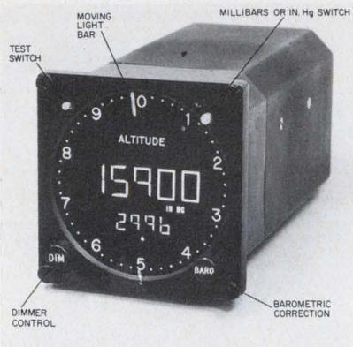
The solid-state encoding altimeter provides a digital display of altitude and barometric settings. It also provides altitude information for transponders operating in mode C.
