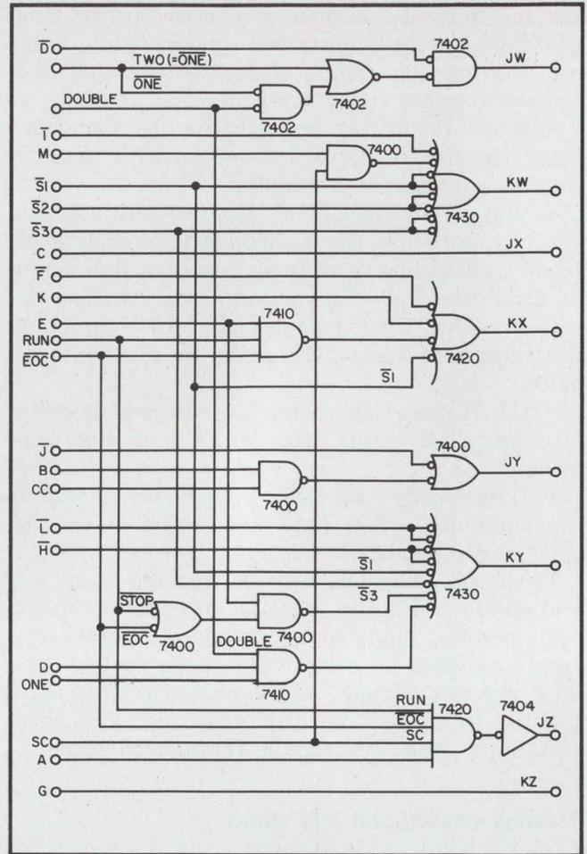
8. The Input-Logic circuit implements the equations for the J-K steering inputs of the Sequence-Events flip-flops. Note that most of the input variables to the gates come from the decoder's output, which represents the sequencer's present state. The present state, together with the signals from external events and from the control switches, determines the system's next state. Changes in the system would be made mainly in this circuit.
