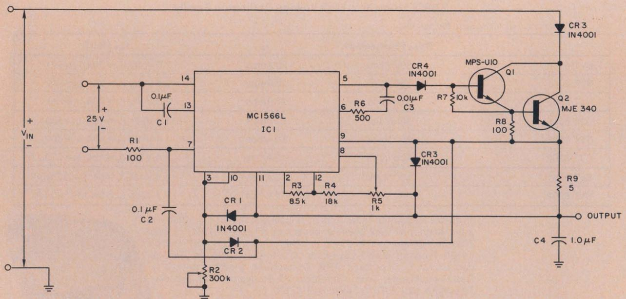
IC voltage regulator provides accurate constant currents because the voltage and current-control
