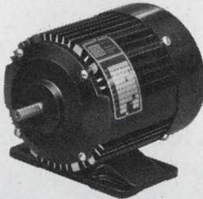
**42R Induction Motor Line:** TEFC ratings from 1/20 thru  $\frac{1}{4}$  Hp. All A-C winding types. Options include capacitor mountings, overload protectors, and special wiring provisions.
