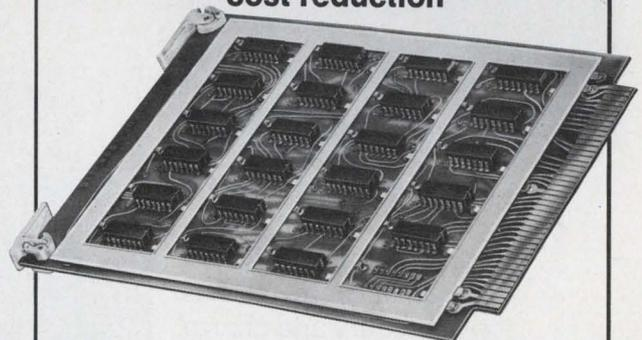
A small, voltage-distributing busbar for PC card application, each Mini/Bus gives you built-in capacitance . . . noise-cutting capacitance that means more reliable, compact circuit packaging at a fraction of multilayer prices. Write for data.
