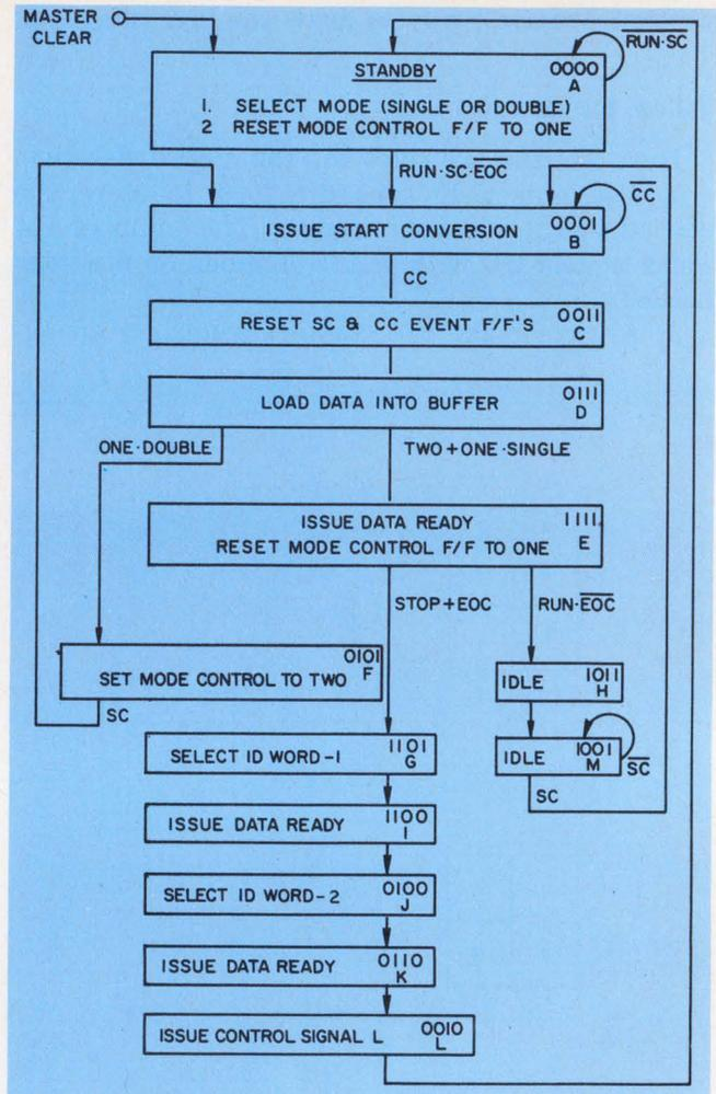
4. A control-loop chart for an a/d control system illustrates the use of idle states to attain a single-bit change at a time, when going from one state to another. Idle states, H and M, serve this function between B and E.
