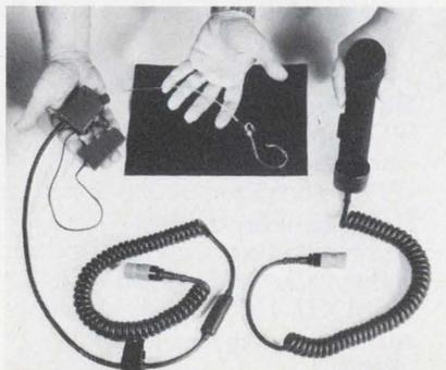
pliable plastic tube fastened to the ear by an adjustable ear-lobe clip and a sliding fastener. Since it does not obstruct the ear canal, face-to-face conversations can be carried on at the same time that the radio is in use.
