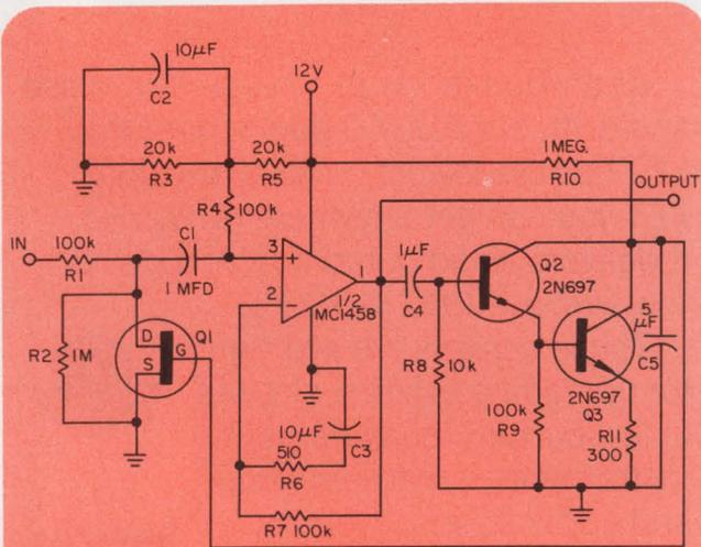
1. Op amp  $A_1$  provides low distortion forward gain for this volume compressor. FET  $Q_1$ , and Darlington pair  $Q_2$  and  $Q_3$ , provide fast-attack, slow-release, agc action.
