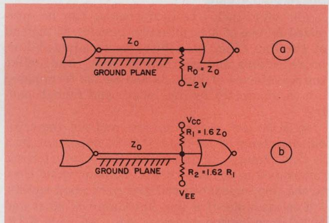
2. Terminations can eliminate reflections. The possible termination techniques include resistor  $R_0 \approx Z_0$  connected to a termination voltage (a) or the use of an equivalent resistor network (b).
