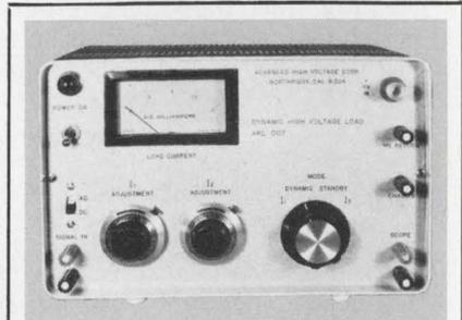
**Electronic high voltage load** for static and dynamic testing of high voltage sources to 30 kV at 2 mA. Switches two independently adjustable load levels from dc to 100 kHz. Provides for ripple, regulation, and recovery time in a single display. Advanced High Voltage Co., 14532 Arminta St., Van Nuys, CA 91402. (213) 997-7222.
