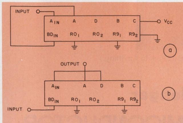
4. The counter configurations provided on spec sheets are only (a) a conventional BCD counter hook-up and (b) a symmetrical-wave output divide-by-ten.
