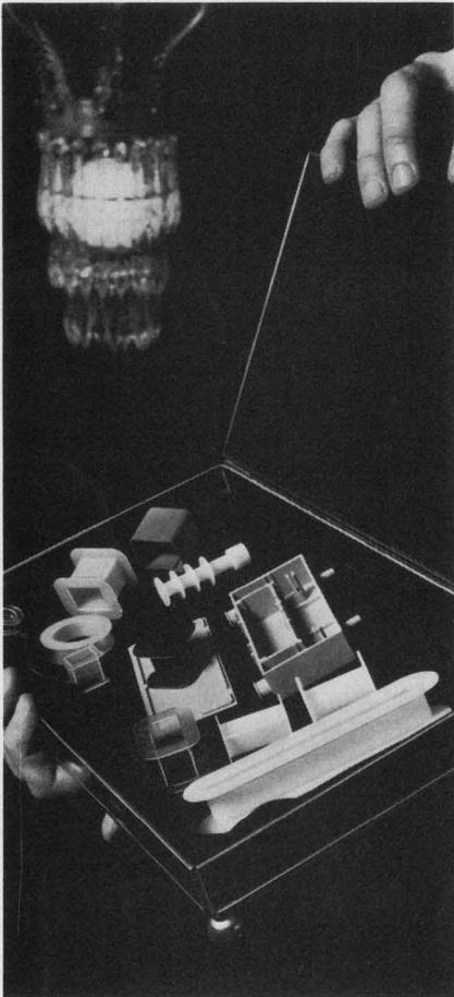
For elegant applications. Custom-made or standard, EPC parts come with thin walls down to 5 mils, tolerances to  $\pm .05\%$  — even threaded bushings. In six different materials: fluorocarbon, nylon, glass-reinforced nylon, DAP, polyester and epoxy. For temperature ranges that go up to 200°C.
