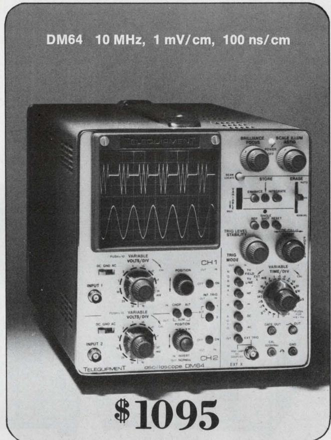
**Lowest cost 10-MHz dual-trace oscilloscope with bistable storage.** The DM64 lets you view displays for up to one hour. Other features include 1 mV/cm vertical, 100 ns/cm time base (40 ns with MAG), triggered sweep, and much more.
