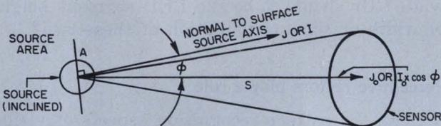
$\phi$  = Source inclination angle with respect to source/sensor axis
