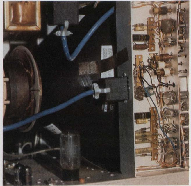
**Metal tapes and conductive paints** are a low-cost means of grounding and bonding. This embossed copper tape, by 3M, drains high-voltage charges from a TV tube.
