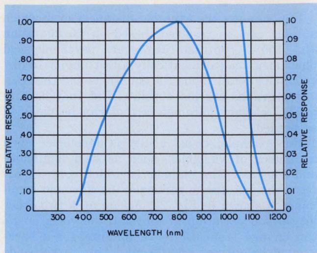
6. Silicon sensor (PIN 10D) calibration curve shows relative spectral response. Responsivity of cell at 800 nm (peak  $\lambda$ ) is 0.379 A/(W/cm<sup>2</sup>).
