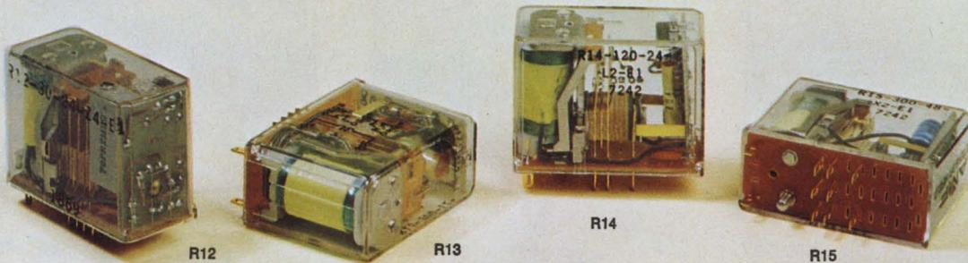
These new solid state time delays—each designed to solve different design problems—are built around our compact, widely accepted R10 relay. Each is available in 2 or 4 Form C contact arrangements and may be mounted directly to a chassis, printed circuit board, special mounting strip or in sockets having solder or printed circuit terminals.
