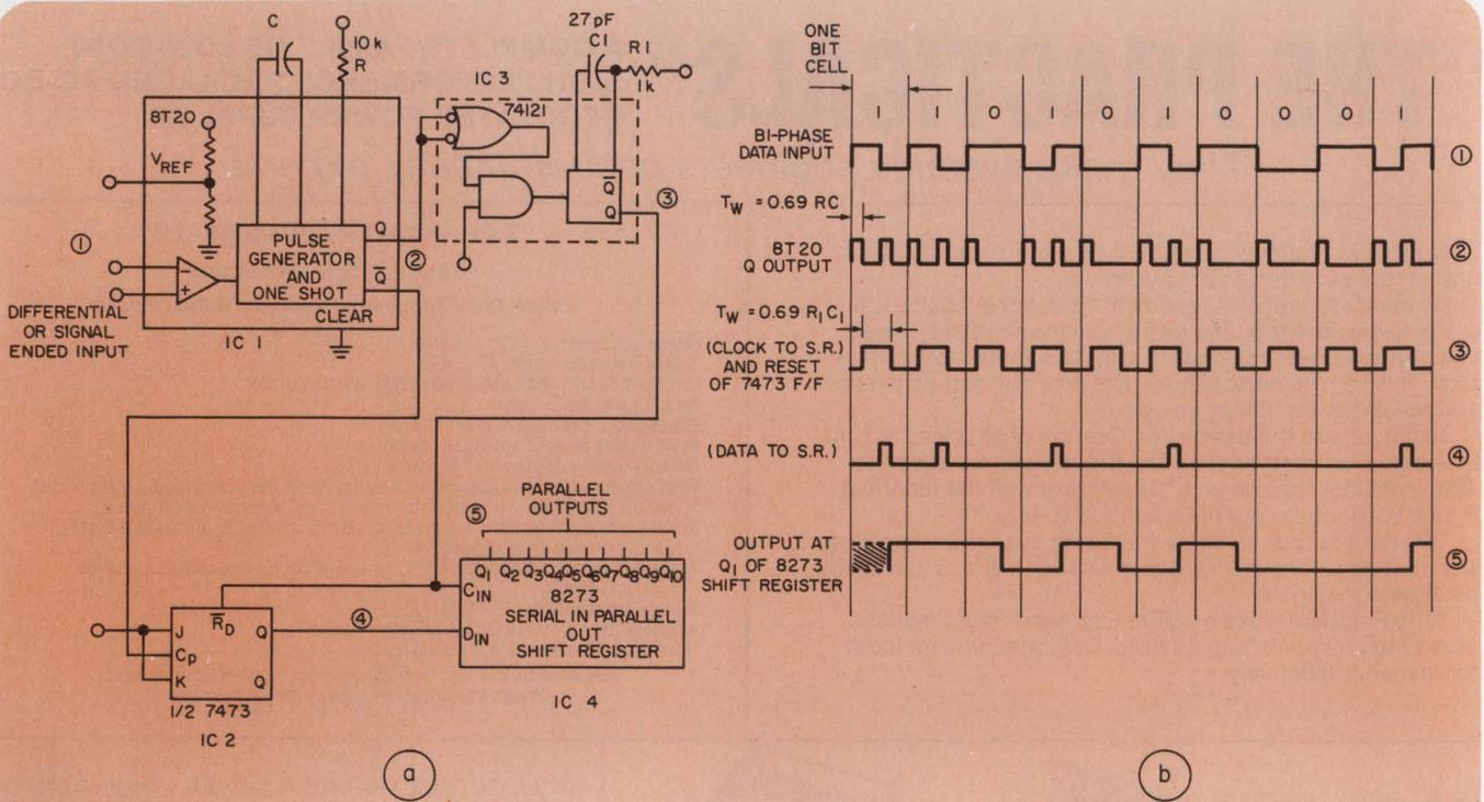
2. Receiver circuit recovers both the clock and the original binary data. The narrow pulses from the Q terminal of IC<sub>1</sub> are stretched by the nonretriggerable one-shot, IC<sub>3</sub>, to obtain the clock. The clocking
