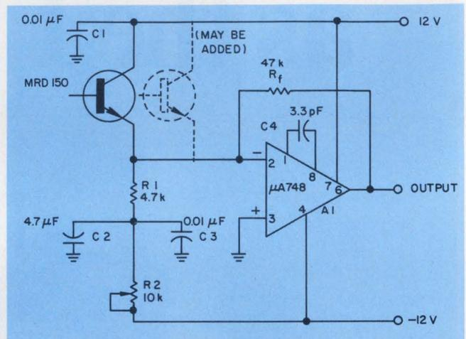
1. Op amp  $\mu A748$  extends the frequency response of the phototransistor by maintaining the device's output at an effective ac ground. Feedback resistor  $R_f$  adjusts gain, and potentiometer  $R_2$  balances out the quiescent current of the phototransistor.
