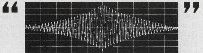
Chamber pressure characteristics point up jet engine combustion problems
