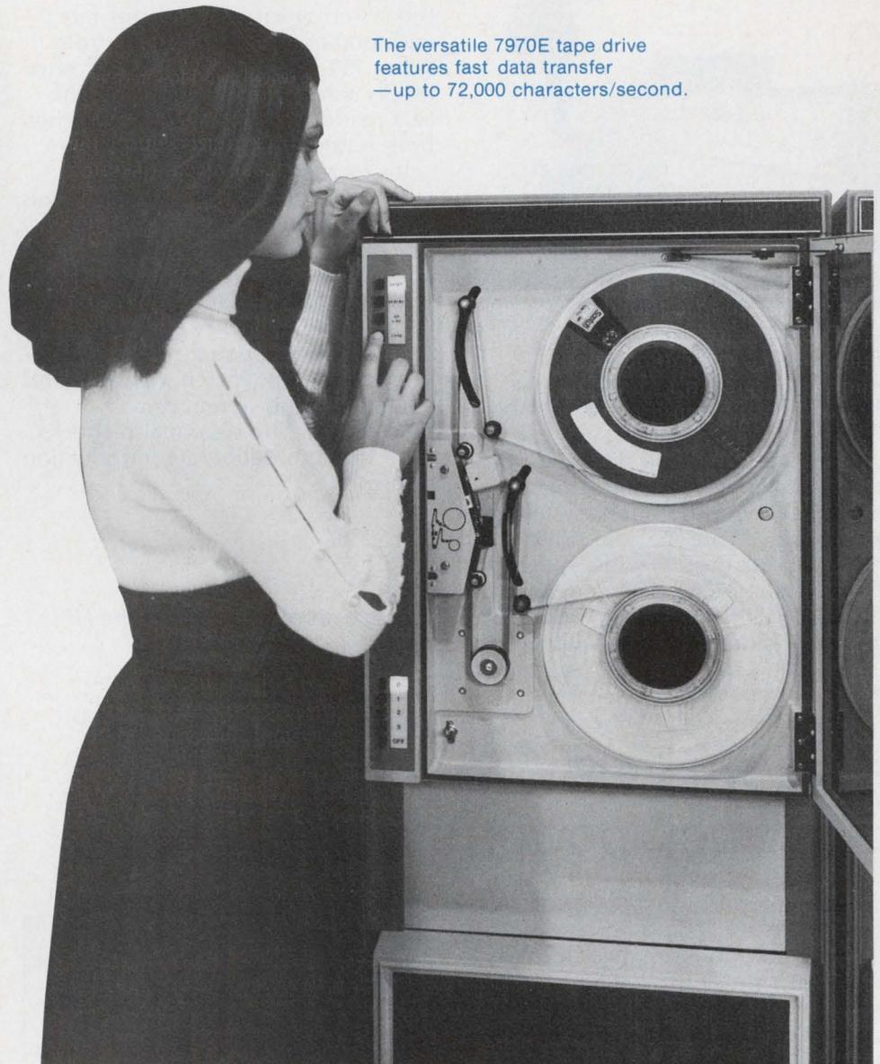
HP's new digital magnetic tape drive can handle virtually any recording problem—200, 556 or 800 cpi NRZI; any speed from 25 to 45 ips; or 1600 cpi phase-encoded recording that is ANSI/IBM compatible. You get 7 and 9 track, multi-density, NRZI and PE capability—all in one read-only tape drive, model 7970E.
