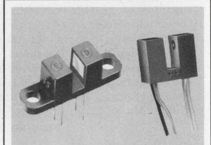
**Hermetically sealed optical switch:** Contains discrete matched hermetic LED/photo transistors. DTL/TTL compatible output. SSOS-700 straight package. SSOS-800 package with flange. Gap dimension between photo transistor & LED is .110". Solar Systems, Inc., 8124 Central Park, Skokie, Ill. 60076. Phone: (312) 676-2040.
