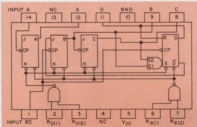
3. Manufacturers' block diagrams provide pin arrangements and the reset-circuit internal wiring, but leave out the important J-K input details.
