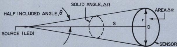
$$\Delta\Omega \cong \Delta a / s^2, \quad s = \text{source/sensor separation}$$
