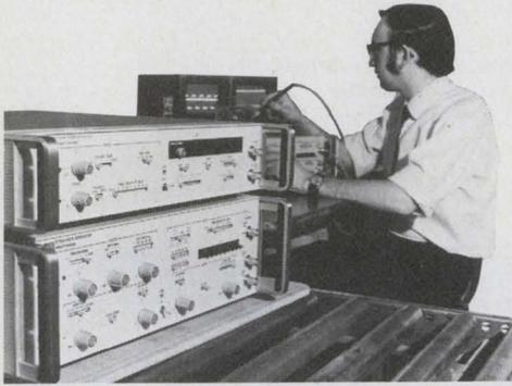
Besides testing PCM equipment, the 3760A/3761A tests computer memories, disc storage, digital recorders, and high-speed logic circuits.
