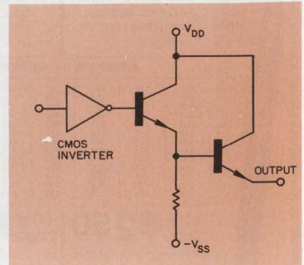
Each of seven output stages has an npn Darlington transistor network for higher drive currents.
