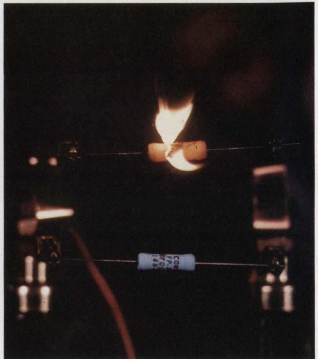
**Consumer electronics** need safe materials and parts. Here, a Corning Glass fusible resistor opens up under a heavy overload while a common resistor type burns.
