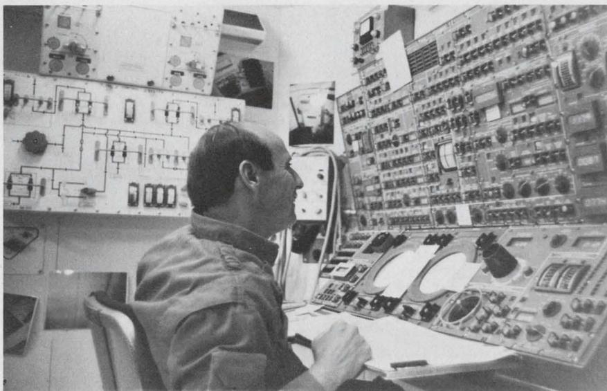
Astronaut Charles Conrad Jr. sits at the control and display panel of the Apollo Telescope Mount, where data from eight telescopes are received on five TV screens, then sent on to earth for immediate evaluation.
