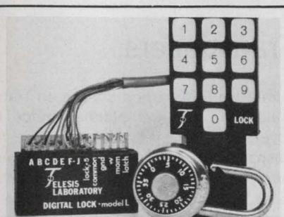
**Low cost digital combination lock** Model L input keyboard and control module. Momentary and latched outputs are enabled by easily programmed 5 digit code(s). Actuation by a 'drunk' or 'observer' may be prevented. Under \$40. +5 to 30V at 30mA. Telesis Laboratory, Box 387 Chillicothe, OH. 45601 (614) 773-1414
