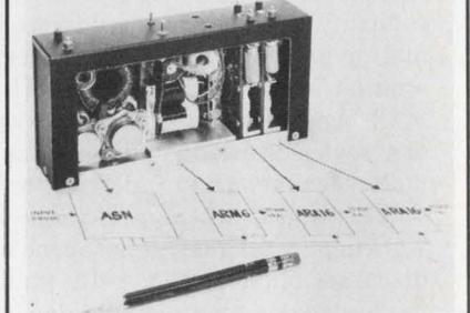
**Miniaturized/modular power supplies.** AC or DC inputs with up to 6 isolated and regulated DC outputs to 150 watts. Over 1200 "Design As You Order" configurations using standard sub-modules. Completed systems provided in pretested, encapsulated miniature packages. Immediate delivery. Arnold Magnetics, Culver City, Ca. (213) 870-7014.
