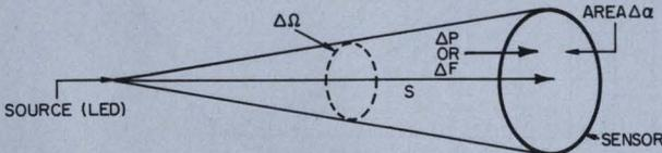
$$\text{Intensity} = \frac{\text{Power (or Flux)}}{\text{Unit Solid Angle}}, \quad J_o = \frac{\Delta P}{\Delta\Omega}$$
