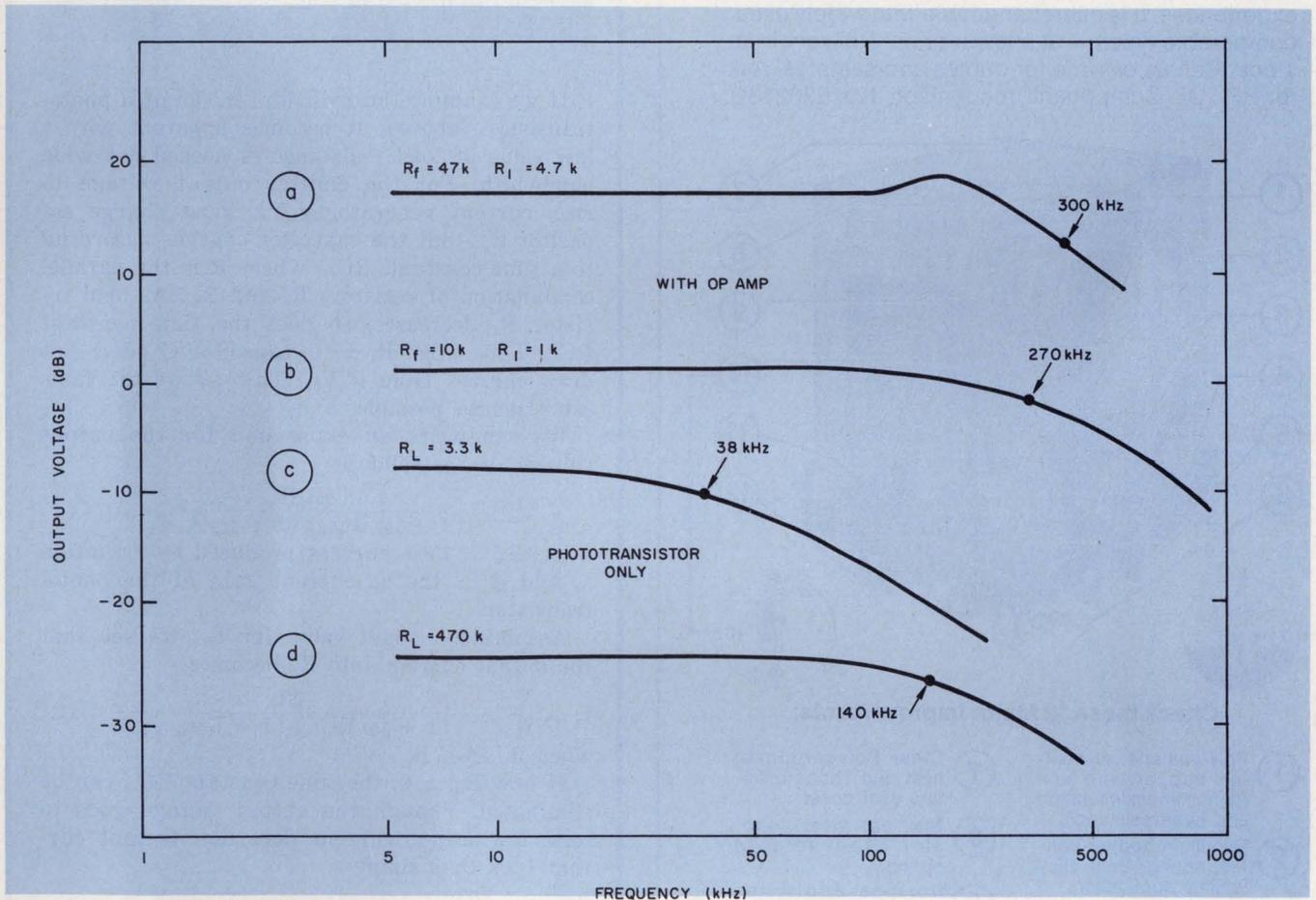
2. Frequency response of the op amp circuit for two different values of gain (a and b) shows marked im-
