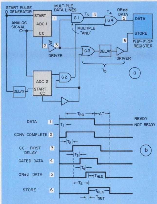
4. System delays rather than actual hardware are emphasized (a). The CC signal (b) gates the a/d output data and generates the Store signal. Data to the register are delayed by arrival of the CC signal at gates  $G_1$ , while the generation of the Store signal is delayed by the driver and composite delays  $T_5$ . Other circuit requirements include the register setup time ( $T_{SET}$ ), data hold time during clocking ( $T_{HLD}$ ) and a minimum clock signal duration at the store input.
