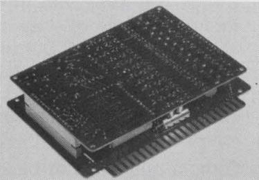
**GOOD SPEED AND STABILITY. ADC700 Series.** 6.5 Microseconds for 12 bits, 3.5 Microseconds for 8 bits. Up to 0.025% full range accuracy and  $\pm 10$  ppm/ $^{\circ}\text{C}$  stability. Voltage switching attains high conversion speed without sacrificing accuracy. Series includes six repairable models. Many options, modifications for special applications. If it's stability, accuracy, speed, or all-around quality performance you need in Data Conversion, contact Phoenix Data now!
