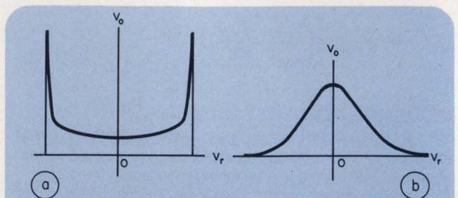
3. Sample outputs from a sine wave input (a) and amplified resistors noise (b) as a function of  $V_r$  show excellent agreement with the corresponding theoretical probability density functions.
