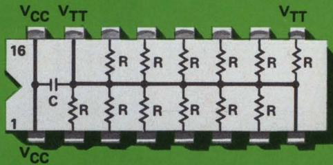
**SERIES 898-41 -2.0 VOLT TERMINATORS** contain eleven resistors for ECL line termination to a -2.0 volt bus. Each unit includes a 0.01  $\mu\text{F}$  decoupling capacitor to bypass the -2.0 volt bus. Standard R values of 50, 75, and 100 ohms are available and are designated 898-41-R50, 898-41-R75, and 898-41-R100.
