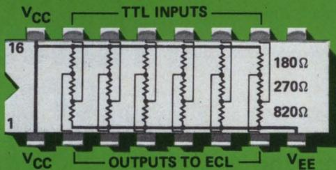
**SERIES 898-45 TTL TO ECL TRANSLATOR** contains six identical three-resistor sections for direct translation from TTL to ECL, both operating between a +5 volt supply and ground.
