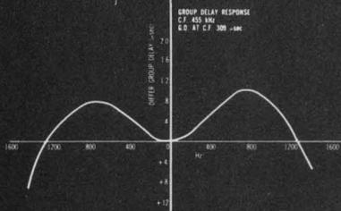
Designed for data transmission, Bulova has a line of group delay crystal filters that offer perfect phase linearity for optimum transmission conditions. Overshoot capable of being kept to 40 db (1%) below the steady state value — designs are so configured as to provide distortion-free selectivity at maximum speed, with a reduced error rate.
