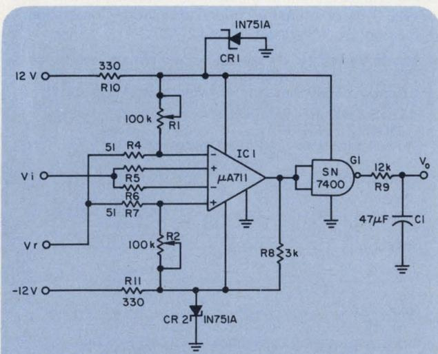
1. Window-comparator circuit produces a dc output proportional to the time during which input signal  $V_i$  falls within a window whose position is determined by reference voltage  $V_r$ . Thus the output is an analog of the input signals probability density function.
