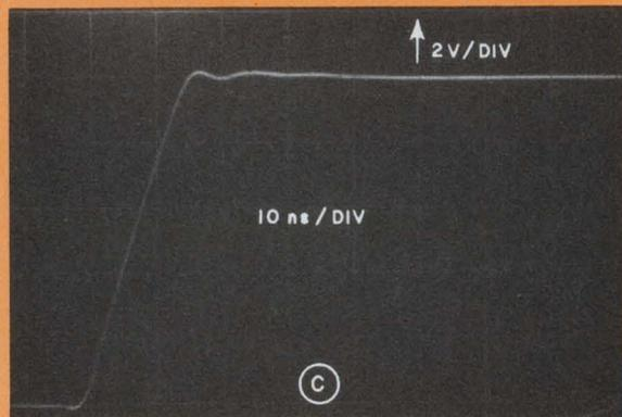
3. **Composite amplifier output measurements** show clean leading edges with little overshoot or ringing. Lower level positive (a) and negative (b) transitions, as well as the 10-V full-power transition (c), settle to within 3% of final value in 20 ns. The amplifier was operated at a gain of  $-10$  with a  $1\text{-k}\Omega$  load. The photos were obtained with an HP 222A pulse generator ( $T_r = 2.8\text{ ns}$ ) and Tektronix 647 scope ( $T_r = 3.5\text{ ns}$ ).
