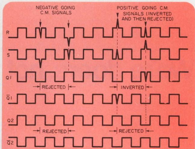
2. Waveform illustrates the excellent common-mode rejection properties of the two reset-set cascaded flip-flops.
