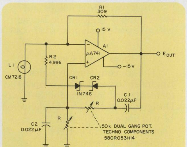
Waveform purity at low frequencies for a Wien bridge oscillator is enhanced by diode limiting. Lamp  $L_1$  stabilizes the loop gain at higher frequencies while the limiting action of  $R_2$ ,  $CR_1$  and  $CR_2$  prevents clipping at low frequencies.
