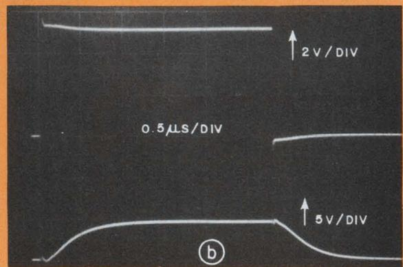
5. **With improper adjustment** of  $R_{N1}$ , the amplifier output (top trace) shows a slight droop (a) or overshoot (b).
