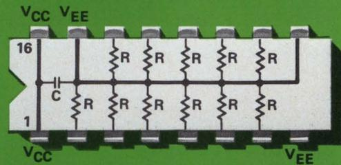
**SERIES 898-42 -5.2 VOLT TERMINATORS** contain twelve resistors for pull-down to the -5.2 volt bus. Each unit contains a 0.01  $\mu$ F decoupling capacitor to bypass the -5.2 volt bus.
