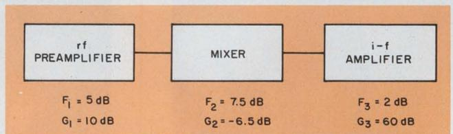
Let's start with the rf preamplifier and mixer. Place a straight edge on the nomogram to intercept the  $F_b$  line at 7.5 dB, for the mixer, and the  $F_a$  and  $G_a$  line at 15 dB, for the rf preamplifier. The intercept with the  $\Delta$  scale is 0.6 dB. This value is the incremental increase in noise figure for the mixer and preamplifier stages. The combined noise figure of these two stages is then
