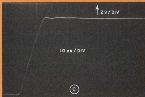
3. **Composite amplifier output measurements** show clean leading edges with little overshoot or ringing. Lower level positive (a) and negative (b) transitions, as well as the 10-V full-power transition (c), settle to within 3% of final value in 20 ns. The amplifier was operated at a gain of  $-10$  with a  $1\text{-k}\Omega$  load. The photos were obtained with an HP 222A pulse generator ( $T_r = 2.8$  ns) and Tektronix 647 scope ( $T_R = 3.5$  ns).
