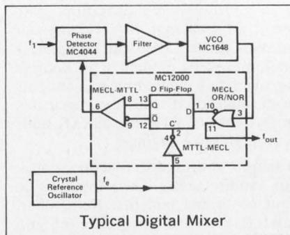
means to generate frequencies up to 250 MHz without the use of tuned circuits. The output frequency can be either a single fixed frequency or a series of programmable frequencies.
