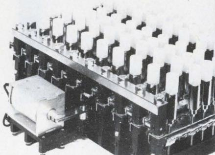
**ALTERNATE ACTION PUSH BUTTON SWITCHES**
