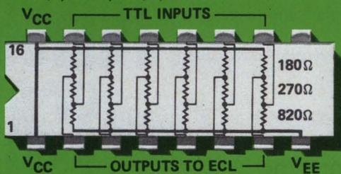
**SERIES 898-45 TTL TO ECL TRANSLATOR** contains six identical three-resistor sections for direct translation from TTL to ECL, both operating between a +5 volt supply and ground.
