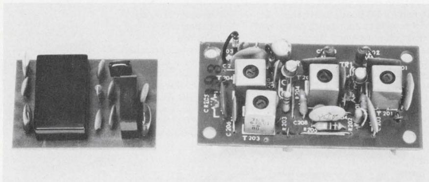
**An integrated sound i-f detector** using Semicon L (left) will be used to replace the more conventional discrete version (right) now used in television sets. The advantages include smaller size and fewer external components.
