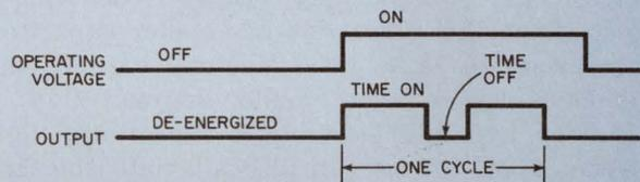
**Repeat-cycle timer**—An ON-OFF cycle repeats as long as the input circuit is energized.
