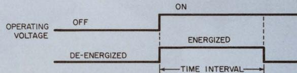
**Time interval on operate**—The load circuits are immediately energized, and remain energized, for only a specified time interval, after the input circuit is energized.
