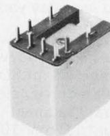
**GP.** A miniature general purpose relay with 2, 4, or 6 PDT contacts, rated 1, 2 or 5 amps, 28 vdc or 115 v, 60 hz. Coil voltages: 6-115 vdc. Consider the GP for copiers, business machines, control or alarm systems, etc. Available with single or bifurcated contacts.
