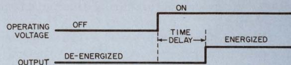
**Time delay on operate**—The load circuits are energized at a specific period of time after the input circuit is energized.
