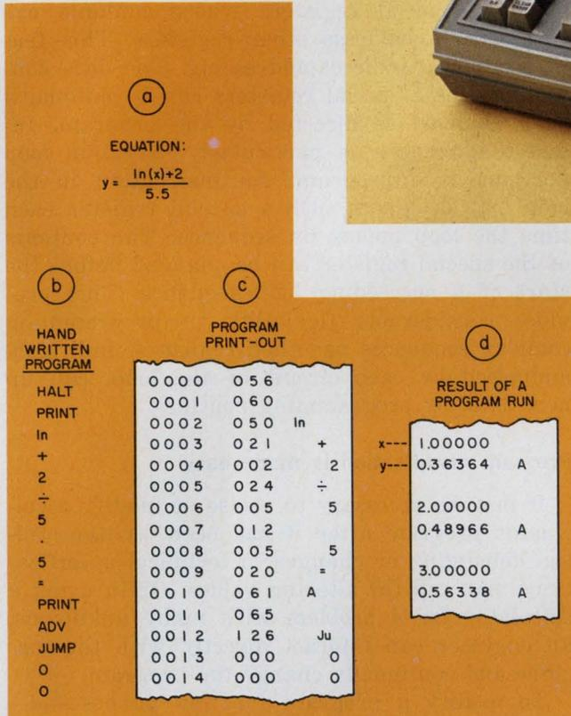
2. An equation containing transcendental functions like natural logarithms is easily programmed on an algebraic calculator. Enter variable  $x$  and answer  $y$  appears.
