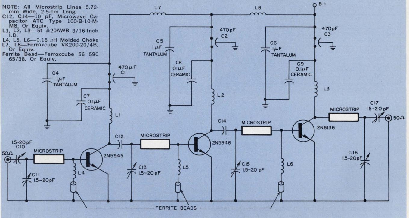
1. A three-stage, 450-to-512 MHz microstrip amplifier. This design features a minimum output power of 25
