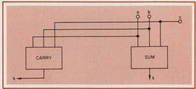
3. Block diagram of a conventional single-bit adder stage that uses single-rail logic. Sum and carry outputs are shown.
