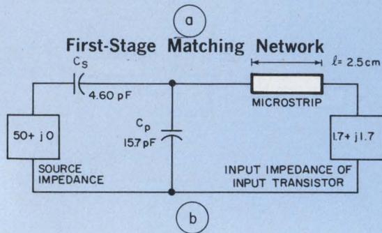
2. Transistor impedances are needed to calculate matching networks. These impedances can be measured or taken from published data (a). The input-stage matching network (b) sees a 50- $\Omega$  source and transistor input-impedance load.
