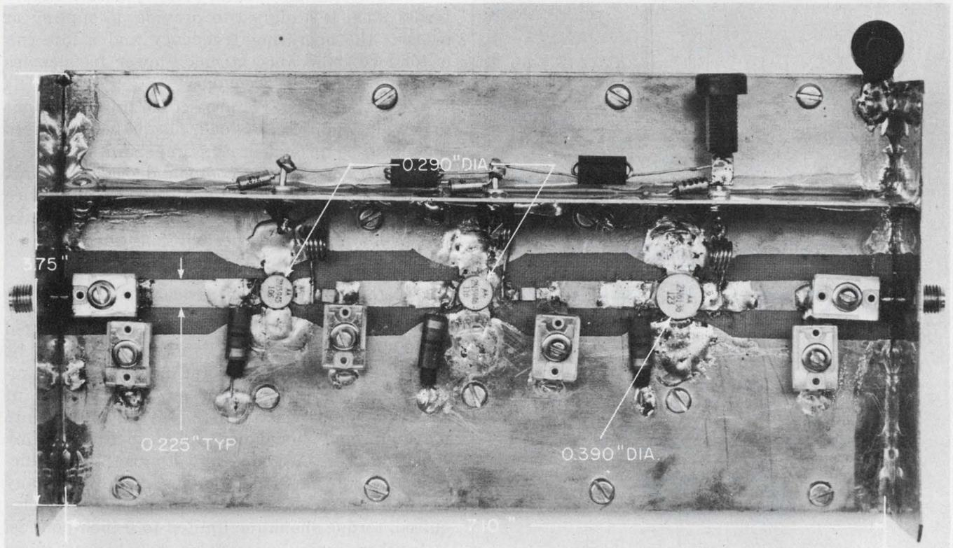
vides an additional 2.5 to 3.0 dB of gain over that obtained with compression trimmers. The chip dielectric capacitor use also reduces the number of tuning adjustments.
