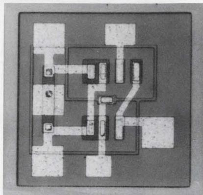
**Semicon L chip** measures 0.06 mm on each side and 0.15 mm thick. Standard processing techniques are used in fabrication.
