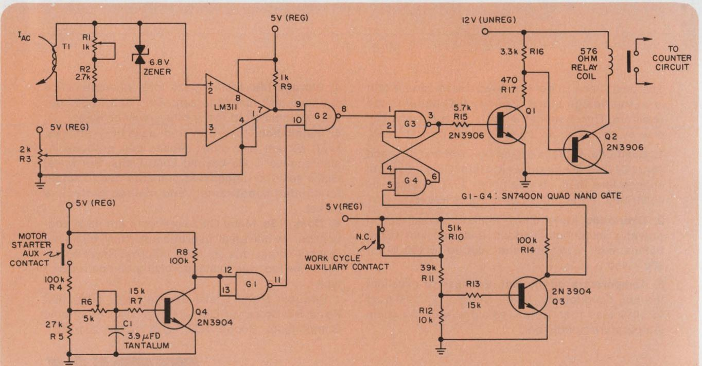
1. A rise in motor load current sensed by coil T<sub>1</sub> triggers an electromechanical counter when work is performed on a part in a manufacturing opera-
