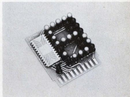
HP's new LED display is easily readable at distances up to 45 feet. The character is 1½ inches high, and average brightness is typically 1.25 millicandelas. Built-in decoder/driver circuitry allows direct addressing using standard BCD code.
