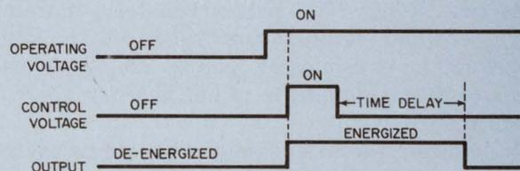
**Time delay on release**—The load circuits are energized when the input control circuit is energized, and they remain energized for a specific period of time after the control circuit is de-energized.
