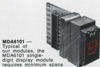
**MDA6101** — Typical of our modules, the MDA6101 single-digit display module requires minimum space in computer, avionic and military systems. Contains a decoder-driver circuit designed to accept four-input BCD (8, 4, 2, 1) code and to provide .27" visual readout of decimal numbers and nine distinct letters. Provides decimal point input and has ripple-blanking input and blanking input/ripple-blanking output terminals for zero suppression and intensity control.
