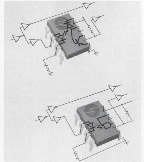
HP offers two new optically coupled isolators that take advantage of our advanced photo IC capability.
