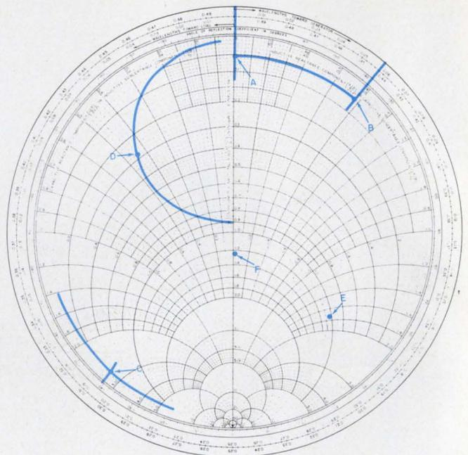
3. Capacitors  $C_s$  and  $C_p$  are calculated from this plot once the microstrip line length is fixed at 2.5 cm—a convenient value for our design. The capacitors for the remaining matching networks are determined in a similar manner.
