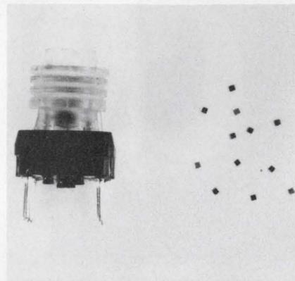
**Small coil** commonly used in transistor radio and TV sets (left) can now be replaced by a single Semicon L chip (right).
