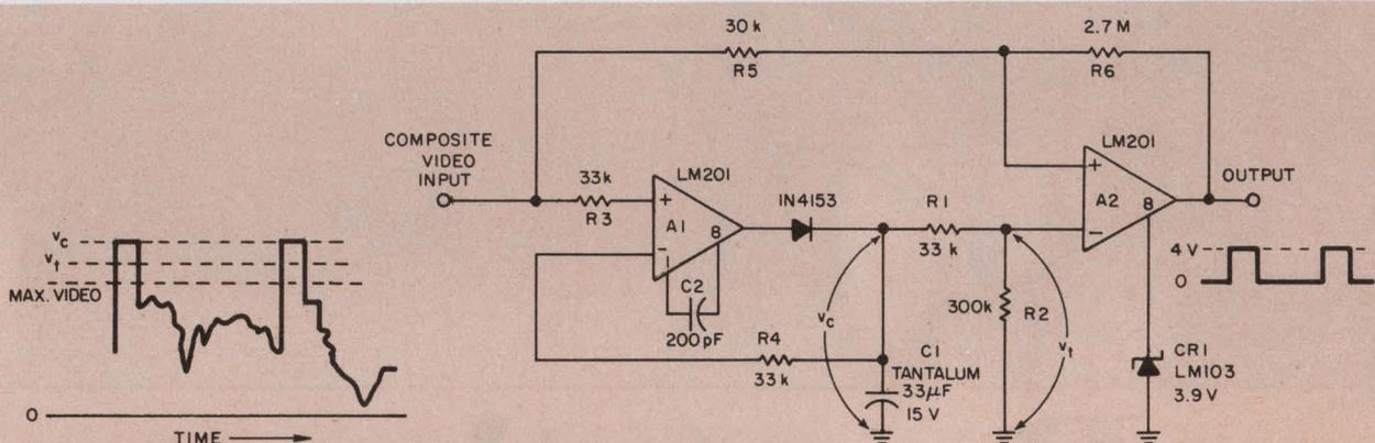
Peak detector  $A_1$  holds capacitor voltage  $v_c$  at the peak value of input pulses. A fixed fraction of this
