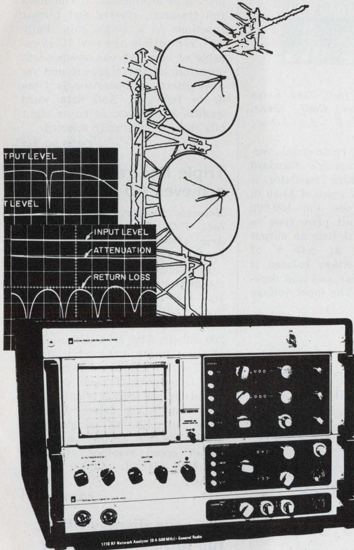
**FOR** cable measurements you need a wide 400 kHz-to-500 MHz sweep range and a simultaneous display of attenuation and return loss.
