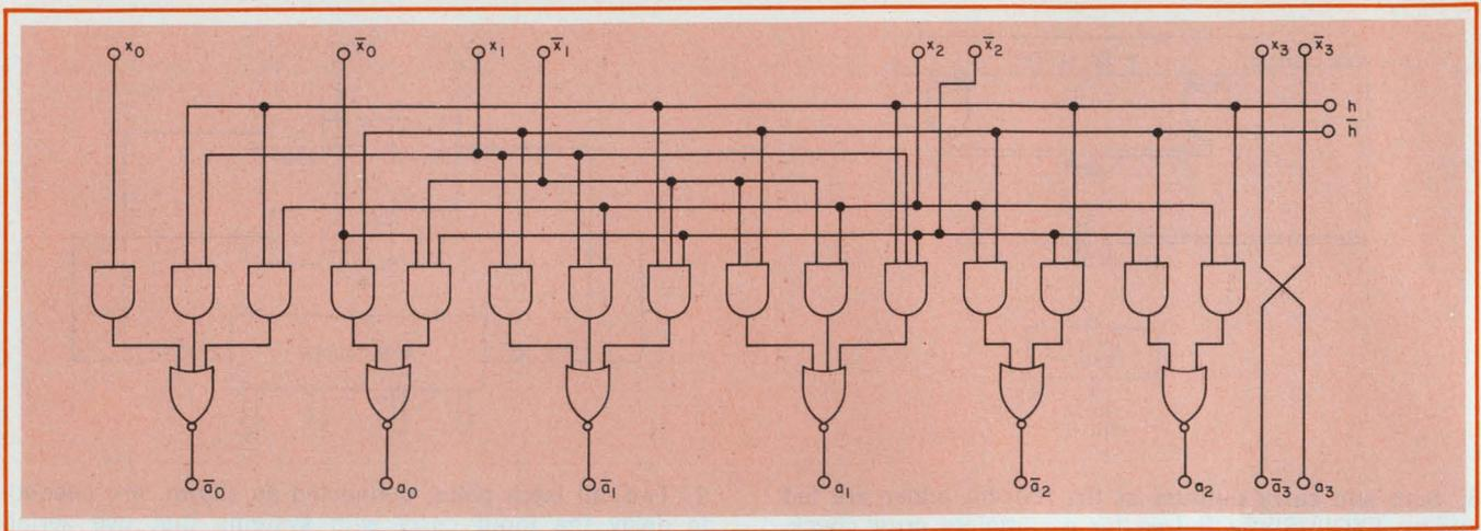
11. Input decimal-correction network adds a count of six to each four-bit group. If a similar network is con-
