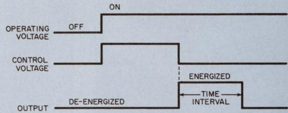
**Time interval on release**—The load circuits are energized after the input control circuit is de-energized and the load remains energized for a specified time interval.
