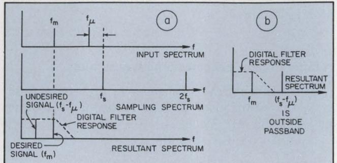
12. Aliasing of undesired signals into the passband is a serious problem in digital filters. Raising the sampling frequency helps reduce this problem.
