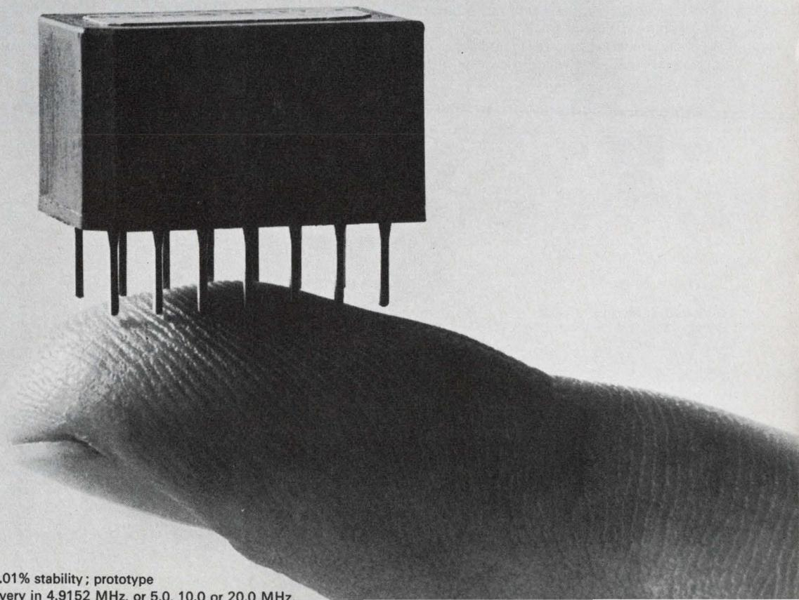
Specifications: 4 to 20 MHz range; 0.01% stability; prototype quantities available for immediate delivery in 4.9152 MHz, or 5.0, 10.0 or 20.0 MHz
