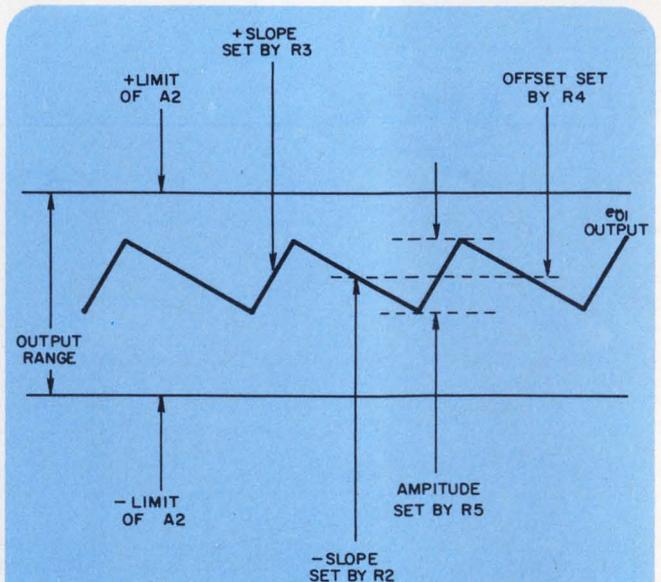
2. Triangular-wave output has positive and negative slopes, which may be varied independently of amplitude by potentiometers  $R_3$  and  $R_2$ .
