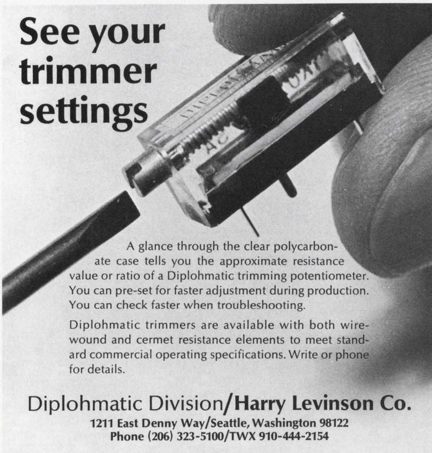
A glance through the clear polycarbonate case tells you the approximate resistance value or ratio of a Diplohmatic trimming potentiometer. You can pre-set for faster adjustment during production. You can check faster when troubleshooting.
