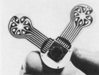
The silicon element—used in differential pressure and direct pressure transmitters—is sealed in a silicon fluid through which the fluid pressure is transmitted.
