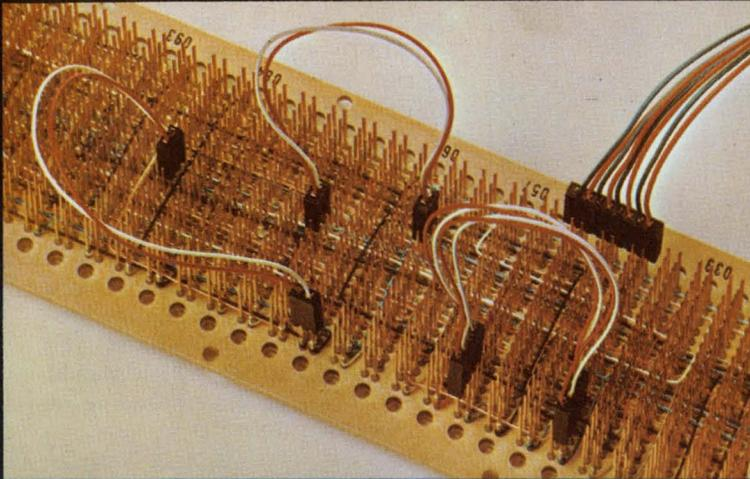
**level 3** Low cost strip connectors (above) are used as jumpers in back plane wiring. Intermates with .025" square or round posts. ■ Circuit Concentration Bay (below) consists of wire wrappable panels that are five times as compact as the telephone distribution frames they replace.
