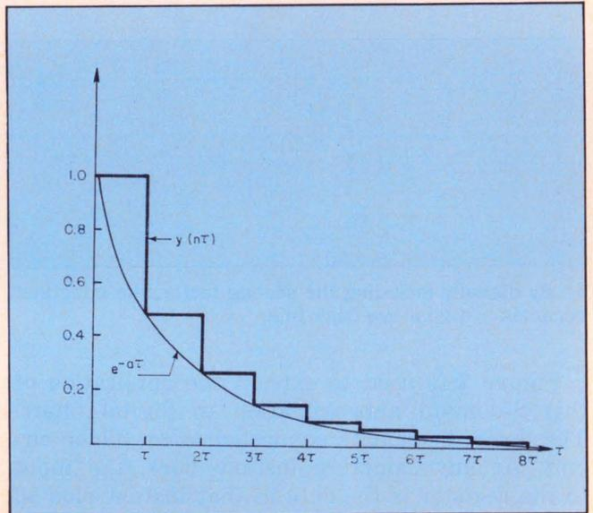
9. The step response of the digital high-pass filter as derived by the S-domain approximation is compared to its theoretical value.
