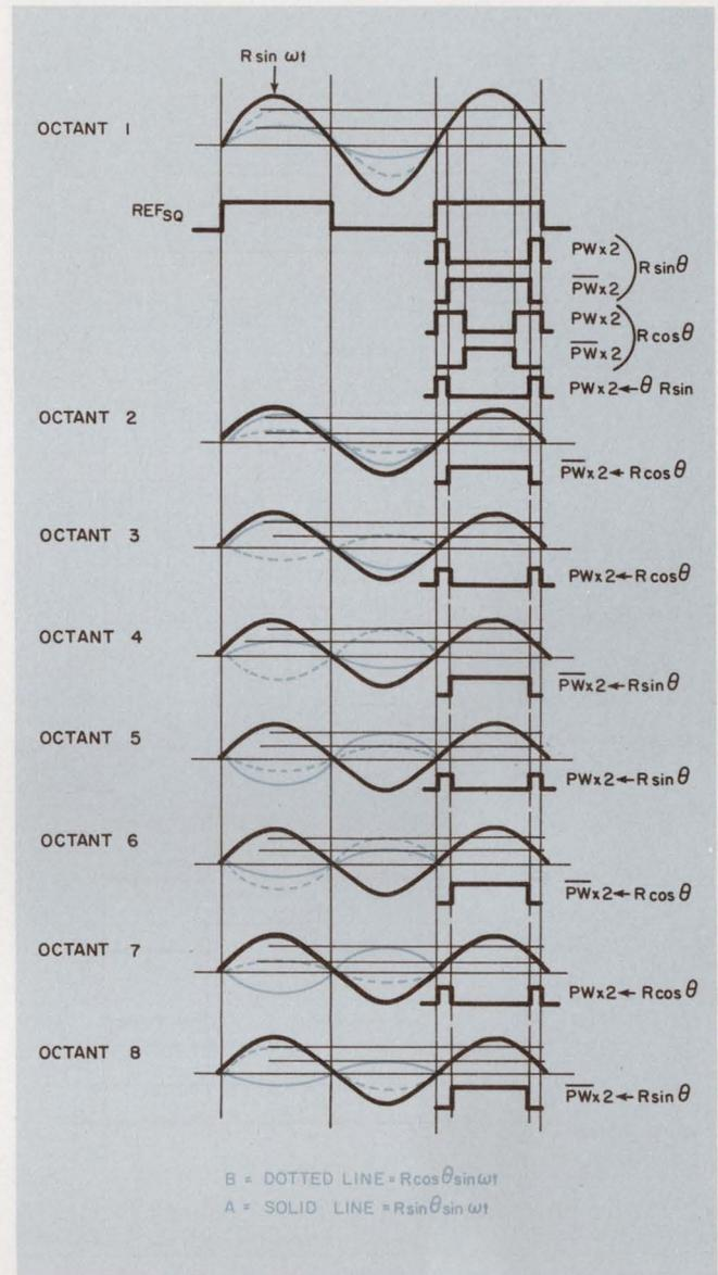
4. Selection of the encoded angle's octant is done after determining the corresponding quadrant (see Table 1) and then "looking" at the waveshapes shown above.
