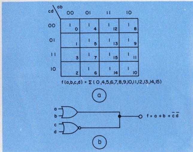
3. Function plotted on Karnaugh map (a) is realized in implied-OR form (b). DeMorgan's theorem is used to re-arrange the function to the implied-OR form.
