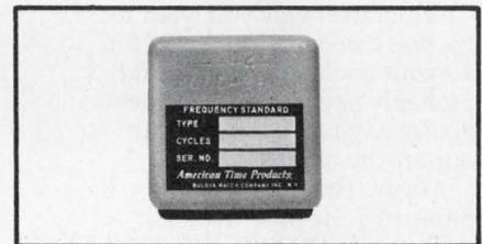
The news in *subminiature fork oscillators* is a unit which uses less than 5 ma. The oscillator, developed by Bulova and designated the FS-11-1, takes up about  $\frac{1}{2}$  cu. in. of space and weighs one ounce. Their units have accuracies up to  $\pm 0.0005\%$ , 90% reliability for 200,000 hrs. and logic circuit compatibility.
