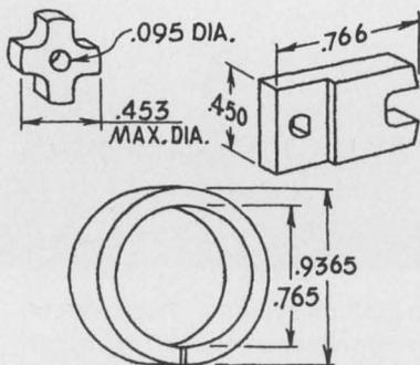
Intricate configurations such as these are typical of the many shapes produced through Indiana General's sintering facility. Precise tolerance and superior finish can eliminate grinding operations to lower your magnet cost in many applications.
