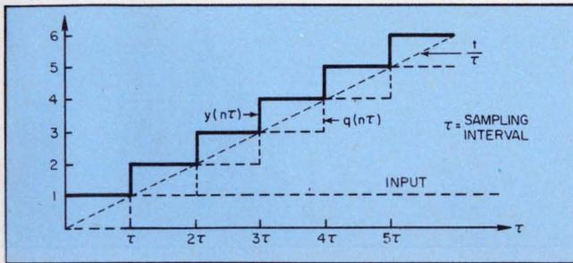
3. The response of the circuit in Fig. 2 to a step input shows that it behaves as an integrator.
