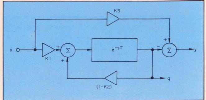
8. Digitally including the scaling factors,  $K_1$ ,  $K_2$  and  $K_3$ , converts the differentiator to a digital high-pass filter.
