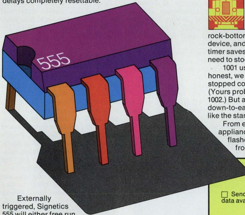
Externally triggered, Signetics 555 will either free run or latch, in adjustable duty cycles from 50% to 0.01%. Timing can be changed 10:1 with control. Operating from 5 to 15 volts with only a 1% change in timing. Output can source or sink 200mA. Temperature stability: 0.005% per °C.
