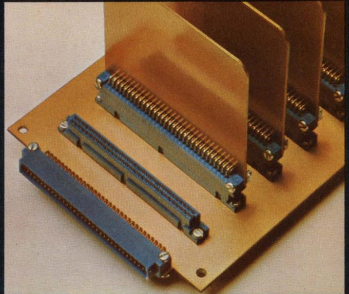
**level 2** Box contact connectors (above) intermate with .025" square or round contacts. Low insertion force. Terminations for crimp, wire wrapping or wave solder. ■ Zero insertion force connectors (below) improve PC board and connector life by eliminating strain and wear.
