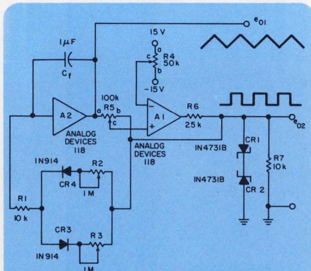
1. Integrator  $A_2$  generates a triangular wave from the square-wave output of comparator  $A_1$ . Resistor  $R_5$  controls amplitude, but has no effect on slope.
