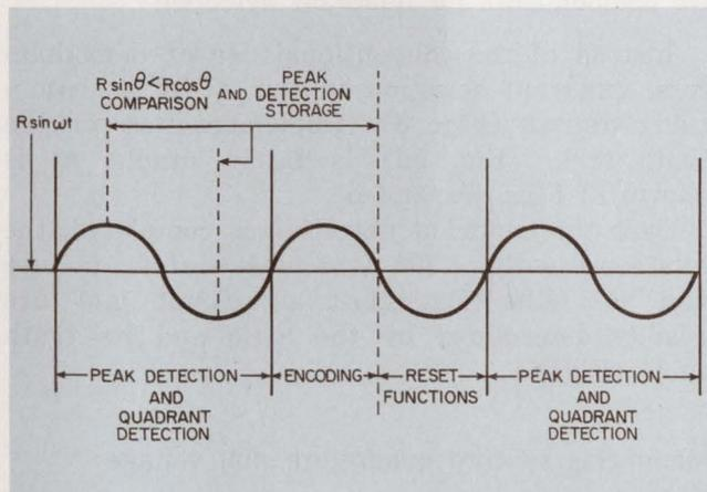
3. Use of a complete cycle of the reference signal ( $R \times \sin \omega t$ ) results in fewer components and simpler logic for timing various encoding events.
