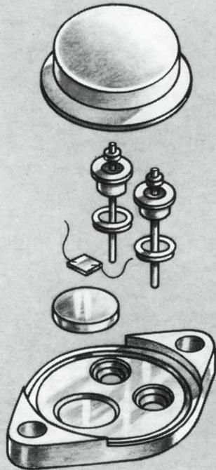
**Steel package—TO-3, glass-to-stem, compression seal**
