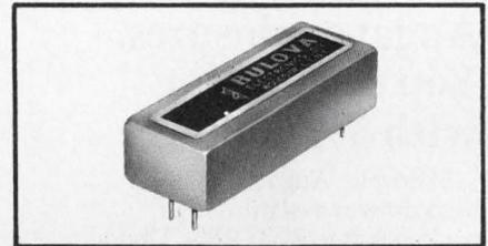
Group delay crystal filters offering perfect phase linearity for optimum data transmission are also available from Bulova. Overshoot is kept to 40 db (1%) below the steady state value. The filters provide distortion-free selectivity, at a maximum speed, and have a reduced error rate. Bulova's complete line of crystal filters meet all transmission specifications from 4 KHz to 150 MHz.
