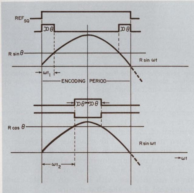
2. To eliminate pulsewidth jitter at large angles, both outputs of the Scott-T transformer ( $R \times \sin \theta$  and  $R \times \cos \theta$ ) are used. The  $R \times \sin \theta$  is used for angles of less than  $45^\circ$ , and  $R \times \cos \theta$  is used for angles of more than  $45^\circ$ .
