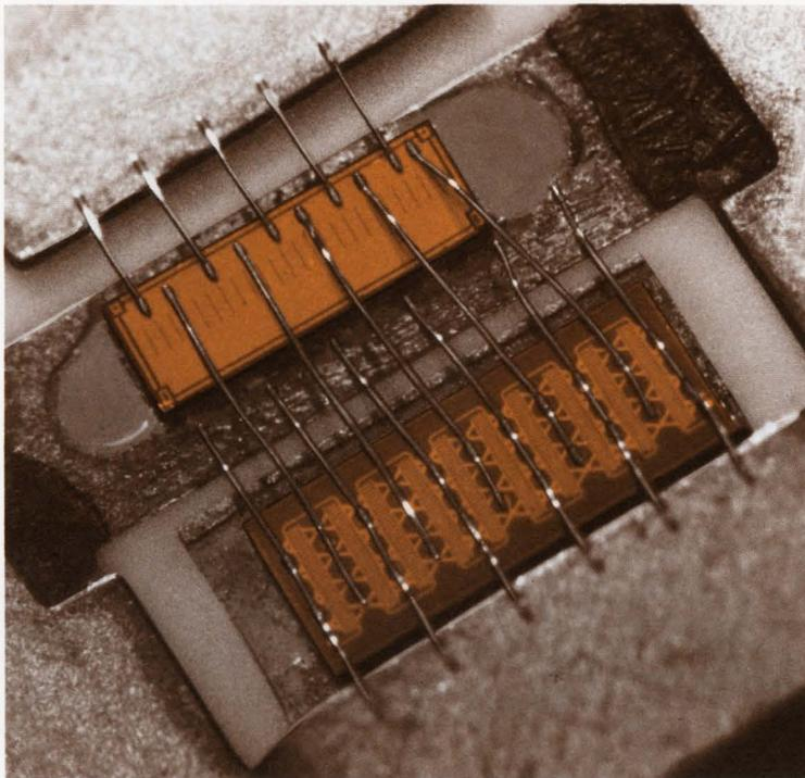
Controlled-Q RF transistors employ MOS capacitor chips to transform base impedance and improve broadband performance.
