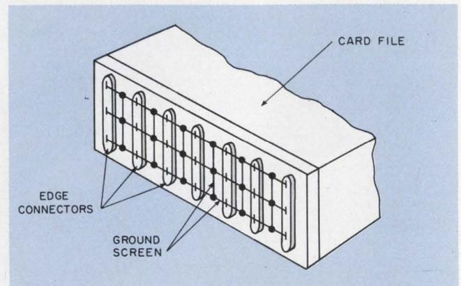
3. Ground screen simulates a ground plane. This construction is useful when a solid plane is not practical, as can be the case in point-to-point wiring.
