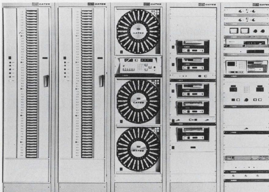
**Automated programming system** by Gates Radio uses cartridges for both music (racks on left) and commercials (carousels in center). A digital clock controls station operation according to a preprogrammed magnetic tape.
