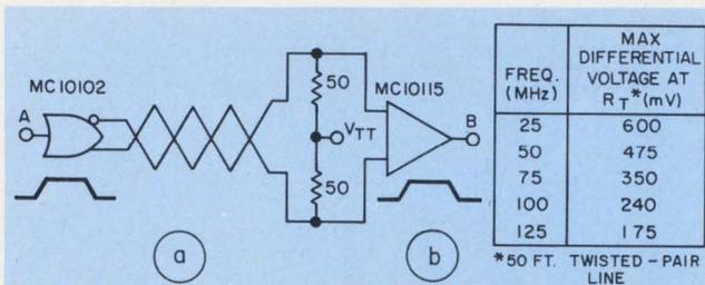
5. Pull-down resistors can also terminate a twisted-pair line (a), providing full output levels to the receiver. Attenuation data for 50 feet of twisted-pair line and 50  $\Omega$  pull downs (b) show higher differential voltages.
