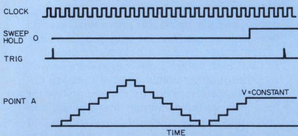
2. Timing sequence for an eight-bit register is illustrated by the waveform for the output at point A.
