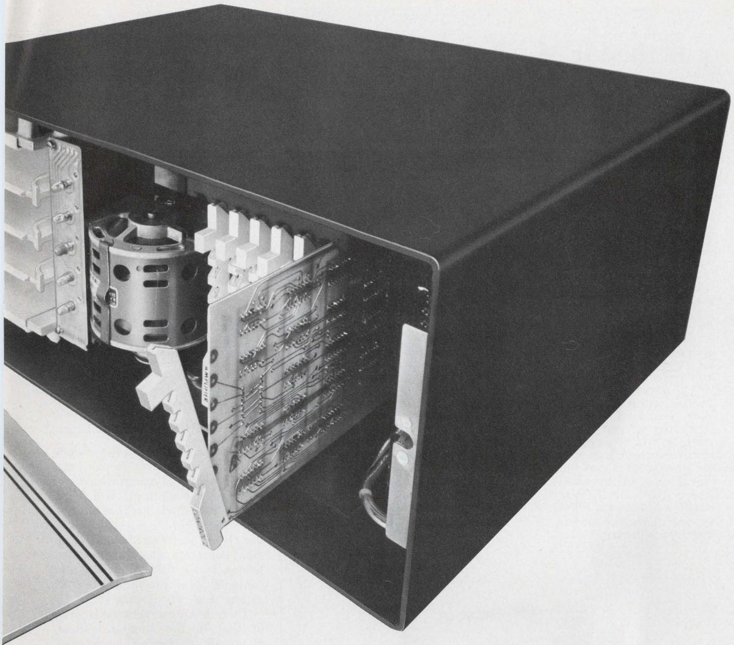
No mechanical gimmicks. Nothing exotic to go haywire. It uses only 3 parts to move tape: a motor, a capstan, and a pinchroller actuator (a pinchroller is built into each CartriFile cartridge). For each additional tape drive, we only add ONE more moving part: an actuator. CartriFile's mechanical simplicity results in unbelievably long MTBF. Just ask our customers.
