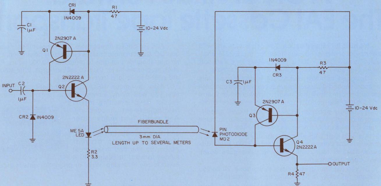
Transmitter and detector operate without standby power. Complementary switches  $Q_1 + Q_2$  and  $Q_3 +$
