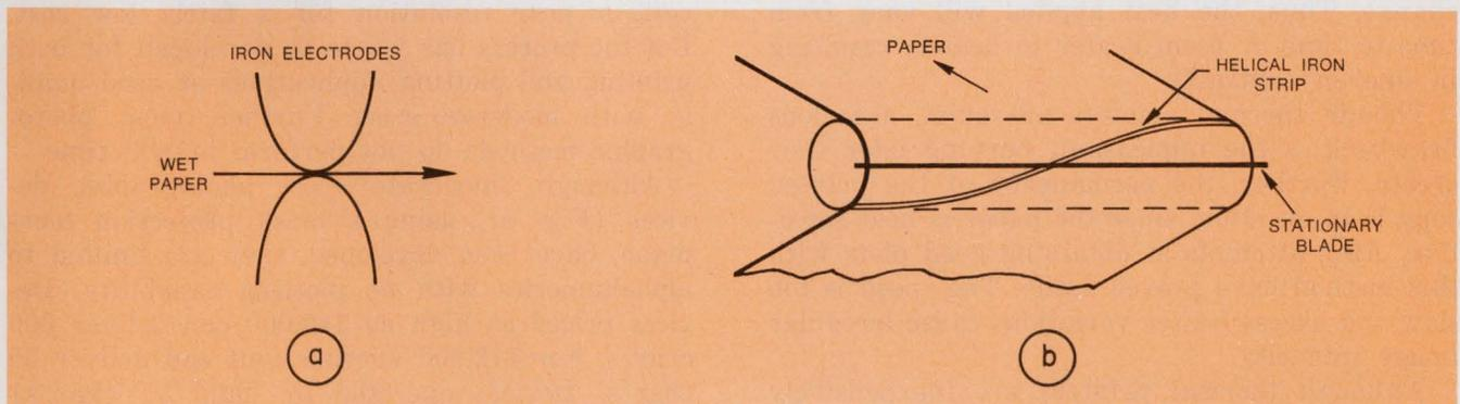
4. Electrolytic printer/plotters are inexpensive, but the poor cosmetics and short life of the copy limit appli-
