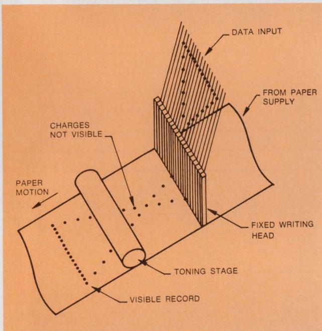
7. **Electrostatic methods**, when properly implemented, provide a good approach to building a combined printer/plotter. Speed is independent of image complexity.
