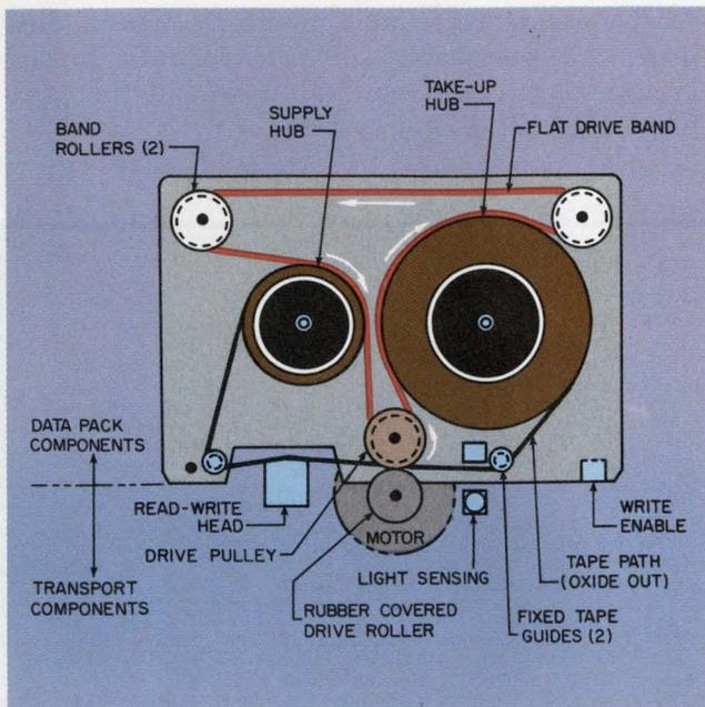
**Data cartridge from 3M Co.** uses 1/4-in tape wound on two coplanar reels. This cartridge accepts four tracks of data recorded at a density of 1600 bpi. A unique plastic drive band maintains tape tension within the cartridge and allows single-point driving at speeds of up to 90 ips.
