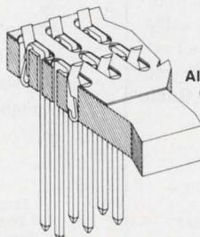
Allows for visual inspection of point of connection to component lead!
