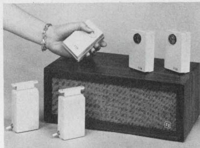
**A radio-frequency burglar alarm** by Electronic Radio Guard, Inc., features easy installation and operation.
