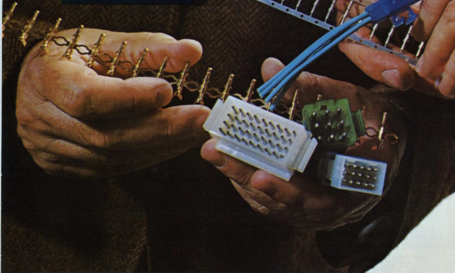
**MAKE YOUR CONNECTIONS: FAST.** With Molex standard and miniature connectors. They're easier to work with. Simplify wiring. Speed production. Save assembly steps. Make installation and servicing extra easy, too. This is why circuitry idea men everywhere are making connections with Molex. From one circuit to 104 or more. Production keyed and available in a variety of colors to meet design requirements. Molex has the
