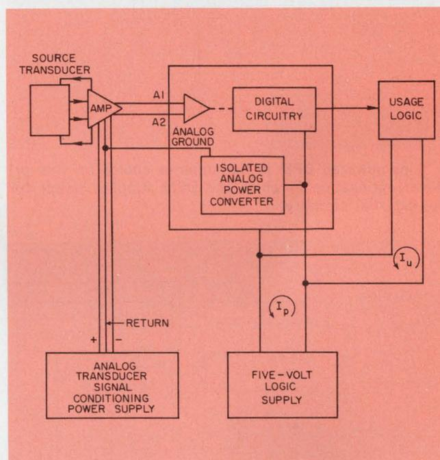
3. Differential inputs plus a power converter eliminate the multiple paths and the erroneous readings.
