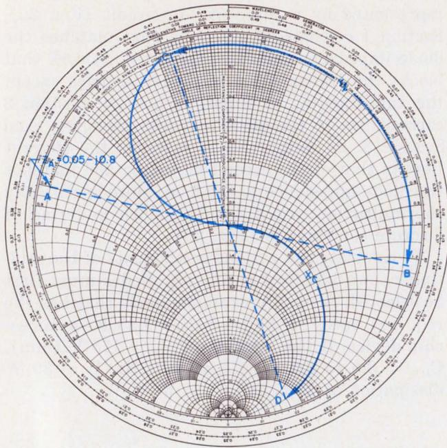
3. The calculation of the input matching elements,  $C_4$  and  $L_5$ , is performed graphically with a Smith chart. All that's needed to start the calculation is  $Z_A$ , one-half of the input impedance of a diode.
