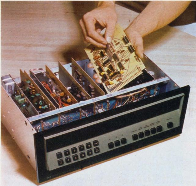
The take over of linear applications by digital circuits is beginning to take place. Initial applications are in TV and FM tuners, like this one from the Heath Co.
