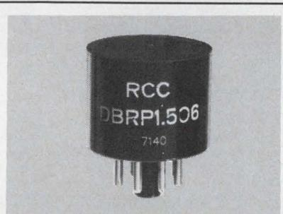
**RCC Dual Silicon Single Phase Bridge Rectifiers** — Two 1.5 Aav bridge rectifiers in one 8 pin plug-in base. Volt. Rat. -50 to 800V., Max. Serv. Appl., 1-99 quant. \$2.95 to \$6.00 dep. on Voltage. Rectifier Components Corp., Freeport, NY. Tel: 516 868-0470
