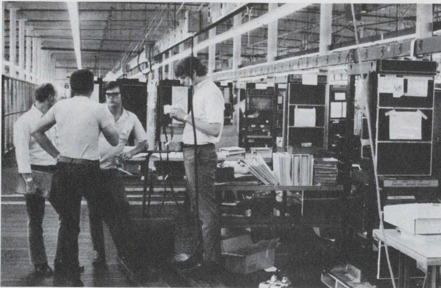
**PDP-11/45 computers are being tested** before shipment by two PDP-11/20 minicomputers at Digital Equipment Corp.'s plant in Maynard, Mass.
