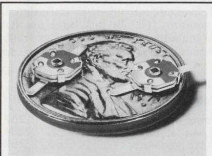
**Thin-Trim® variable capacitors** are designed to replace fixed tuning techniques. Applications include crystal oscillators, CATV amplifiers, communication and test equipment. Series 9410 has high Q's with five capacitance ranges from 1.0 - 4.5 pf to 10.0 - 50.0 pf. Johanson Manufacturing Corporation, Boonton, N. J. (201) 223-2676
