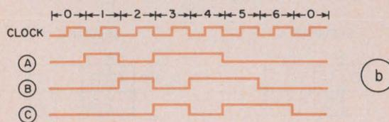
**5. The final divide-by-seven counter, using two AND gates and one OR gate. The timing waveforms are in b.**
