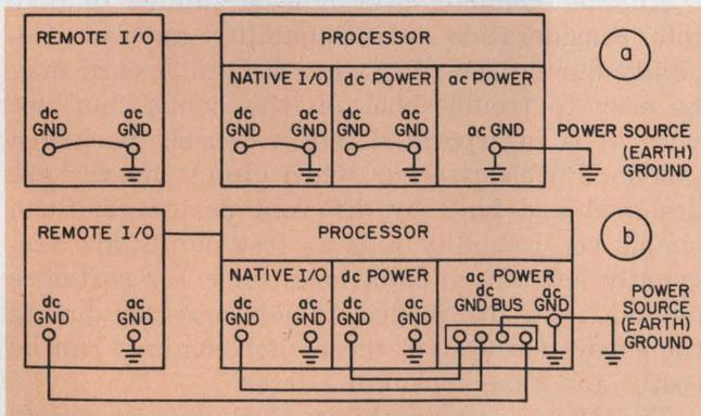
2. Ground loops develop when individual subsystems are integrated into a total system and dc ground points are connected to multiple ac grounds (a). By tying together all dc grounds and then connecting them to a single ac ground, the problem is eliminated (b).
