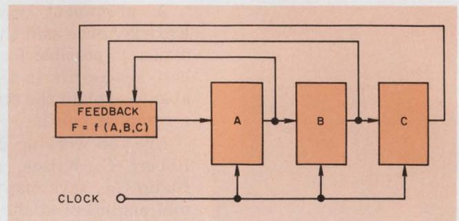
1. Three-stage shift counter with feedback to the first stage. The goal is to determine the minimum logic.
