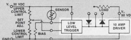
As an ON-OFF controller, LMD-1 can control any parameter convertible into resistance change. A 0.5 kW load can be controlled with only 80 nA typical bias input from the sensor. Schematics are available for applications at right.
