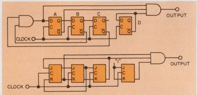
9. J-K and D-type divide-by-10 counters are obtained by using divide-by-five and divide-by-two counters.
