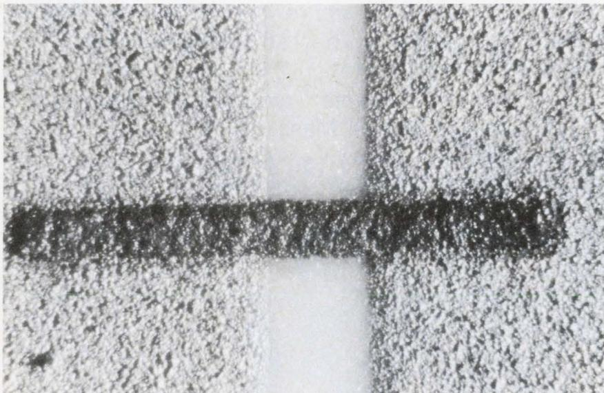
Photomicrograph shows a two-terminal switch 10-mil wide by 15-mil long (dark line), terminated by Pd/Ag conductors. The light gray alumina substrate, 20 mils thick appears between the conductors.
