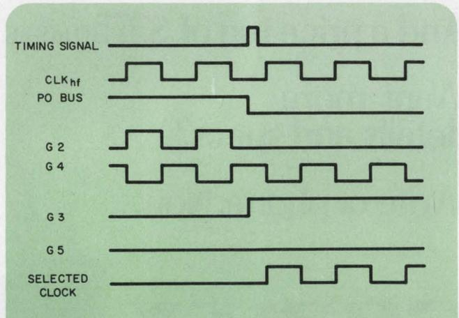
2. Waveforms show the selected clock in relation to the various gate outputs. Maximum phase uncertainty is equal to the period of  $CLK_{hf}$ .
