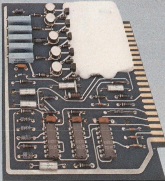
For protection against moisture, dirt, ozone, radiation and many solvents and chemicals, select this conformal coating. It flows on easily and cures at room temperature to a tough silicone rubber with excellent dielectric properties. Information retrieval number 224.
