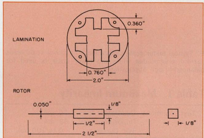
5. Lamination and rotor used in the breadboard model. The magnetic rotor is suspended in a low-friction pivot. Rotational restraints are not needed since there is no moving coil or flexible conductors.
