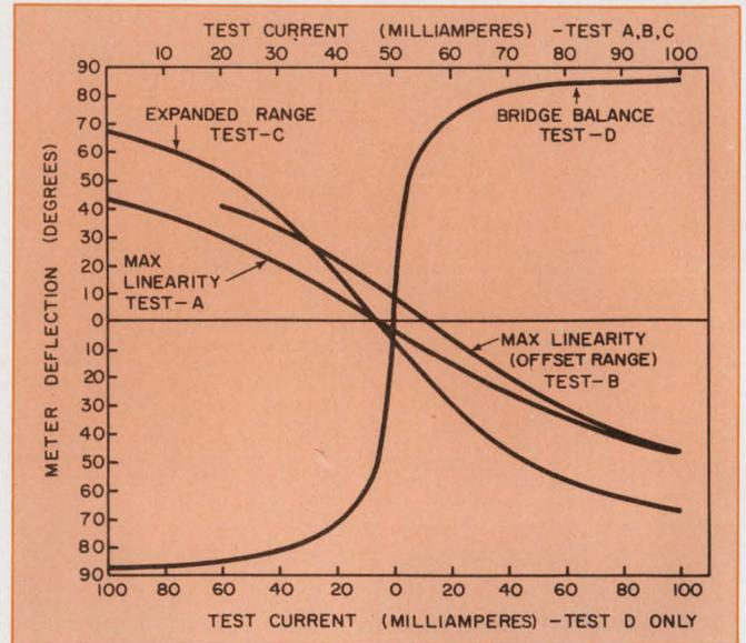
7. The results of various tests conducted with the model define the device characteristics for various operating modes. The curve resembling a magnetization curve gives the performance in the balanced condition.
