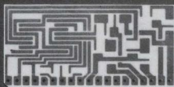
2. METALLIZED THICK FILM CONDUCTOR
