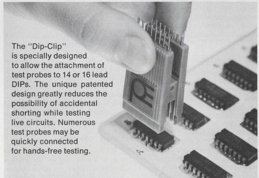
The "Dip-Clip" is specially designed to allow the attachment of test probes to 14 or 16 lead DIPs. The unique patented design greatly reduces the possibility of accidental shorting while testing live circuits. Numerous test probes may be quickly connected for hands-free testing.
