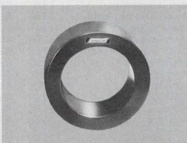
**Dynacor® miniature square-loop tape cores** (2 kHz to 500 kHz) in O. D. sizes from .203" to .675" at low cost. Low-power/High freq. for magnetic amps or guaranteed max. magnetizing current at hi-freq. over wide temp. range. For DC to DC converters. Dynacor, 1010 Westmore Ave., Rockville, Md. 20850 (301) 424-6900.
