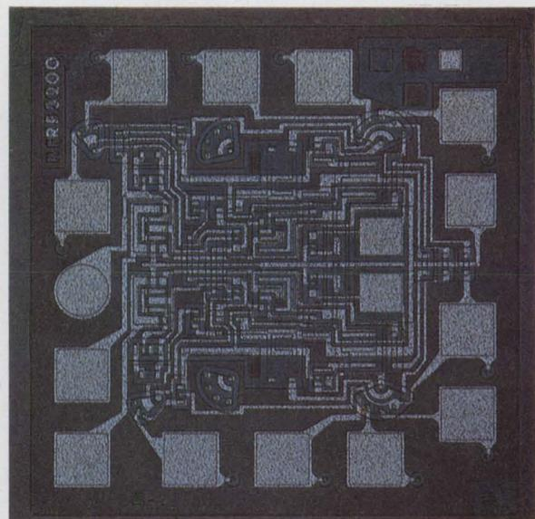
An AND-input J-K flip-flop is offered in the RAY III series from Raytheon Semiconductor. Termed the RF3200, it has a listed speed of 10 ns.
