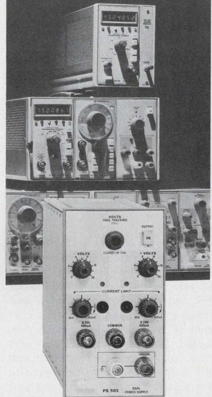
These high density, easy to operate supplies are designed for today's devices. Ideal for circuit investigation, device testing and educational applications. The PS 503 is a dual power supply with precisely regulated, shortproof outputs variable independently or at a constant ratio. All plug-ins have a +20 V floating supply and +5 V ground referenced supply.
