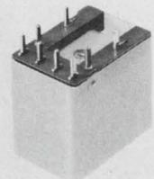
**GP.** A miniature general purpose relay with 2, 4, or 6 PDT contacts, rated 1, 2 or 5 amps, 28 vdc or 115 v, 60 hz. Coil voltages: 6-115 vdc. Consider the GP for copiers, business machines, control or alarm systems, etc. Available with single or bifurcated contacts.
