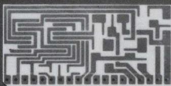
2. METALLIZED THICK FILM CONDUCTOR
