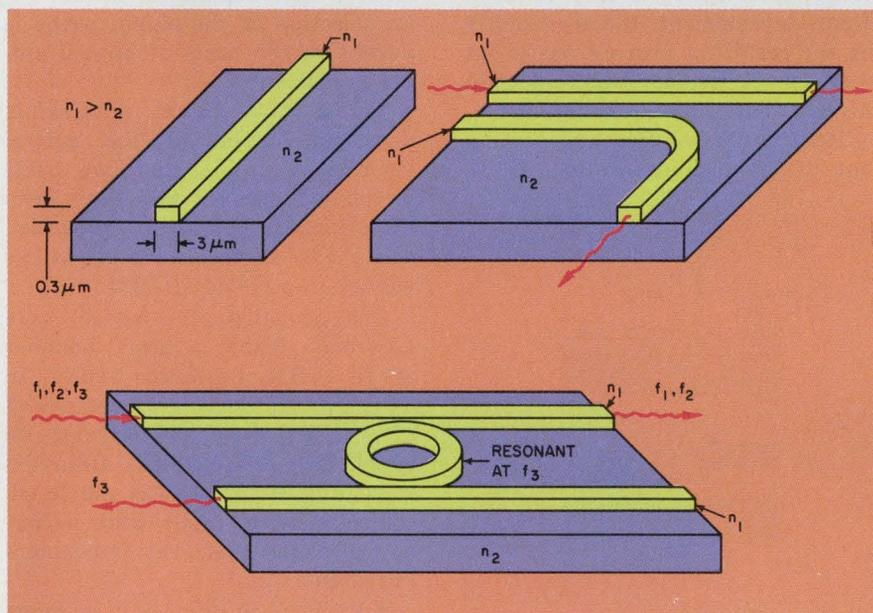
**1. Representative types of proposed passive waveguide structures for optical integrated circuits. They range from a simple, single-mode structure (a) to a directional coupler (b) and to a frequency-selective filter (c).**
