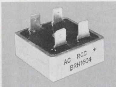
**RCC BRH1600 series 16 amp./65°C. single phase silicon bridge rectifiers.** Available voltage types of 50 to 800 volts peak with single cycle surge current ratings of 125 amps. peak. 1-99 quant. \$3.30 to \$6.60 dep. on voltage type. Rectifier Components Corp., Freeport, N.Y. 516-868-0470.
