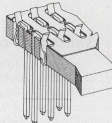
Robinson-Nugent invites your attention to its new, unique one-piece contact/terminal concept. When inserted in board, the unit becomes a properly aligned, self-supporting connector/socket for ICs or a complete back panel solderless interconnection system.
