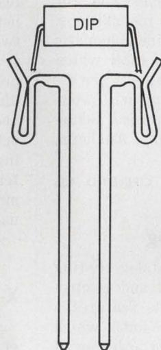
**Permits extremely short lead-length** - as short as .035" below device for full contact!
