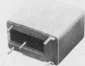
**Series 38.** DPDT, 3 amp 28 vdc contacts. Coil ratings 3-24 vdc. Applications include business machine controls, antenna rotor controls, industrial process controls, etc.
