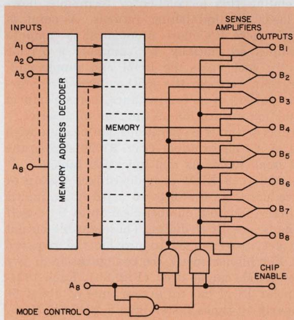
B. Some ROMs have variable configurations. This MM 4230/MM 5230 model, for example, can be either a  $256 \times 8$  or  $512 \times 4$  ROM.
