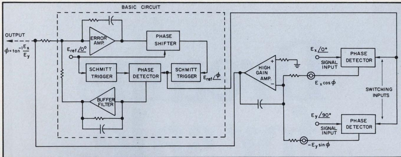
5. An all-electronic resolver is an interesting application for the wide-range phase shifter. Outputs from the two extra phase detectors,  $E_x \cos \phi$  and  $E_y \sin \phi$ , are dc analogs of the resolved sin/cos components of the ac
