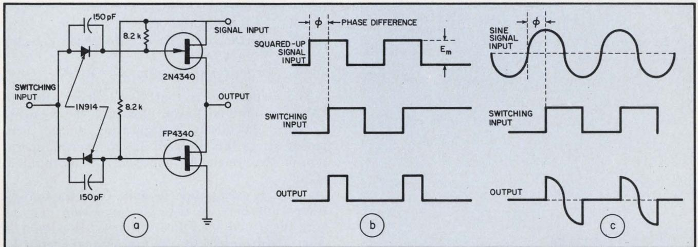
3. This typical phase detector circuit provides a pulsed output. Its average value is directly proportional to the phase difference of the inputs when a squared-up signal input is applied, as in 3(b). The phase-detector output
