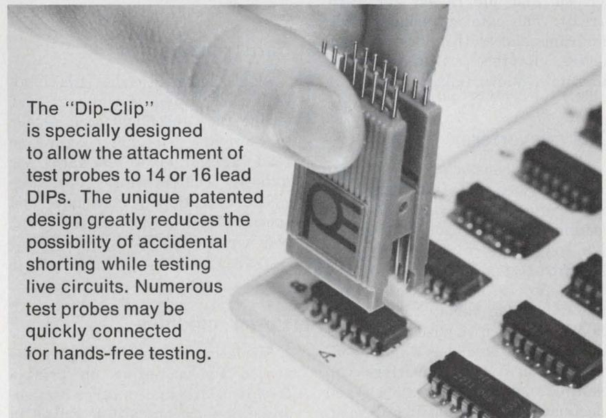
The "Dip-Clip" is specially designed to allow the attachment of test probes to 14 or 16 lead DIPs. The unique patented design greatly reduces the possibility of accidental shorting while testing live circuits. Numerous test probes may be quickly connected for hands-free testing.
