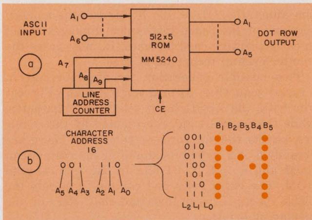
5. A raster-scan circuit for the generation of ASCII characters (a). The output provides the dot-row information for a typical 5 x 7 character (b). This technique is often used for TV monitor tubes. A total of 8 x 5 x 64 bits are stored in the ROM.
