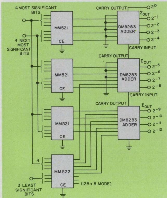
2. This four-ROM lookup table is more efficient for deriving accurate mathematical functions, such as  $\sin x$ . It can generate 2048 values of  $\sin x$  by the use of an interpolation technique.
