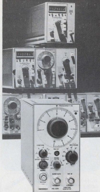
The FG 501 is a .001 Hz to 1 MHz function generator with sine, square, triangle, pulse, and ramp outputs. Harmonic distortion is low. VCF input has 1000:1 range. Gate/burst input has phasing variable from  $-90^\circ$  to  $+90^\circ$ .
