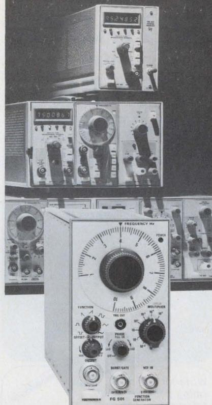
The FG 501 is a .001 Hz to 1 MHz function generator with sine, square, triangle, pulse, and ramp outputs. Harmonic distortion is low. VCF input has 1000:1 range. Gate/burst input has phasing variable from -90° to +90°.
