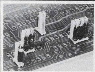
**Verti-Mount Insulators** permit vertical mounting of DO-7, DO-34, and DO-35 diodes and 1/8-, 1/4-, and 1/2-watt resistors on printed circuit boards. Verti-Mounts increase packaging density by 200%. Robison Electronics, Inc., 2134 W. Rosecrans Avenue, Gardena, Calif. 90249. Phone: (213) 321-0080.
