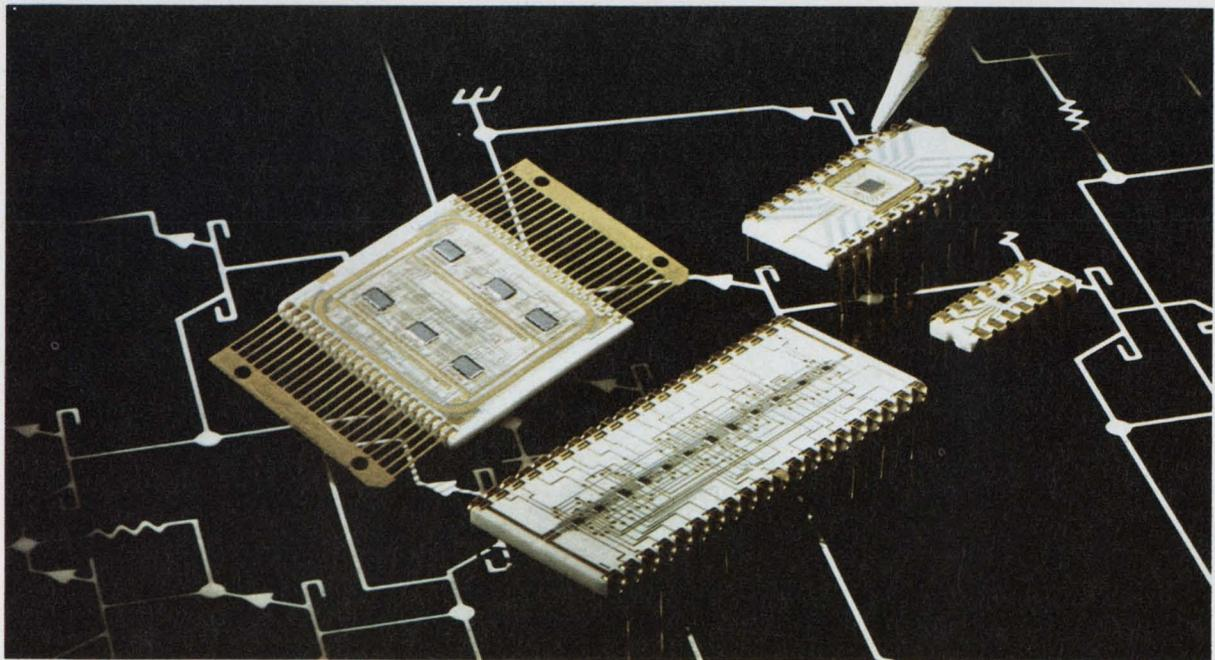
**Beam-lead low-power Schottky TTL boasts 19 pJ speed-power product—the lowest of any standard line. Not intended for the higher speed ranges, the**
