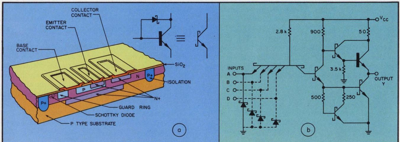
2. A Schottky barrier diode in parallel with the base-collector junction of saturating npn transistors (a) form the basis of S-TTL. There is no stored charge and the Schottky diode has a lower forward voltage drop than a
