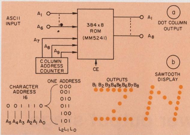
6. An alternate character-generation technique, vertical scanning with a ROM (a), provides high-resolution characters for sawtooth-scan CRTs or paper-tape printers (b). In all,  $6 \times 8 \times 64$  bits are stored in the ROM. The character matrix is  $7 \times 5$ .
