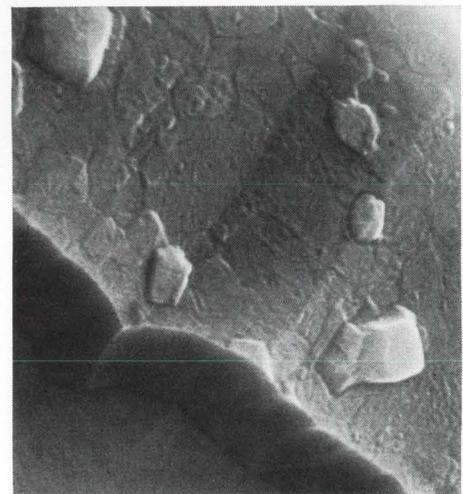
6000 X magnification shows excellent metal coverage over an oxide step. The scanning electron microscope has become a major tool in RCA's diagnostic and high-reliability procedures.
