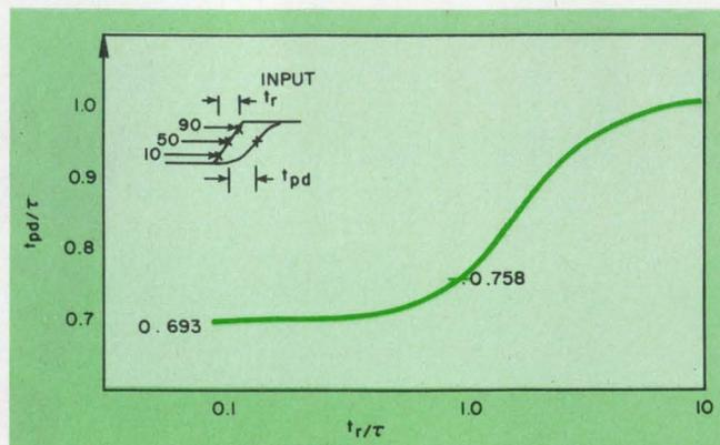
2. Propagation delay is minimum for a zero-rise-time (step) input pulse, and it approaches a maximum value of  $\tau$  for infinite rise time.
