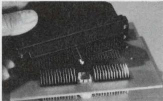
And there's more. The DL *Instamate* contact accommodates #20 through #30 AWG solid or stranded wire. The contact mating life exceeds 10,000 cycles — 20 times the norm. There are contact arrangements with 96 or 156 positions on a .100" grid. Removable con-
