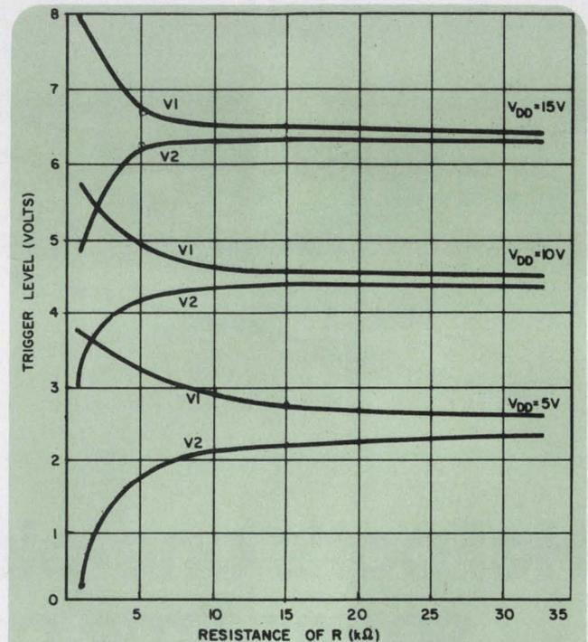
2. Trigger levels plotted against resistance of R for three values of dc supply voltage  $V_{DD}$ . V1 is the ON trigger, V2 is the OFF.
