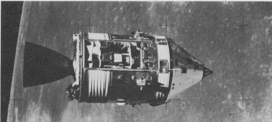
The Lunar Sounder radar will orbit the moon in Apollo 17's service module, similar to the Apollo 15 module shown here. Retrieval of the radar's film will require a walk in space from the command module and back.
