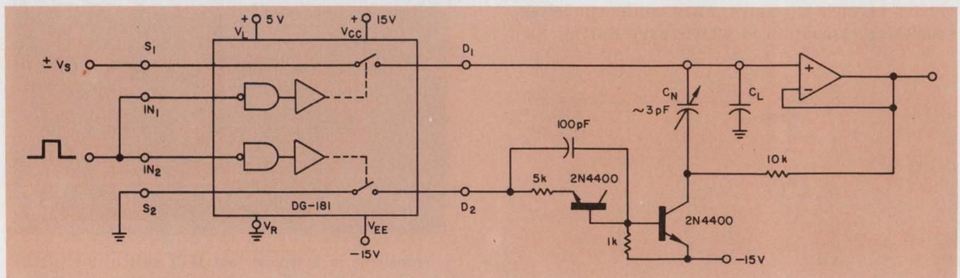
7. This neutralization circuit is almost perfect over a  $\pm 15$ -V signal range. It uses a dual driver and the DG181
