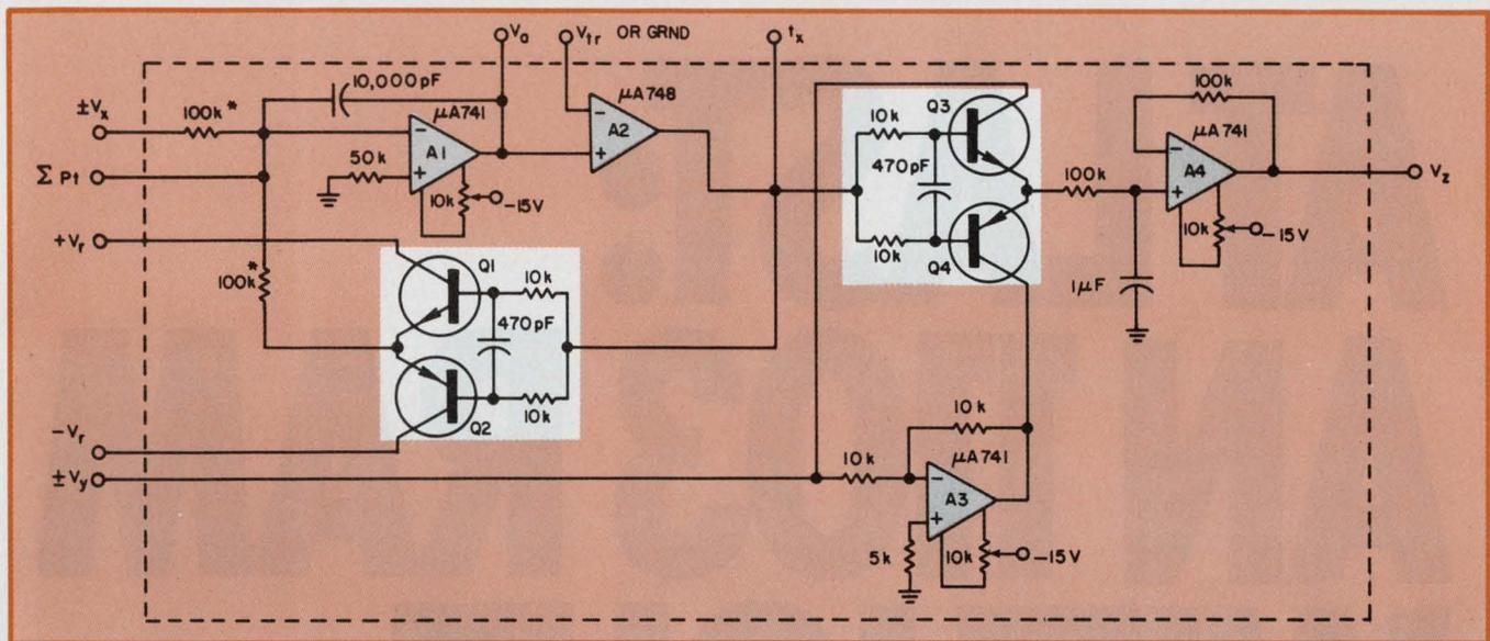
5. This precision four-quadrant multiplier/divider can be built discrete or hybrid (in a single flat pack). It requires
