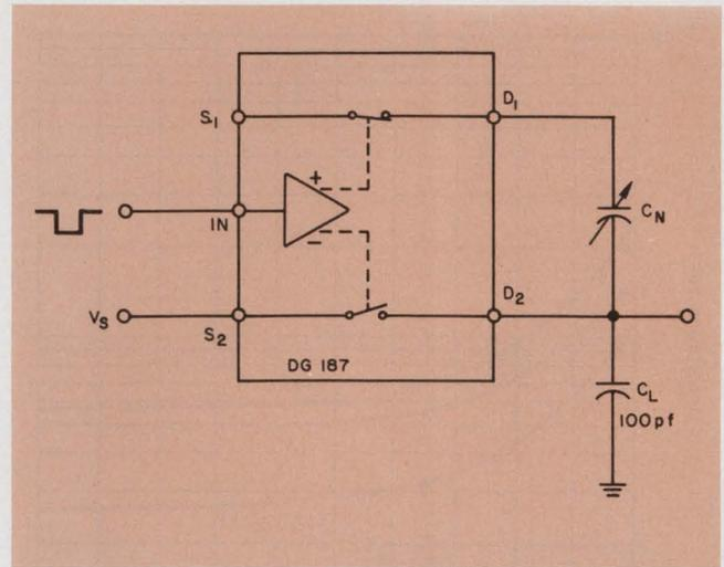
6. This basic neutralization circuit has the advantage of simplicity, but it offers complete neutralization at only one value of signal voltage.
