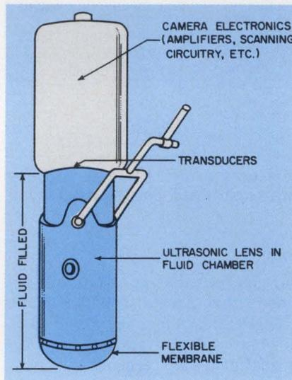
The lower half of this ultrasonic imaging camera is filled with fluid to transmit the high-frequency signals to a patient's body.
