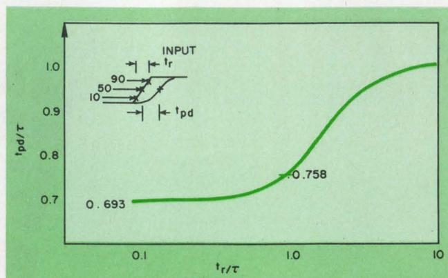
2. Propagation delay is minimum for a zero-rise-time (step) input pulse, and it approaches a maximum value of  $\tau$  for infinite rise time.
