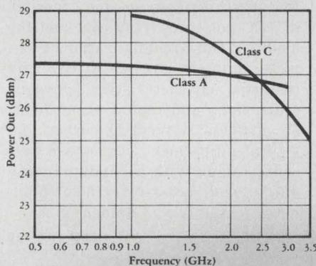
output or linear driver, it offers low distortion from 2 to 4 GHz. Yet it costs the same as the small signal HP 21.
