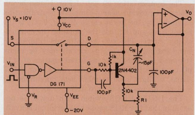
10. The single-switch PMOS DG171 is easily neutralized because the driver output is available at a terminal pin. A npn transistor provides charge transfer to the neutralizing capacitor  $C_N$ .
