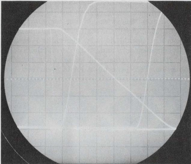
3. The  $t_{PLH}$  of a typical TTL gate increases from 10 ns to 20 ns as the input fall time increases. The dotted line in this double exposure is the 1.5-V reference level.
