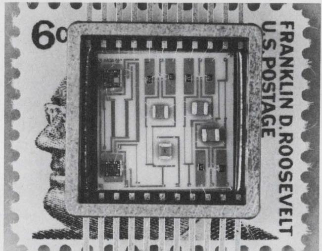
This dual multiplier/divider (5/8 by 5/8 flatpack) is used by General Electric's AICS department on several aerospace programs for precision analog computation.
