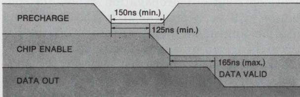
**No Precharge and Chip Enable overlap requirements.** The 3534 requires only that the Precharge pulse stays low for a minimum of 150ns and that at least 125ns delay occur from the start of Precharge to the start of Chip Enable. The Data Out is valid 165ns after the Chip Enable goes low but is independent of Precharge.
