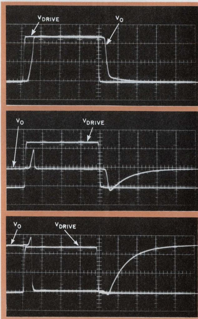
5. Transients in a typical fast JFET switch, the GD187. Here  $R_L = 10$  k $\Omega$ ,  $C_L = 30$  pF and the scales are 2 V/div and 500 ns/div. From top to bottom,  $V_A = +5.0$ , and  $-5$  V.
