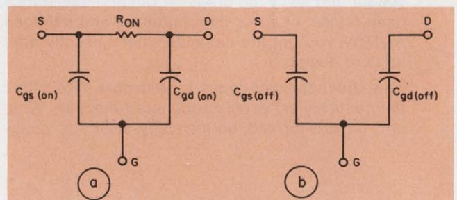
2. The ON (a) and OFF (b) equivalent circuits of a JFET are useful in the noise analysis.
