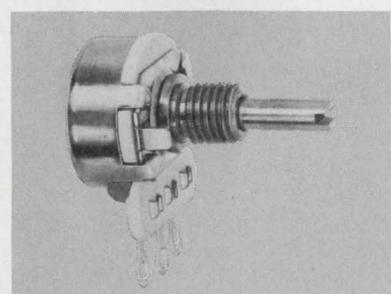
**New CTS series 205** 5/8" dia. Cer-mide® thick-film variable resistor. Excellent environmental char.; and immediate design versatility. 1 w power @ 70°C; 50Ω-5meg-Ω resistance; ±20% tol.; dust shield; many mounting styles and shaft types. Only 82¢ in quantity. Power switch available. CTS Keene, Inc., Paso Robles, Calif. 93446. (805) 238-0350.
