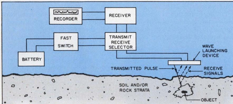
**Electromagnetic Subsurface Profiling system** uses a fast switch to produce nanosecond, time-limited pulses, which are transmitted and received by a specially designed antenna.
