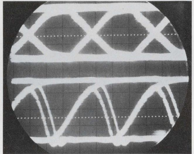
5. Eye patterns reveal the dynamic response of the logic. A random input waveform is at top and the response at bottom. The output lacks the clearly defined "eye" of the input. Clock rate is 50 Mb/s.
