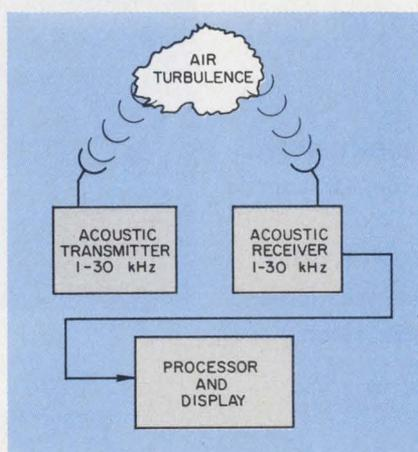
Acoustic radar for detecting aircraft wake turbulence.
