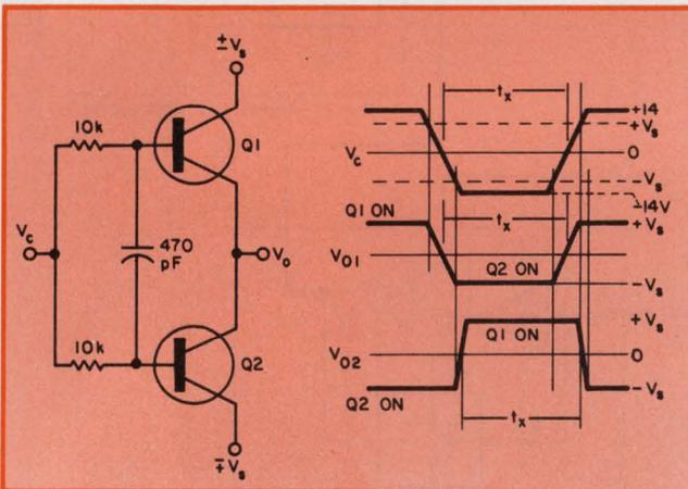
4. Bipolars switch accurately, in spite of their limitations. Output ( $V_o$ ) waveforms depend on the polarity of the voltage to be switched,  $V_s$ .  $V_{o1}$  is the output with  $+V_s$  on the collector Q1.  $V_{o2}$  is the output with  $+V_s$  on the collector of Q2.
