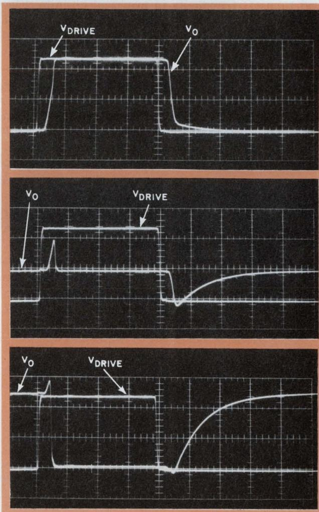
5. Transients in a typical fast JFET switch, the GD187. Here  $R_L = 10$  k $\Omega$ ,  $C_L = 30$  pF and the scales are 2 V/div and 500 ns/div. From top to bottom,  $V_A = +5.0$ , and  $-5$  V.
