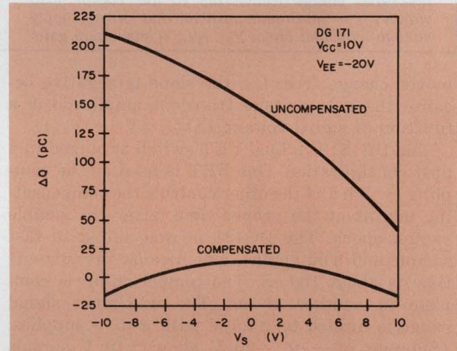
9. Compensation with the circuit in Fig. 10 reduces transferred-charge variation for PMOS FETs like the DG171, with ON resistances of 40 to 100  $\Omega$ . Variation in transferred charge is greater for the uncompensated DG171 than for the uncompensated DG181 (Fig. 8) and full compensation is not as complete.
