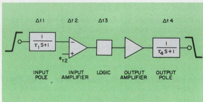
1. How circuit components contribute to propagation delay. The input-pole contribution depends on input-waveform transition times.
