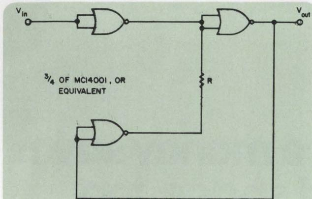
1. A low-cost, versatile Schmitt trigger requires only three logic-gate elements and one resistor.
