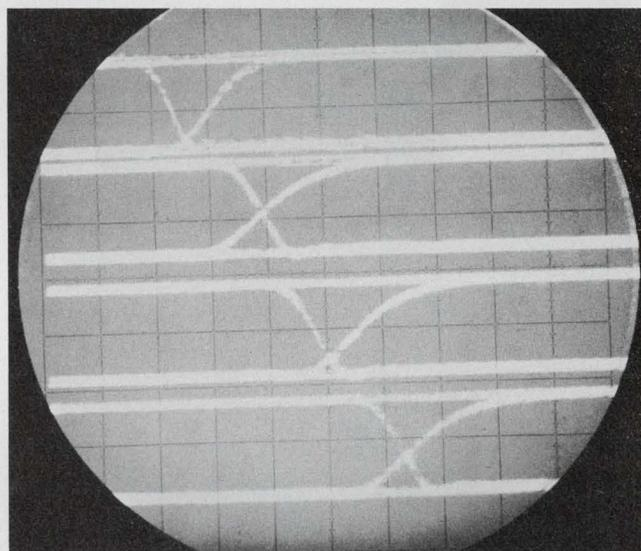
6. Stage-by-stage delays of a four-gate Nand circuit are checked with a pseudorandom generator. The "Xs" depict both positive and negative transition delays. Deflection factors are 10 ns/div. and 2 v/div.
