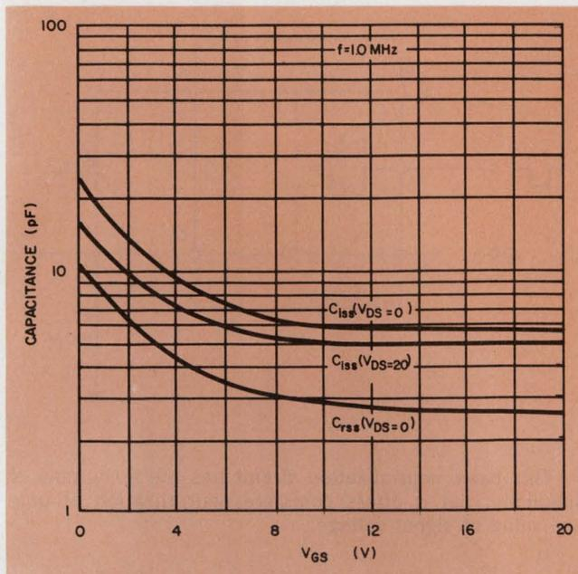
3. Capacitance vs gate-to-source voltage for 2N4091, 4391 and 4856 JFETs.  $C_{r_{ss}}$  is the gate-to-source capacitance;  $C_{i_{ss}}$  is the sum of gate-to-source and gate-to-drain capacitances.
