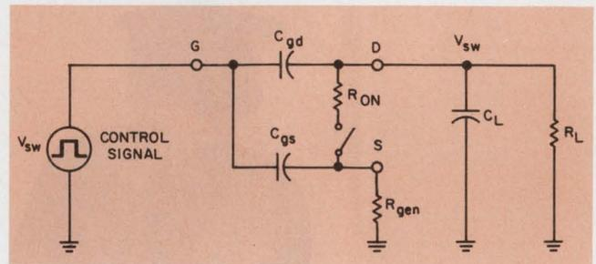
1. Gate-pulse edges form switching transients as they are coupled to the load through FET capacitances.
