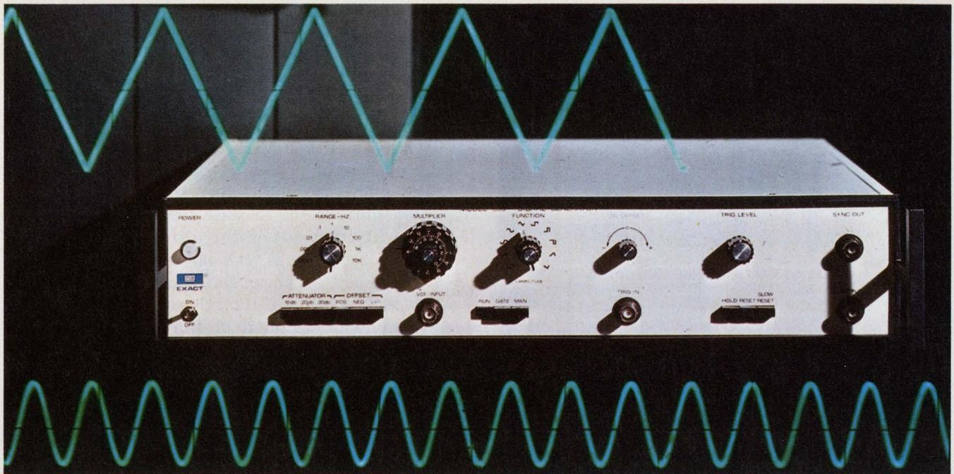
The basic triangle from which other waveforms are derived is synthesized from a 2000-bit staircase in Exact's \$1250 Model 335. Exceptional stability results over frequencies from an ultra-low 10  $\mu$ Hz to 50 kHz.
