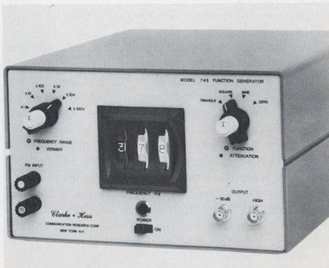
**Thumbwheel switches set frequency** to 3-digit resolution in the Clarke-Hess 745, a \$475 instrument for 10 mHz to 1.1 MHz. Frequency can be swept to twice the upper-dial frequency.
