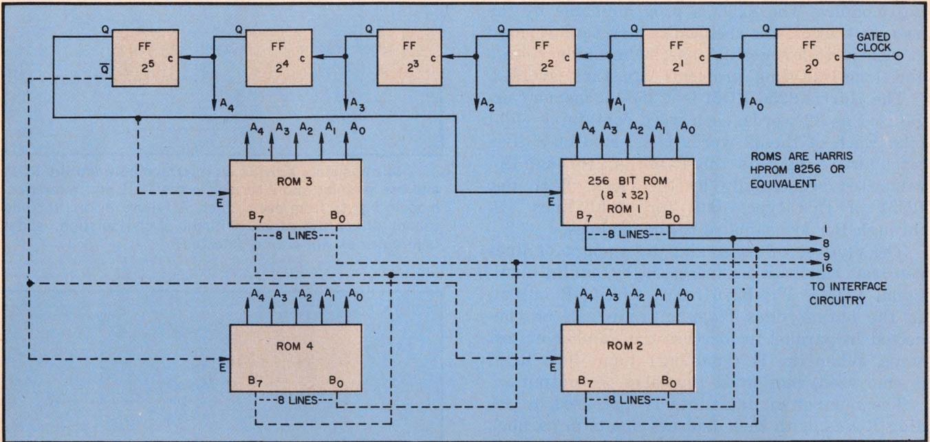
2. **More ROMs increase test capacity.** Also shown is a flip-flop address counter, stepped by clock pulses, which
