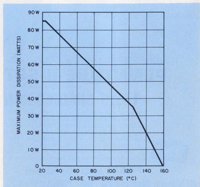
2. The maximum allowable power dissipation of the hybrid regulator goes down as a case temperature goes up, but the case can be cooled to boost dissipation.
