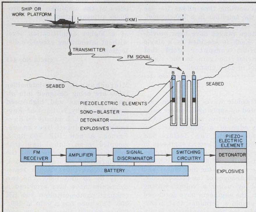
Transmitter suspended beneath surface ship sends FM signal to sono-blast unit A. The explosion activates piezoelectric elements in sono-blasters units B, causing each in turn to explode.
