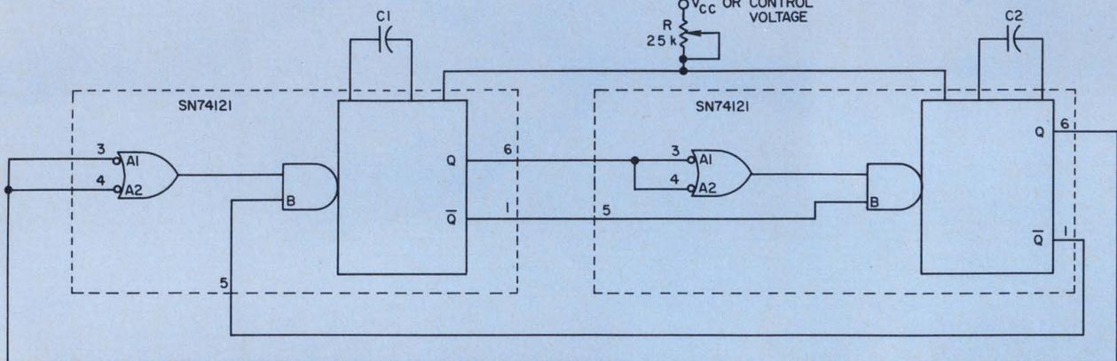
Multivibrator and truth table for logic inputs, where  $t_n$  is the time before and  $t_{n+1}$  the time after
