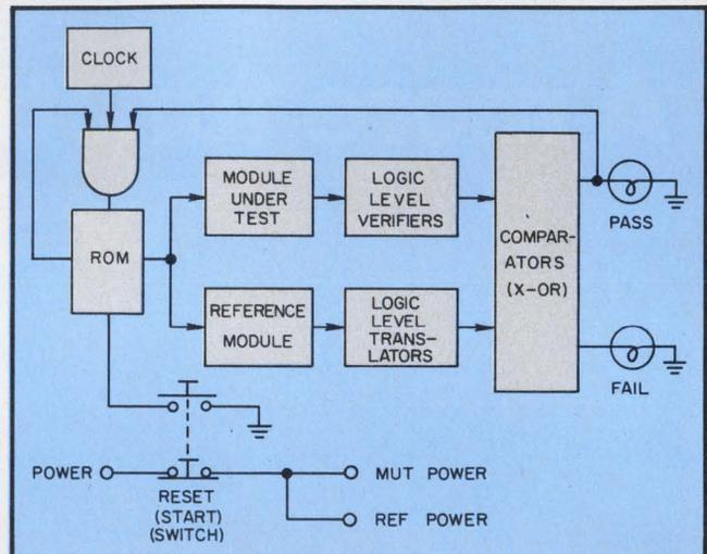
1. The essential elements of a semi-automatic module tester. The test sequence is initiated by closing the reset (or start) switch, enabling the ROM and also applying power simultaneously to the module under test (MUT) and the reference module, so they start in the same initial states.
