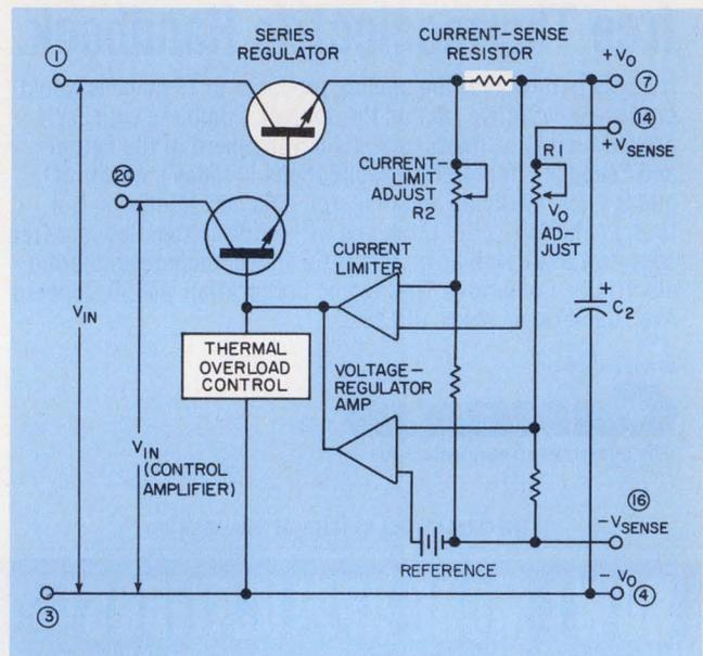
1. The basic hybrid regulator, designed for raw-dc input, has a power section (in white) and a control section. Circled numbers are package pin numbers.
