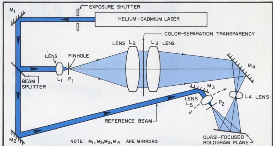
Three color-separation transparencies are recorded with this system as three overlaid holograms on a common photoresist area. Each hologram is made with the reference beam positioned at a different angle.
