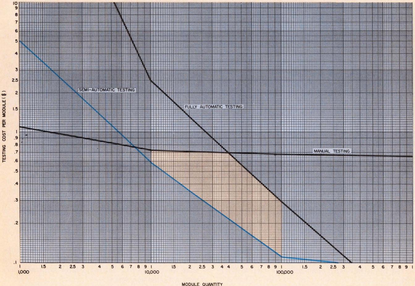
Unit test cost varies with digital-module quantity for the three approaches shown: manual, semi-automatic and
