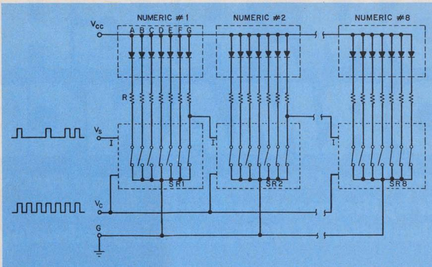
External connections are reduced by connecting the shift registers so that the last parallel output of one becomes the input for the next. The eight registers operate as a single 56-bit register.
