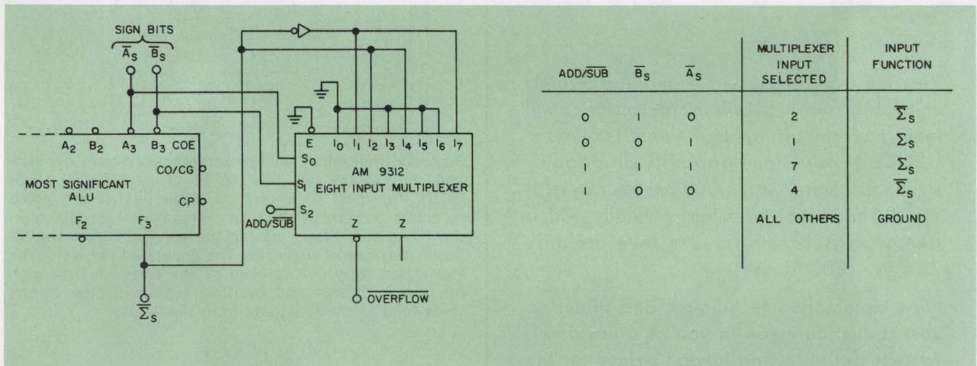
2. An eight-input multiplexer allows detection of overflow conditions in a binary adder. The delay is equivalent to
