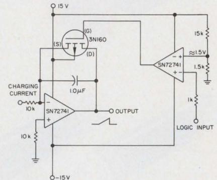
2. Alternate circuit, with another SN72741 op amp used as a differential comparator.
