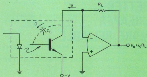
2. Capacitive feedback can be eliminated by removing the collector voltage swing with an op amp. The response is then determined by the op amp.
