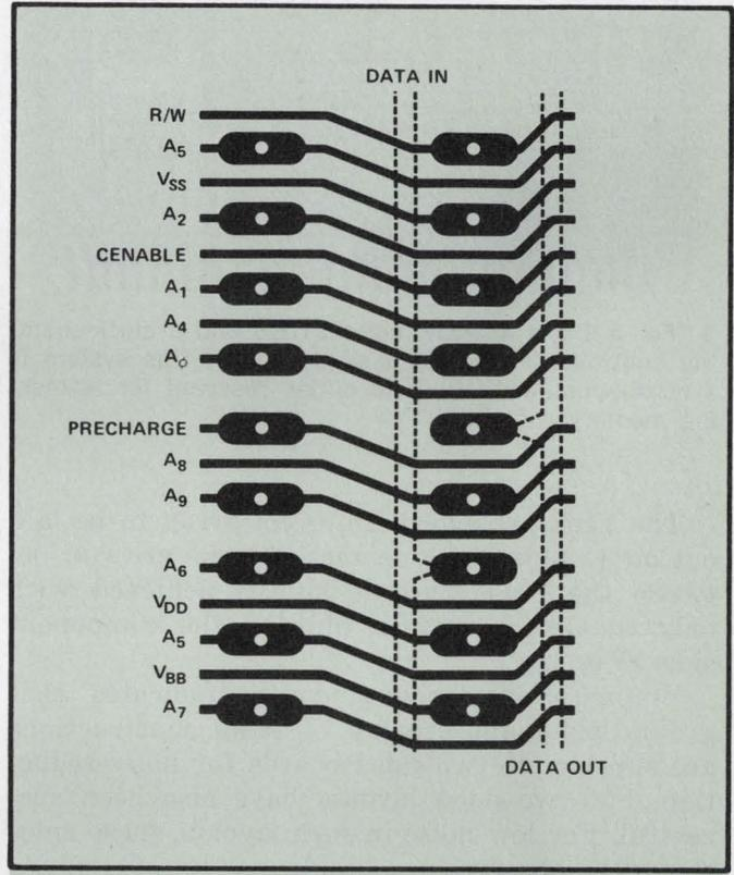
2. An array of 1103s can be laid out on 1/2-by-1-inch centers. Leads are routed between pins on the component side. On the opposite side, data-in and data-out busses interconnect the packages.
