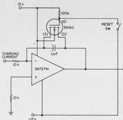
1. Corrected drawing, with reset switch tied to gate of MOSFET.
