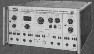
An important feature of our totally new line of 200 and 400 line Analyzers/Integrators is a digital bin marker which provides accurate read-out of amplitude and frequency information.
