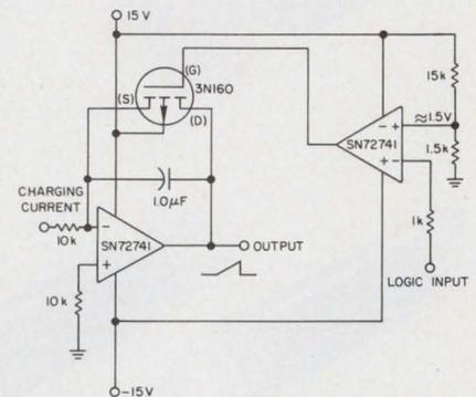
2. Alternate circuit, with another SN2741 op amp used as a differential comparator.
