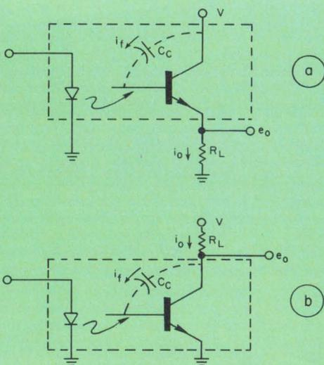
1. Internal capacitive feedback in phototransistors is shown for emitter-follower (a) and common-emitter (b) configurations.
