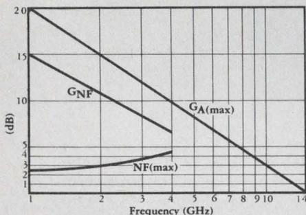
guaranteed noise figure of 4.5 dB at 4 GHz with 6.5 dB gain when biased for optimum NF (10 V, 5 mA). With 3 dB more gain across the band than the HP 21, the HP 22 is useable to 8 GHz
