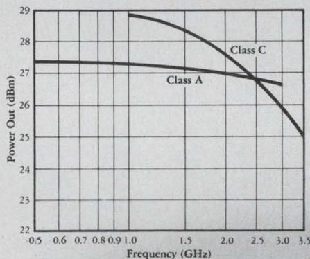
output or linear driver, it offers low distortion from 2 to 4 GHz. Yet it costs the same as the small signal HP 21.
