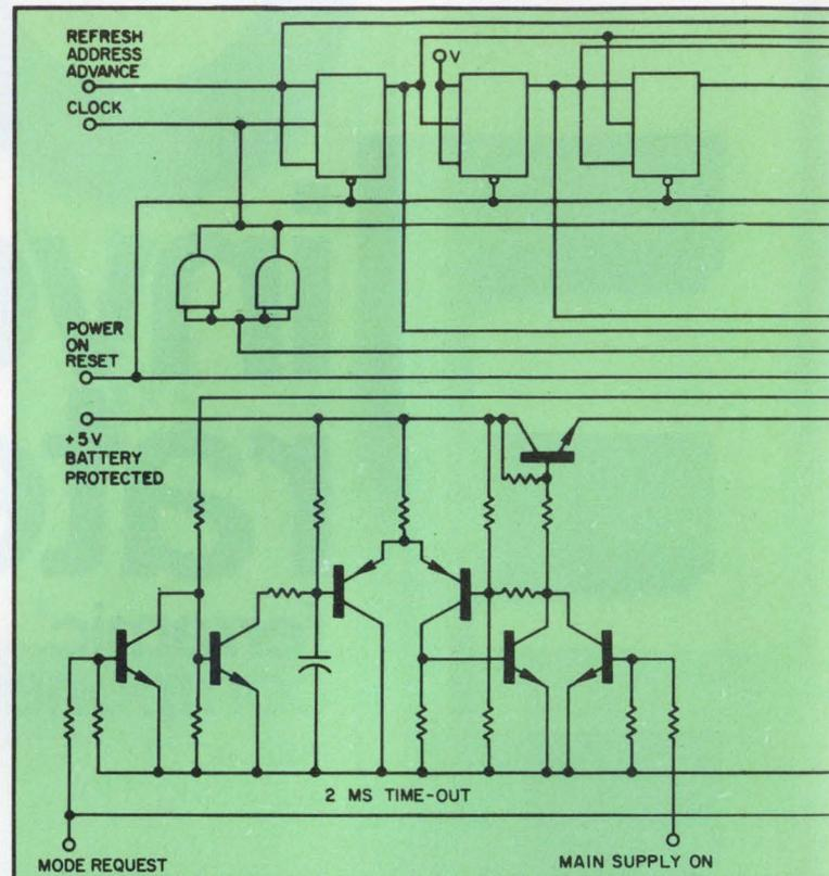
1. Low-Power Data Retention control circuit provides two modes of operation. In normal operation, one refresh cycle is executed every 60  $\mu$ s. In the data retention only mode, a burst of 32 consecutive
