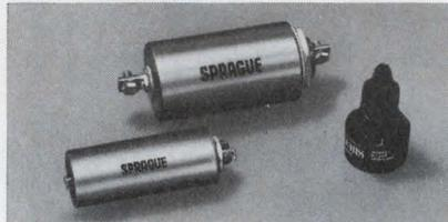
**U.L. LISTED FILTERS.** Series JX5000 for EDP equipment and general-purpose use. Rated 125/250 VAC, 0-60 Hz, 1 thru 50 amps. 60 db @ 150 kHz, 80 db from .5 MHz thru 1 GHz. Special designs and rectangular multi-circuit units also available. Write for Engineering Bulletin 8210 or; **CIRCLE 886 ON READER SERVICE CARD.**
