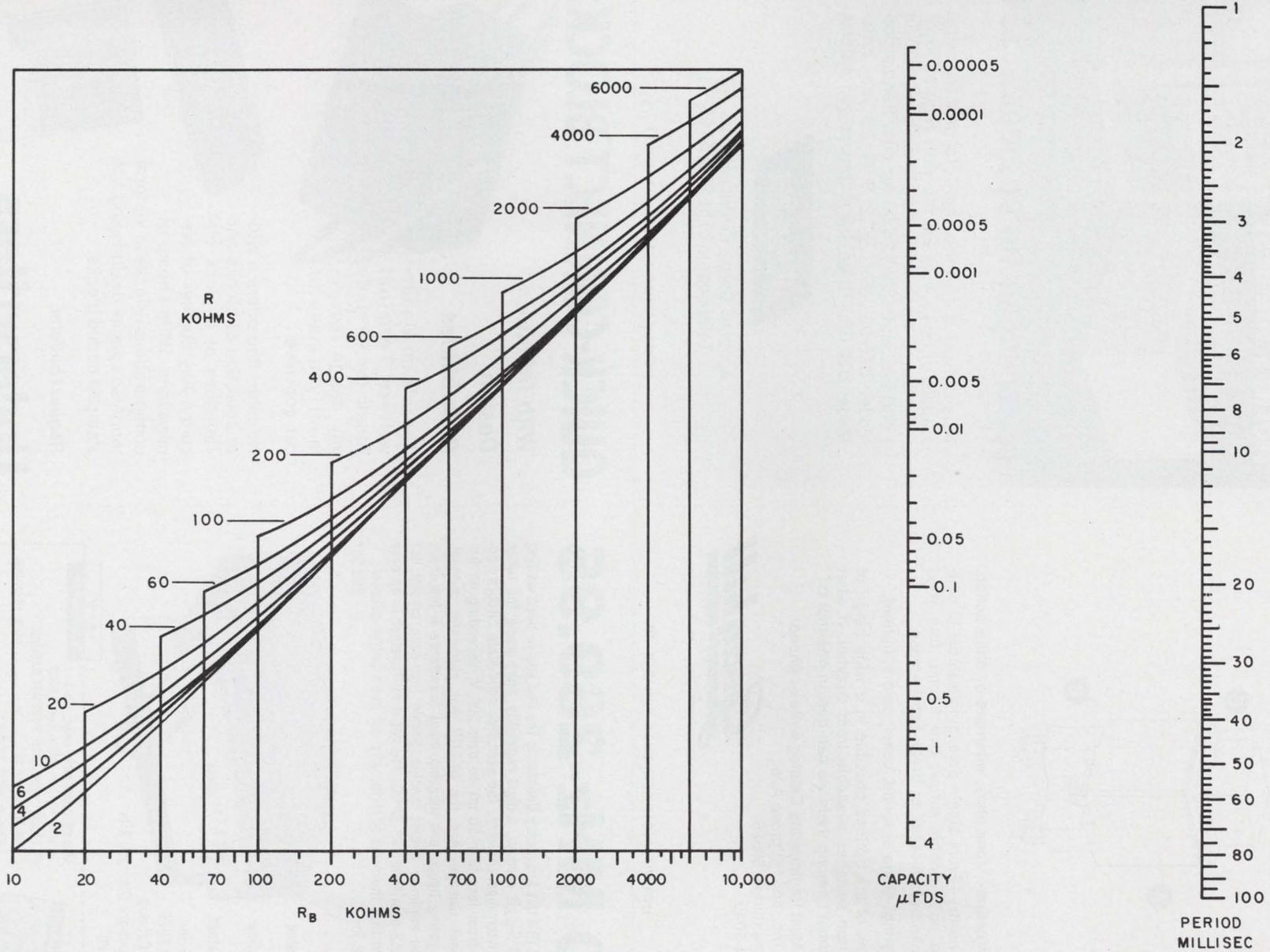
2. **Oscillation period is determined as a function of circuit variables.** From  $R_B$  at the bottom of the graph, proceed straight up the curve representing  $R$ . At the  $R$
