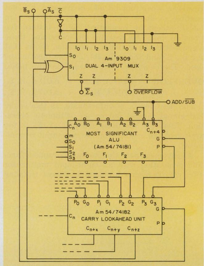
3. A dual four-input multiplexer produces both overflow and sign signals for this 16-bit arithmetic logic unit (ALU). The most significant bit of the ALU is connected to create a permanent "carry propagate" condition in the F3 position, thus making the carry-out from the F2 position available externally. The generated output of the look-ahead carry unit is used as the carry into the sign bit, and both sign and overflow signals appear at the same time as the F outputs from the ALUs.
