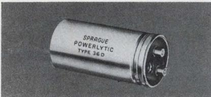
**TYPE 36D POWERLYTIC® CAPACITORS.** For use in computer power supplies, control equipment, energy storage, etc. Low impedance construction. Up to 650,000  $\mu$ F at 3 V. Ratings from 3 to 450 V. Can be operated at 85°C. Tapped 10-32 terminals simplify filter bank assembly. Write for Engineering Bulletin 3431D or; **CIRCLE 887 ON READER SERVICE CARD.**
