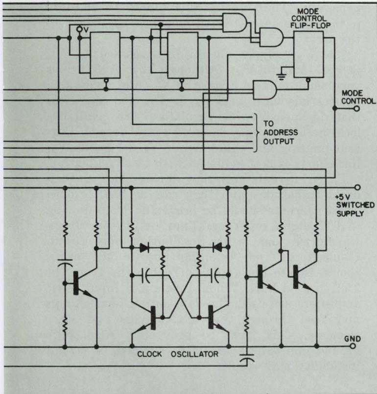
refresh cycles is executed every 2 ms. In this latter mode, power to the TTL controller logic is switched off between bursts, adding to the savings in power consumption.
