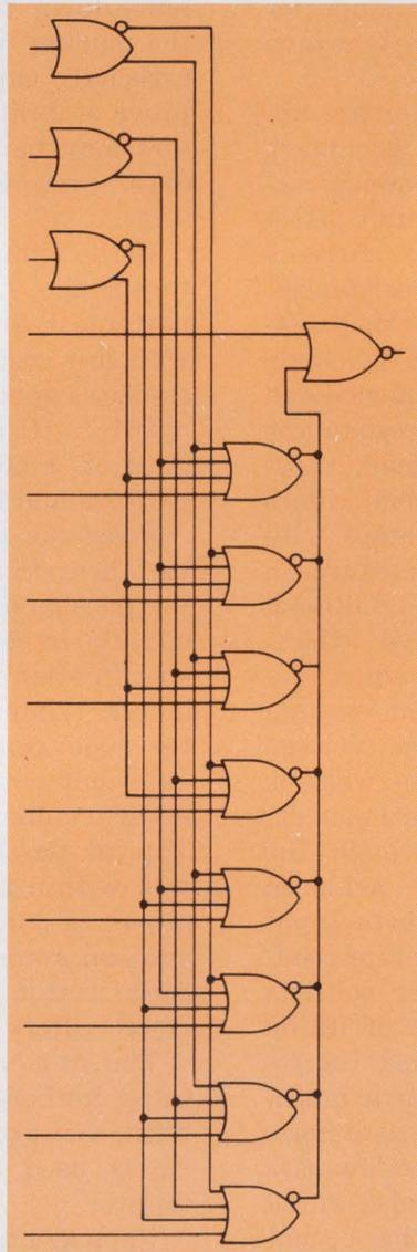
**MC10164 8-Line Multiplexer** — For use wherever data multiplexing or parallel to serial conversion is desirable. Full parallel gating permits equal delays through any data path. The output incorporates a buffer gate with eight data inputs and an enable. A high level on the enable forces the output low. The MC10164 can be connected directly to a data bus due to its open emitter output and output enable.
