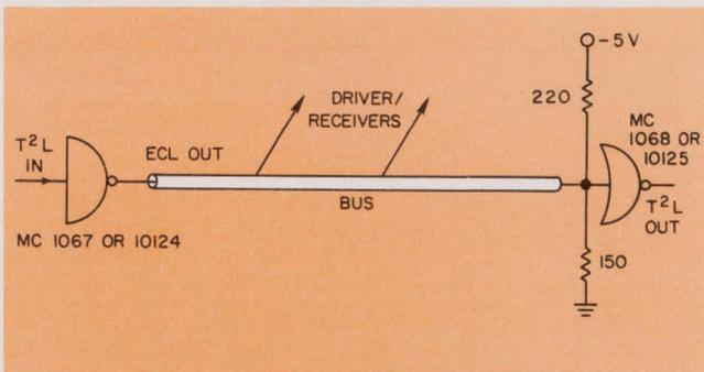
4. For very high-speed operation, drivers with emitter-follower outputs are used together with receivers that have transistor-base inputs. The emitter followers can supply large currents, while the base inputs require very little current. The  $F_{ct}$  is about 16%.
