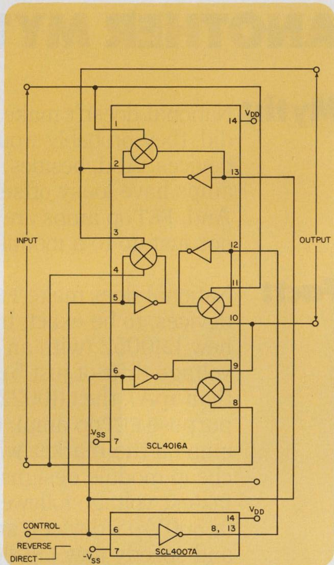
An SCL4016A quad bilateral switch reverses the polarity of analog signal inputs, with an SCL4007A acting as a control-signal inverter.
