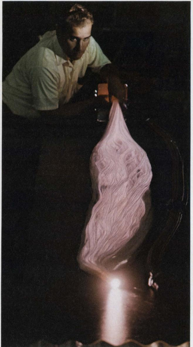
The image scope, above, by Bendix Electro Optics has its protective housing removed to demonstrate the path of the light rays in the bundle.
