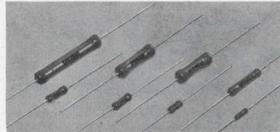
**BLUE JACKET® RESISTORS.** Vitreous-enamel power wirewound. Unique all-welded end-cap construction eliminates moisture paths along leads, anchors leads securely to resistor body. Expansion coefficients of vitreous enamel, ceramic body, and end caps are closely matched. Write for Engineering Bulletin 7410E or;
