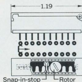
Siemens is introducing a completely new kind of programming switch for closely racked PC boards and for other tight-space applications.
