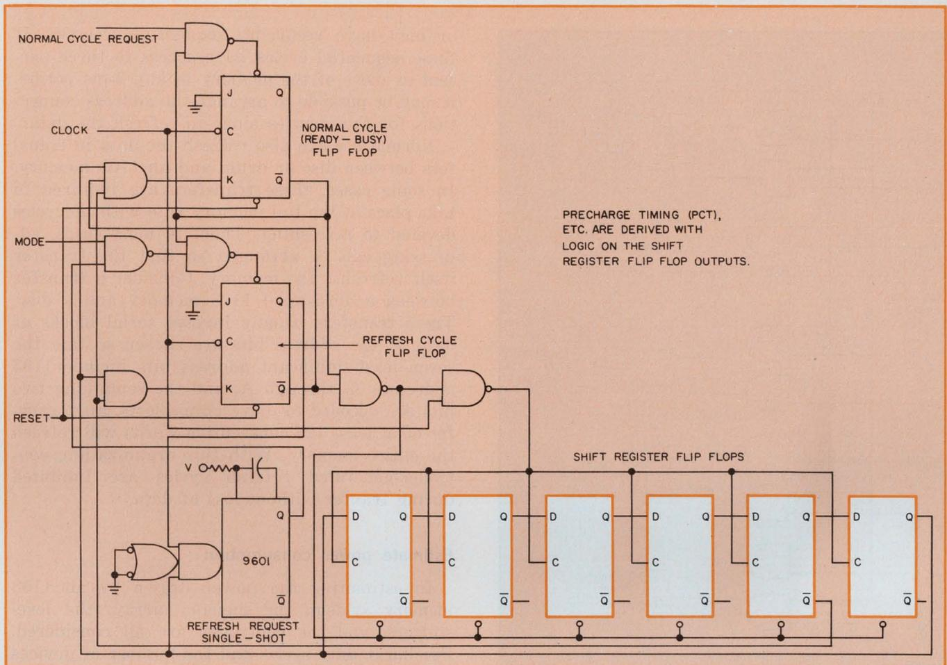
5. Controller uses a shift register instead of delay lines to generate timing signals, but access time is increased by the interval from cycle request to the next clock
