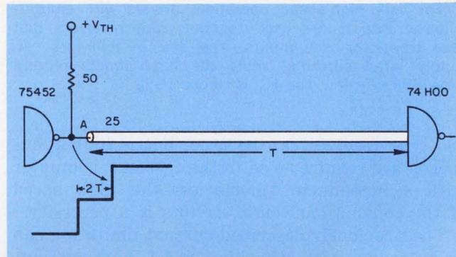
2. **Medium-speed bus circuits** use open-collector T<sup>2</sup>L logic, so several circuits can be tied together by the bus. Furthermore a collector pull-up resistor is used to terminate the bus line. The figure of merit for this circuit is 28%. This system is most used in minicomputer-based configurations.
