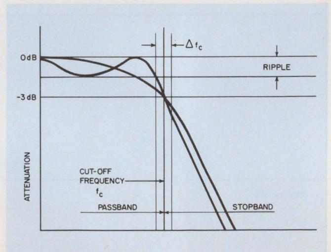
2. **Network-related characteristics** provide the theoretical basis for a filter design. But component tolerances, temperature effects and physical limitations restrict the filters that can be realized.
