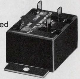
**JDB Series** is a Dual Thin-Line reed-triggered triac for use on printed circuit boards. Designed for interfacing solid state circuits to 120 V 60 Hz loads such as contactors, fractional HP motors and solenoids. Form A contacts will switch 1.7 amps. at 25° C ambient or 1.0 A rms 60 Hz at 55° C ambient.
