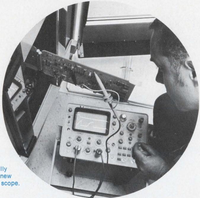
Servicing computers and peripherals can be less costly, especially if you use HP's new 1707A portable scope.
