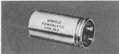
**TYPE 36D POWERLYTIC® CAPACITORS.** For use in computer power supplies, control equipment, energy storage, etc. Low impedance construction. Up to 650,000  $\mu$ F at 3 V. Ratings from 3 to 450 V. Can be operated at 85 C. Tapped 10-32 terminals simplify filter bank assembly. Write for Engineering Bulletin 3431D or;
