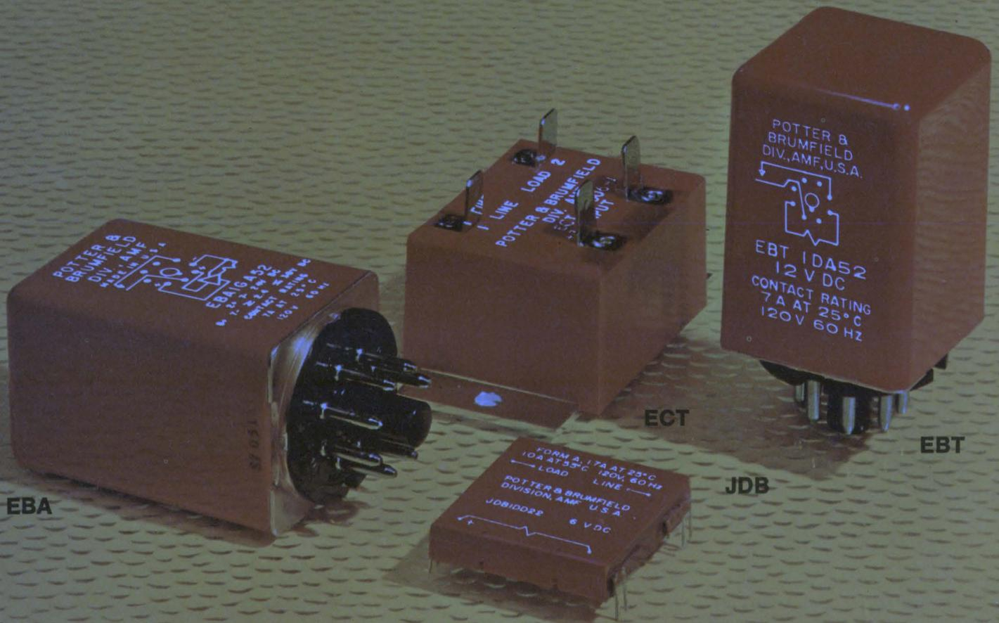
The expected minimum life of P&B Solid State Hybrid Relays is in excess of 10 million operations for standard load current and ambient temperature combinations.
