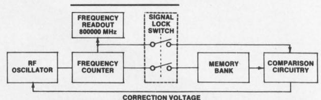
"Signallock" is a patented circuit which enables the output of the built-in rf oscillator to be locked into the crystal time base of the built-in counter. When the Signallock mode is switched in, the digital readout is stored in a memory, and then continuously compared to the generator's output frequency. If an error exists between the output frequency and the memory frequency, a correction voltage is fed back to the oscillator, causing frequency to return to the original setting.
