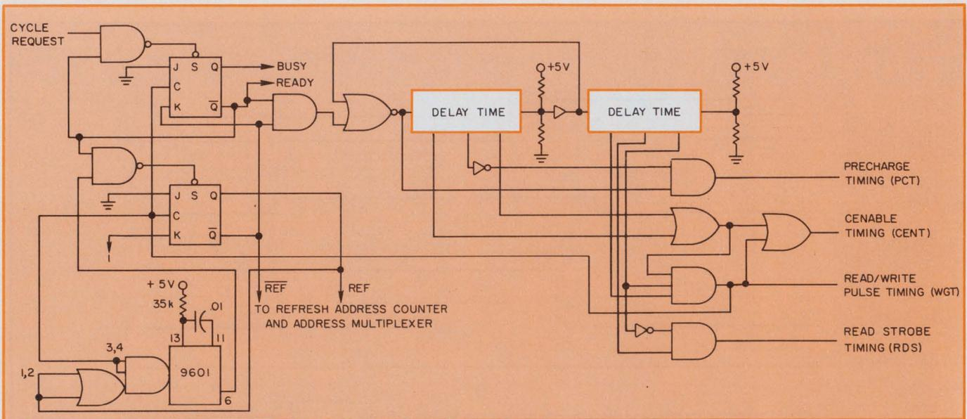
3. Controller uses delay lines to produce cycle timing signals. A refresh cycle generated by a single-shot multivibrator is requested every 60  $\mu$ s. The timing of
