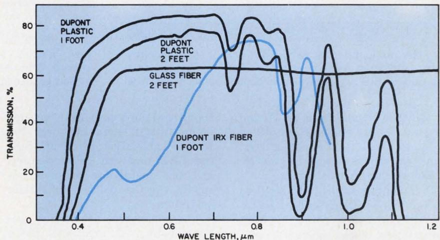
2. Plastic fibers have higher transmission than glass in the visible range. But attenuation in the plastic increases sharply in the near infrared. A new plastic duPont IRX fiber is improved at  $9 \mu\text{m}$ .
