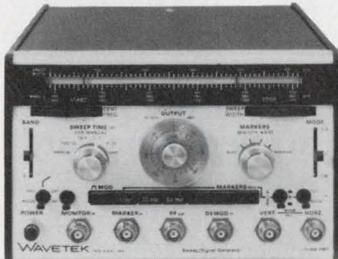
Solid-state, varactor-tuned and swept oscillator permits zero to full-band sweep width and FM modulation.
