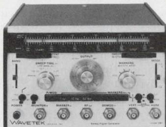
Programmability and/or remote control of frequency, bandwidth and output level.
