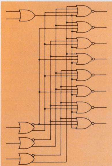
**MC10162 Binary To One-Of-Eight Decoder** — Decodes a three bit input word to a one-of-eight output. A high level on either enable forces the outputs low. Features true parallel operation; ie, propagation delay from every input to any given output is the same, eliminating unequal delay times found in other decoders. Allows easy expansion of memories or other computer addressable functions, and can be used as a data distributor.
