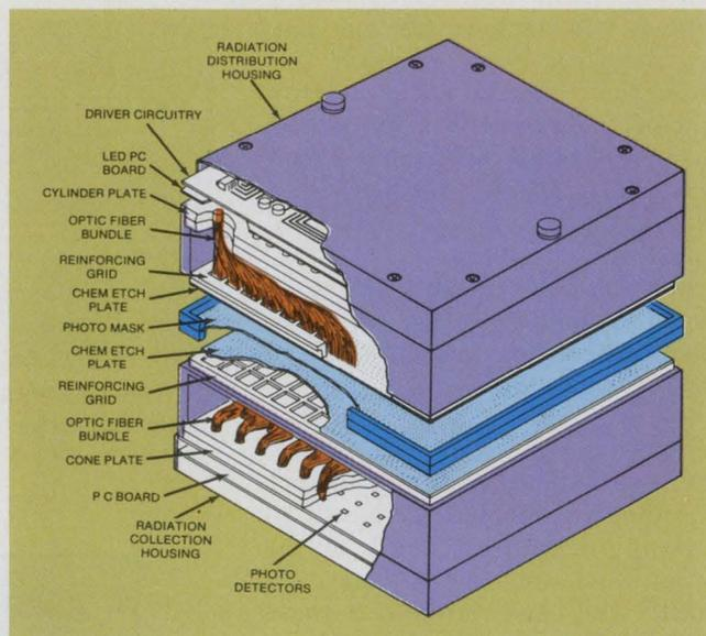
fiber bundles, left, are potted in position over photosensors. The basic mask area is about 5 x 5 inches with a storage density of about 4000 bits per square inch.
