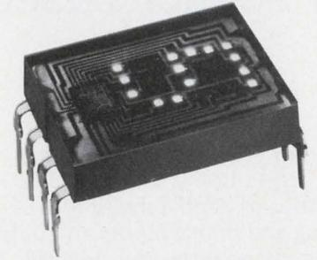
*The 5082-7300 numeric display is completely TTL-compatible.*
