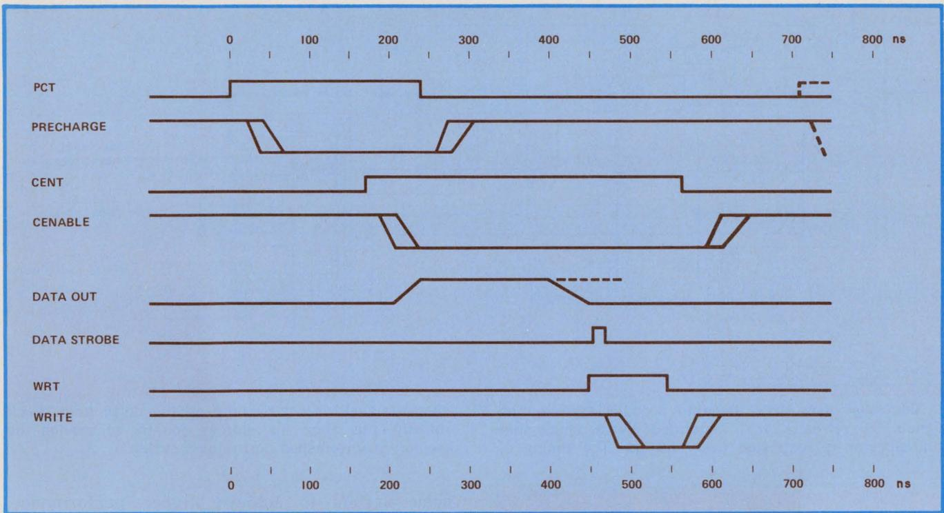
2. **Gates and drivers in the timing path** introduce delays and add to rise time. They also make relative timing of signal transitions more critical and increase access
