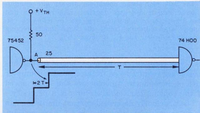
3. **The degree of mismatch** between the line and the terminating resistance depends on the noise immunity of the bus circuits. Gate switching time is delayed by the line in each direction. The height of the pedestal, for a  $V_{TH} = 3.5$  V, is equal to  $3.5(25/75) = 1.2$  V. The  $f_{ct}$  is about 12%.
