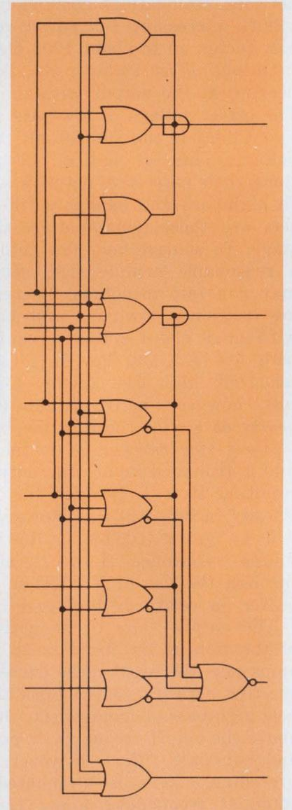
**MC10179 Lock-Ahead Carry Block** — A powerful MSI function consisting of 10 low power gates internally connected for the look-ahead carry function. Recommended for use with the MC10181 4-Bit ALU, or the MC10180 Dual Arithmetic Unit, to accomplish high speed arithmetic operations on long words. Highly useful for reducing system package count for the function generation of several variables.
