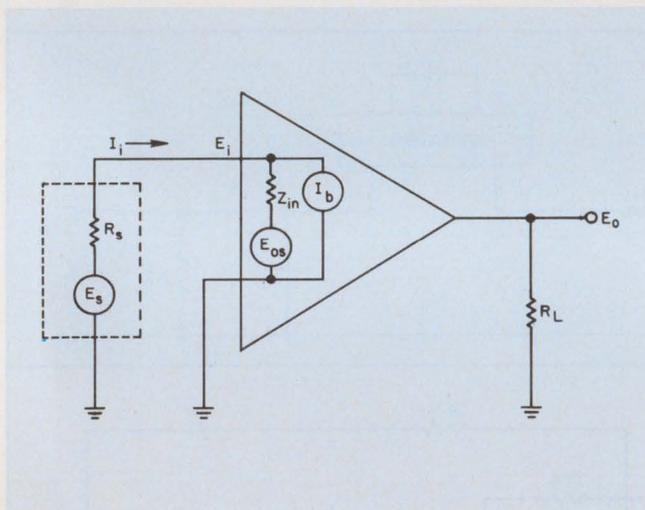
1. **Amplifier-related characteristics** pose special problems to the filter designer. The value of  $Z_{in}$ , for example, may not be the in-circuit value, since the impedance is often used to adjust frequency characteristics.
