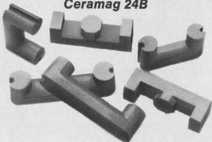
Tektronix, Inc. selected 24B for their "U" and "E" cores. This proven material has seen years of service in flybacks for television. Ideal for power applications, it can be operated at higher frequencies than laminated steel. It is cool running, due to low losses under power conditions and controlled power permeability. Tooling is available for a wide range of "U", "E" and "I" configurations.
