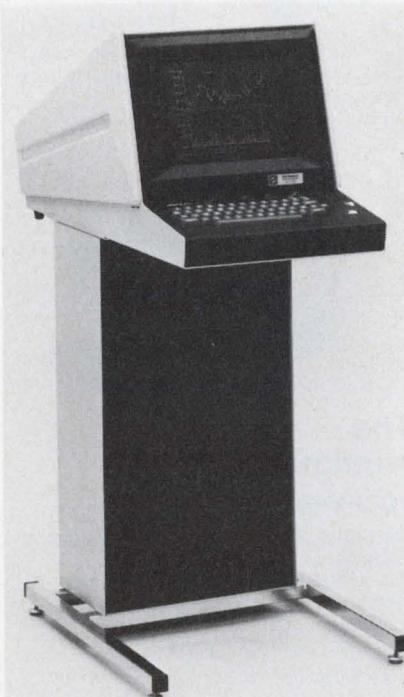
**A new low-cost CRT terminal with both graphics and alphanumeric capabilities comes in a pedestal configuration. Its top display section can be detached for desktop viewing.**
