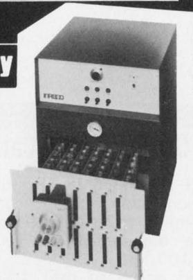
The INRECO static handling system is a must for testing I.C.'s, diodes, transistors, resistors, etc. Devices are clipped to special test P.C. cards which are inserted into inner door mounted connectors. With the door in place and the required temperature in the chamber, all the devices may be powered and/or sensed individually by the scanner plugged into connectors on the door exterior.
