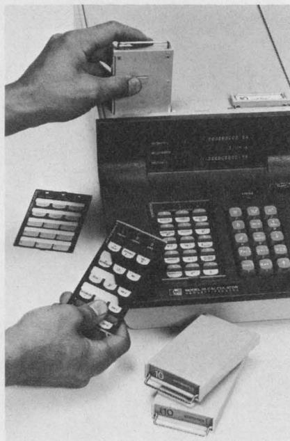
function blocks include separate (ROM) memories so they *do not* draw on the main calculator memory, leaving it fully available for further problem-solving power. A third keyboard plug-in option, the *User Definable Function* block, allows you to customize individual keys for operations uniquely important to you and your discipline.
