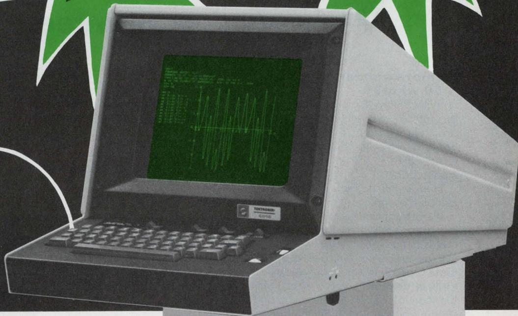
**NEW 4010**—The new Tektronix 4010 Terminal is an engineering and business oriented computer display terminal with interactive graphing and alphanumeric capabilities. It is hardware and software operational with a host of popular mini-computers, with IBM 360/370 systems and presently with over 20 timesharing systems.
