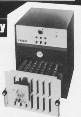
The INRECO static handling system is a must for testing I.C.'s, diodes, transistors, resistors, etc. Devices are clipped to special test P.C. cards which are inserted into inner door mounted connectors. With the door in place and the required temperature in the chamber, all the devices may be powered and/or sensed individually by the scanner plugged into connectors on the door exterior.
