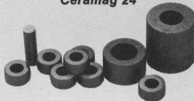
Toroids of Ceramag 24 were used by Tektronix, Inc. for transformer cores. Again, this is a proven material, widely used by the computer industry for pulse transformer cores. It has a tightly controlled initial permeability, and tooling for a variety of sizes is also available.
