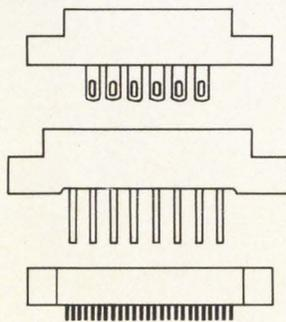
**EB 7** New .156" model with reliable bifurcated bellows contacts. Single row (6, 10, 15, 18, 22 contacts). Double row (12, 20, 30, 36, 44 contacts). Solder eye terminals. For 1/16" board.
