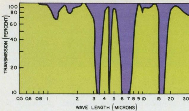
3. Transmission losses are strongly frequency-dependent, as shown by the nominal atmospheric transmission characteristics. Emitter characteristics should always be matched to the transmission media.
