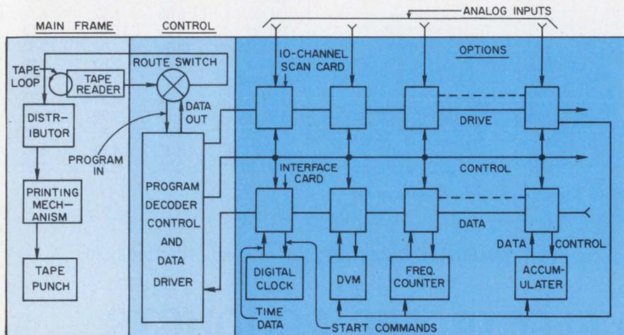
The 7100 data logger processes 100 analog inputs with optional 10-channel cards. Other options include a clock, DVM, counter and accumulator.
