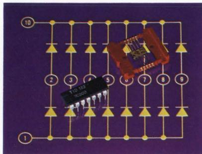
Reliability is outstanding because these coredrivers are manufactured like ICs. Thus, there are a reduced number of connections and glass-to-metal seals, better uniformity of device parameters, smaller size and less weight, no pressure contacts, no whiskers and no crossed bonding wires.
