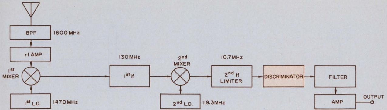
1. Conventional L-band receiver uses a phase-shift discriminator. Amplitude stabilization is performed by the
