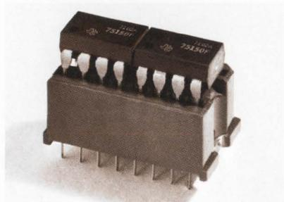
Anything more severe than an instantaneous short circuit knocks out most MODEM line drivers. But not TI's SN75150 dual line driver—it meets EIA RS-232C specifications to the letter, not just to the "intent." The SN75150 outputs are capable of enduring sustained shorts to ground or any voltage up to 25 volts in magnitude. Inputs are TTL/DTL compatible for ease in interfacing to logic systems.
