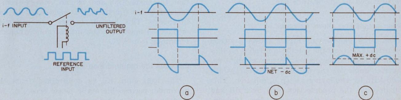
3. The phase detector can be thought of as a switch that is opened and closed by the square-wave reference signal. For the waveforms shown, the reference and intermediate frequencies are equal and the loop is locked. When the signals are out of phase by 90° (a), a zero
