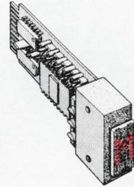
For that man/machine interface where ease of recognition and high reliability is a must - the **Monsanto MDA111 Alpha-numeric** is a natural. This module display contains all circuitry needed for immediate readout in all 64 ASCII characters. Just supply a six-bit binary word and +5 volts/-12 volts to the input terminals and you're in business.
