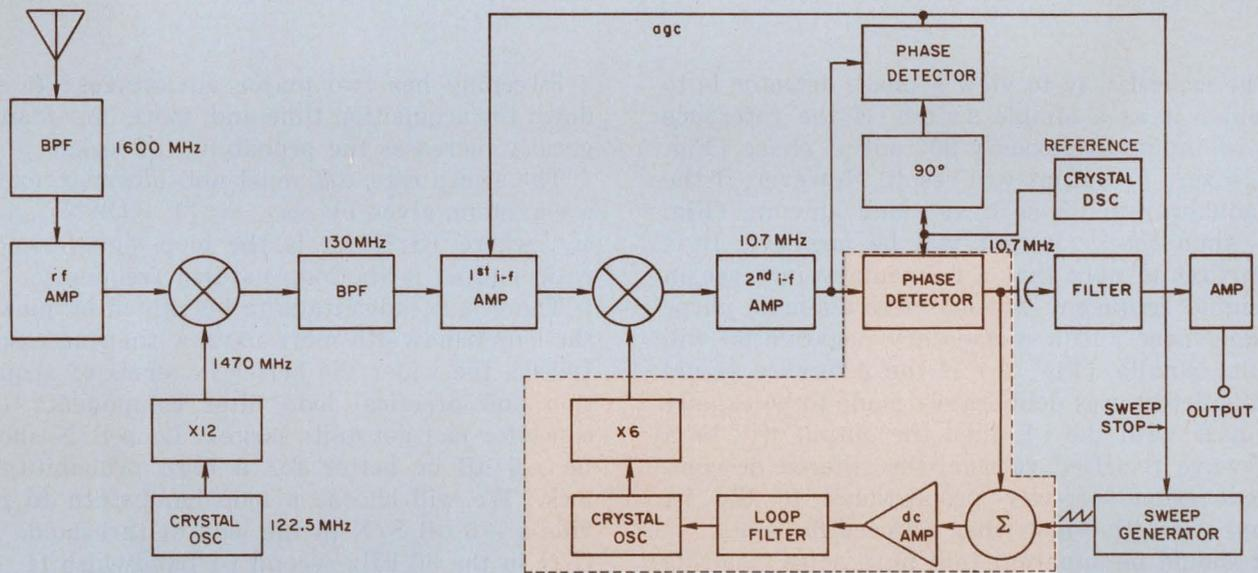
2. This phase-locked satellite receiver uses quadrature agc. The agc signal not only controls the gain of the first
