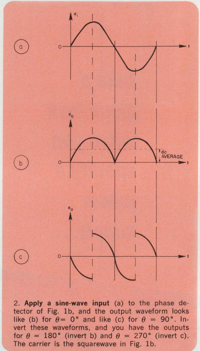
2. Apply a sine-wave input (a) to the phase detector of Fig. 1b, and the output waveform looks like (b) for  $\theta = 0^\circ$  and like (c) for  $\theta = 90^\circ$ . Invert these waveforms, and you have the outputs for  $\theta = 180^\circ$  (invert b) and  $\theta = 270^\circ$  (invert c). The carrier is the squarewave in Fig. 1b.
