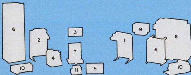
**A wide variety of peripherals are available** for minicomputers including: (1) standard and (2) heavy-duty teleprinters; (3) high-speed paper tape reader and punch; (4) punched-card reader; (5) mini and (6) standard magnetic disc memory; (8) high-speed line printer; (9) CRT display; (10) plotters; (11) modem for communicating with other computers. Many special peripherals are available for test and control applications.
