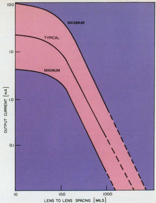
4. The separation of source and sensor is the main factor affecting transmission in many applications. The effect of lens-to-lens spacing is shown for a TIL24/LS600 coupled pair.
