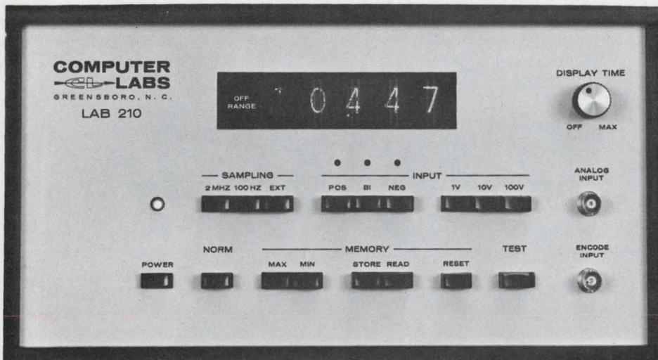
**Measure pulse heights with a DVM instead of a scope?** Now you can with the new LAB 210 TRANSVERTER. It's a 10-bit A/D (encoding rates to 2 MHz) with a Nixie tube display showing four significant digits,  $\pm$  sign, and over-range indication. That's 10 times scope accuracy . . . and a lot more readability!
