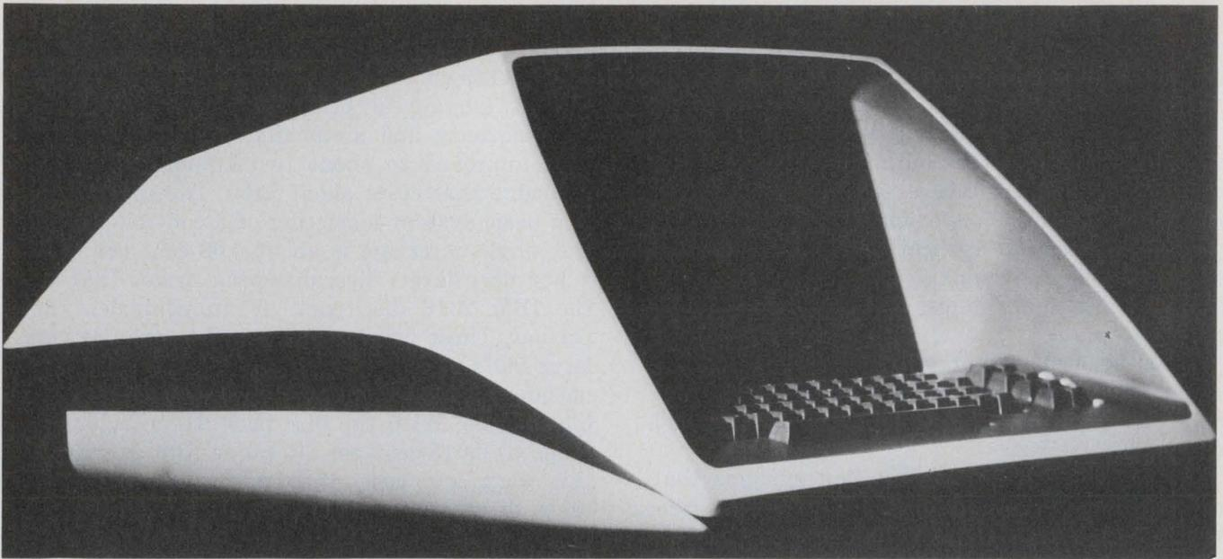
**Low-cost CRT/keyboard terminals have begun to compete** with teleprinters in applications where the output is not retained. This Digital Equipment Corp. DECterminal I
