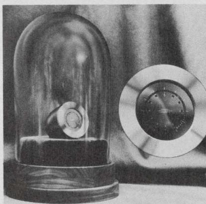
**Light-emitting diode clock** has a face made of 72 diodes, arranged in two concentric circles. Two small batteries can operate the clock for at least a year, with the clock face displaying the time continuously.
