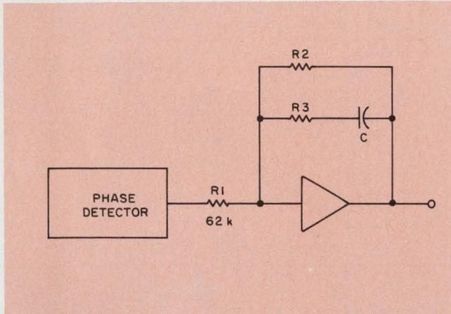
9. This active filter configuration combines the dc gain and lead-lag characteristics needed by the phase-locked loop. Time constant  $\tau_1 = R_2C$ , and  $\tau_2 = R_3C$ . The amplifier can be a standard IC operational amplifier.
