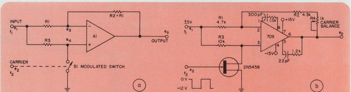
1. You can build a phase-detector/modulator (a) with only an op amp, a carrier-modulated switch and a resistor network. For a phase detector, the input signal and the carrier have equal frequencies.
