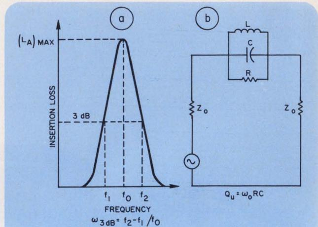
1. The characteristic curve of a doubly loaded bandstop filter (a) defines peak attenuation,  $(L_A)_{\max}$ , and fractional 3-dB bandwidth,  $\omega_{3dB}$ . The filter's equivalent circuit is shown in b.
