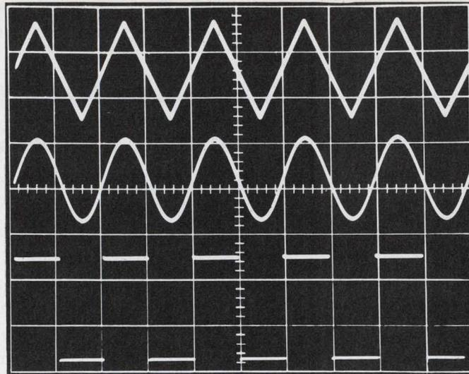
actual unretouched photograph of triangle, sine and square waves generated by the Heath EU-81A and displayed on the Heath EU-70A dual trace scope. Frequency 1 kHz.
