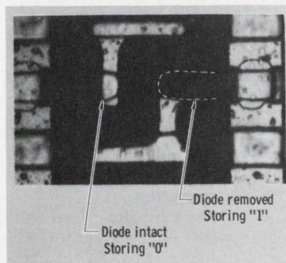
Silicon-on-sapphire ROM chip (left) contains an array of 40 by 128 diodes for a density of 3300 bits. Results are depicted of the ROM's custom encoding by a laser tool (right). Left arrow shows an intact diode, for memory state ZERO, while arrow on right shows the diode removed by the laser, for memory state ONE.
