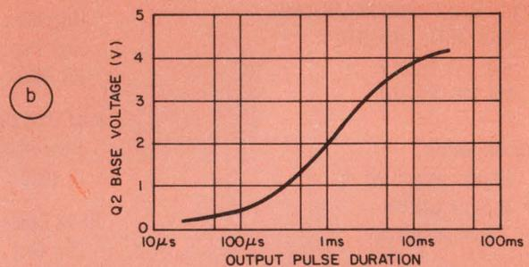
This dual-output monostable (a) permits direct control over pulse duration by changing the setting of potentiometer  $R_3$ . Both capacitor ( $C_1$ ) charging rate and comparator ( $A_1$ ) threshold level are used to vary output pulse width. The curve (b) shows the control range of 1600:1.
