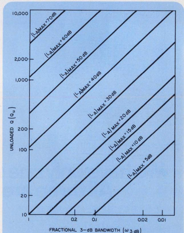
2. A log-log plot of unloaded Q vs fractional bandwidth almost reduces bandstop-filter design to the reading of this graph. Once the band limits are set and the peak attenuation and resonant frequency are selected, the filter's unloaded Q can be found with a straight edge.
