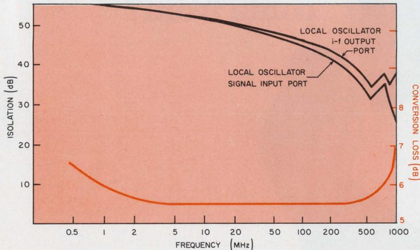
A new 0.5-to-1000-MHz double balanced mixer, costing as low as \$29.95, exhibits high-performance characteristics. Its conversion loss (bottom curve) is mostly flat at about 5.5 dB throughout most of its frequency range. The top curve shows the mixer's isolation.
