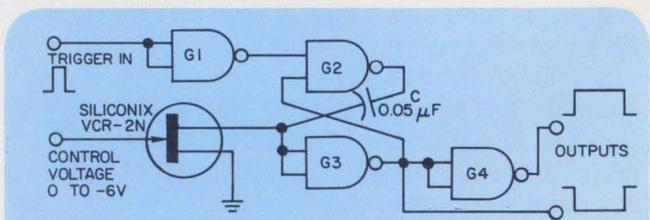
Output pulse duration can be varied from 1.2 to 120  $\mu$ s with this voltage-controlled one-shot. Although the delay is not linear with control voltage, duty cycles of up to 80% can be achieved.
