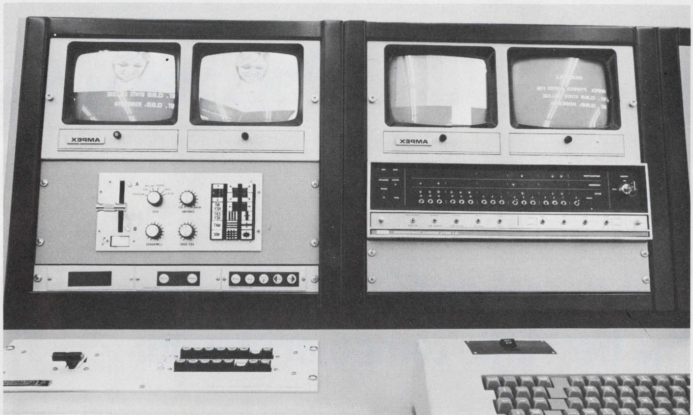
The heart of the Ampex PYRAMID educational system is the NOVA minicomputer. The system, a set of modular subsystems which function as peripherals, allows each student to start, stop, replay, hold, or discontinue his
