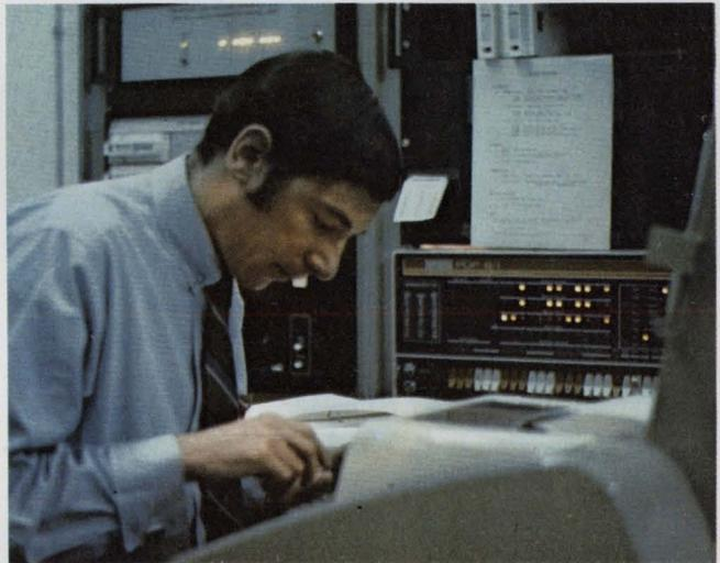
**A minicomputer directs tests, classifies devices and logs data** in the sophisticated J283 IC test system made by Teradyne of Boston. Here Norman Turner, software development engineer, works on a new job program which fixes pin and source assignments, source values and reject criteria.
