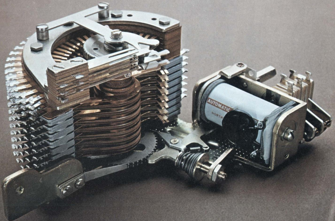
Our Type 45 rotary stepping switch is made to be forgotten. We build them to work hard, fast and long without constant fiddling or adjusting. They've got to be able to work in heat or cold, take bumps and grinds and still click-click along with close-spaced consecutive operations.
