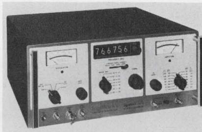
Continuously tunable over the frequency range of 50 kHz to 80 MHz in seven bands, a new rf signal generator uses a patented digital frequency lock circuit known as "Signalok" to achieve ultra-high stabilities of  $\pm 10$  Hz.
