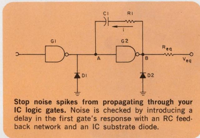
Stop noise spikes from propagating through your IC logic gates. Noise is checked by introducing a delay in the first gate's response with an RC feedback network and an IC substrate diode.
