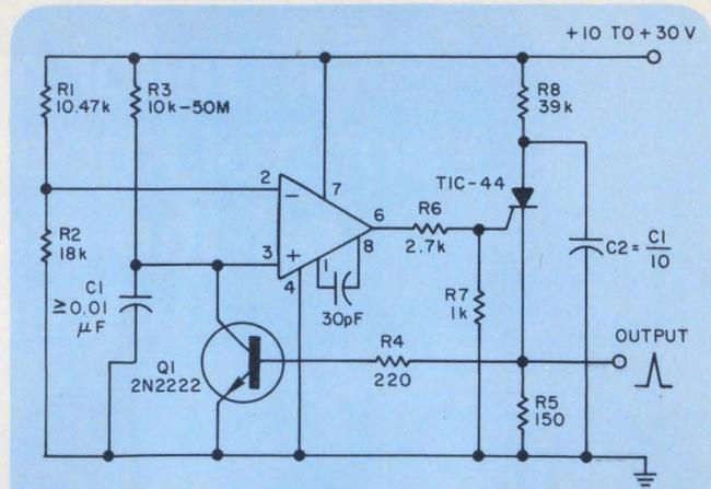
Vary the timing cycle of this pulse generator from 1 ms to 1000 s by simply tweaking some of the passive-component values. High accuracy and temperature stability are main features.
