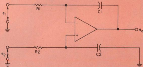
Equal time constants,  $R_1C_1 = R_2C_2$ , permit differential integration with a single amplifier. The circuit output is the true integral of the input difference voltage. Capacitor  $C_2$  replaces an op amp.
