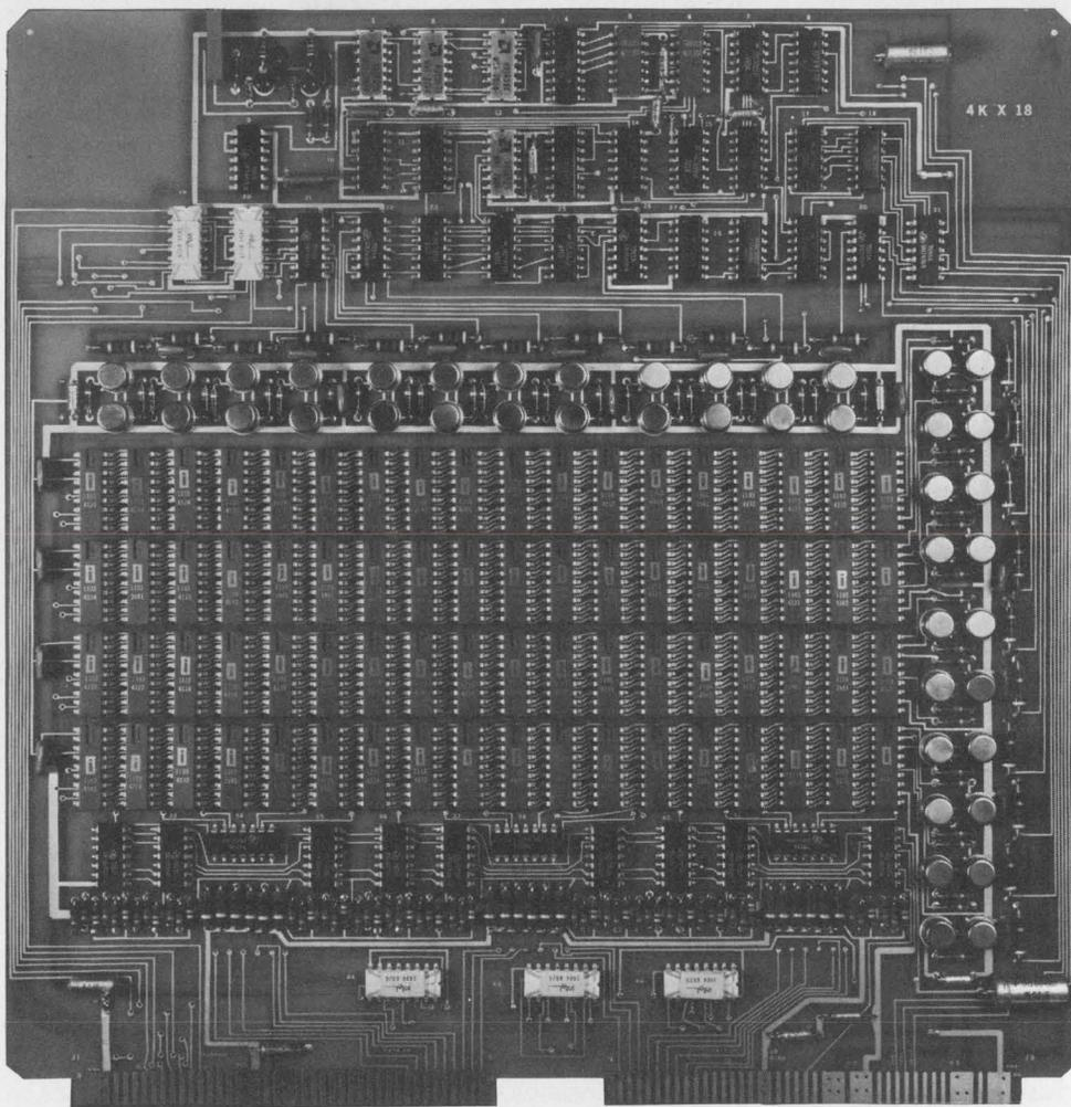
At left is a REAL 72,000-bit semiconductor memory built with Intel 1103's, the 1024-bit silicon-gate MOS RAM that's winning the price performance competition in main frame memories.
