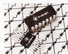
Ten new monolithic diode matrices—programmable by selectively opening the fusible link in series with each diode—offer up to 48 diodes in flat pack or C-DIP. The ten come in two series: TIDM1 (10 nsec) and TIDM2 (25 nsec).
