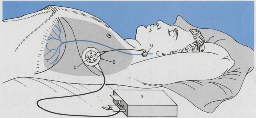
**Electrophrenic respiration equipment** includes a battery-run transmitter (A) which transmits signals through the antenna (B) to an implanted receiver (C) connected by subcutaneous wires to implanted electrodes (D) surrounding the phrenic nerve.
