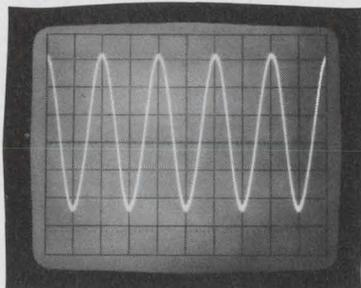
Conventional scope display of 5 MHz signal appears undistorted →
