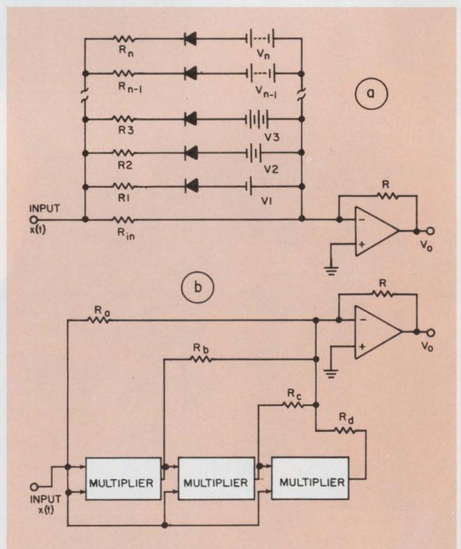
1. Don't use dozens of biased diodes (a) to generate arbitrary functions; multipliers are simpler to apply (b), and they give more accurate results.
