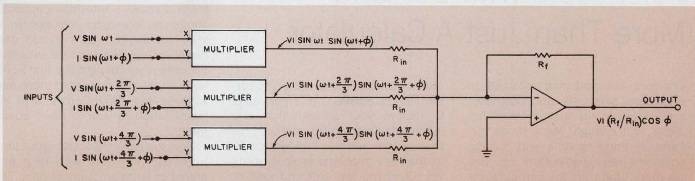
3. No filters are used in this power-measuring circuit, yet it provides a ripple-free dc output proportional to the
