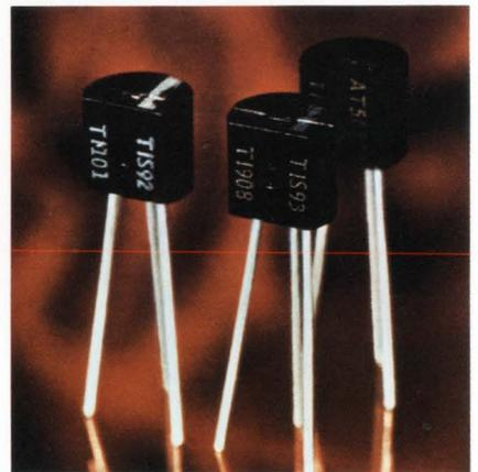
And these transistors have been approved in practically all known sockets requiring power dissipation greater than 400 mW.
