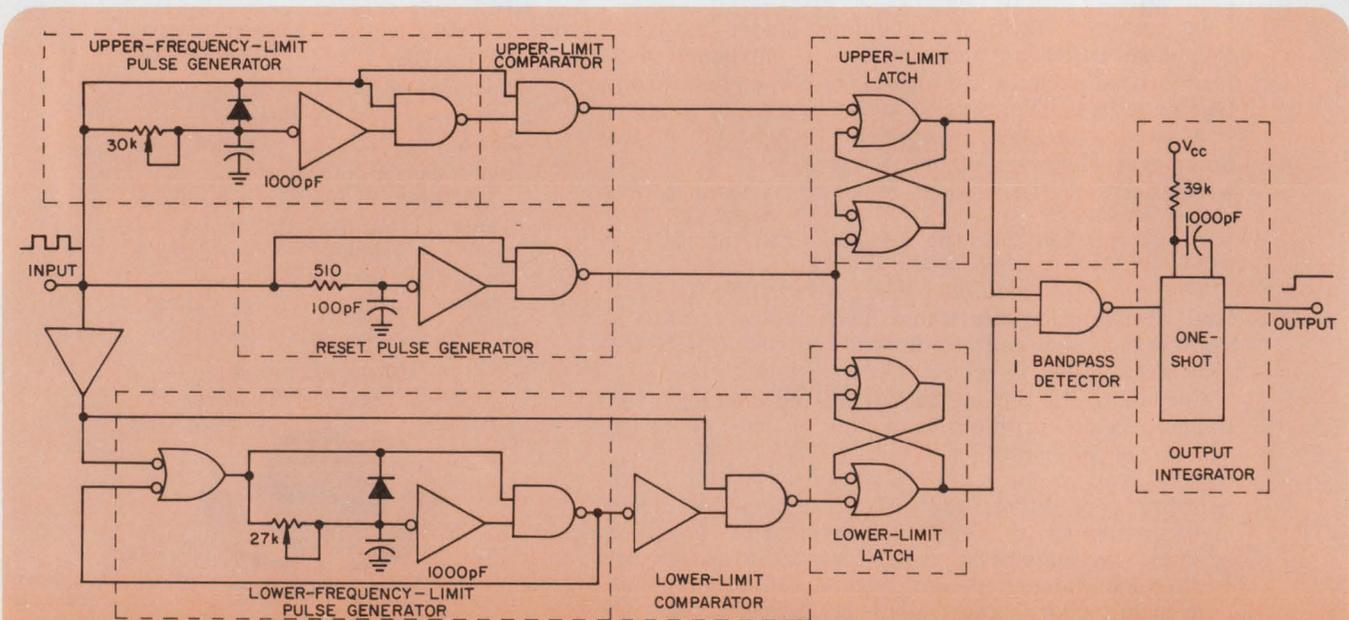
The output of this tone detector is a sharp, narrow, square pulse that is produced when the input frequency is within the preset passband. The upper and lower limits are individually tunable; thus both
