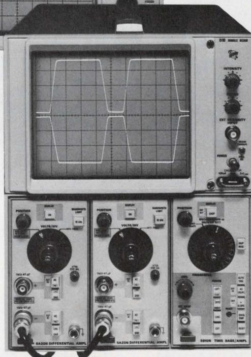
The low-priced 5103N Oscilloscope System offers cost-saving innovations never before available in any oscilloscope. Today, this series consists of six vertical amplifiers, three time bases and a three-plug-in mainframe compatible with four interchangeable display modules. Bandwidth is DC-to-2 MHz, depending upon the amplifier plug-ins.
