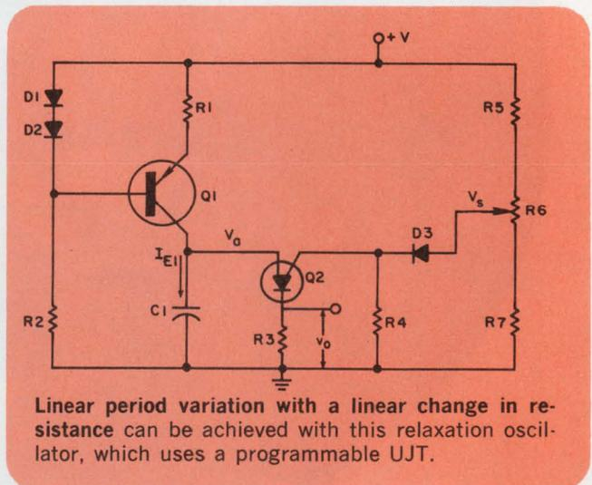
Linear period variation with a linear change in resistance can be achieved with this relaxation oscillator, which uses a programmable UJT.
