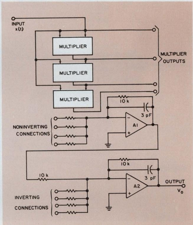
2. Polynomials with both positive and negative coefficients can be generated by this circuit because of its extra op amp. Just connect the multiplier output to one of the summing resistors on  $A_1$  for a positive coefficient, or to  $A_2$  for a negative coefficient.
