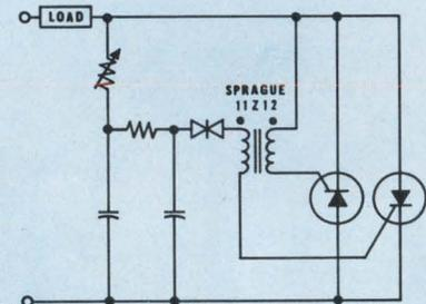
This breakdown-diode/transformer triggering circuit is a typical application for Type 11Z12 Trigate Pulse Transformers.
