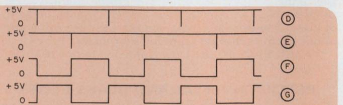
pulses and square waves that are capable of directly driving logic circuits.
