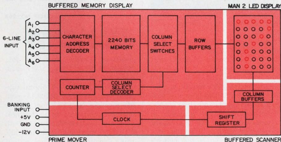
The MDA111 LED display package has four sections: a buffered memory display with a six-line input, a clock with a blanking input and power supply voltage lines and a MAN-2 35-dot LED display.
