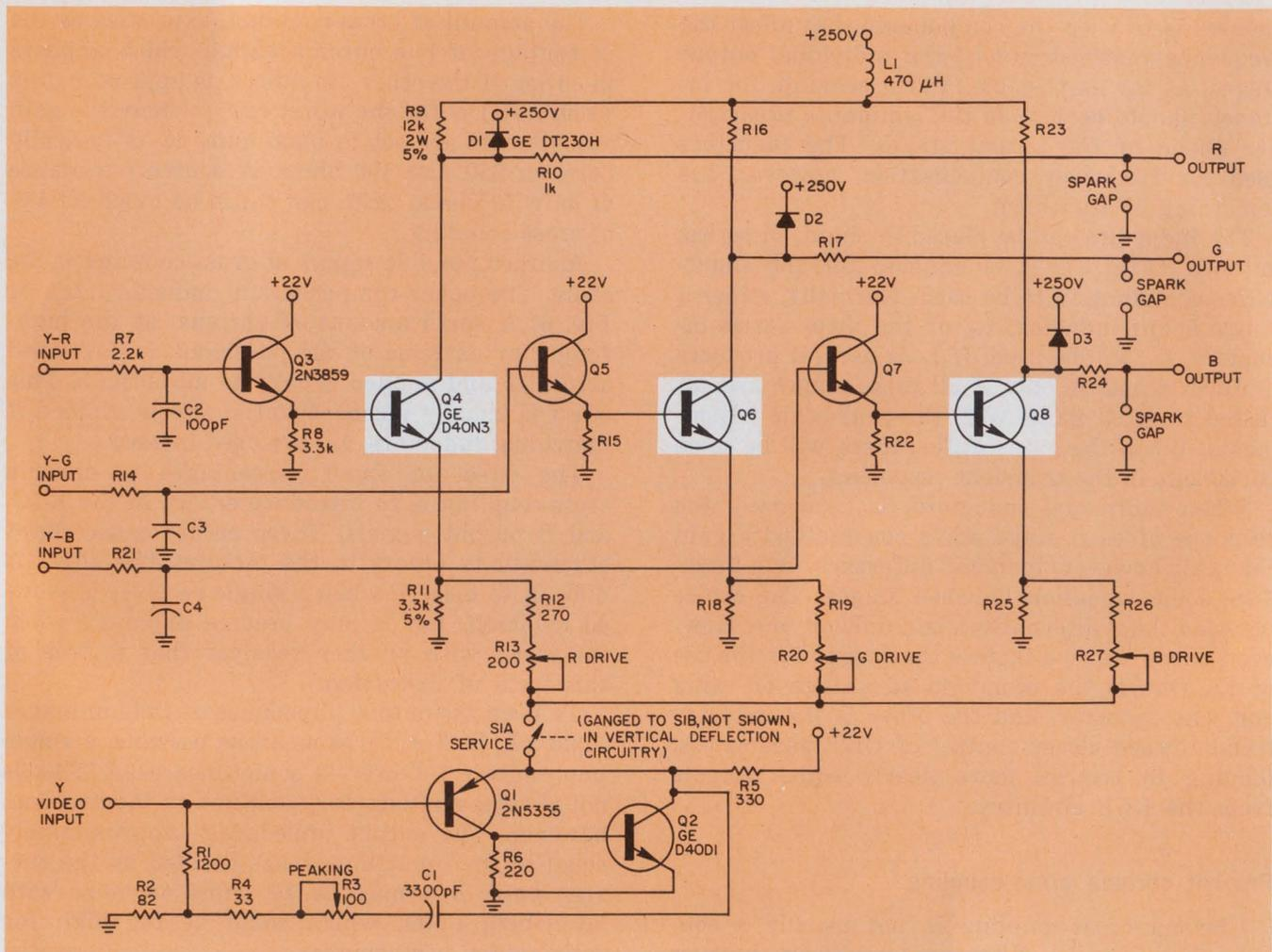
8. This complete RGB video amplifier uses a single shunt inductor for frequency compensation. Note how the low-impedance luminance preamplifier,  $Q_1$  and  $Q_2$ , of Fig. 7 is used to prevent chroma cross-coupling. The low-pass R-C filters on the three color-difference inputs are needed to attenuate the 3.58-MHz chroma carrier. And
