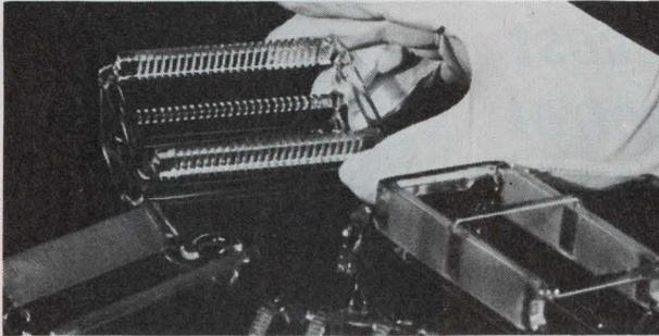
Newly designed carrier boats from Amersil are a marked improvement over slotted plate and slotted rod carriers for low and high temperature diffusion applications. This construction provides more secure wafer spacing for uniform diffusion.
