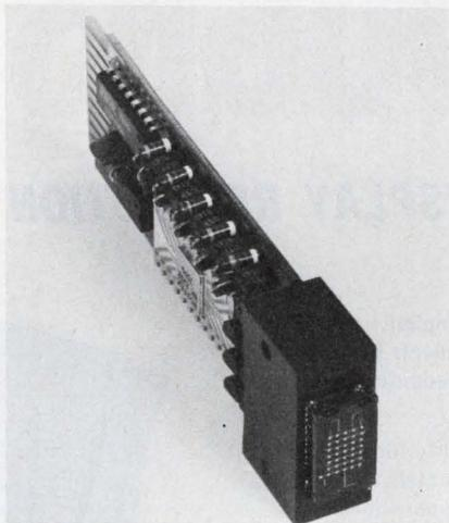
A complete alphanumeric LED display consisting of a 35-dot matrix readout and all the necessary driving circuitry in one package can now be purchased at \$68 in OEM quantities.
