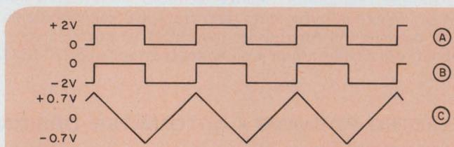
2. Available outputs include a fully adjustable triangular waveform, negative-going synchronization
