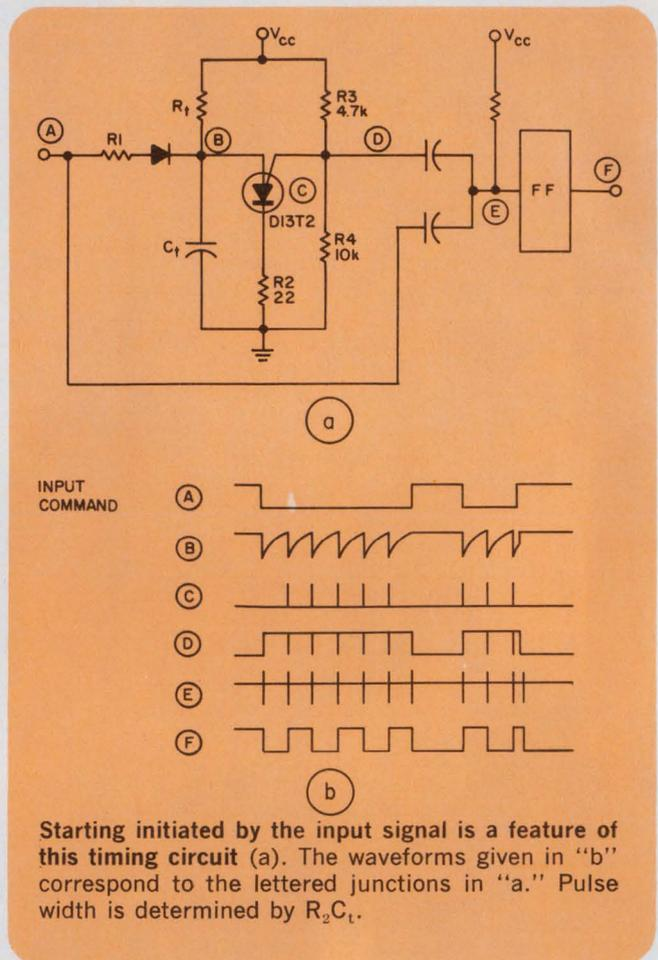
Starting initiated by the input signal is a feature of this timing circuit (a). The waveforms given in "b" correspond to the lettered junctions in "a." Pulse width is determined by  $R_2 C_1$ .
