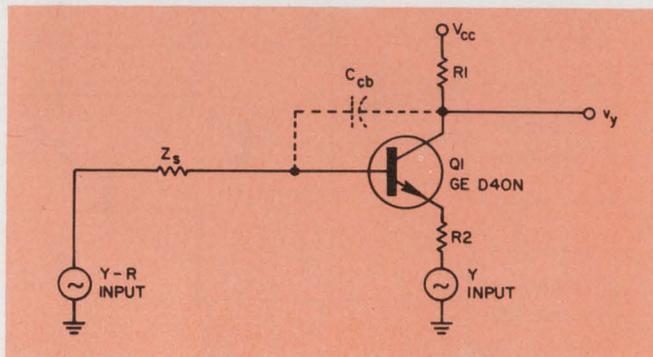
white level. The gain may be adjusted by changing either the collector resistance,  $R_1$ , or the emitter resistance,  $R_2$ , with a potentiometer. These potentiometers have an appreciable amount of stray capacitance that, in the collector circuitry, adds to the load capacitance. For this reason it is often preferable to place them in the emitter circuitry. There, the impedance is so low that the additional capacitance has no significant effect.
