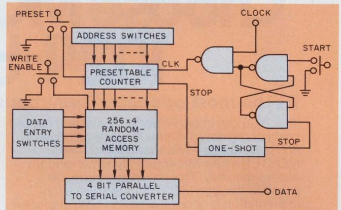
3. The random-access memory simplifies the programming when a large number of bits is to be stored. The presettable counter lets the operator select what information in the memory is to be transmitted. The RAM must be reprogrammed after each power interruption.
