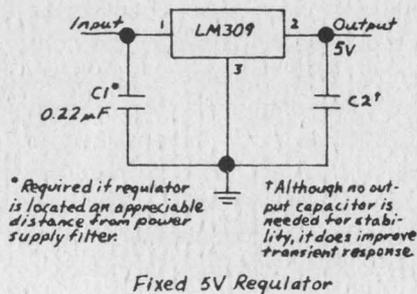
The easy-to-use LM 309 is a complete 5V regulator on a single silicon chip. Designed for local regulation on digital logic cards, the 309 neatly eliminates distribution problems caused by single-point regulation.
