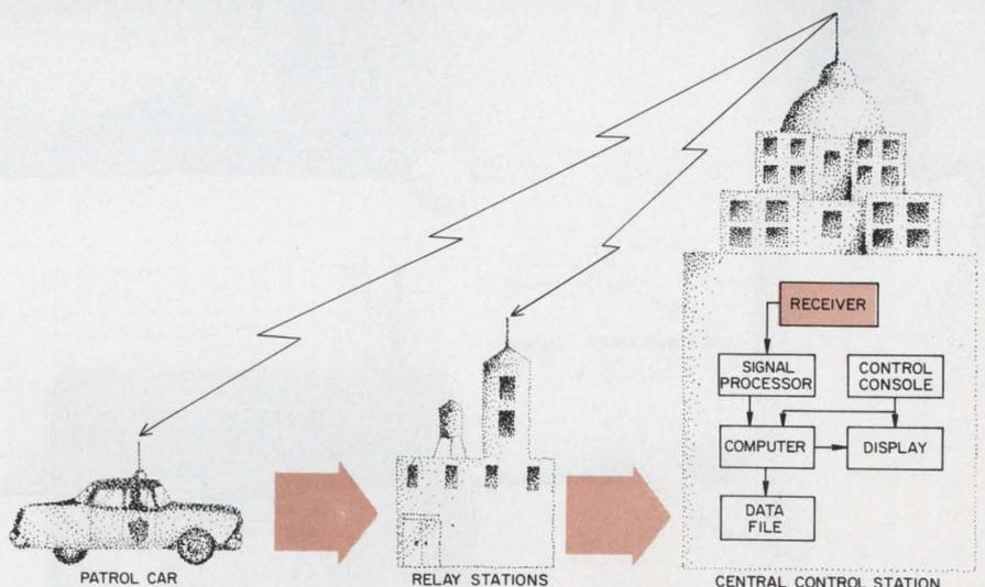
To locate a police car, signals from a central station trigger a pulse train from a transponder in each vehicle. This signal goes to relay stations and then to a computer that calculates time-of-arrival differences.
