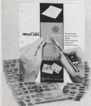
Circuit Zaps® are 1 ounce copper circuit component patterns, pads, and conductor paths, precision-etched on 5 mil (.005") glass epoxy base material, backed by a special pressure-sensitive adhesive. Circuit Zaps® completely eliminate the artwork, photography, photoprinting, touch up, etching, stripping, and other time-consuming steps in PC board development.
