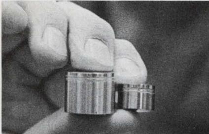
A miniature **nonthermal radio-isotope-fueled betavoltaic battery** has been developed by the Donald W. Douglas Labs of the McDonnell Douglas Astronautics Co., Richland, Wash. The battery is available in several sizes providing power levels from microwatts to a few milliwatts with useful lifetimes up to ten years.
