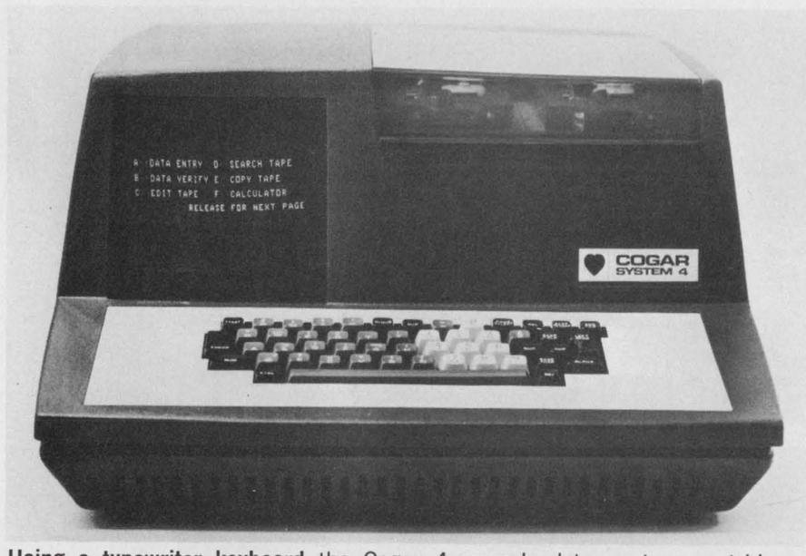
Using a typewriter keyboard the Cogar 4 records data on tape cartridges.
