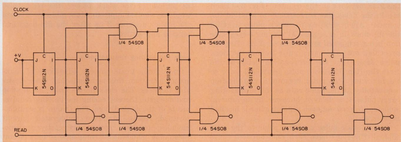
2. The features of both the synchronous and ripple counters are combined in a counter whose speed is limited
