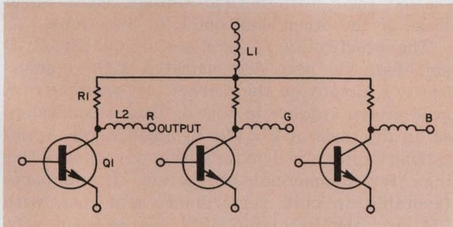
The amount of cross-coupling, expressed as the percentage of one chroma signal which appears in either of the other amplifiers, is approximately  $(100Z_s/R_2)\%$  for the worst case—where the gain adjustments are set to maximum.  $R_2$  is typically between 250 and 400 ohms. A source impedance of only 10 ohms, then, can cause as much as 4% of cross-coupling.
