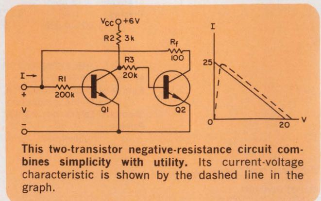
This two-transistor negative-resistance circuit combines simplicity with utility. Its current-voltage characteristic is shown by the dashed line in the graph.
