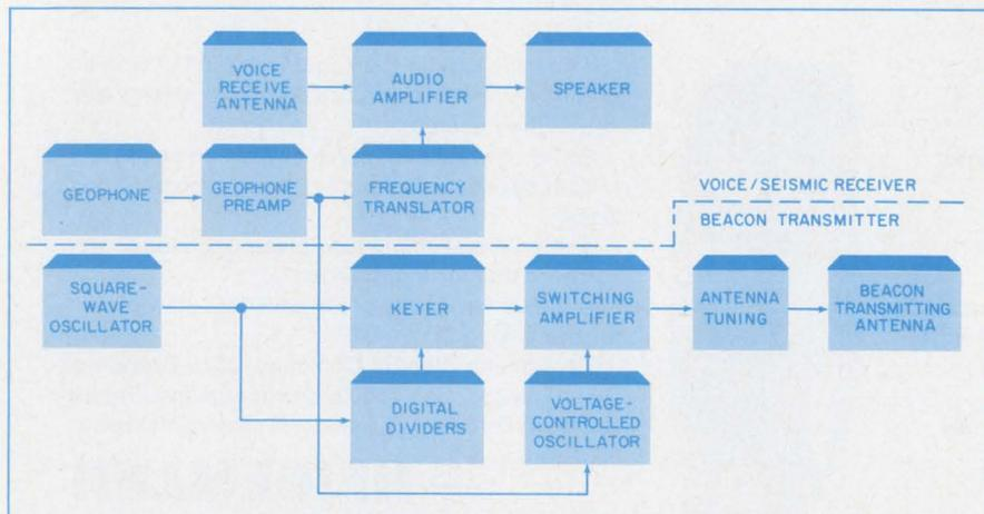
**This subsurface system** permits a trapped miner to receive instructions from a rescue team on the surface by through-the-earth voice communications. He replies with coded signals sent by a pushbutton square-wave oscillator.
