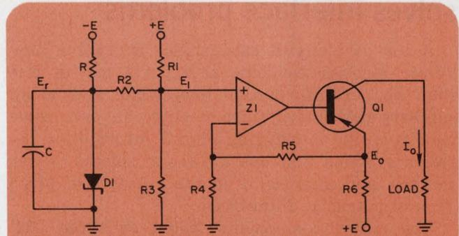
A very accurate, stable constant-current supply makes use of op amp  $Z_1$ . Neither the zener diode,  $D_1$  nor the amplifier carries any load current. The output transistor,  $Q_1$ , which supplies the load, has its  $V_{be}$  within the feedback loop to minimize the effect of this parameter on performance.
