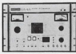
For the on-line processing of underwater acoustic signals, radar, sonar and other data where the maximum frequency resolution is always sought, new UA-9A series 1,000-line and 2,000-line Low Frequency Real-Time Spectrum Analyzers have been designed by Federal Scientific, originators of the Ubiquitous® analyzers.
