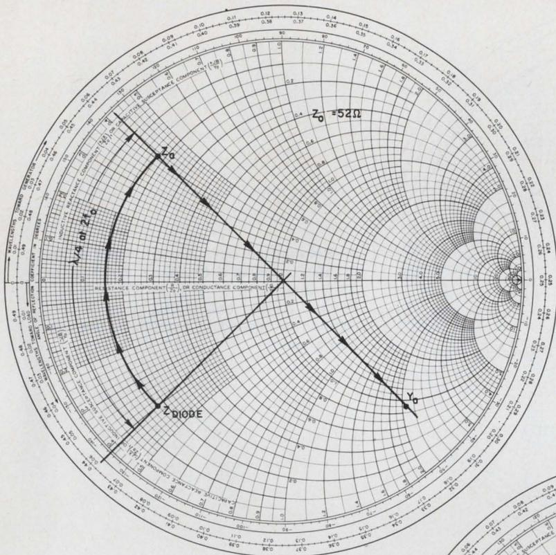
1.  $Z_{\text{diode}}$  is rotated an eighth of a wavelength at  $f_0$  by the line connecting the input filter to the diode. This transforms it into  $Z_{\text{in}}$  or, equivalently, to  $Y_{\text{in}}$  which turns out to be  $50 \Omega$  in parallel with an inductance.
