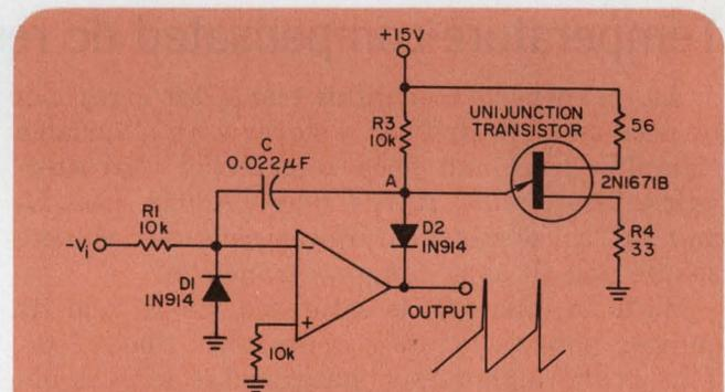
A voltage-to-frequency converter with 0.4% linearity can also operate as a sawtooth generator. This uncomplicated inexpensive circuit provides good temperature stability, too.
