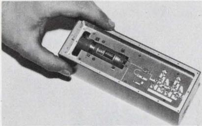
A new dual-two-stage filter that is able to use YIG-tuning techniques and still be compatible with microwave integrated circuits is now on the market. The unit has two separate two-stage filters within the same magnetic structure, yet measures a mere 0.75 inch in diameter and 2.1 inches in length.
