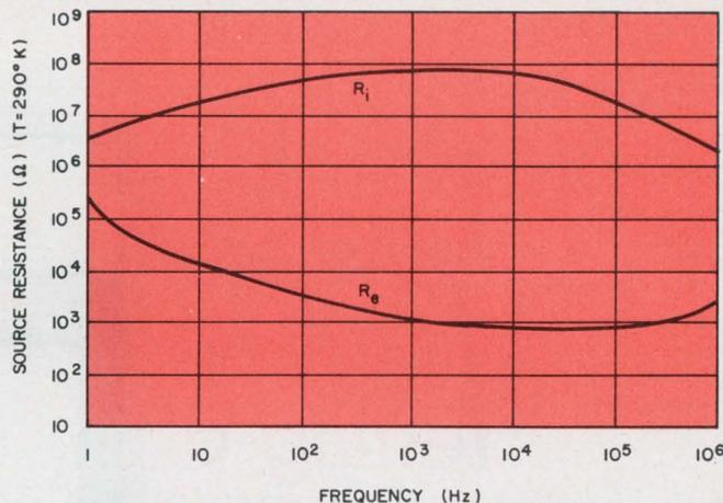
2. A plot of  $R_e$  and  $R_i$  is roughly equivalent to a 3-dB noise-figure contour in the region where the curves are widely separated. This particular amplifier has a minimum noise figure of 0.03 dB at 10 kHz.
