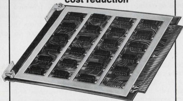
A small, voltage-distributing busbar for PC card application, each Mini/Bus gives you built-in capacitance . . . noise-cutting capacitance that means more reliable, compact circuit packaging at a fraction of multilayer prices. Write for data.
