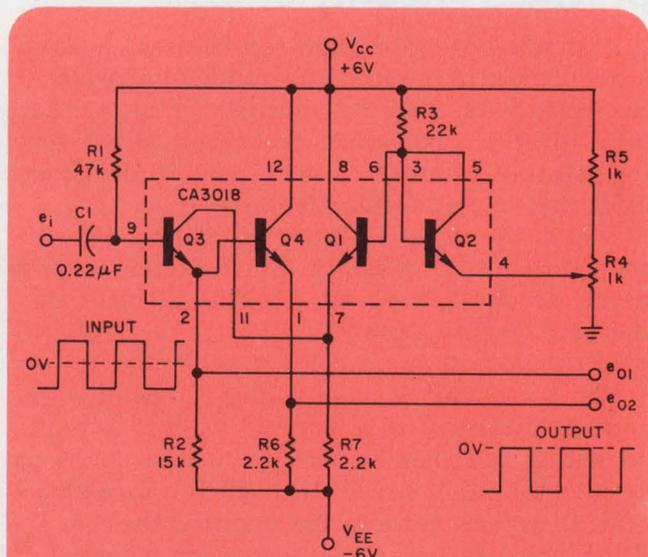
Monolithic quad transistor array with a minimal number of external components yields a low-temperature-coefficient dc restorer with adjustable clamping level and emitter-follower output.
