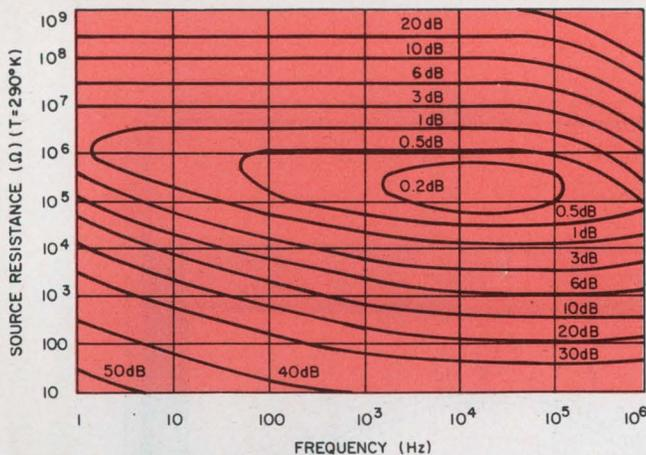
1. Noise figure is a constant for a given contour. Note that the NF is a single-valued function of source resistance and frequency, although there are two values of  $R_s$  for each combination of frequency and NF.
