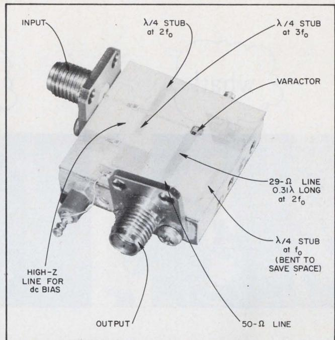
5. The complete doubler is only 1 inch square. It can provide an output of 1 W at 4 GHz with an efficiency of 45%. The unit has a maximum VSWR of 1.5 : 1 and a 1-dB bandwidth in excess of 5%.
