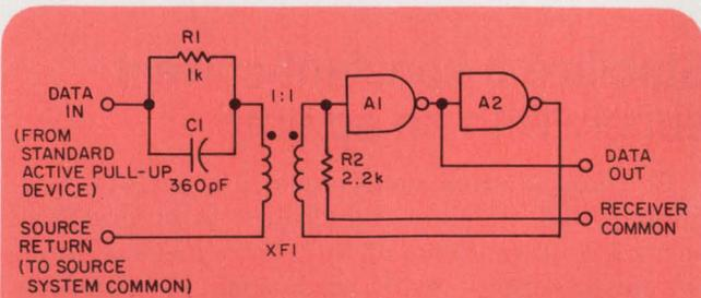
An interface circuit, acting as a line-driver/receiver, can cut parts cost to under \$5 per information line. Dual-in-line quad transformers and integrated-circuit hex inverters are used.
