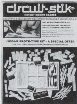
The PROTO-TYPE KIT CONTAINS a total of one hundred eighty parts — enough to mount over four hundred electronic components and allows "instant" fabrication of several printed circuit boards. CIRCUIT-STIK'S printed circuit sub-elements are pre-etched, pressure sensitive adhesive substrates: pre-drilled, pre-plated-fluxcoated-ready for mounting and soldering of discretes, I.C.'s, transistors, connectors, and other electronic components. (U.S. patent #3,538,389 and other patents pending)
