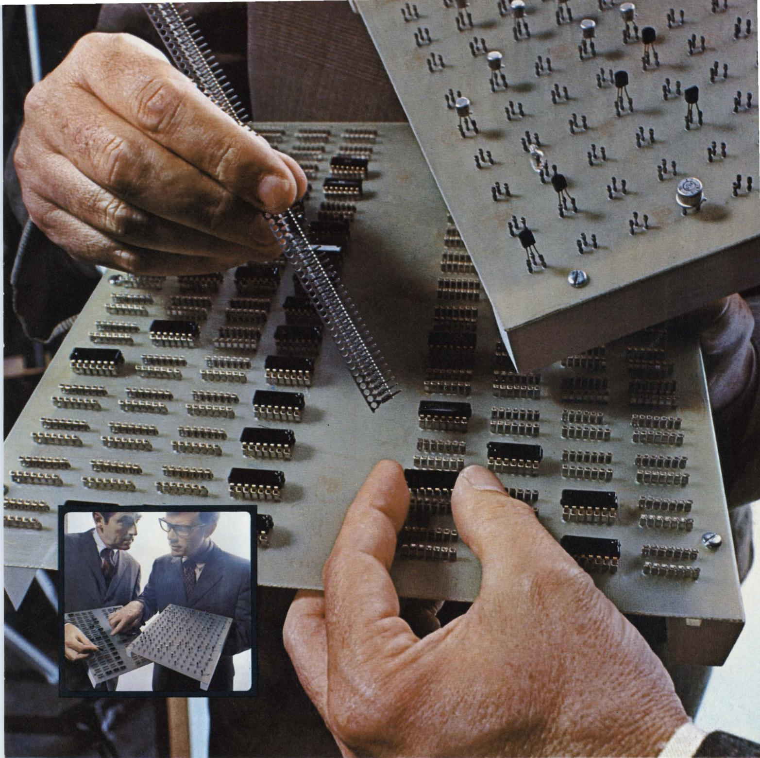
**HERE'S A NEW AND BETTER WAY:** To make printed circuit board connections. Reliably. At low, low cost. They're Molex Soldercon<sup>®</sup> terminals. Integrated circuit and transistor terminals. Offering the convenience of plug-in I.C.'s and transistors *without* the cost of insulators. They fit directly on the board. And there is equipment available to do the job *automatically*. Fast! Soldercon terminals save time. Money. Speed installation. Make
