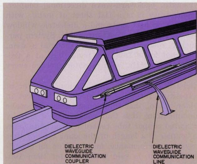
3. Bandwidths of up to 500 MHz are possible with a dielectric waveguide communications link. A length of waveguide on the vehicle couples energy from the line. The waveguide consists of a semicylindrical rod of polyethylene, bonded to a metal shield.
