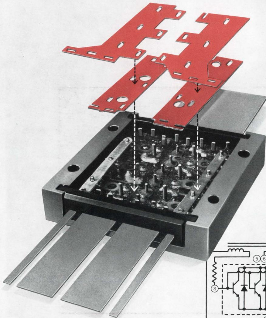
Exploded view shows one of the standard interconnections of the RCA hybrid power module as used in a common-emitter inverter. That portion within the dotted lines in the circuit schematic represents the RCA module.
