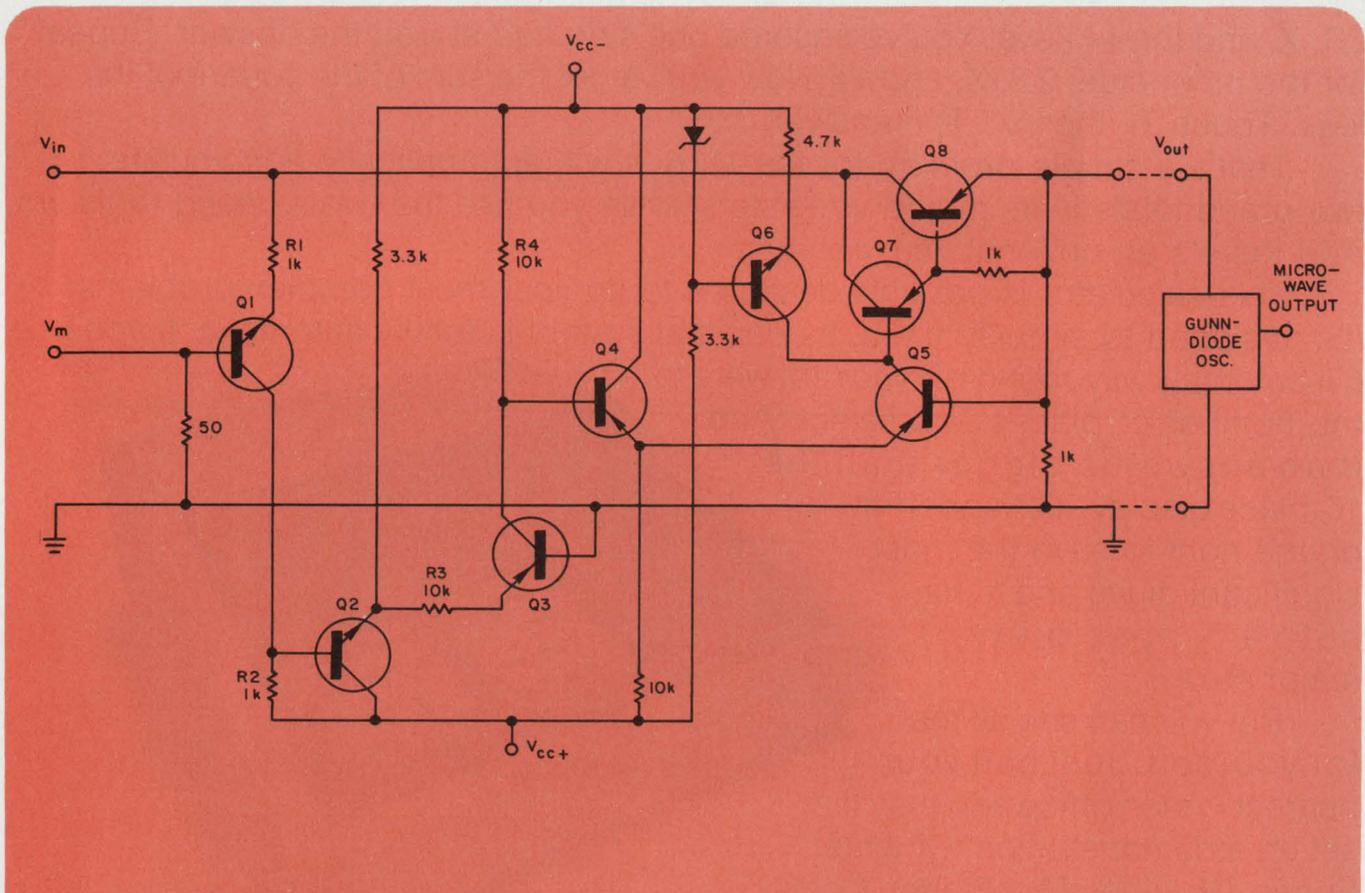
**This modulator for X-band Gunn diodes** supplies 100 to 300 mA at 7 to 12 V dc. Its output resistance is extremely low, to prevent bias oscillations of the diode. Transistors  $Q_1$ ,  $Q_2$  and  $Q_6$  are ITT
