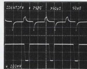
■ **PEAK-TO-PEAK AUTO TRIGGERING** is the only *truly automatic* triggering. It makes triggering as simple as pressing three push-button controls: P-P AUTO AC INT
