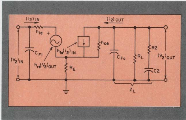
5. With the second stage described by its mid-frequency equivalent ac model (hybrid configuration), the input and output capacitance  $C_{F1}$  and  $C_{F0}$  are defined by the Miller Effect.
