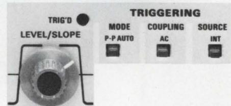
Now a triggered sweep is obtained regardless of the LEVEL/SLOPE control position.
