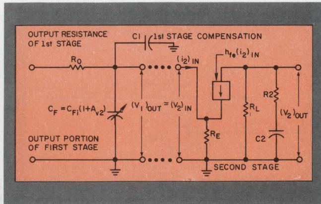
6. Valid ac model of combined first and second stages of the device, with  $C_{F0} = 0$  and with the effect of h-parameters reduced for analytical simplicity. Note that  $C_{F1}$  is a function of the second-stage gain,  $A_{V2}$ , the impedance of which decreases with an increase in frequency; this variation in  $C_{F1}$  is compensated by  $C_1$  connected in parallel.
