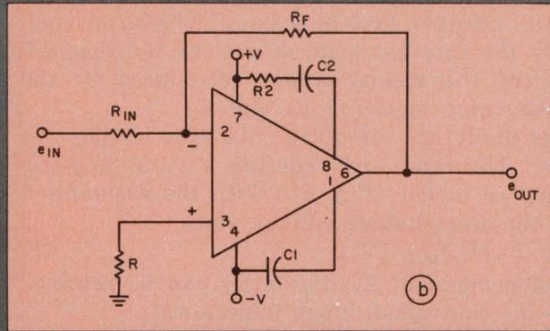
1. The recommended compensation specified by the manufacturer employs a single capacitor that introduces a simple 20-dB roll-off at low frequency and stabilizes the device against temperature variations and parts re-
