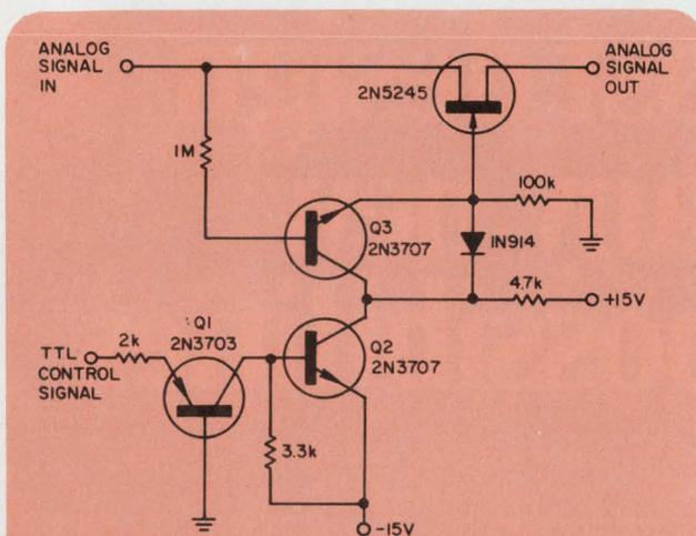
This low-cost TTL-compatible analog gate is ideal for a myriad of instrumentation and telemetry applications. It is based on the analog-gate circuit described in another Idea for Design,<sup>1</sup> with transistors  $Q_1$  and  $Q_2$  added to make the circuit compatible with TTL logic levels.
