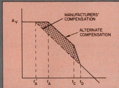
2. Bode plots of both compensation techniques are compared by graphical superposition to illustrate the increased gain for the extended frequency domain. Note the addition of another pole and zero to the Bode plot.
