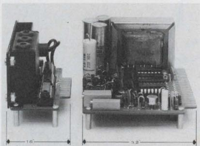
Separate display and a/d converter plug-in modules can mount together or remotely through a cable.
