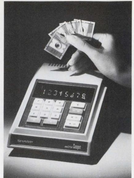
Sharp calculator is mechanized with four MOS/LSI chips and a clock generator. Each chip contains 900 MOS transistor equivalents.
