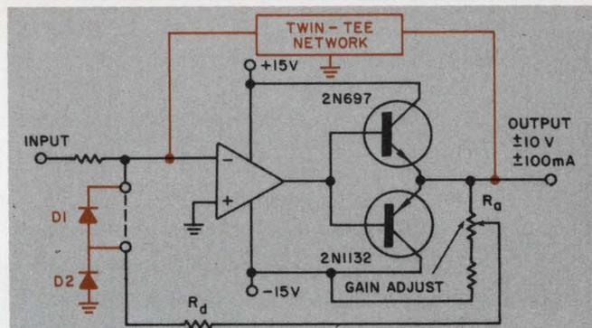
1. The emitter followers boost the op-amp power to about 0.5 W. With the dashed line connected and the colored components omitted, the circuit is a linear amplifier. The reverse case yields an oscillator-driver.
