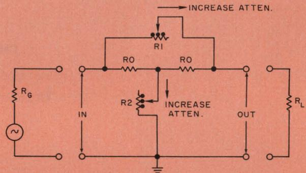
$$R_G = Z_{in} \quad R_L = Z_{out} \quad Z_{in} = Z_{out} = R_0 \quad (R_1)(R_2) = R_0^2$$
