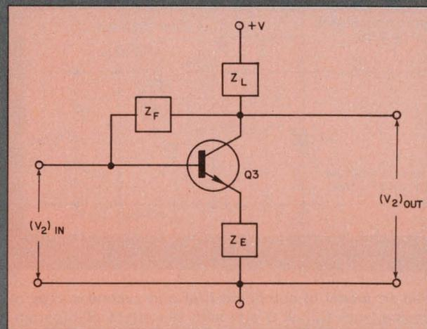
4. The device's second stage is redrawn (a) for analytical simplicity. Internal as well as compensation (external) feedback elements are recognized. The second
