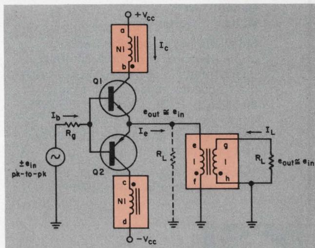
3. The generalized split-load output stage has an  $N_1:1$  turns ratio between the collector windings and the output windings. In the analysis in the text it is assumed that  $\beta$  is high enough to consider  $I_e = I_c$ .
