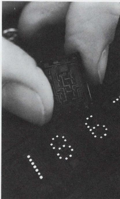
A new solid-state LED numeric display features 5-V logic-level compatibility and a 4-by-7 dot matrix. It also includes a decoder-driver and a memory on the same substrate, plus a red filter, for a cost of only \$10.
