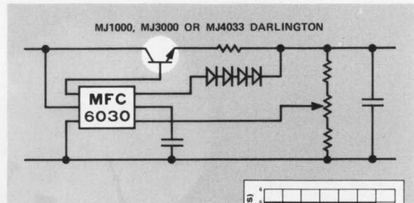
A short-circuit protected supply with 3, 5, and 10 A outputs obtained with MJ1000, MJ3000 or MJ4030 Darlington and an MFC6030 regulator. For each output, load regulation is 0.08% when used as 5 V regulator. Short-circuit characteristics indicate limiting performance with each Darlington. MFC6030 Functional Circuit has 38 V maximum input voltage, 200 mW maximum load current and 3 V minimum voltage differential.
