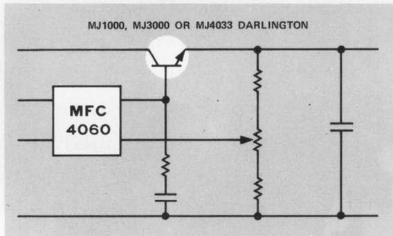
Economical "Darlington + Functional" circuit performs as 3, 5, or 10 A, 5 V regulator. An MJ1000 ( $I_{out} = 3$  A) affords load regulation of 0.02% @ 0°C, 0.2% @ 25°C and 0.04% @ 75°C. An MJ3000 ( $I_{out} = 5$  A) furnishes 0.04% load regulation for each temperature. An MJ4030 ( $I_{out} = 10$  A) yields load regulation of 0.04% @ 0°C and 25°C and 0.06% @ 75°C. MFC4060 is the same as MFC6030 except for current limiting 30 V outputs possible for both circuits.
