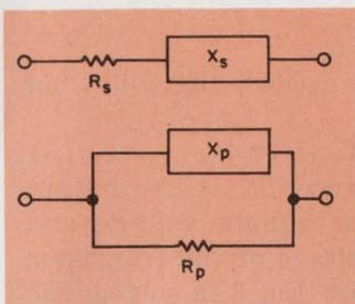
1. At any specified frequency, a series resistance-reactance pair can be represented by a parallel equivalent. The parallel resistance equivalent,  $R_p$ , will always be greater than the series resistance,  $R_s$ .
