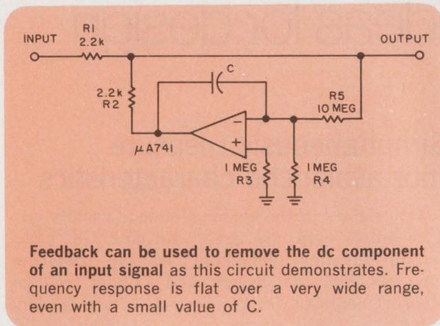
Feedback can be used to remove the dc component of an input signal as this circuit demonstrates. Frequency response is flat over a very wide range, even with a small value of C.
