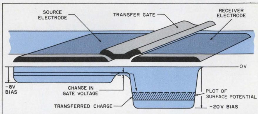
1. The schematic view of GE's new surface-charge transistor shows that the charge on the larger source electrode has been transferred from its center open potential region (bounded by the two lines in the potential plot) to the smaller receiver electrode by means of a small increase in negative gate voltage. Device voltage gain is proportional to the ratio of the source electrode to the receiver electrode areas.
