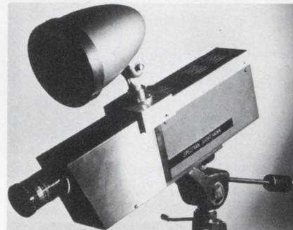
The new **Night Hawk TV camera system** of Spectran, Inc., can see in total darkness and provides a picture as bright and clear as one taken under bright lighting. It also performs equally well under visible lighting. The camera system consists of an IR source, a CCTV camera and a tube mounted on the camera for converting IR light to visible light.
