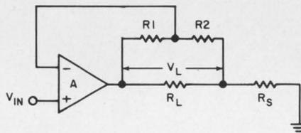
$$\frac{V_L}{V_{IN}} = \frac{1}{\frac{1}{A} \left( 1 + \frac{R_o + R_s}{R_L} \right) + \frac{R_s}{R_L} + \frac{R_2}{R_1 + R_2}}$$
