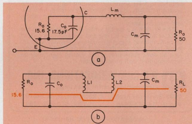
4. Output capacitance  $C_0$  can be integrated into a matching network (a) at the output of a transistor. The easiest way to see how the circuit works is to imagine the inductor,  $L_m$ , to be broken into two series inductors,  $L_1$  and  $L_2$  (b). The colored line shows how the impedance is affected by the inductors.  $C_0$  cancels out the effect of  $L_1$  at  $f_0$ ;  $C_m$  does a similar job for  $L_2$ .
