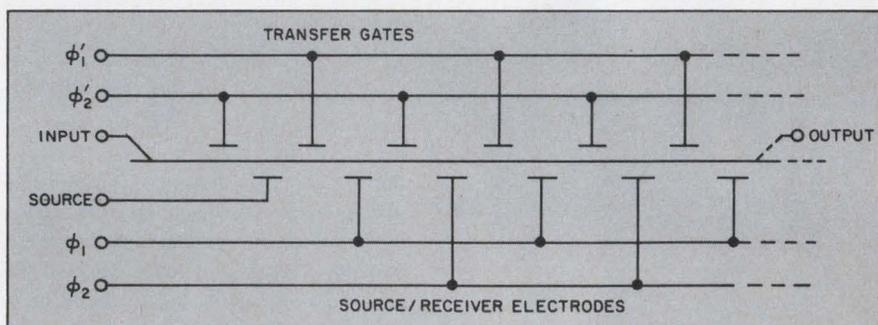
2. A serial type of surface-charge transistor shift register has a sequence of electrodes deposited on a single silicon substrate. Two driving phases are required, with bits entering the register at the left-hand source.
