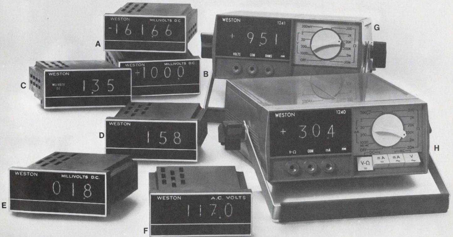
A. 4 1/2-digit bi-polar Model 1294    B. 3 1/2-digit bi-polar Model 1292    C. 2 1/2-digit Model 1260    D. Event Counter Model 1266    E. 3-digit Model 1261
