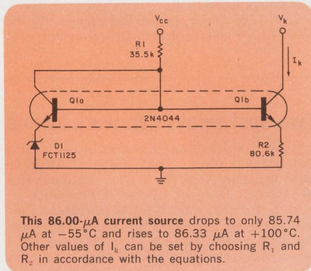
This 86.00- $\mu$ A current source drops to only 85.74  $\mu$ A at -55°C and rises to 86.33  $\mu$ A at +100°C. Other values of  $I_k$  can be set by choosing  $R_1$  and  $R_2$  in accordance with the equations.
