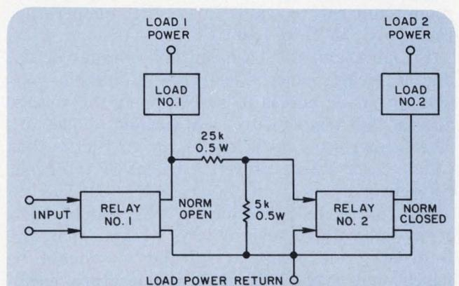
With no input, relay No. 2 is kept energized by the trickle current through load No. 1. This keeps load No. 2 normally on.
