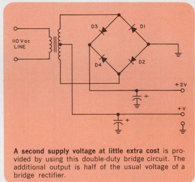
**A second supply voltage at little extra cost** is provided by using this double-duty bridge circuit. The additional output is half of the usual voltage of a bridge rectifier.
