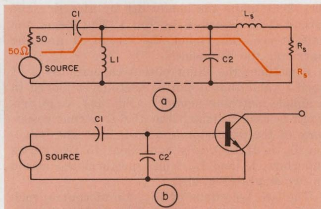
3. The parasitic inductance compounds the problem by making two impedance changes necessary (a). The colored line represents the impedance (to ground) of the various portions of the circuit.  $L_s$  raises the transistor resistance  $R_s$  above  $50 \Omega$  so that  $C_2$  is needed to bring it down again.  $L_1$  and  $C_2$  can be combined, resulting in  $C_2'$  and a two-capacitor matching network (b).
