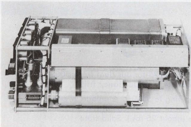
2. **This 1-kW uhf amplifier is only 6.5 × 7.5 × 17 inches.** The package contains the cavity, power supply, control and monitoring circuitry, and low-pass output filter. Only the heat exchanger is packaged separately.
