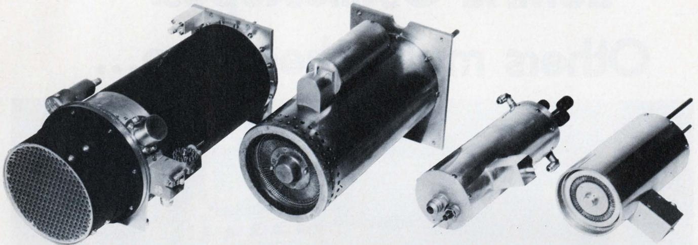
1. **Dramatic size reductions are possible** when a fluid dielectric is used. These are all 1-kW uhf cavities covering 225 to 400 MHz. Starting from the left, the first one is an air-cooled production unit that has been used in many installations. The second cavity uses the same tube, but has a re-entrant output circuit, which reduces its
