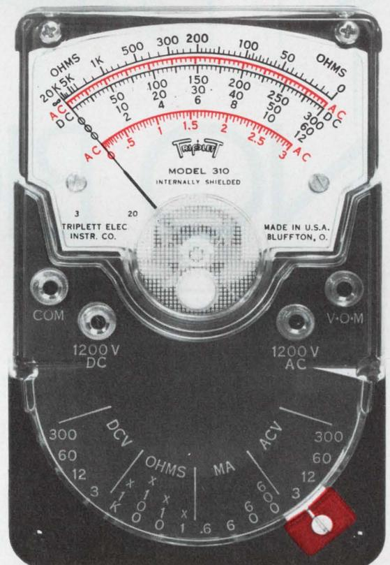
1. Hand size V-O-M with provision for attaching AC clamp-on ammeter.
