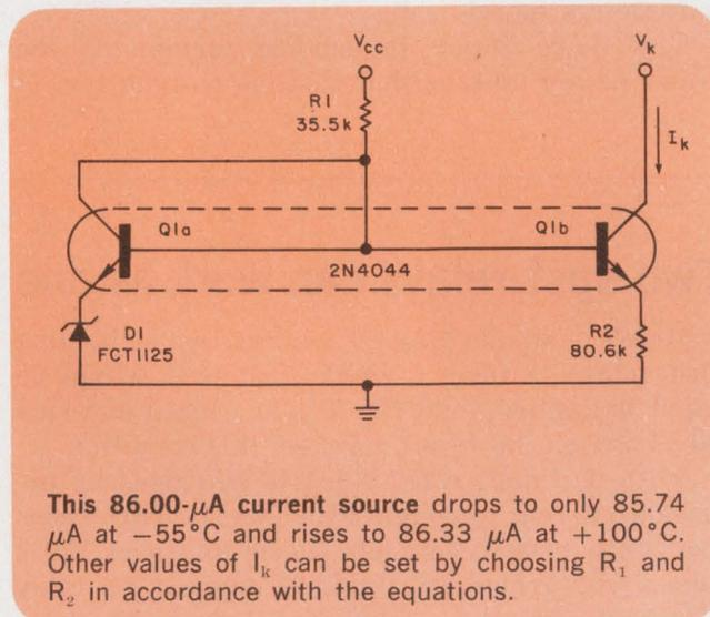
This 86.00- $\mu\text{A}$  current source drops to only 85.74  $\mu\text{A}$  at -55°C and rises to 86.33  $\mu\text{A}$  at +100°C. Other values of  $I_k$  can be set by choosing  $R_1$  and  $R_2$  in accordance with the equations.
