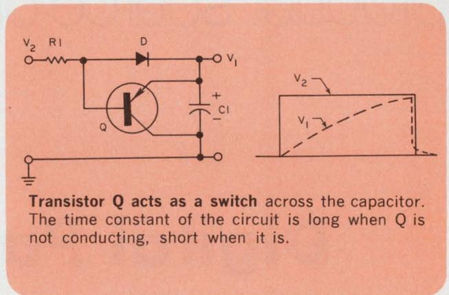
**Transistor Q acts as a switch** across the capacitor. The time constant of the circuit is long when  $Q$  is not conducting, short when it is.
