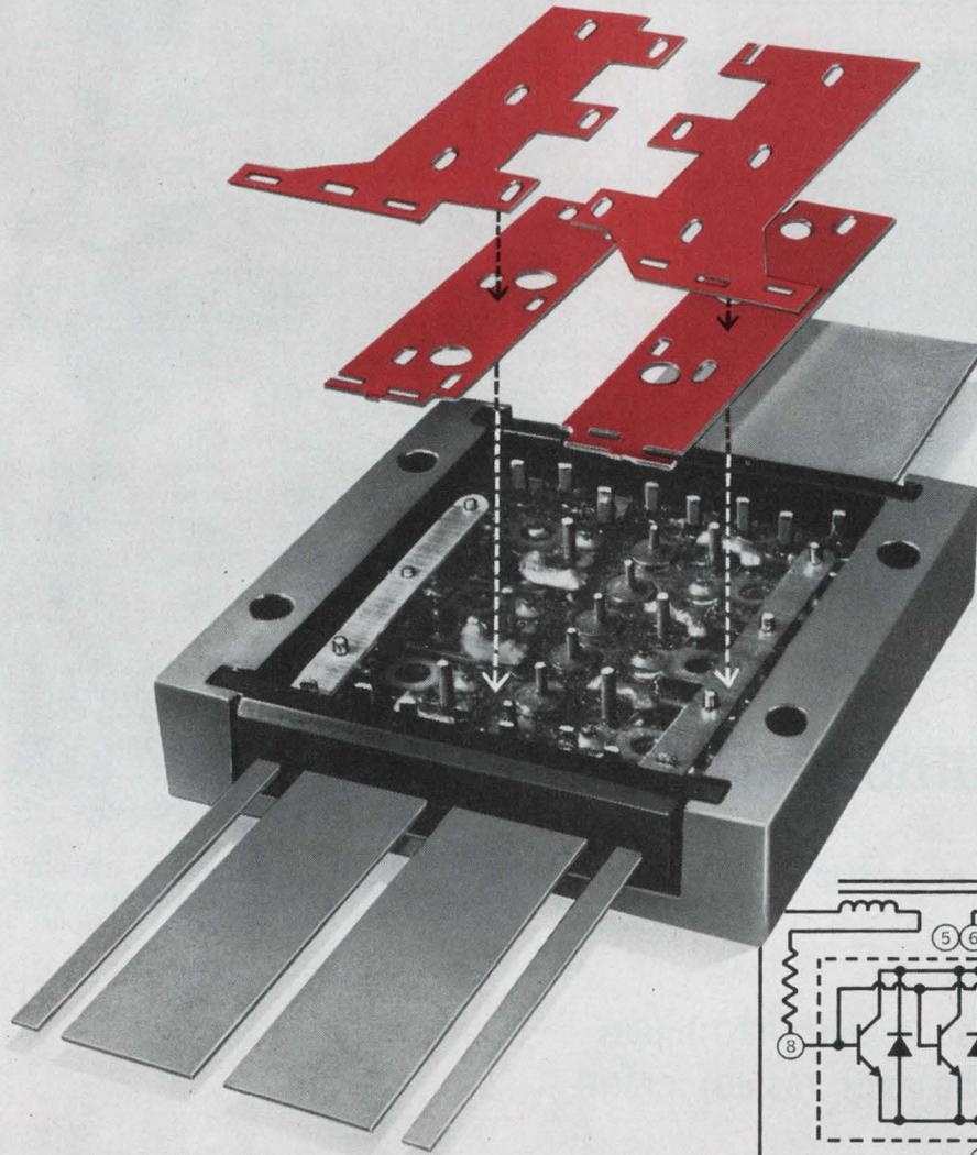
Exploded view shows one of the standard interconnections of the RCA hybrid power module as used in a common-emitter inverter. That portion within the dotted lines in the circuit schematic represents the RCA module.
