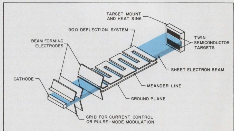
**Electron Beam Semiconductor** operates at kilowatt level and is scheduled to go into production at Watkins-Johnson in six months.
