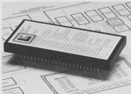
**Standard MOS/LSI devices, such as this data communicator developed by Larse Corp., may eventually replace pneumatic equipment now used for control functions in factories.**
