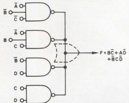
(Incidentally, this circuit is the correct wired-OR implementation for F, as shown on p. 90 of the article.)
