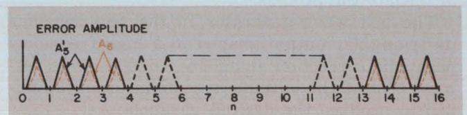
4. A higher-order harmonic, here called  $A'_5$ , can be passed through a diode. The square-law diode characteristic generates an error-correcting parabolic curve,  $A_6$ .
