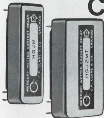
Compare the new Clare HGJ Relays with any other mercury-wetted contact relays. You'll get more speed, less noise, and less jitter — in less space than any other! Take your choice: 0.340" profile for true half-inch pcb spacing, 0.400" profile for higher sensitivity. Single-pole HGJM, two-pole HGJ2MT. Both are capable of switching low level to 2 amp max, 500 v max (100 va max, ac or dc).
