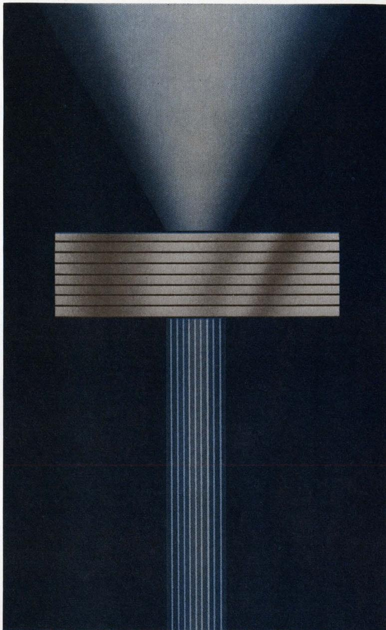
Until now, no one has been able to produce holes in thick metal at anything smaller than a one-to-one ratio. We put our world leading technology in photomechanical reproduction to work and came up with a way to laminate sheets of etched metal in perfect register. We can produce sharply cornered holes of any design in metal much thicker than the width of the hole.
