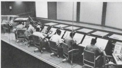
Three 7-by-7-foot translucent screens present in six colors the positions and tracks of ships, aircraft and drones on the sea ranges to the north and south of Puerto Rico. The information is fed both through a computer and manually by operators at consoles. Projection is from the rear of the screen.
