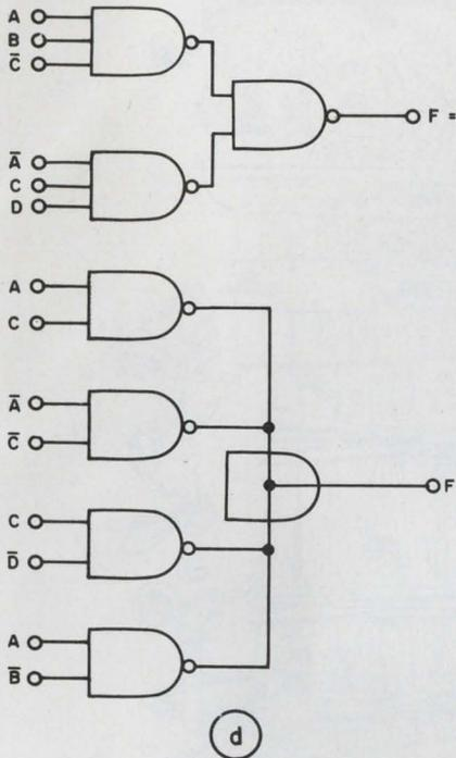
Mr. Pappa's point on serviceability is well taken. The wired-OR does present a problem when the output, F, is at a permanent ground. Granted that all DTL outputs must be removed to find the defective gate, we really are only interested in determining which IC package is bad.
