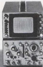
100 MHz frequency range, here's a storage scope with bandwidth
