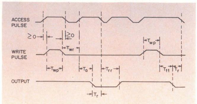
5. The cycle times for all possible memory operations can be determined from the switching characteristics. For example, the WRITE to READ cycle time is the sum of WRITE pulse width ( $T_{wp}$ ) and the recovery time ( $T_r$ ).
