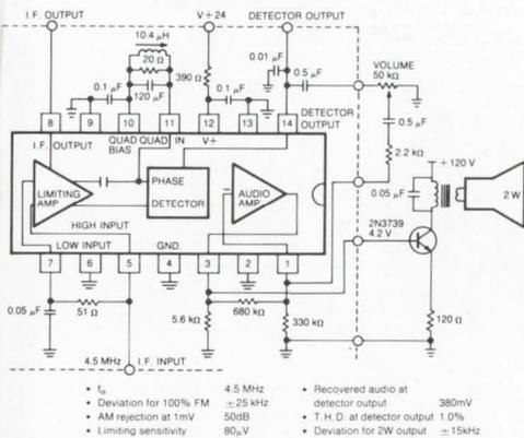
Use 'em in TV, mobile receivers, line-operated and automobile FM and as synchronous AM detectors.
