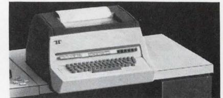
**model 37 series:** One of the most versatile heavy-duty terminal lines going. Generates all 128 characters of ASCII. Operates at 150 wpm. Prints in upper and lower case.
