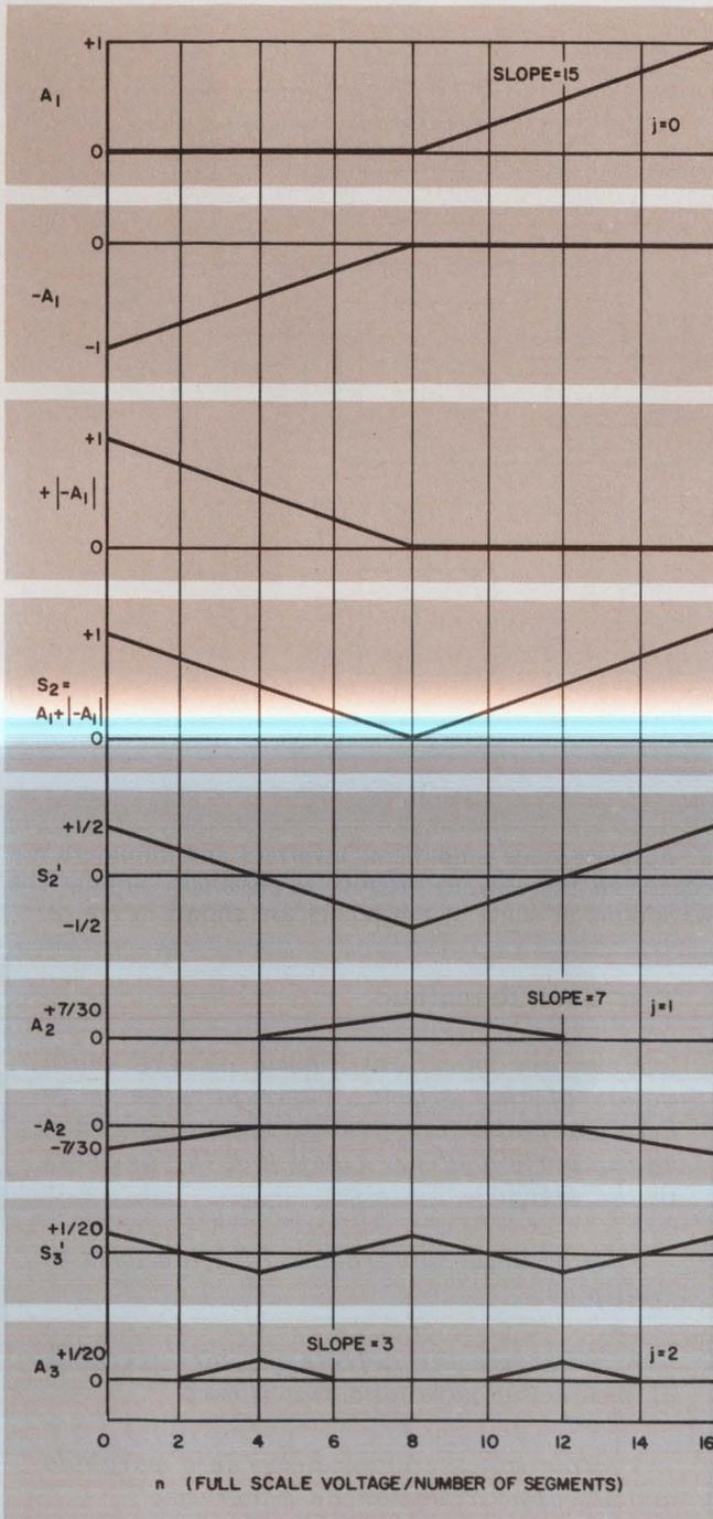
2. The outputs of the triangular-wave generators are  $A_1$ ,  $A_2$  and  $A_3$ . Their slopes decrease in the ratio 15:7:3.  $A_1$  is not shown, but its slope is one. The curves  $S'_2$  and  $S'_3$  are input signals in the circuit shown in Fig. 6.
