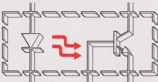
Couple a GaAsLITE to a silicon detector, and you get almost perfect isolation between input and output; 100,000,-000,000 ohms. Our opto isolators listed here do just that, and more. They give high performance at great speeds for very low cost. Scan the details. Each is packaged for mass production handling, and each is priced to suit quantity applications.
