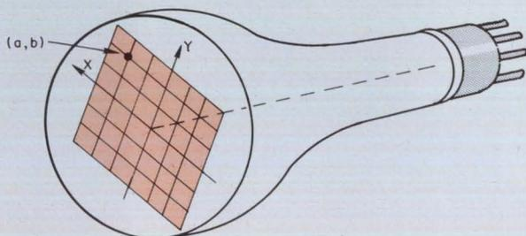
2. The first step in compensating for distortion is to divide the CRT face into a grid. The X and Y deflection voltages for each point determine the correcting network.
