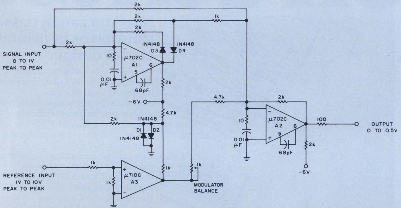
Modulator's reference input may be a sine function or complex wave shape.  $A_3$  produces a square wave
