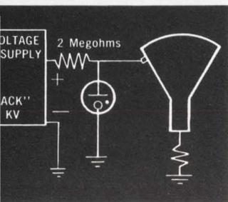
In this circuit example, a Corotron M42D-9.7 (9,700 volts) regulates a high voltage power supply for a computer data display system cathode ray tube. The Corotron provides reliable line and load regulation, and clarity of the CRT display.
