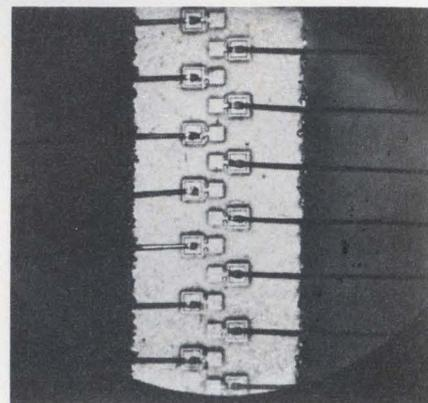
A Typical Array with .0033" x .0033" InSb Elements Spaced .0033" Apart.
