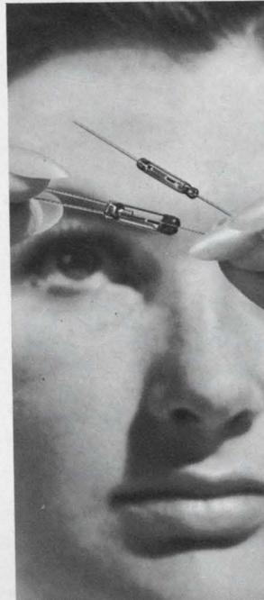
Hamlin's miniature, mercury-wetted switches offer all the advantages of high-speed, reed switches with the low contact resistance and high-power capacities of mercury switches. Precise, "on-off" actuation makes mercury-wetted switches ideal for applications where contact bounce cannot be tolerated. Available in form A (100 VDC) and form C (28 VDC). Useable length as low as .835". Write for catalog. Hamlin, Inc., Lake Mills, Wis. 53551. Or call 414/648-2361.
