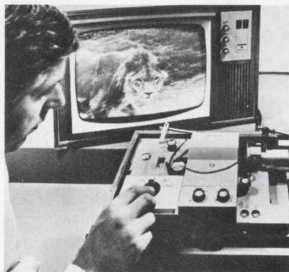
Conventional Super-8 movies can now be transmitted to any number of black-and-white television screens by a new system that resembles an ordinary tape recorder. The equipment consists of a projector and a small video camera which picks up the image for transmission to the TV screen. Either spools or cassettes of film can be used, and sound can be recorded on pre-stripped film through the equipment. The manufacturer is Vidicord Holdings Ltd., Condon, England.
