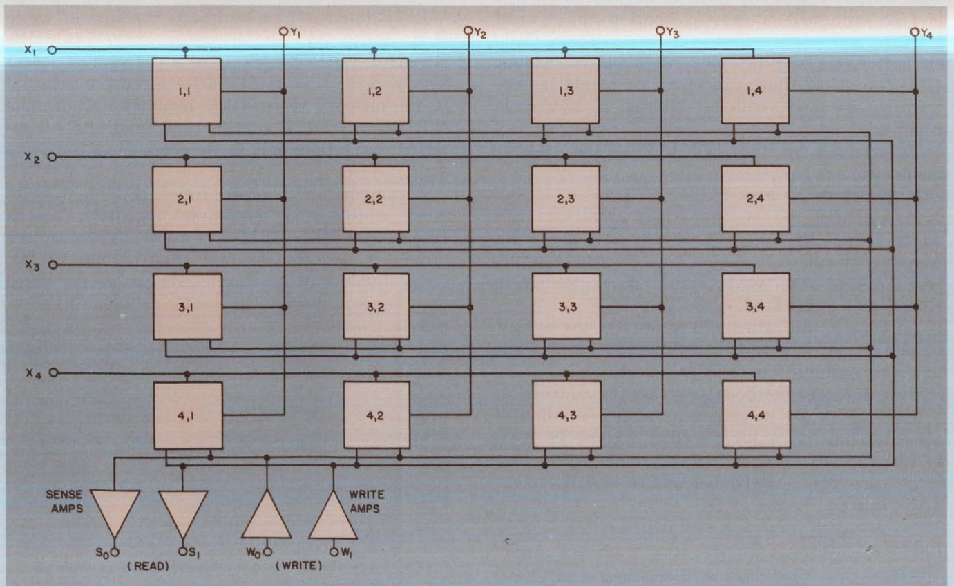
3. Compare the use of coincident selection for this 16-by-1-bit RAM with the linear selection used in Fig. 2.
