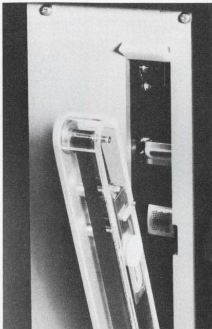
A new data storage system called Comfile provides the data access and organization styles of discs and drums at the low costs associated with magnetic-tape cartridge systems. At the heart of the new system is a 30-inch-long magnetic-tape loop capable of storing up to 72,000 characters of data. This stored data is accessible within an average time of 315 ms.
