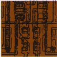
Fairchild's 9300 is the world's most versatile shift register. And we can prove it. The 9300 Four-bit Universal Register can perform as a high-speed shift register, modulo N counter, up/down counter, storage element, four clocked D-type latches, a programmable divider, a binary to BCD shift converter, serial to parallel converter (and vice versa), and a dozen other functions. It's a prime example of the kind of versatility inherent in Fairchild's entire MSI family.
