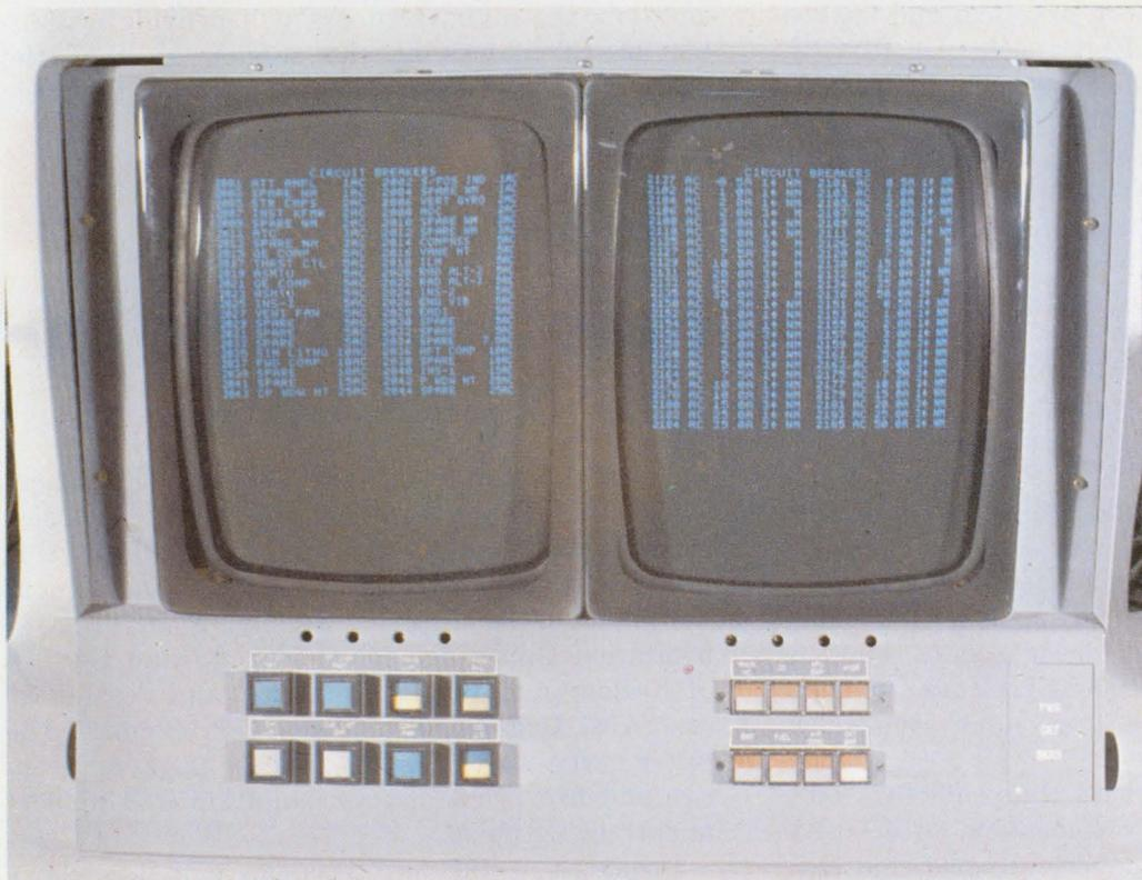
Cathode-ray tube display center is used in Bendix Corp.'s new Airborne Display and Electric Management System (Paper 17.2).
