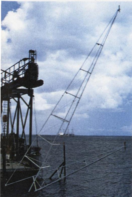
**At the underwater tracking range** off St. Croix, 11 hydrophone arrays (similar to the one at left) are anchored at the bottom of the sea, where they track with great precision any moving object that is equipped with a time-synchronized pinger. Ships evaluate their new torpedoes, Asroc rocket-torpedoes, their sonar and other gear. Much of the show is run from a console (below).
