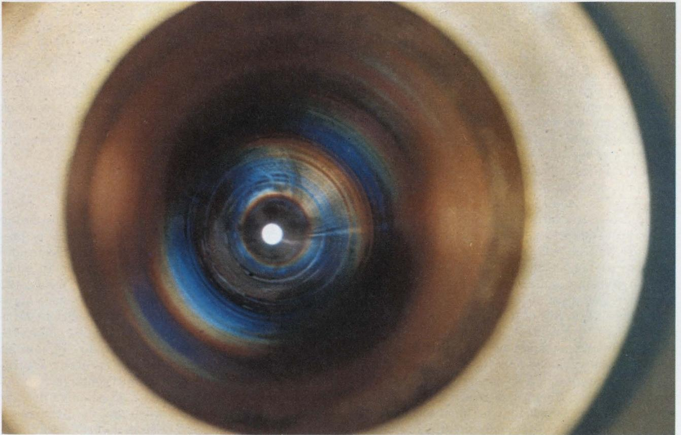
View down a helical waveguide symbolizes an experimental millimeter-wave communications system that is now under investigation at Bell Telephone Laboratories,
