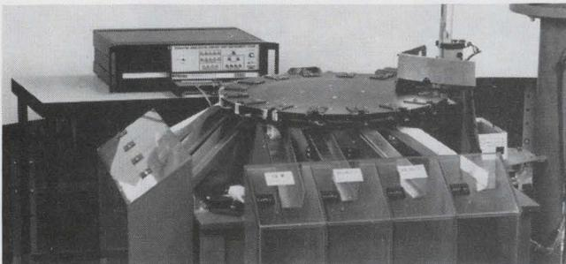
thorough testing. Lots are first sample-tested dynamically. Once a lot passes these tests, DEC puts every IC in that lot through a full battery of functional and dc parametric tests. And it manages these dc and functional tests with an instrument that isn't much bigger than a breadbox and that costs less than a Cadillac. The instrument is a Teradyne J133.
