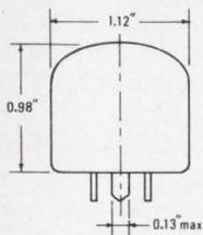
**ORP66:** The ORP66 cadmium sulphide photoconductive cell offers shock and vibration resistance and high sensitivity in a hermetically sealed envelope. It has wide spectral response, peaking at 630nm. It is intended for on-off as well as variable brightness control applications.
