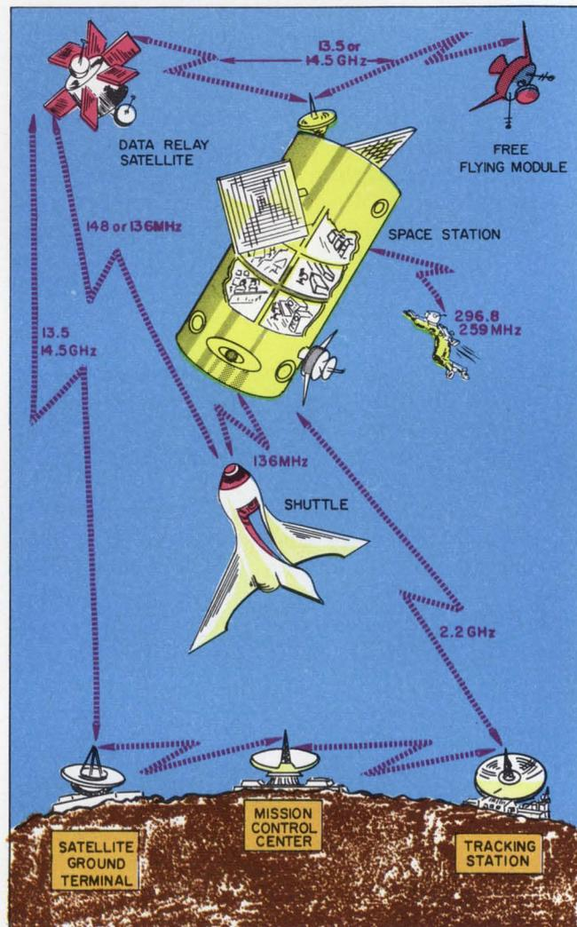
**Twelve-man, earth-orbiting space station will get replacements and supplies via shuttle, communicate by a relay satellite, be equipped with free-flying modules, and permit its scientists to work outside.**
