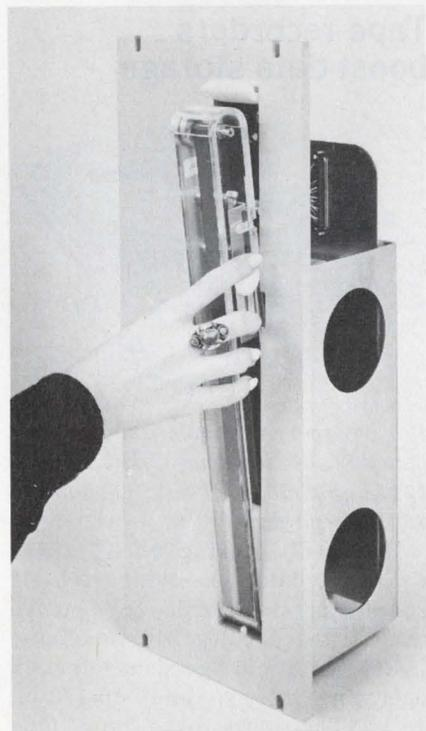
Easy loading, low cost and high density are some of the features of a random-access data storage system. A single tape-loop magazine stores up to 72k characters.
