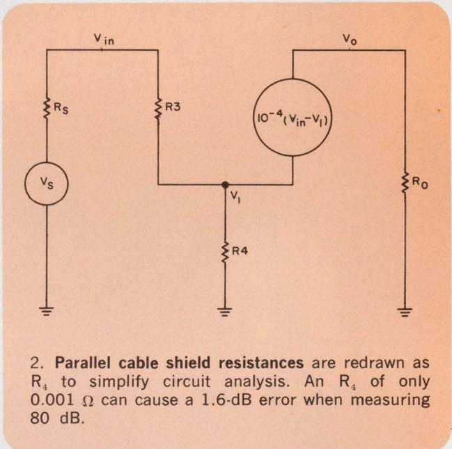
2. Parallel cable shield resistances are redrawn as  $R_4$  to simplify circuit analysis. An  $R_4$  of only  $0.001 \Omega$  can cause a 1.6-dB error when measuring 80 dB.
