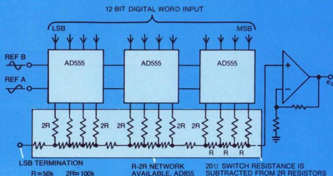
Second in a series of monolithic IC D/A converter circuits, the Analog Devices Model AD555  $\mu$ DAC is intended for applications which require variable reference inputs. This feature permits full 4 quadrant multiplication of the analog and digital inputs, useful in many avionic applications such as digital-to-synchro conversion, digital gain control, etc.
