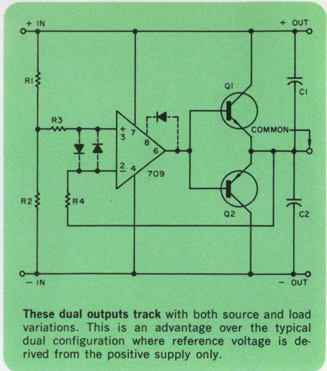
**These dual outputs track with both source and load variations. This is an advantage over the typical dual configuration where reference voltage is derived from the positive supply only.**
