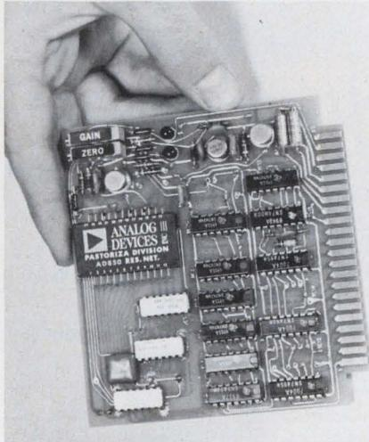
A new successive-approximation 12-bit analog-to-digital converter features a relative accuracy of 0.0125%—including buffer amplifier and comparator errors.
