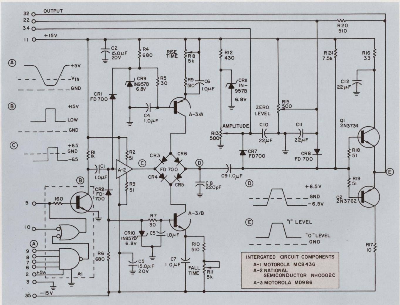
2. The complete circuit can be assembled on a standard 3-1/2-by-4-inch plug-in printed-circuit card. Rise and
