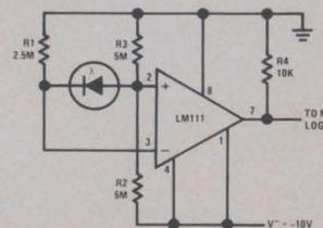
c. Comparator for Low Level Photodiode
