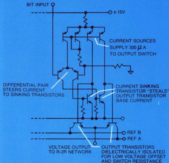
12-BIT MULTIPLYING D/A CONVERTER
