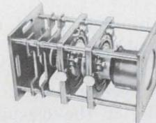
Low cost Coil and Tube positioners provide six independent degrees of freedom for yoke, focus, centering and alignment coils without jump or backlash. Tubes, such as CRTs, Scan Converters, Storage Tubes and Image Intensifiers, are firmly held and may be dismounted without removing the coil assemblies.
