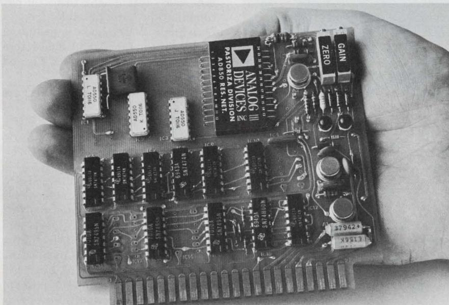
**Precision 12-bit analog-to-digital converter** offers a relative accuracy of 0.0125%. The unit uses monolithic weighted switches and a thin-film resistor network in its d/a section to achieve ultra-stable performance.
