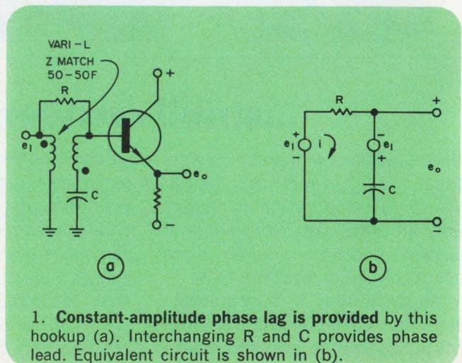
**1. Constant-amplitude phase lag is provided by this hookup (a). Interchanging  $R$  and  $C$  provides phase lead. Equivalent circuit is shown in (b).**
