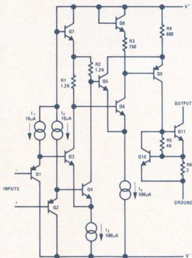
FIGURE 1. Simplified Schematic of the LM111
