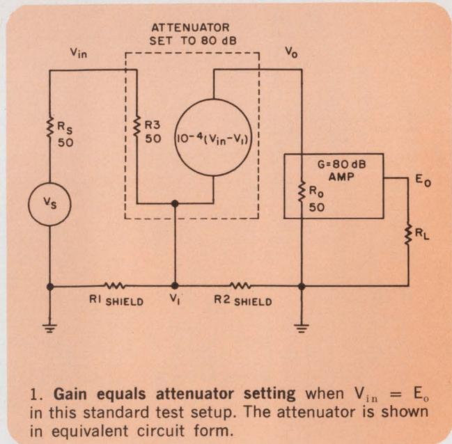
1. Gain equals attenuator setting when  $V_{in} = E_o$  in this standard test setup. The attenuator is shown in equivalent circuit form.
