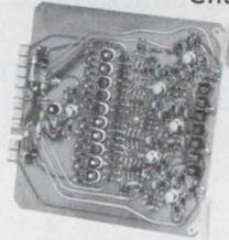
Plug-in cards include generators for dynamic focussing, correction circuits for linearity, regulators for static focussing and centering, and amplifiers for blanking, video, dynamic focussing and deflection.
