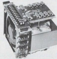
CELCO Deflection Amplifiers assure fast and accurate deflection of the electron beam in CRT or Storage Tube Displays. These all-silicon units, working at up to 120 V p-p can provide as much as 16 A p-p of output current. Features include wide bandwidth with excellent linearity and transient response.
