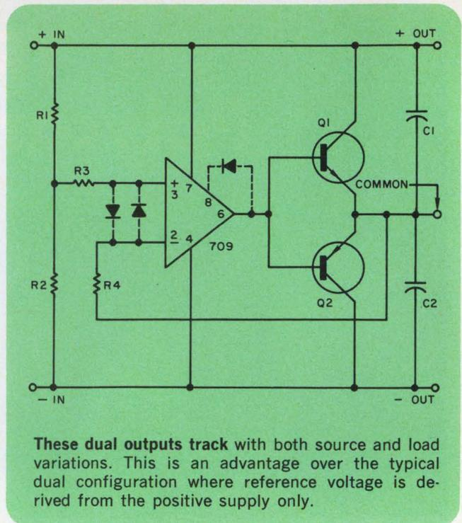
**These dual outputs track with both source and load variations. This is an advantage over the typical dual configuration where reference voltage is derived from the positive supply only.**
