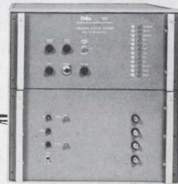
CELCO Precision Display Systems are completely self-contained X-Y monitors with wide bandwidth to 1.0 MHz, linearity to 0.1% and fast slew rates. These flexible
