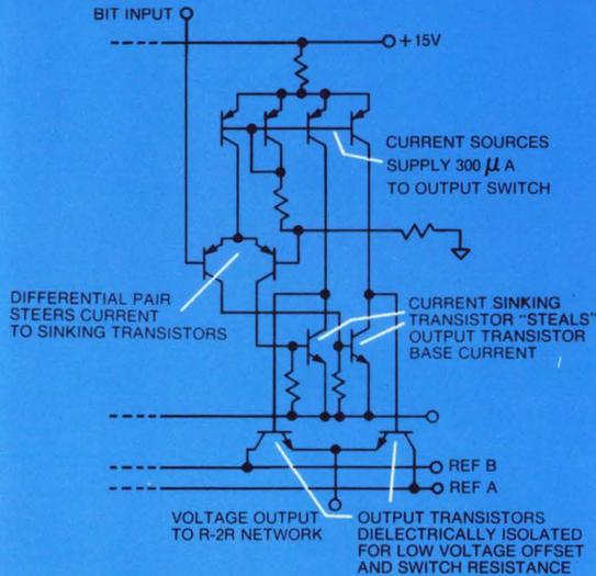
12-BIT MULTIPLYING D/A CONVERTER
