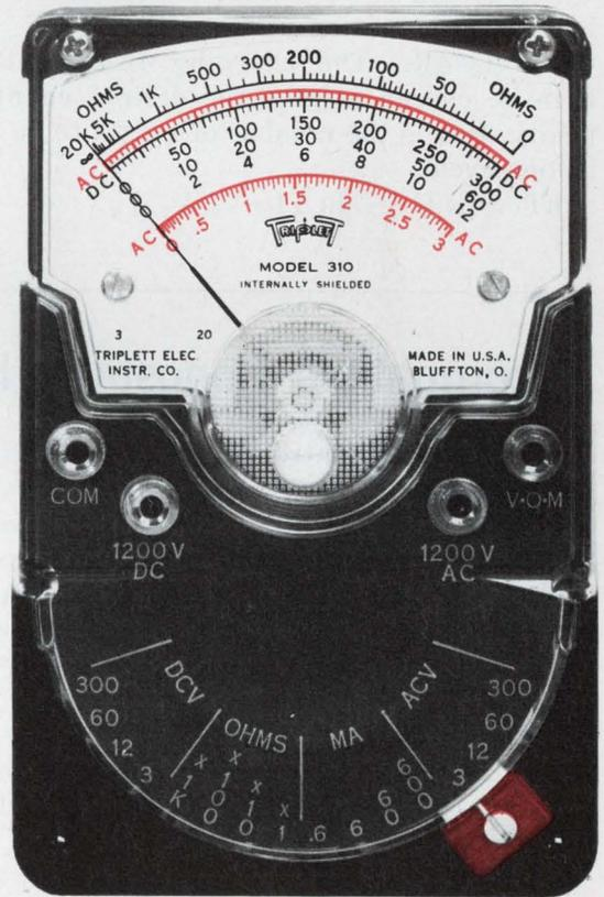
1. Hand size V-O-M with provision for attaching AC clamp-on ammeter.
