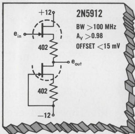
Half the device acts as a current generator for the source follower. Since the FETs are matched to less than 15 mV,  $V_{GS1} = I_D R_1 = I_D R_2 = V_{GS2}$  and near zero offset is achieved.
