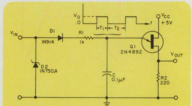
**UJT counter uses zener diode** to equalize input pulses. Capacitor  $C$  must be selected to allow complete discharge during pulse spacing period  $T_2$ . Component values are for a divide-by-7 counter.
