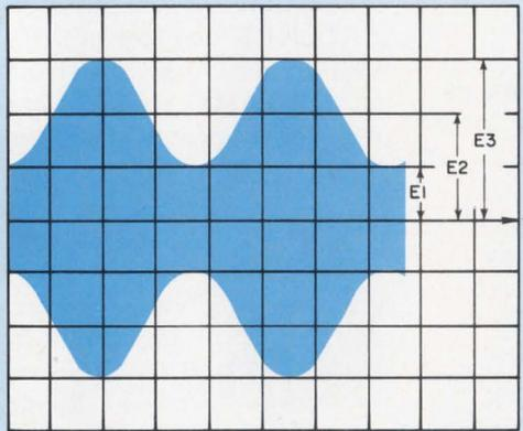
1. Dynamic range information is given explicitly in the time domain. Oscilloscope or power-meter measurements are particularly valuable at low-modulation rates when carrier and sidebands are very close together.
