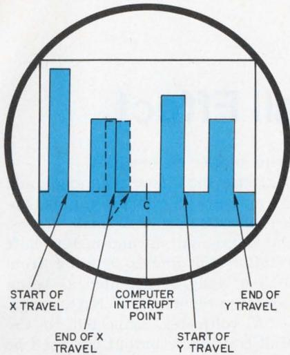
Real-time examination of machine tool travel, the way Autovue might show it. Under normal conditions, the X and Y rate of travel would be the same (solid trace). Improper lubrication, a faulty bearing or dirt might cause the travel to be reduced (dashed line). Maintenance personnel could observe this and schedule service. The computer interrupt would stop the process automatically if the operation degraded to that point.
