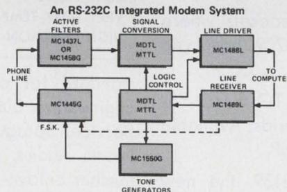
**Frequency-Shift Keyer . . .** The MC1445G is a dual-input, logic-controlled tone switch that can connect either of two tone generators to an output line. It also has a low-impedance emitter-follower output stage.
