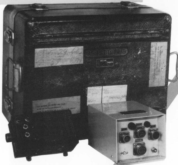
This fiberglass case, designed and manufactured by H. Koch & Sons to house the instruments shown in front of it, was shipped from Dayton, Ohio, in October, 1951, and arrived back in Dayton in June, 1952. During this eight months it travelled a total of 19,000 miles by rail, air, boat and truck including three months storage in Panama. (The route is shown on the map.) At the end of the odyssey, both the instruments and the case were in perfect condition.
