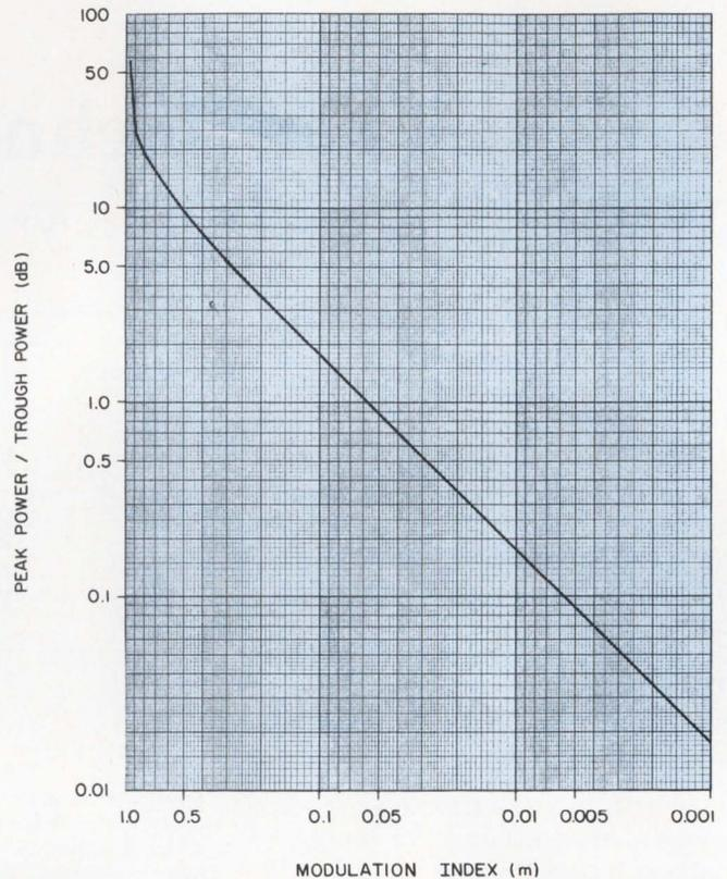
2. When a power meter is used to make time-domain measurements, this plot of peak-to-trough power ratio vs modulation index is a convenient tool. The power ratio is measured in decibels.
