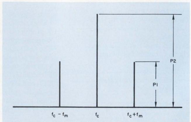
3. Bandwidth data stares at you from the face of a spectrum analyzer display. This frequency-domain measurement is probably the easiest to perform as long as the sidebands are clearly separated from the carrier.
