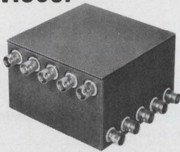
Model SMR-55HA is a computer compatible 5 x 5 building block device. Permits hot switching to 3W and 100% random access. Hermetically sealed reeds are used in a broadband stripline matching structure.
