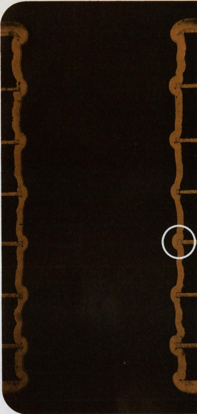
Left: Cross-section (enlarged 70 diameters) of plated hole through typical 8-plane Collins etch-back circuit board.
