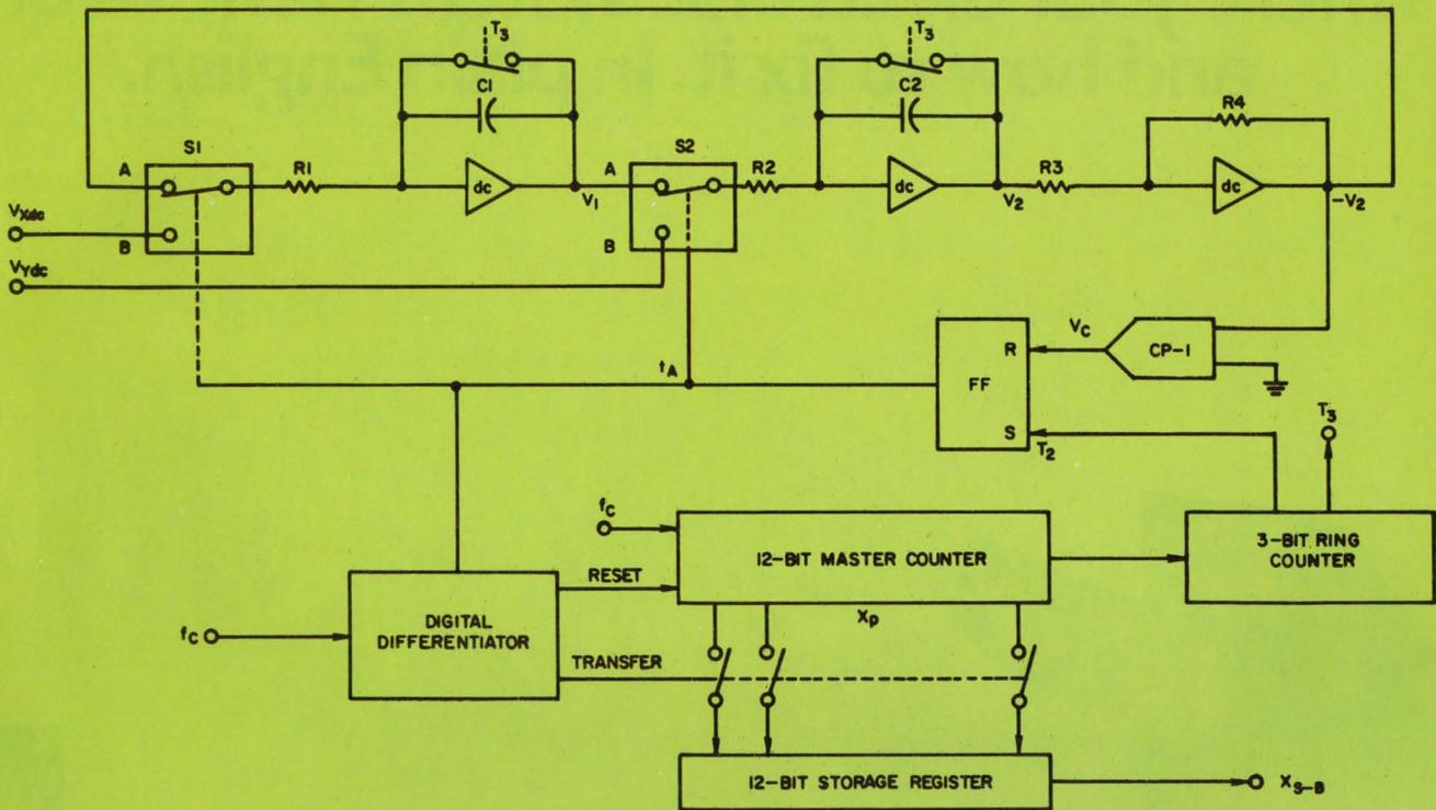
34. The Type V converter is controlled by a 12-bit master counter. Integration time constant dependence
