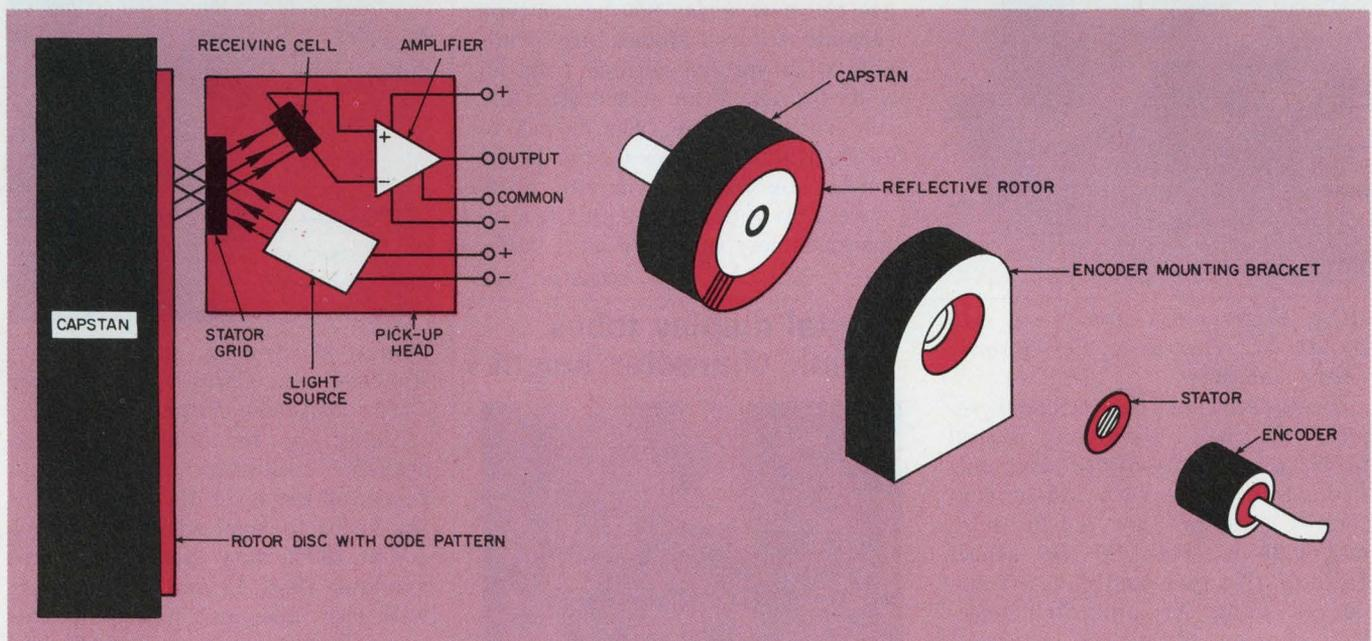
**Reflective-surface rotary encoder** permits digital speed control without increasing mass or sacrificing acceleration time. Code pattern on reflective plastic disc is
