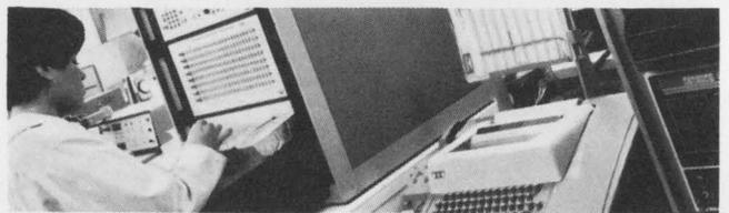
National's array of J259's handle the testing of its digital IC's smoothly and economically. For its linear-IC testing, National has turned to Teradyne's J263 computer-operated linear-IC test system.
