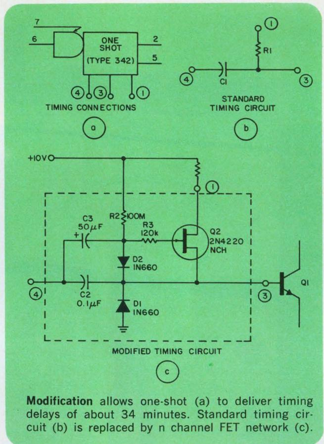
**Modification** allows one-shot (a) to deliver timing delays of about 34 minutes. Standard timing circuit (b) is replaced by n channel FET network (c).
