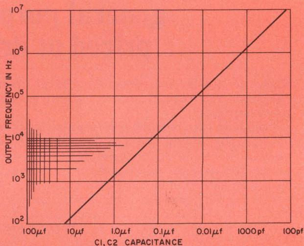
2. Linear relationship exists between capacitance and frequency for a wide range of capacitor values.
