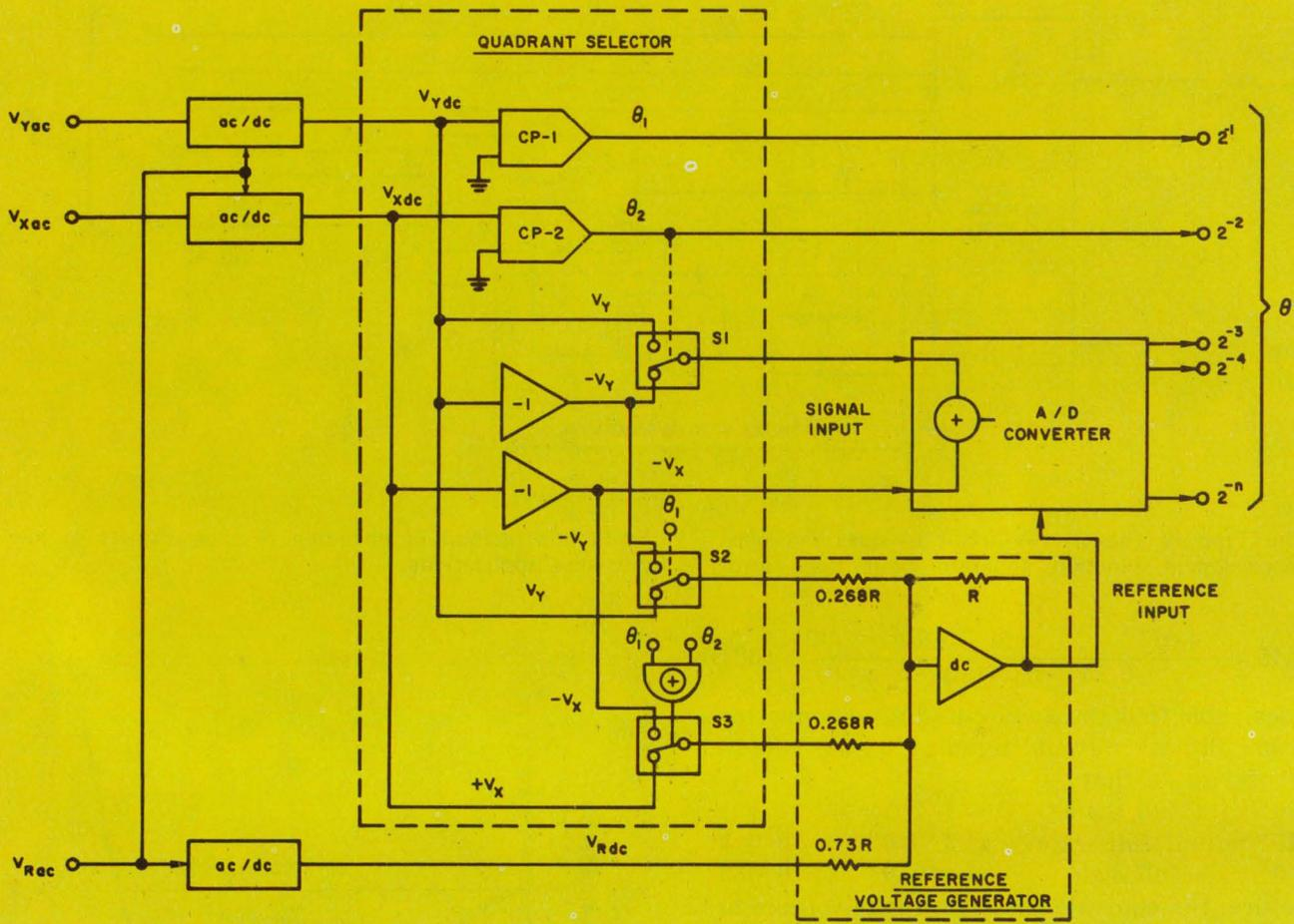
30. A reference voltage generator is used in the Circuit II design. Thermally induced variations in the transfor-
