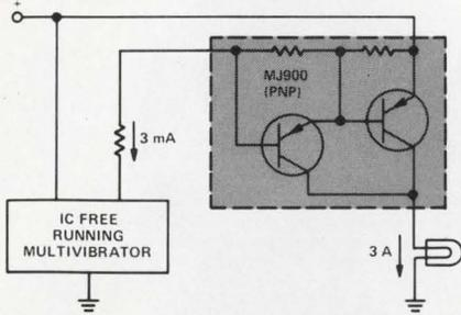
**Innovate With I/C's.** Drive the 3 A darlington with power levels derived from integrated circuit logic gates. Go from milliamperes to amperes directly, compatibly, easily.
