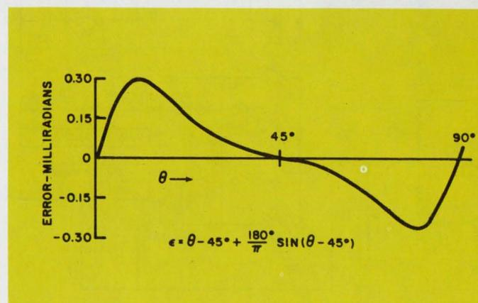
29. Greater precision is theoretically available from the Type IV converter—Circuit II. Error between  $\theta$  and its approximation (Eq. 59) from  $0^\circ$  to  $90^\circ$  is  $< 1.0$  minute of arc.
