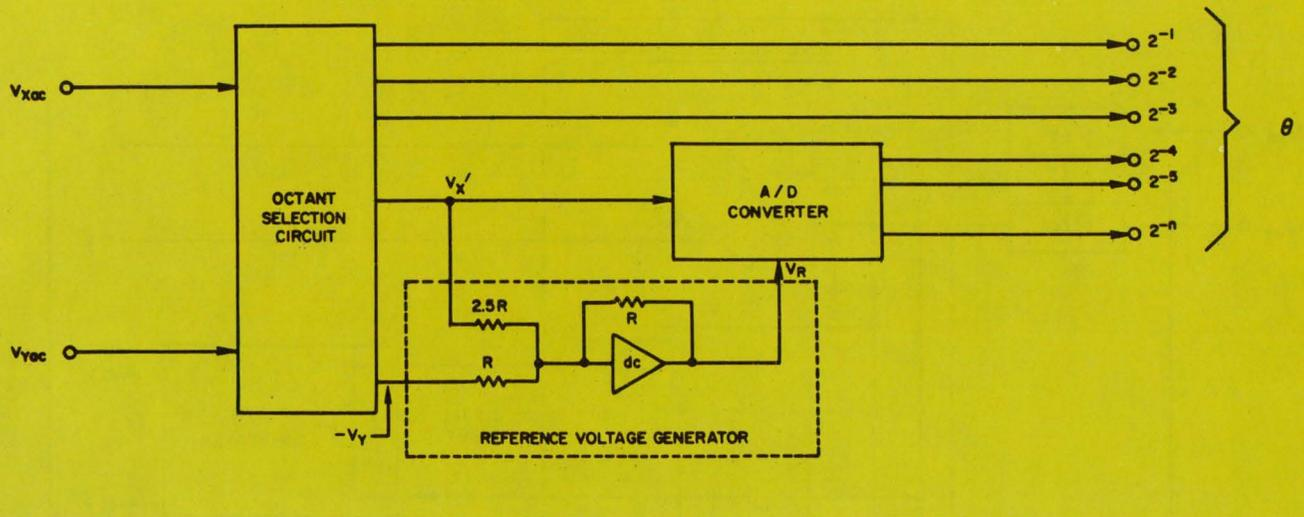
27. The Type IV converter—Circuit I—does not need a linear-segment function generator, but large error
