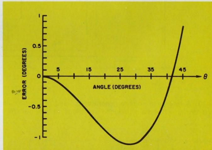
28. The accuracy of Circuit I is the difference between  $\theta$  and its approximation,  $\sin\theta/(\cos\theta + K \sin\theta)$ . Maximum error from  $0^\circ$  to  $45^\circ$  for  $K = 0.25$  is  $< 1.2^\circ$
