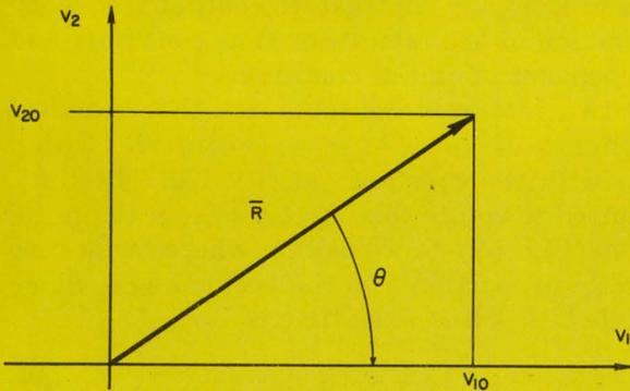
33. The imaginary vector  $\bar{R}$  has the two integrating capacitor voltages  $V_{10}$  and  $V_{20}$  as components.  $\bar{R}$  rotates with a constant velocity,  $K\omega$ .
