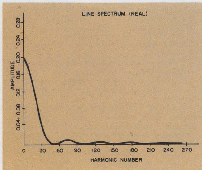
3. The real line spectrum of a triangular wave is plotted from the transform of the time function.
