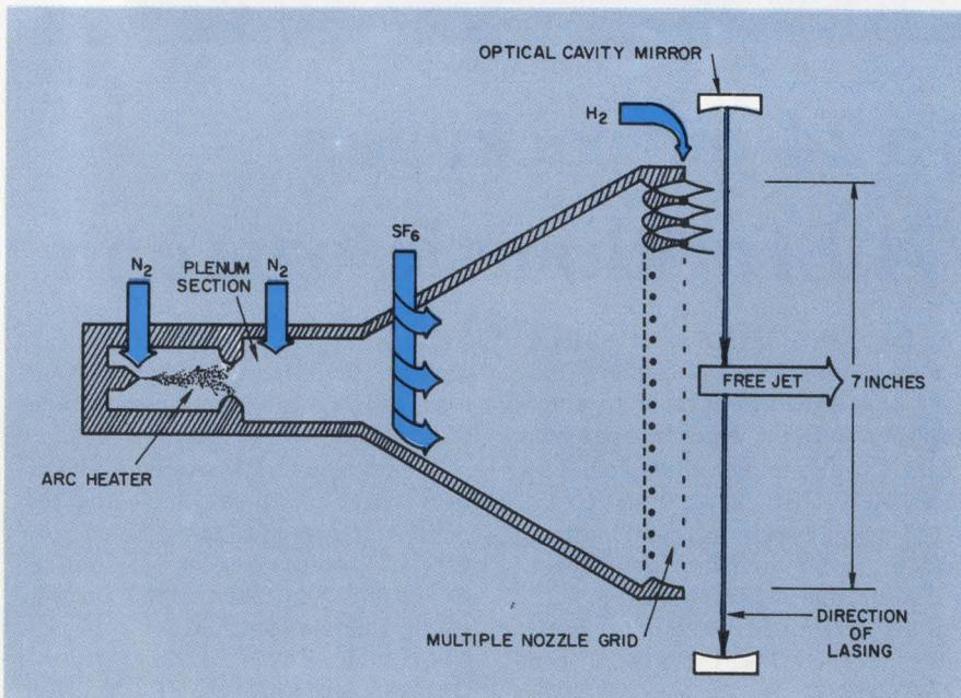
Cw chemical lasing can be achieved through the above scheme. Sulfur fluoride is injected into hot nitrogen, causing the fluorine to separate out. Hydrogen is mixed with the fluorine atoms to create vibrationally excited hydrogen fluoride. The hydrogen fluoride passes through an optical cavity at supersonic speed and changes state, causing lasing in the cavity. Light is given off at 2.6 to 2.9 microns.
