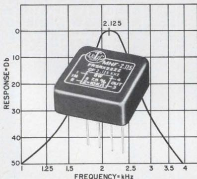
Designing for modem applications? You'll find this MNF 2.125 band-pass filter precisely what you need. It has a center frequency of 2125 Hz and a pass band from 2025 to 2225 Hz within 1 db. Impedances are 10K ohms source and load.
