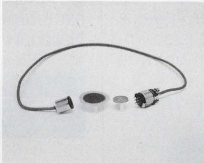
A new incremental optical encoder with a remote reflective disc controls speed digitally without adding mass. It eliminates the need for shaft couplings and extra bearings.
