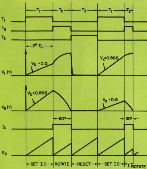
35. Operation of the Type V converter is divided into three modes.  $T_1$  sets initial conditions,  $T_2$  rotates vector  $\bar{R}$ ,  $T_3$  resets integration capacitor voltage to zero.
