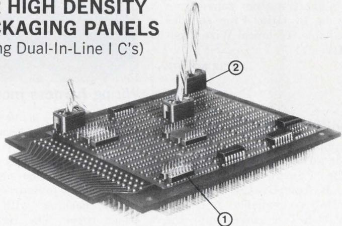
Provide greater flexibility in prototyping and packaging. Facilitate interposing of discrete components. Plugs have 14 and 16 leads with pins on .100" centers and .300" between rows.
