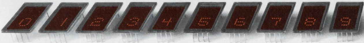
For \$25 each in 1 K lots, HP sells you a hermetically sealed, IC-compatible display with on-board decoder-driver. You just plug the module in; it accepts direct 4-line BCD input. You also get a 5 x 7 dot matrix character that prevents ambiguous readings and a parallax-free design in a package that's one inch high and practically flat. It's the brightest display idea since the tube.
